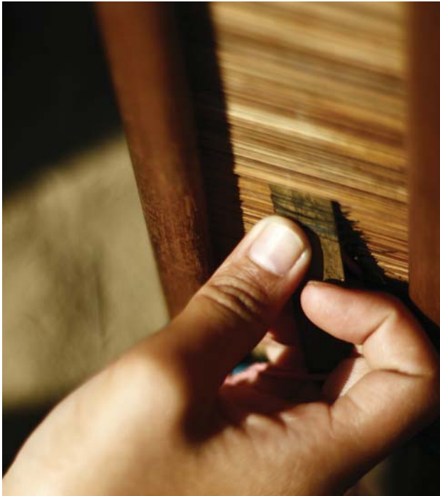
A device created by Tai Phakes made of bamboo and wood which they use to keep threads separated in weaving process.
