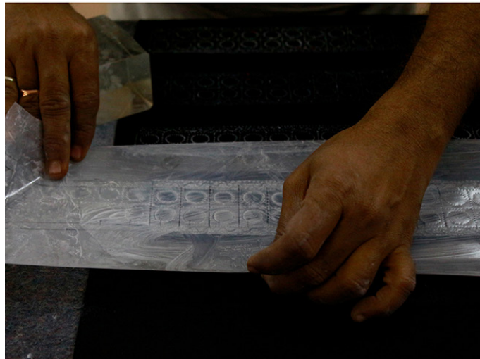
The mixture of kerosene and chalk powder is applied on pierced gateway sheet.
