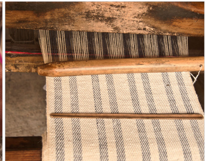
Small piece of bamboo pole used as fly-shuttle.
