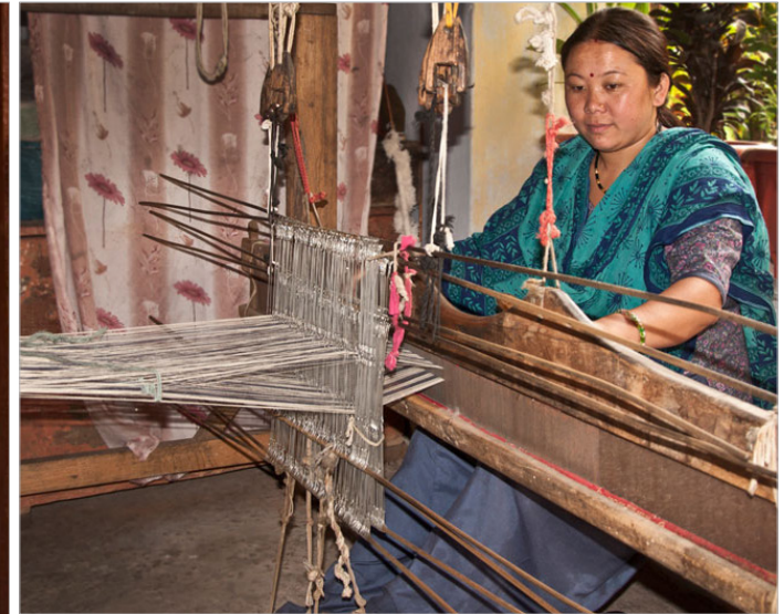
Weaving is done using traditional pit loom..
