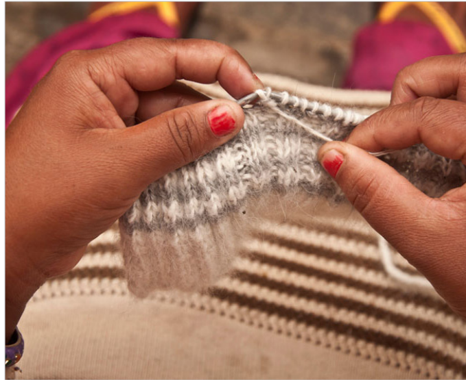
The new loop is pulled based on immediate existing loop.
