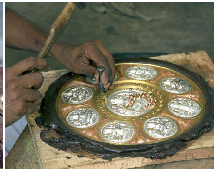
Fixing the beads by hammering.
