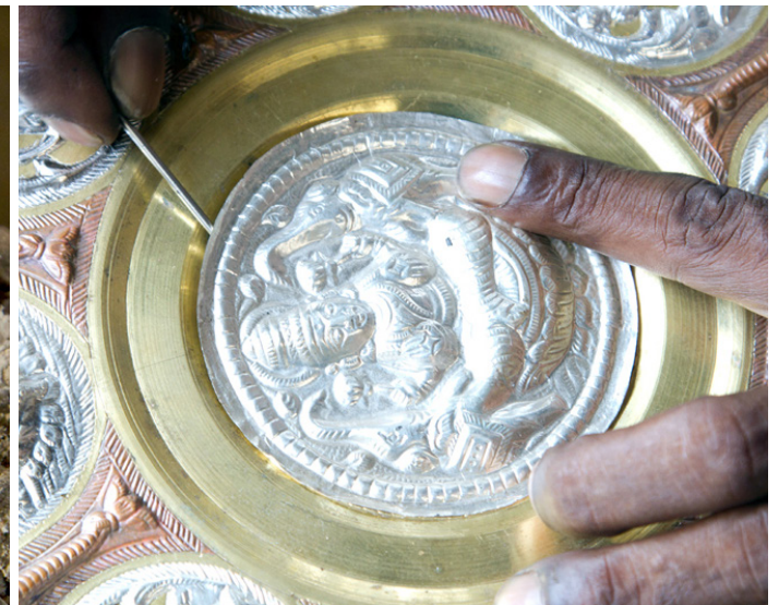
Natural glue is melted and filled inside the carved sheet. Silver sheet is being fixed with glue.
