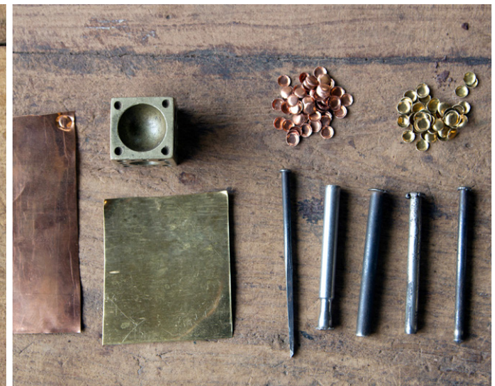
Copper and brass metal sheets used to create the beads.
