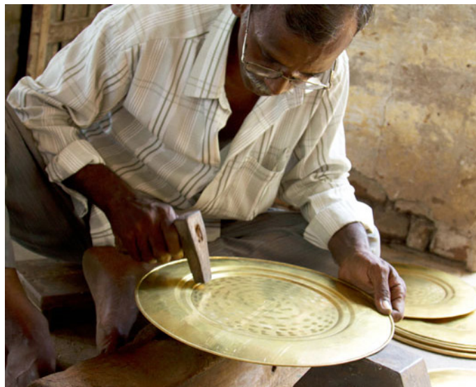
Beating the plate with hammer to obtain depth.
