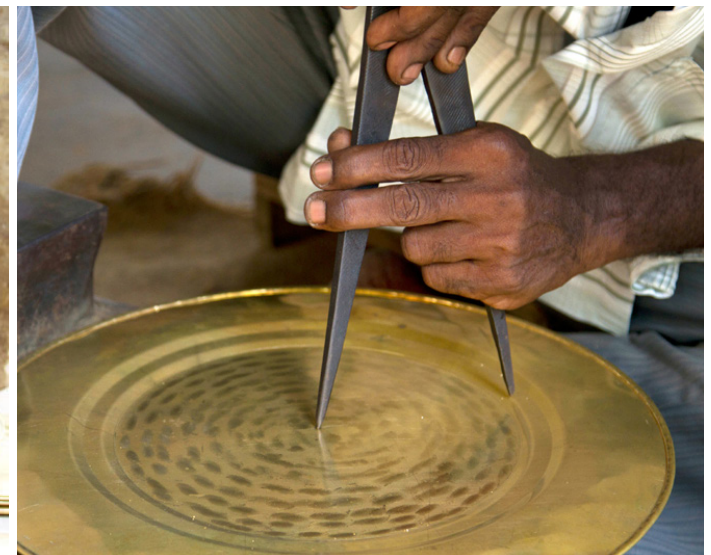
Compass is used for accurate measurement.
