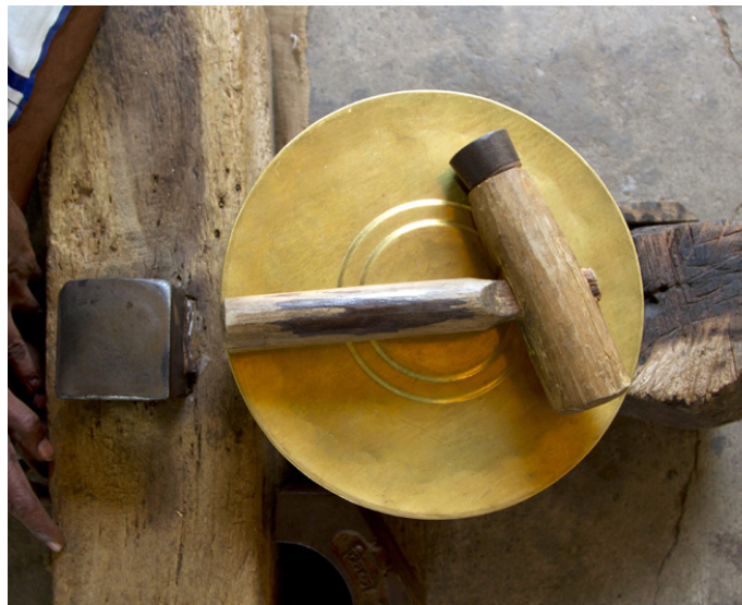
Hammer used to create the patterns over the plate.
