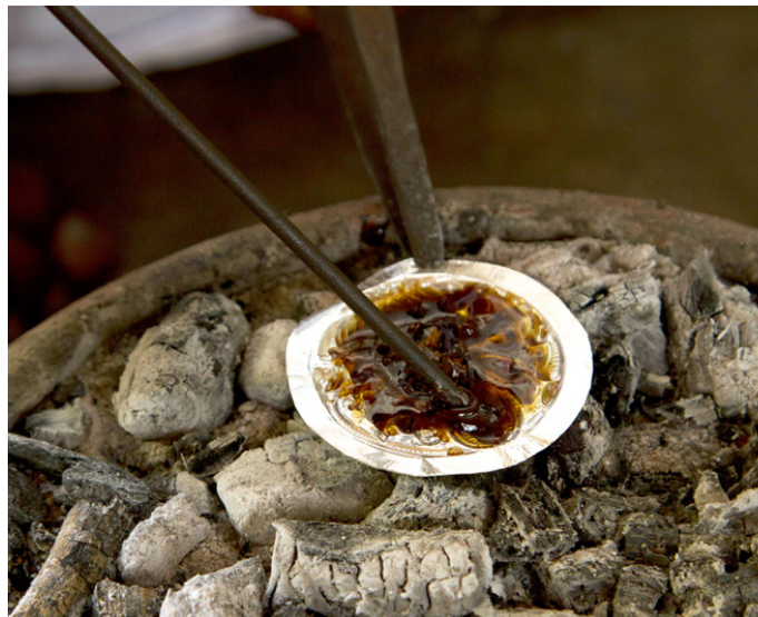
Natural glue is melted and filled inside the carved sheet. Silver sheet is being fixed with glue.
