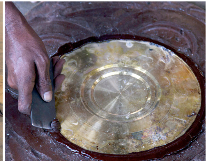
The excess lac covered on the plate is removed.
