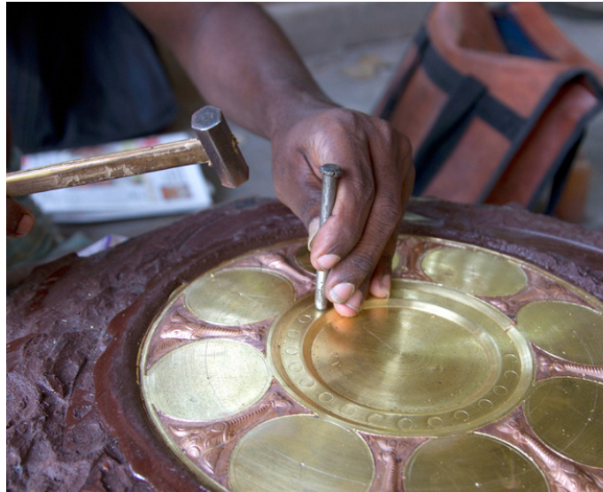
Engraving the rough design on the plate.
