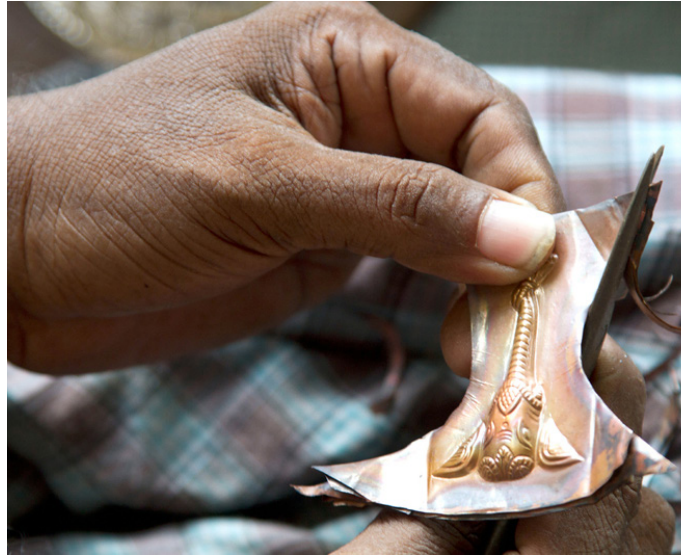
The excess copper sheet is cut.
