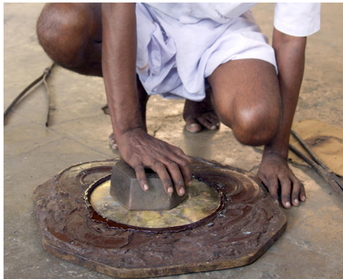
The weight pressed on the plate for proper fixing.
