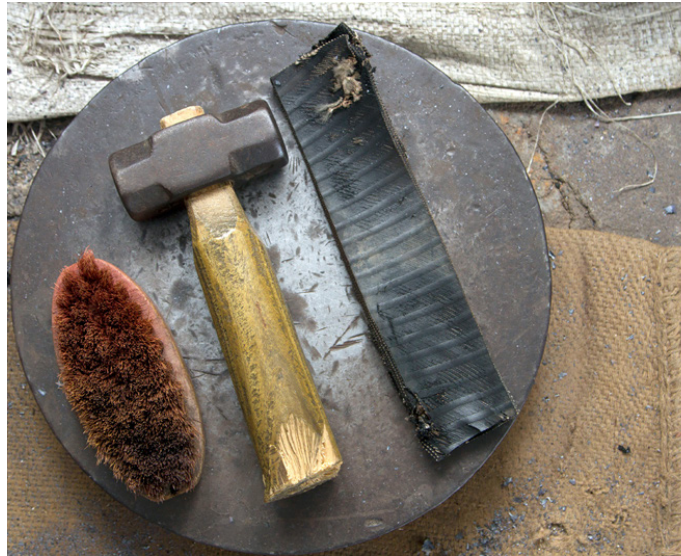
Rubber sheet used to hammer the product.
