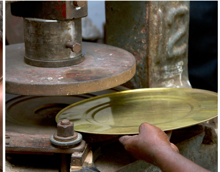
The plate is being removed after the initial shaping process is complete.
