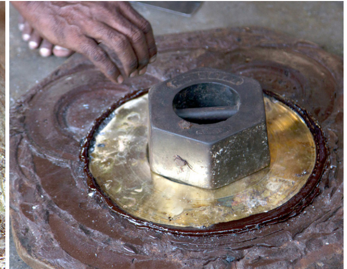
The plate is pressed on the lac with the help of heavy weight.
