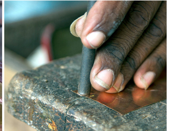
The metal sheet is punched to cut the small circular beads.
