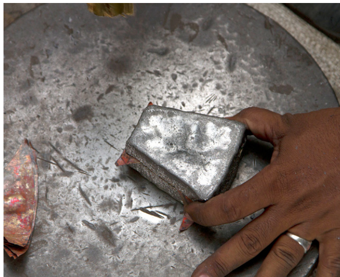
The copper sheet is placed between the moulds.
