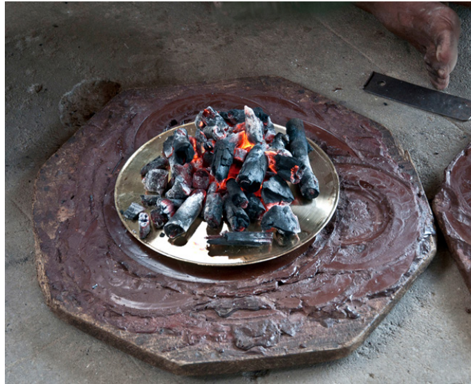
Charcoal is filled on the metal plate.
