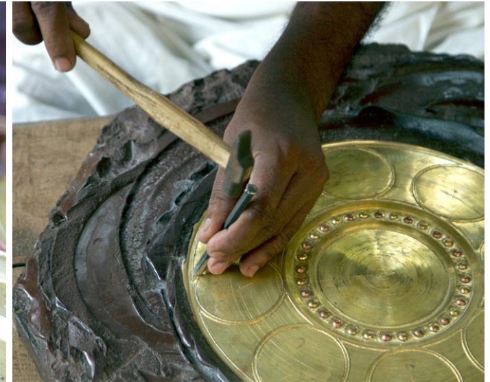
Engraving the circles to fix the copper and silver motifs.
