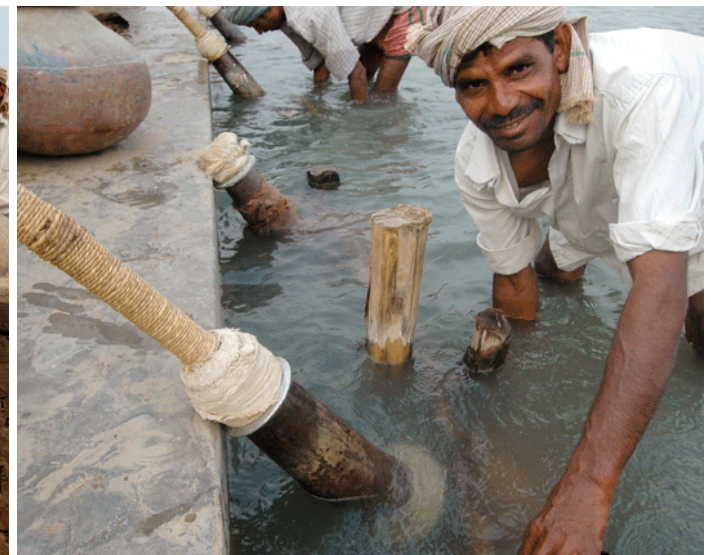
The vessel at the other end of the tube in which the 'attar' is collected.
