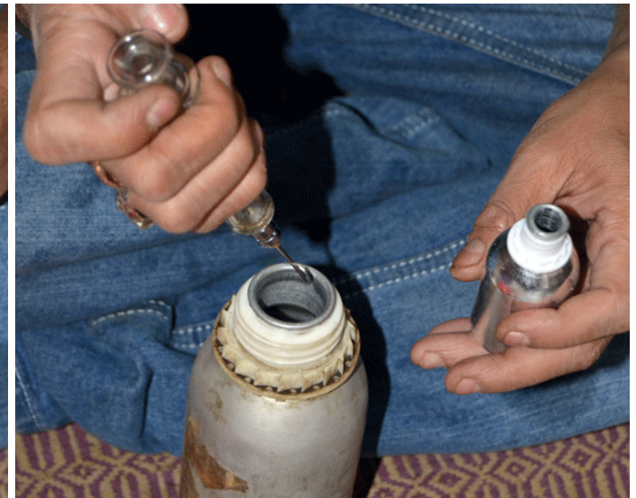
'Attar' being sucked into the syringe, to be poured into glass bottles.
