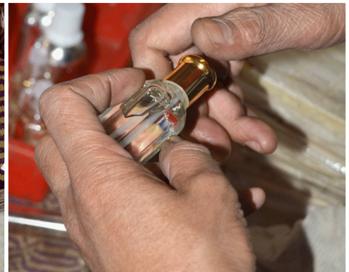
Metal caps being wound onto the glass bottles.
