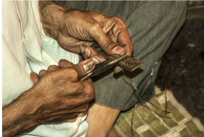
Gauge plate is used to convert the wire into thin string.
