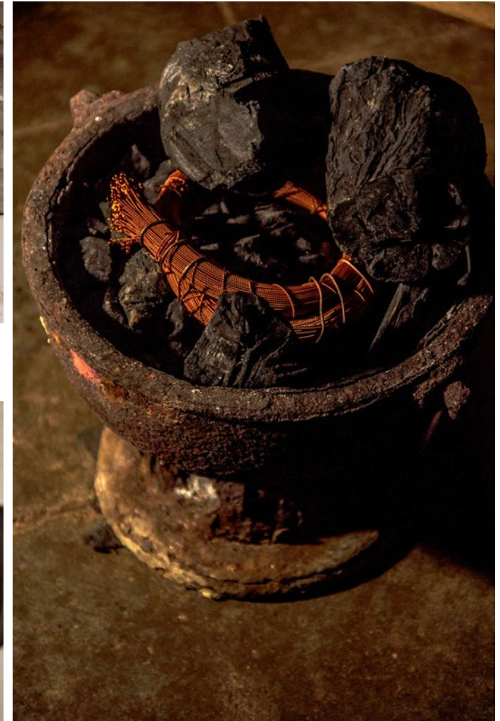
Brazier is used to heat the twisted copper wire to remove chemical coating.
