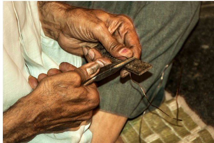
String is pulled through the gauge plate's holes using long nose plier.
