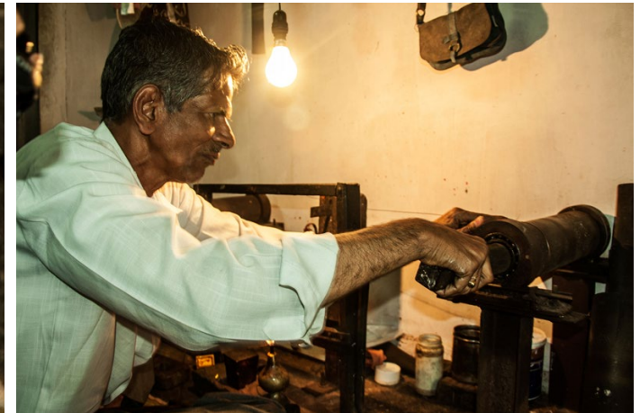
Metal wire is rolled traditional machine called as Ghad using lever.
