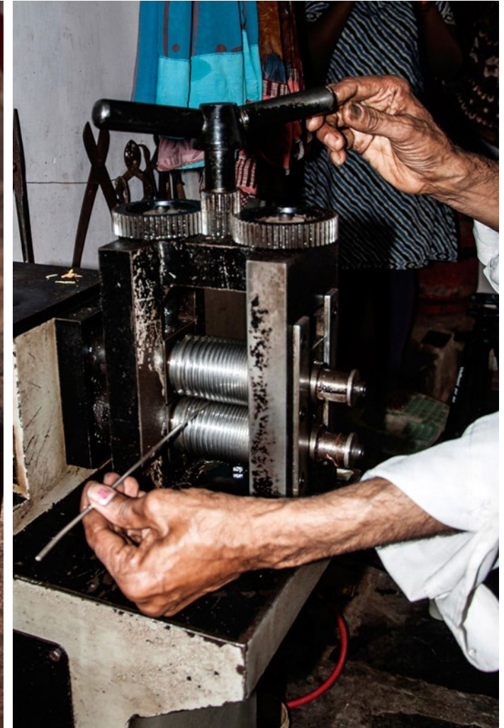
The rod is passed through the rolling machine to convert into a wire.
