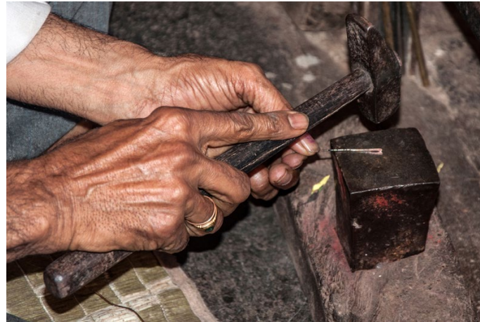
The edge of the wire is hammered to make the edge sharp and pointed.
