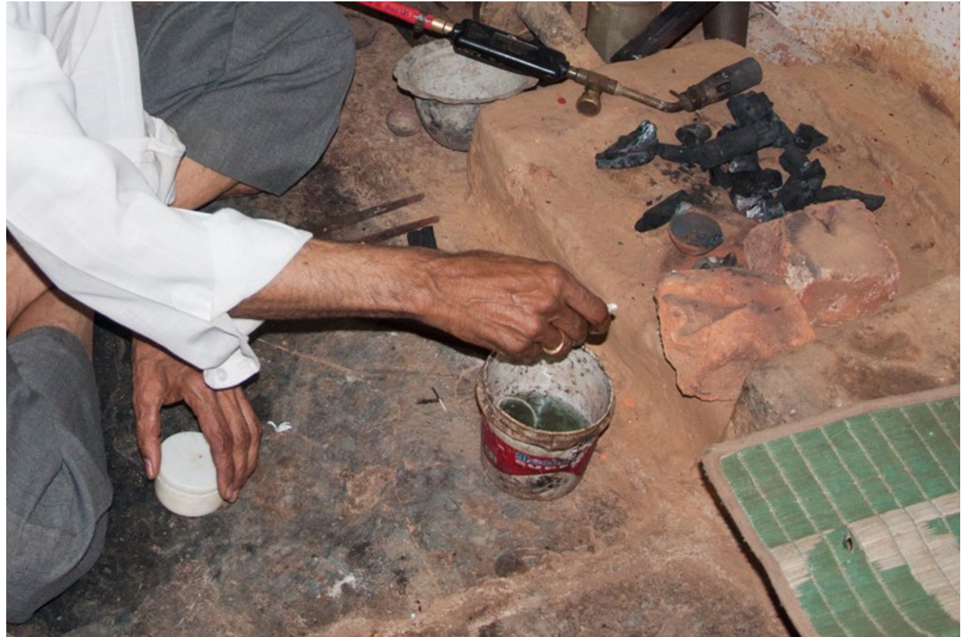
Rod is dipped in diluted sulfuric acid to remove impurity's.
