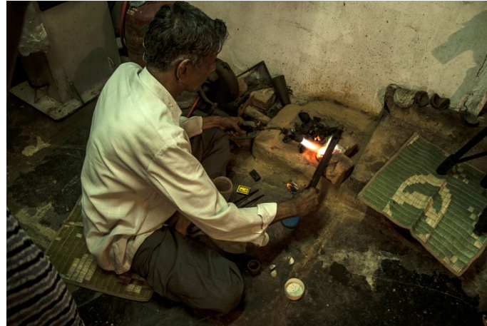
The metal is heated with the help of a flame torch.
