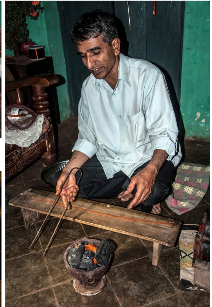
Brazier is used to heat the twisted copper strings to remove the chemical coating.
