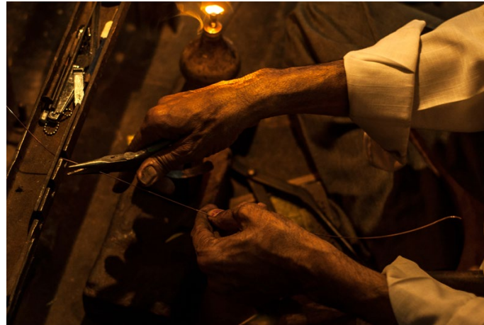
Metal wire is drawn until the required thickness of the string is obtained.
