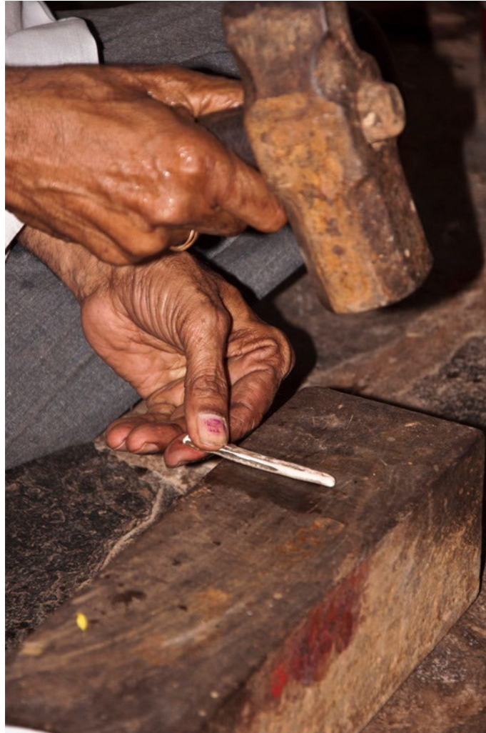
The rod is hammered to expand the length.
