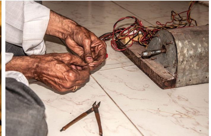
The string is folded and attached to a twisting electric motor.
