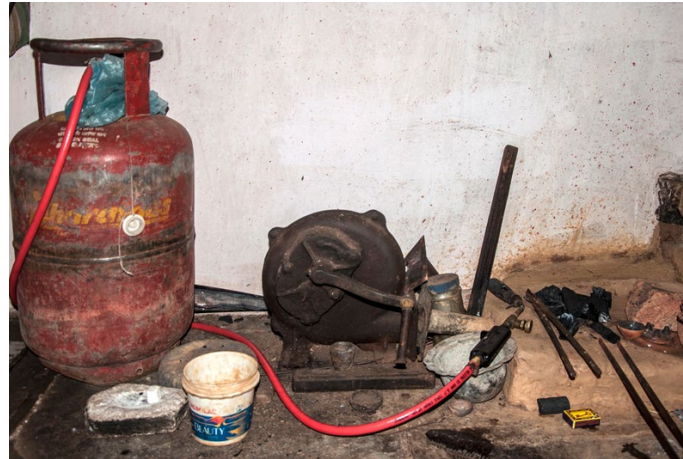
Manual blower and torch is used to produce the fire.
