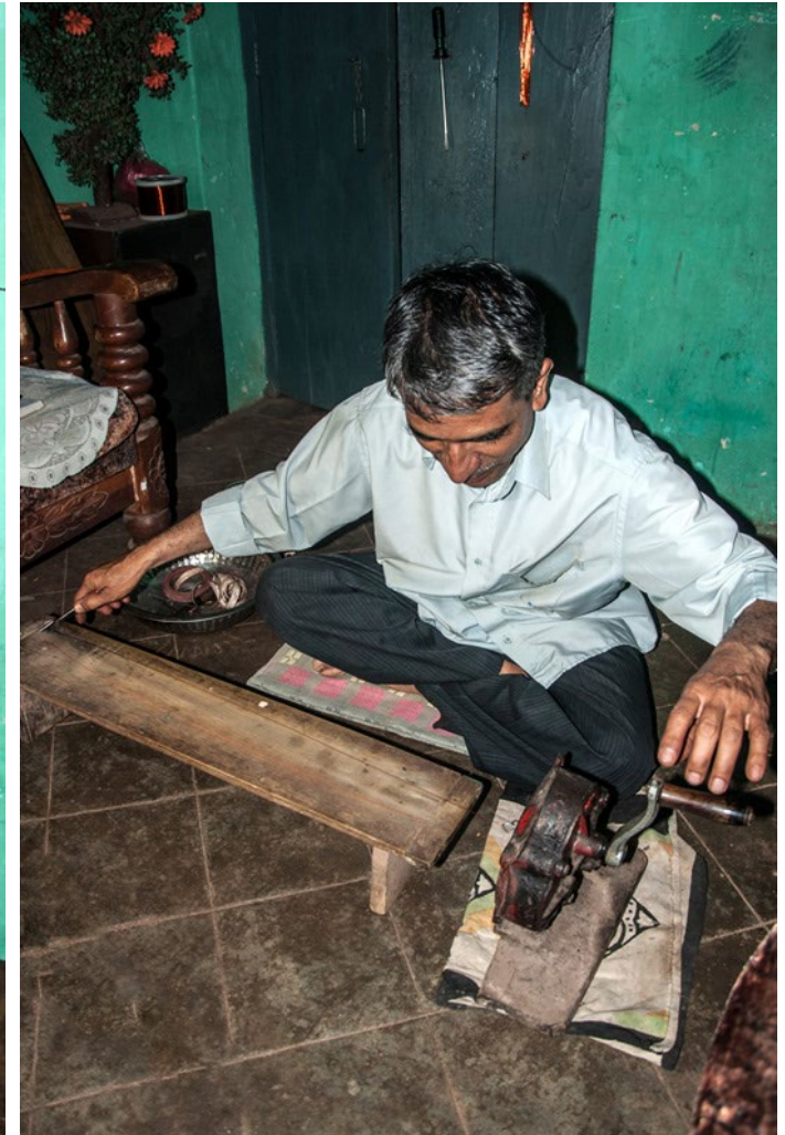
The 64 inches of copper wires are folded into half and twisted using the hand twister.
