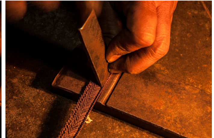
Sides of the knitted Baajubhand are hammered with a flat chisel for embossing the corner.
