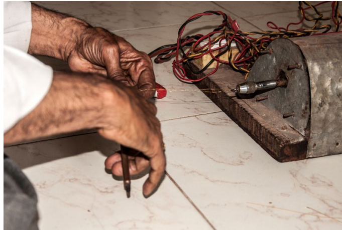
Wire is attached to an electric motor for the twisting.
