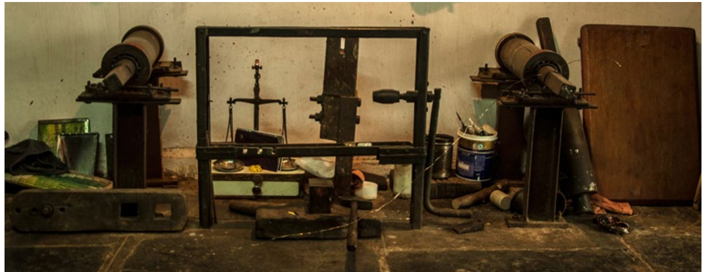
Traditional machine called as Ghad is used to convert the wire into thin string.
