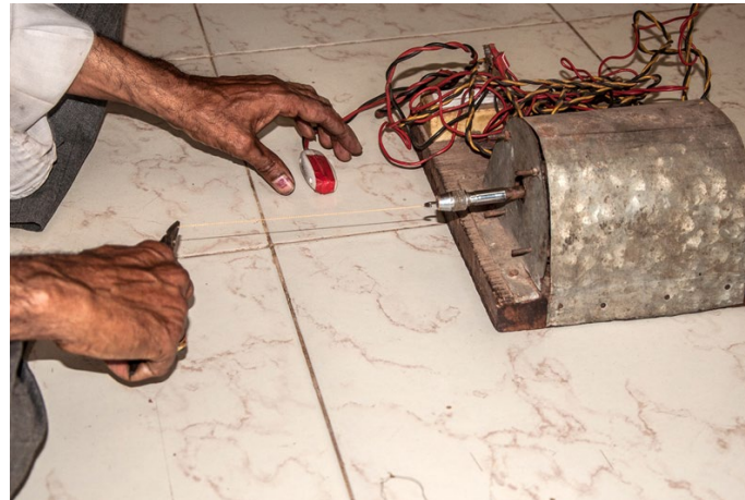
Strings are twisted using the electric motor.
