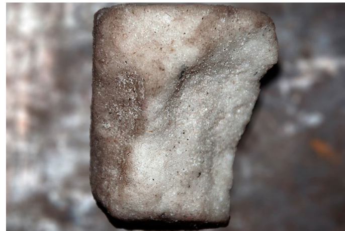
Navasagara powder act as catalyst in melting process.
