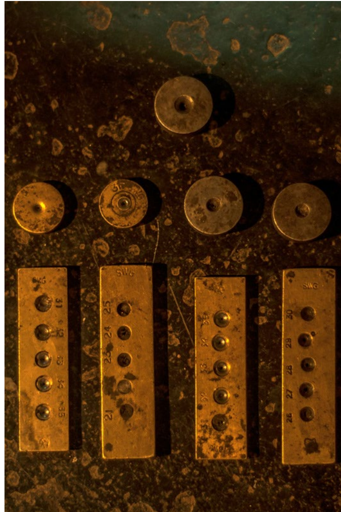
Different size of gauge plate is used to convert the wire in to required diameter of string.
