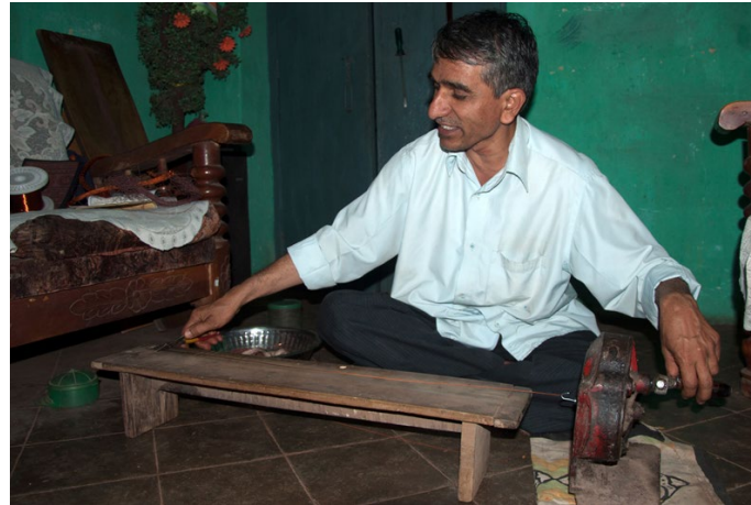
The twisting process reduces the length of the string 6 inches.
