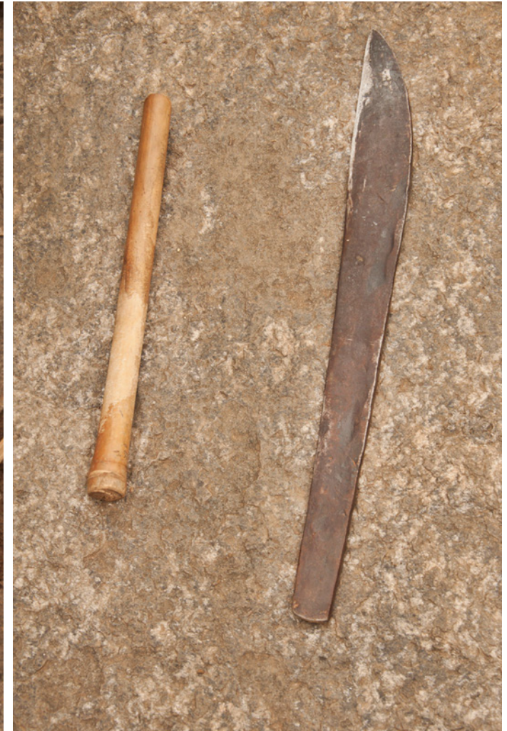
Khurpi (knife) is used to cut the bamboo and Belan (wooden stick) used as support to the knife while peeling the outer skin of bamboo.
