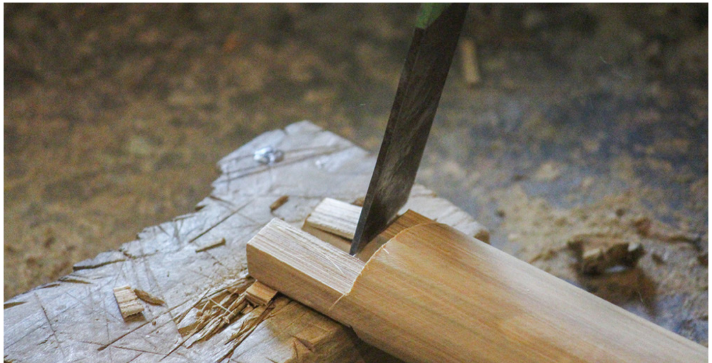
The bamboo is cut at an angle to make a holder.
