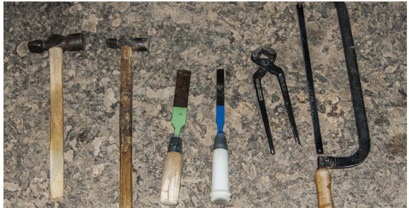
Hammer, Chesil, nail plier and hawk saw blade are used to cut the bamboo to required shape and size.
