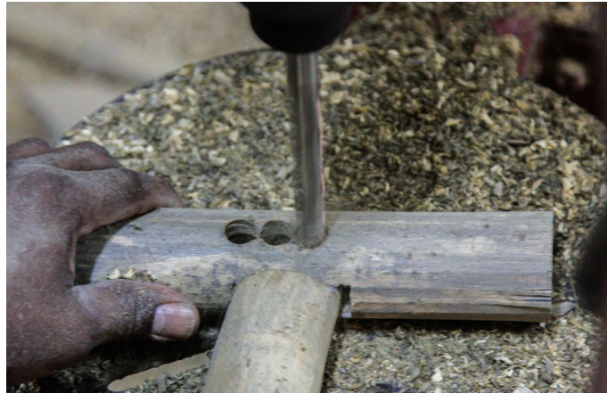
Holes are made on frame to using drilling machine.
