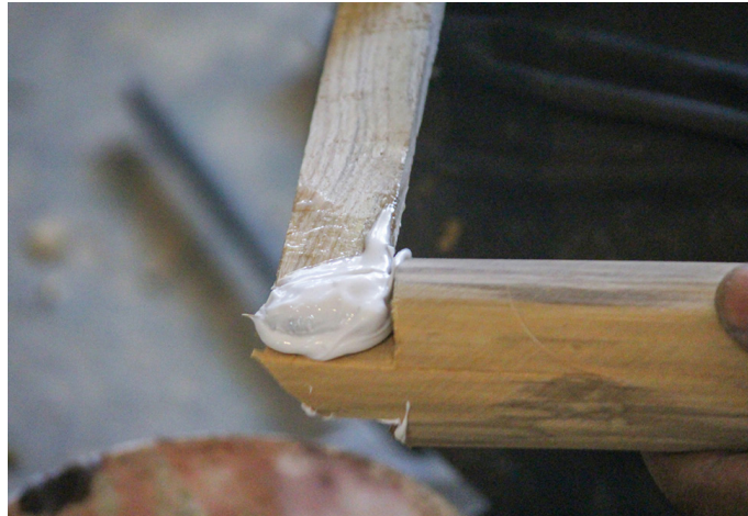
Fevicol is applied on the holder of the bamboo.
