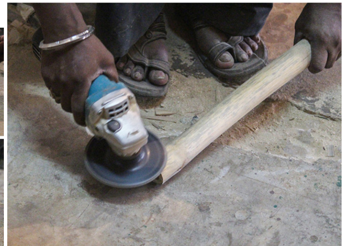
Using buffering machine the bamboo is smoothen on the surface.
