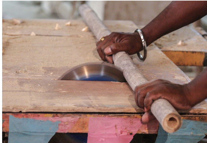
The bamboo is cut into required size using a saw machine.
