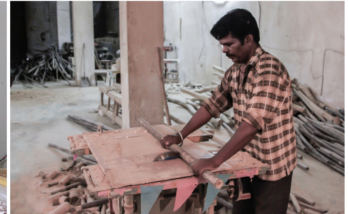
Mr. Asit kumar saha, technical consultant of jute service extension center. Skilled artisan cutting bamboo in required length.
