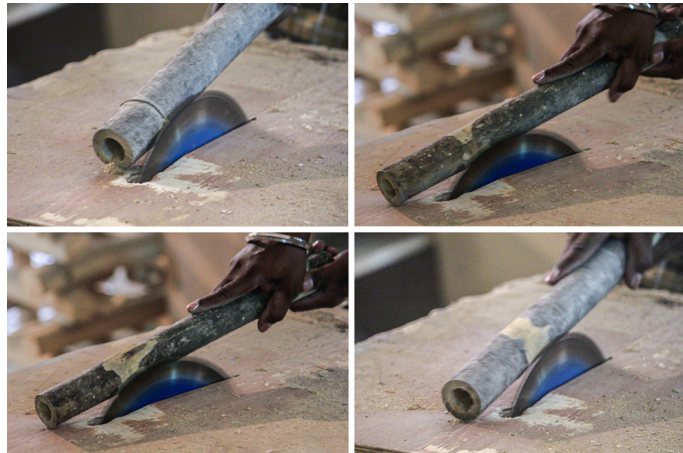
The nodes are removed from bamboo.
