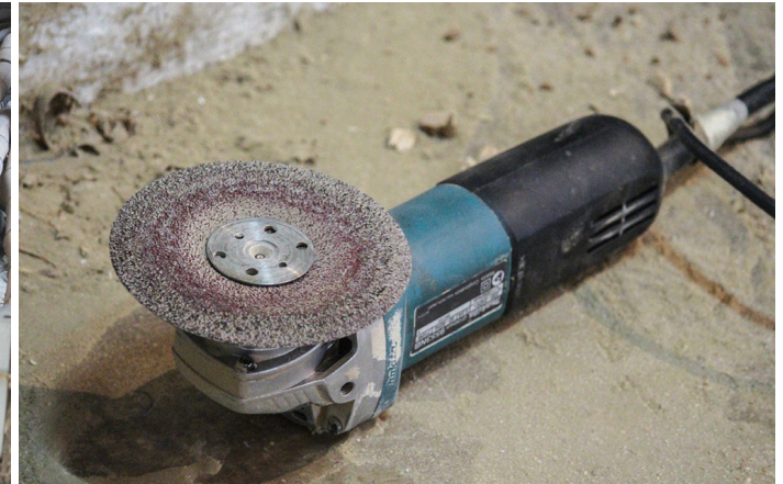
Buffering machine used to smoothen the surface of the bamboo.
