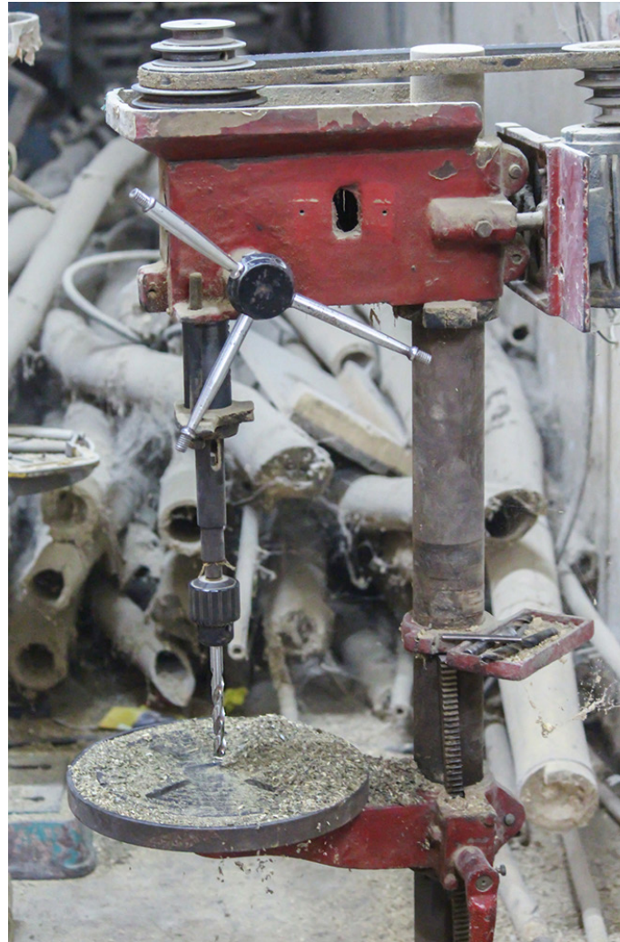
Drilling machine is used to make holes on bamboo.
