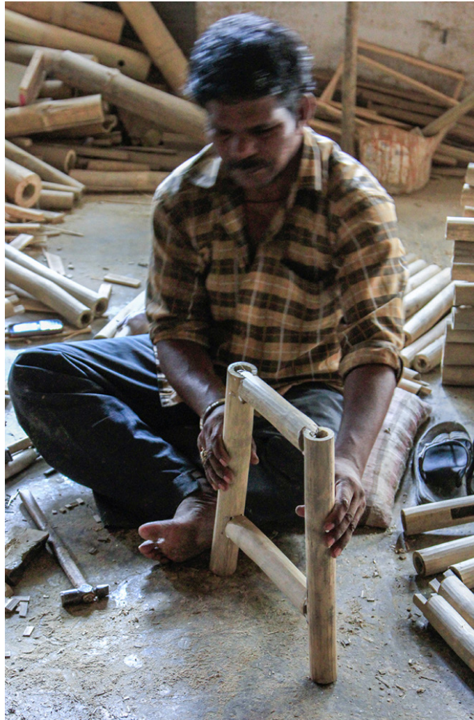
Bamboos are assembled together to make frame.
