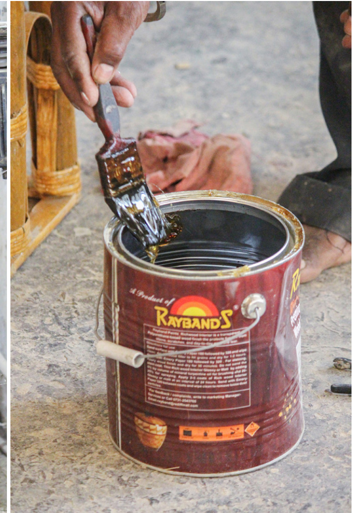
Varnish is applied on bamboo to give a glossy finish.
