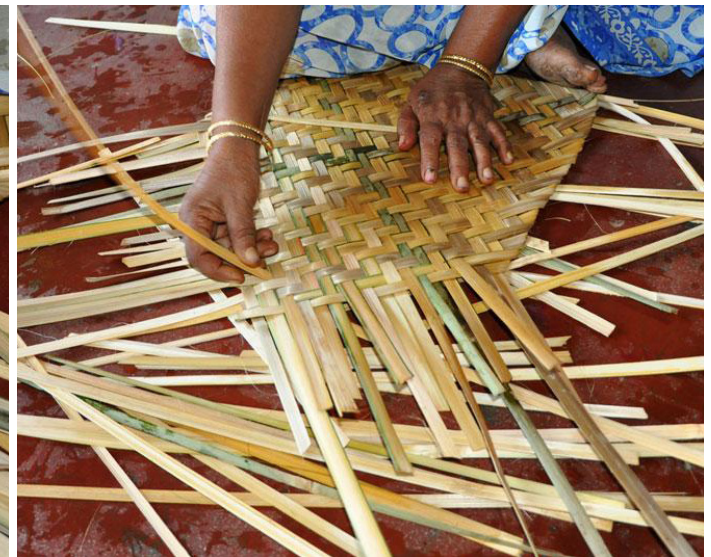
The extra bamboo strips are left to make handle of sieve.
