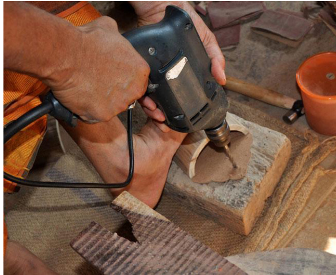
Drilling tool to make holes.
