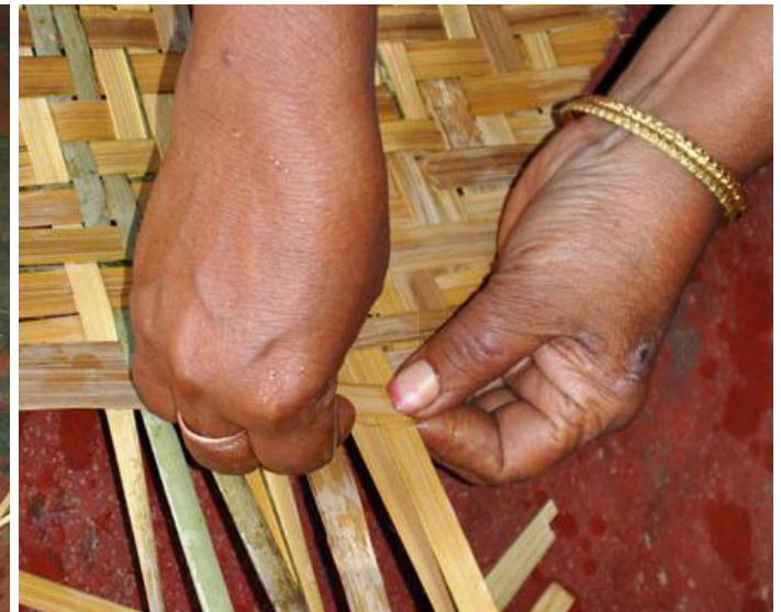
Artisan arranging bamboo splits to start weaving.
