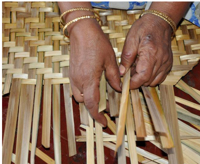
Artisan weaving the base of sieve.
