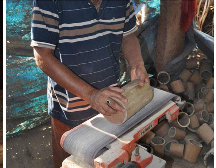
Polishing machine used in bamboo smoothing process.
