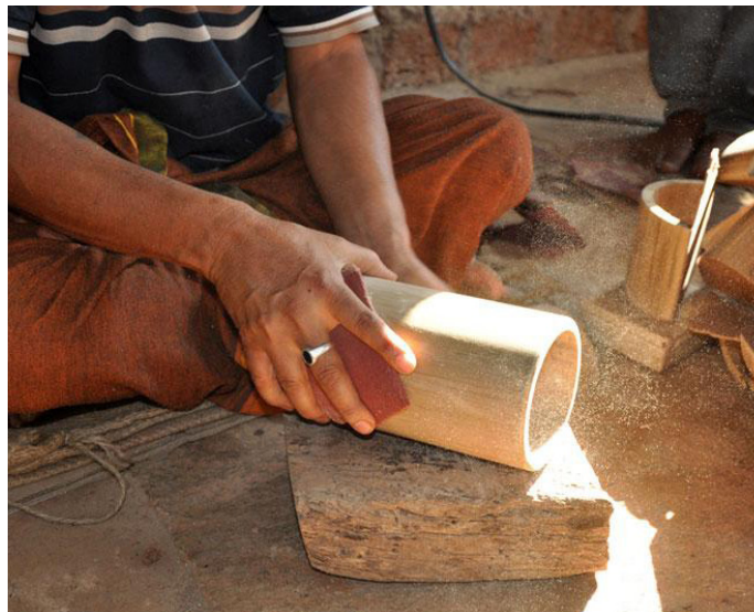
Rough surface is manually smoothed.
