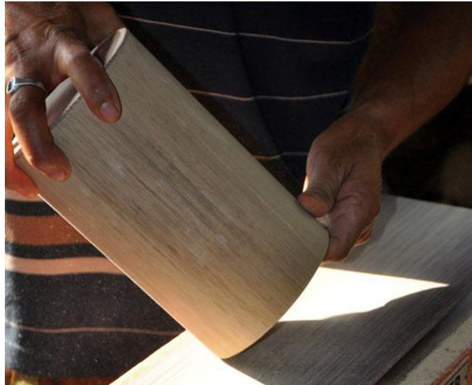
The sharp edges are buffed to make even.
