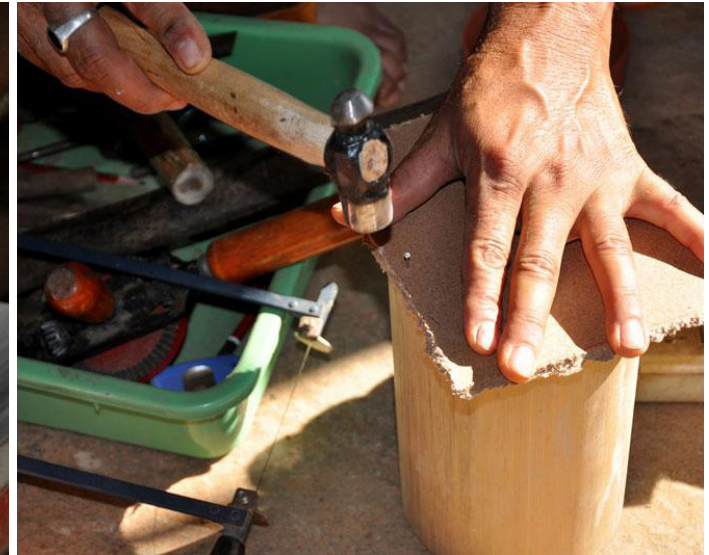
Base of the product is being fixed by nailing.
