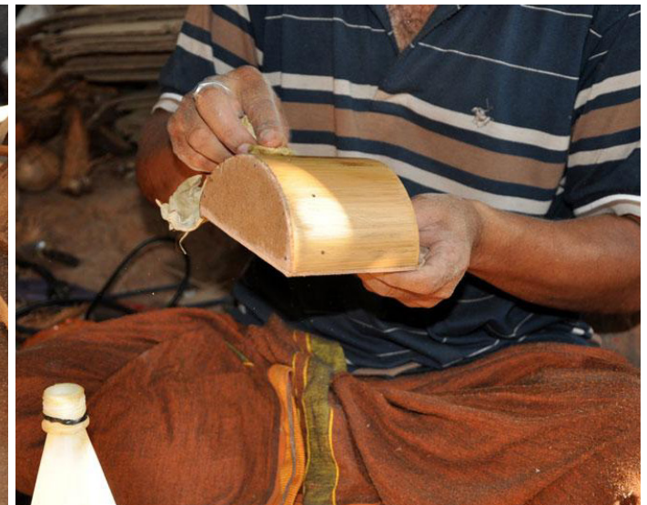
Product is coated with wood polish before painting.
