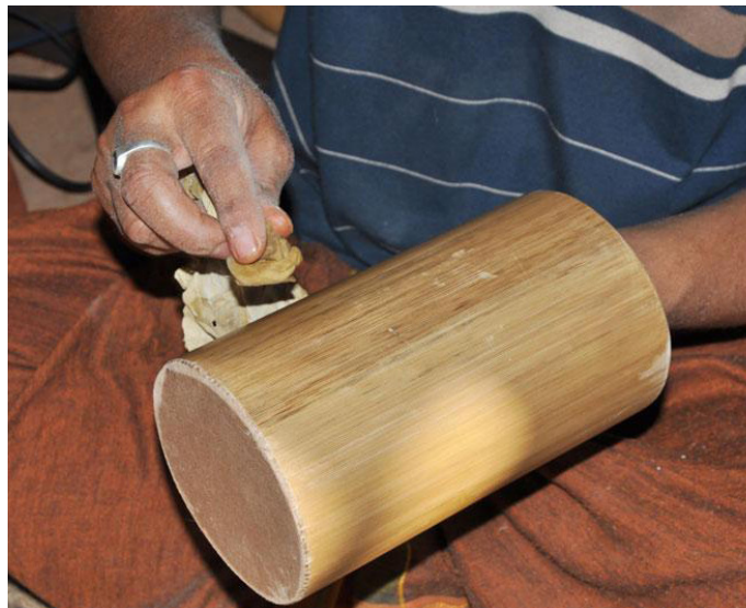
Wood polish is applied on product using cotton cloth.
