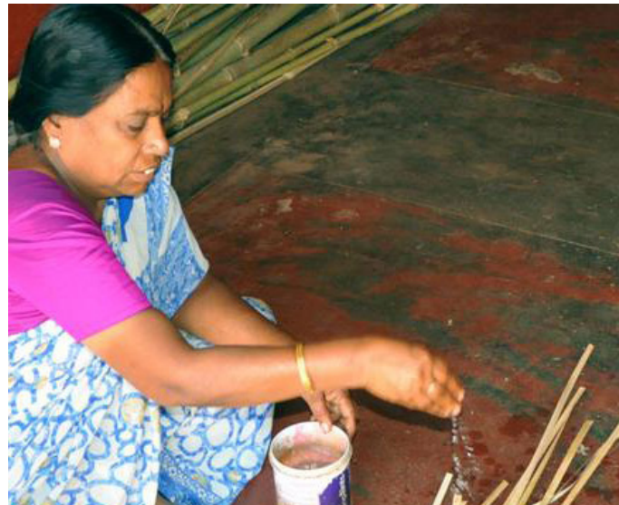
Bamboo is treated with water to make it soft.
