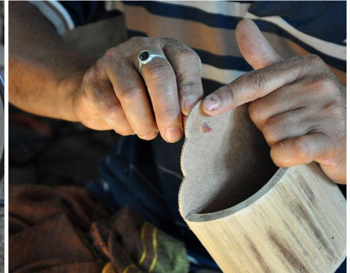
The cavity is again smoothed with sand paper.
