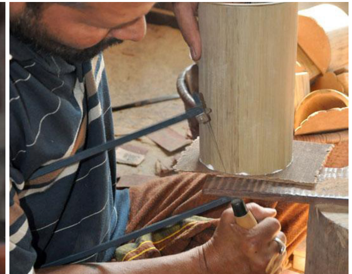
Hacksaw blade helps to remove excess wooden sheet.
