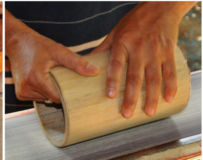
Surface of bamboo is being smoothened.
