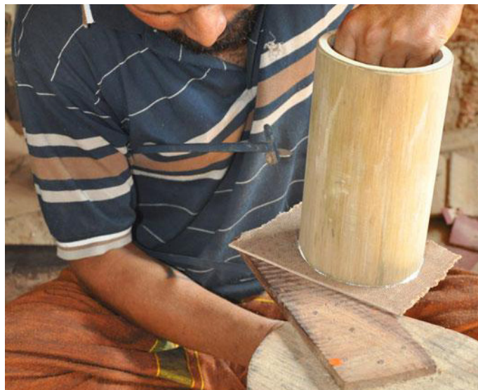
Excess wooden base is removed by cutting.
