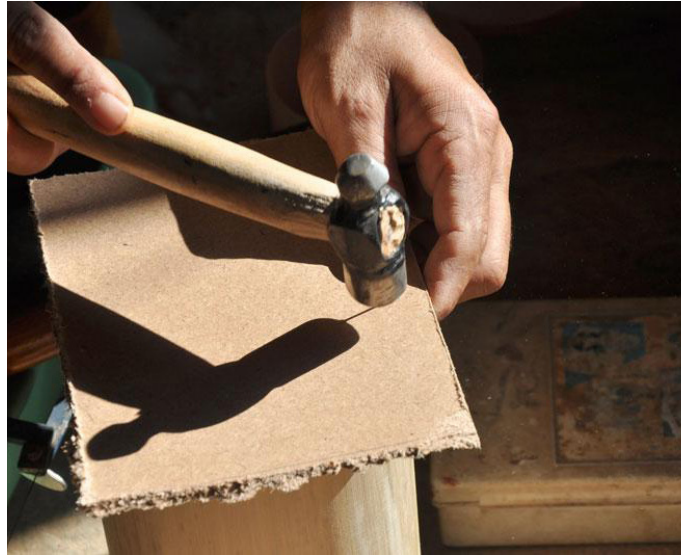
Thin wooden sheet used to cover the base of bamboo product
