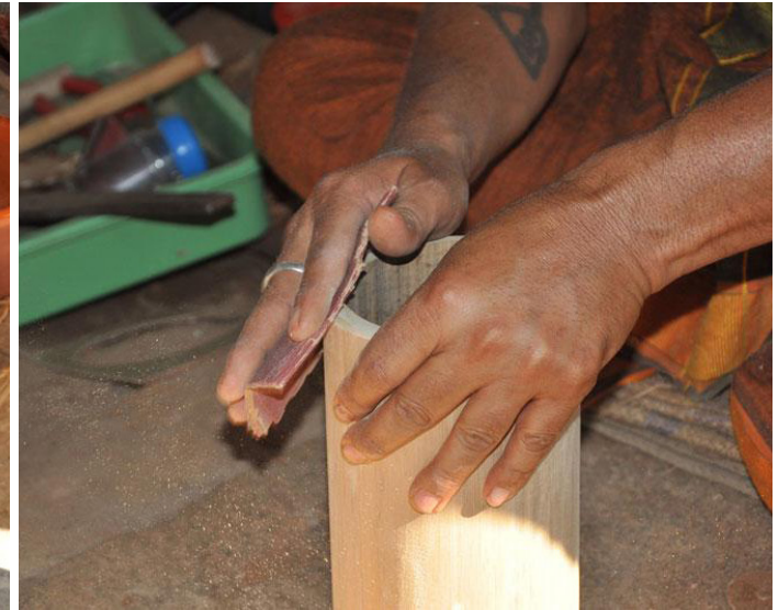
Sand paper used to smoothen the surface manually.
