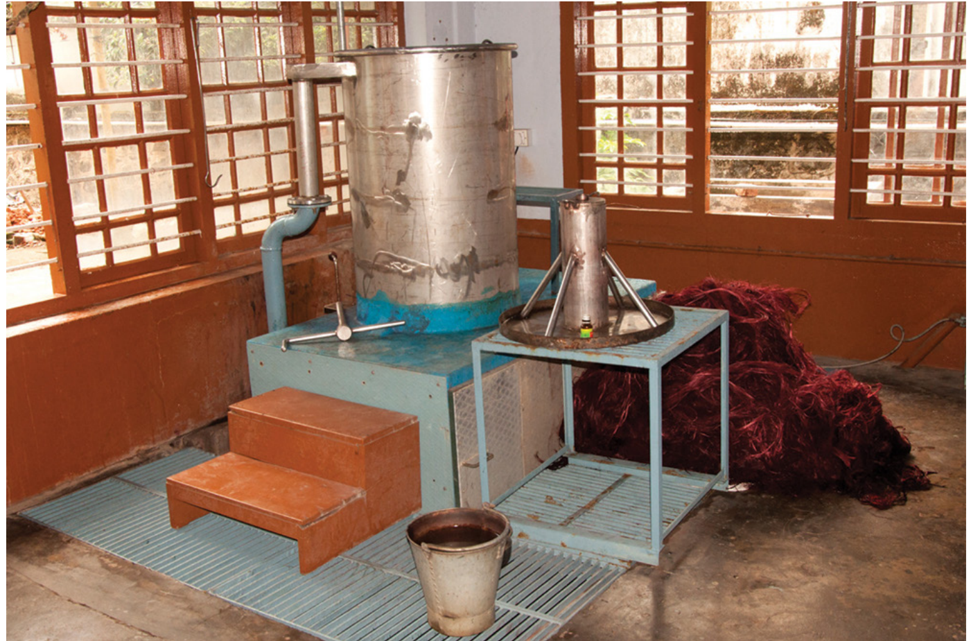
Dyeing machine is used in dyeing the fibres in large scale.
