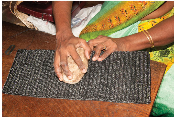
Removing minute procuring fibers and smoothen the body of the basket with the help of stone.
