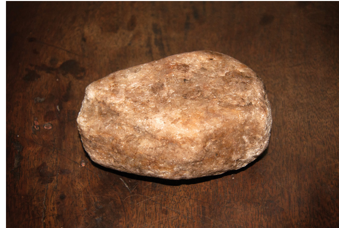
Soap stone used in removing small procuring fibres and to smoothen the surface.
