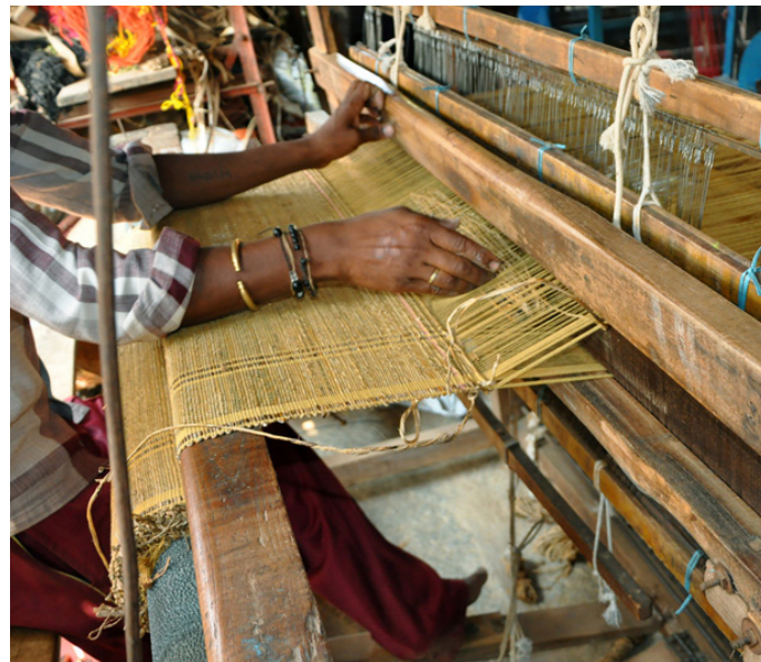
Joining the warp and weft threads.
