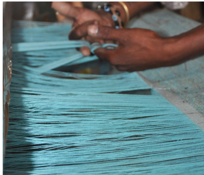
The threads are attached to the weaver's beam.
