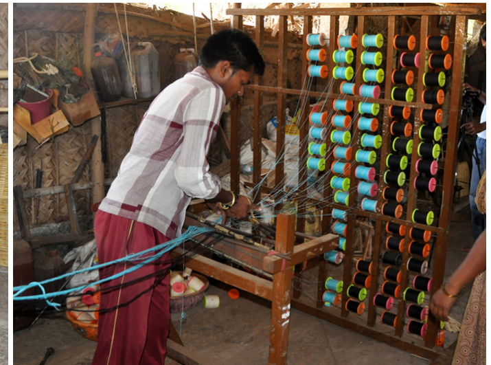
The spools are fixed to the warping machine to prepare the warp.
