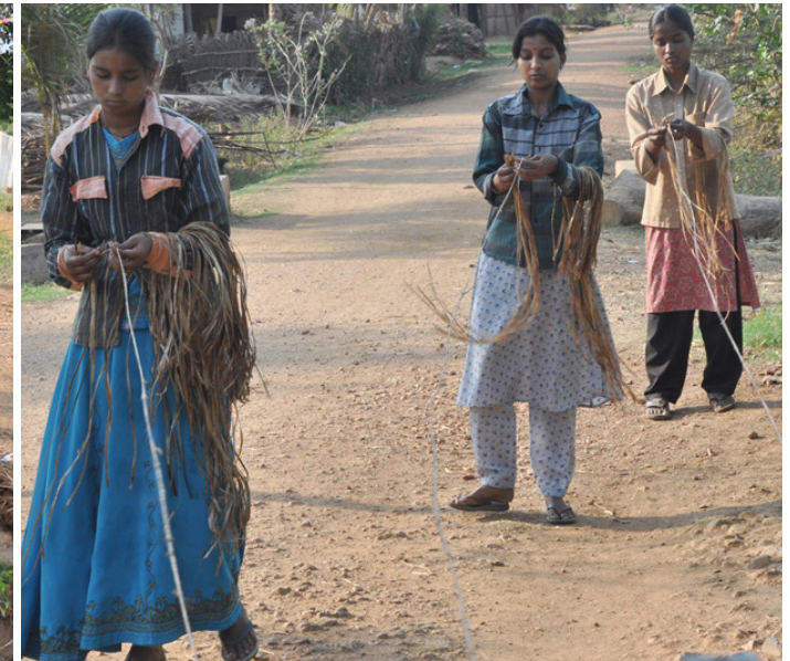
Continues addition of banana fiber is required to get a lengthy yarn.
