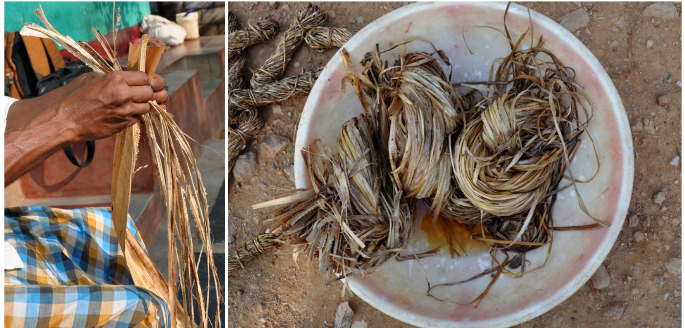
Banana bark is split into small slices. The fibre is soaked in water before twisting.
