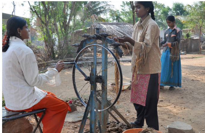
Banana yarn is prepared using spinning wheel.
