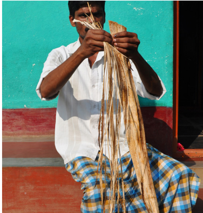
Artisan engaged in peeling thin fiber strips from banana bark.
