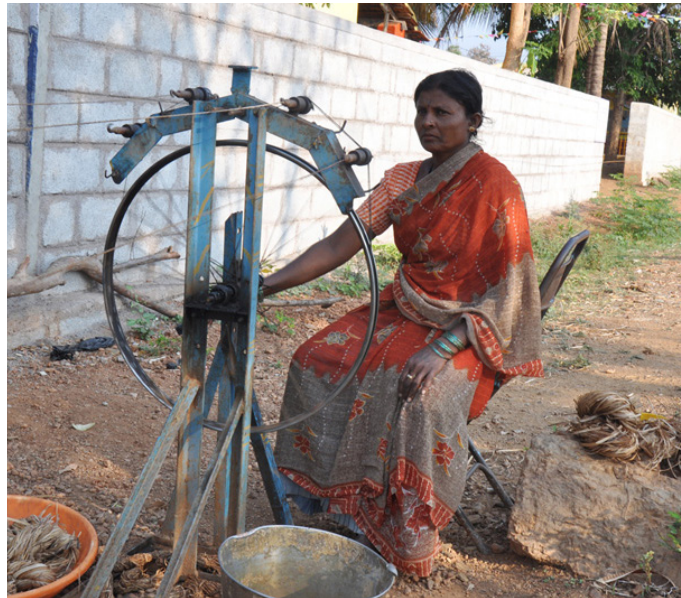
Artisan engaged in working on spinning wheel to make banana yarn.
