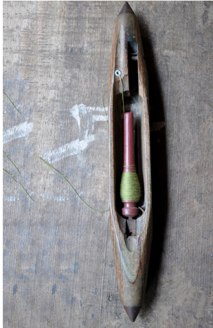
Fly shuttle of cotton thread used to decorate mats.
