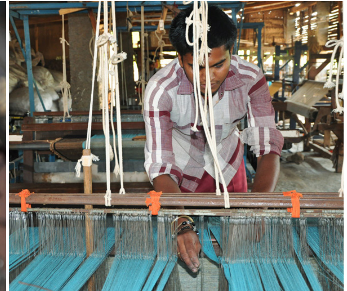
Weaver loading the warp into the loom.
