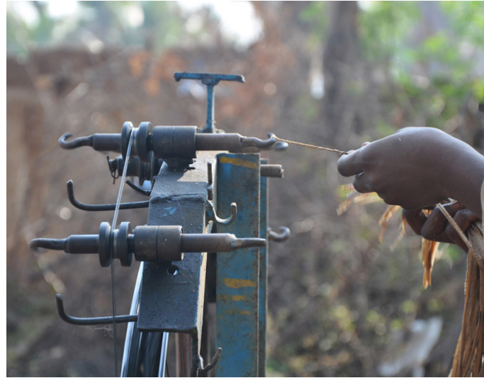
Banana bark strands are hooked to spinning wheel.
