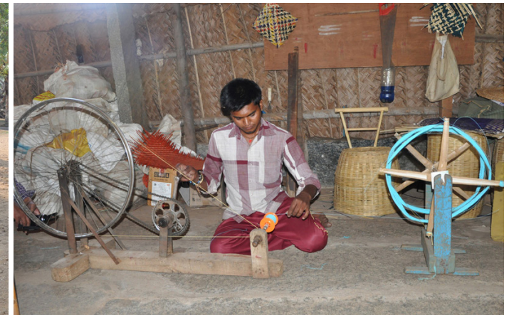
Artisan filling the spindle with threads using spinning wheel.
