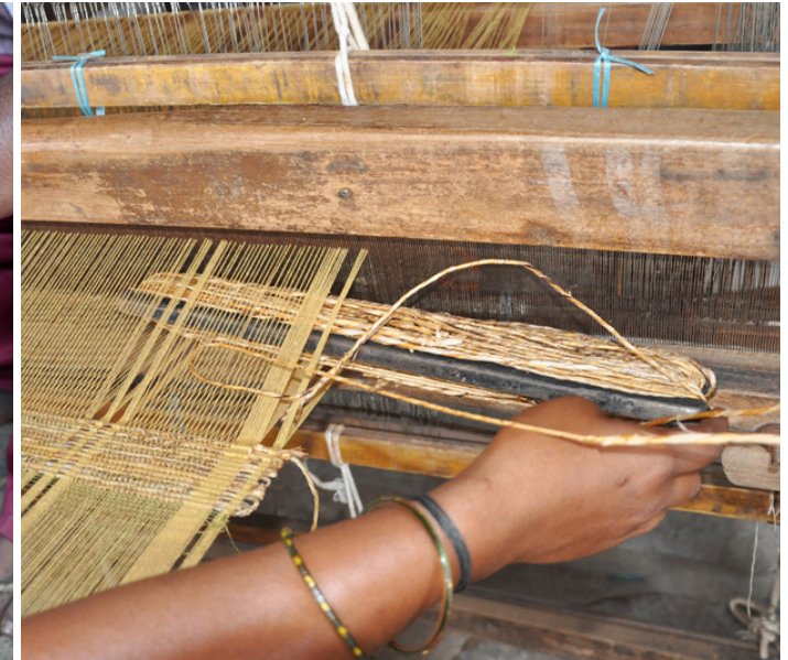
View of inserting fly-shuttle into the warp threads.
