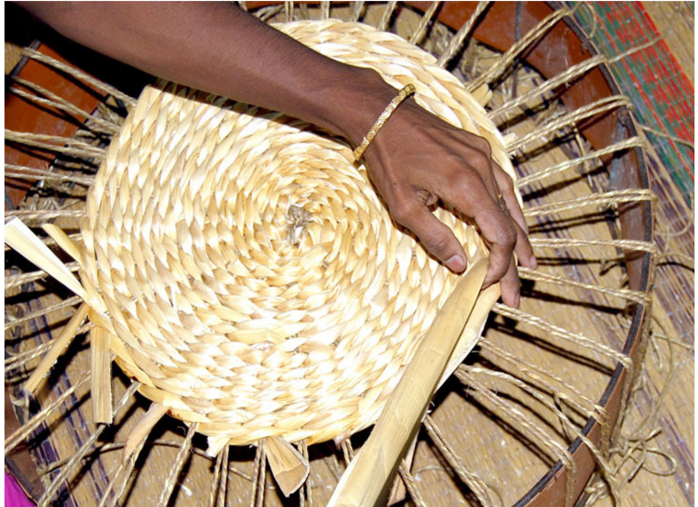
The banana fibre twine is used in the weaving process of the basket/cushion.
