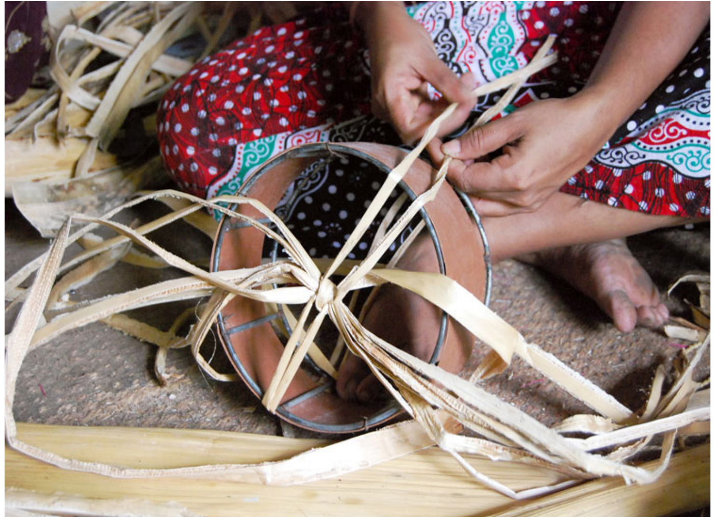
The craft person is weaving the banana fibre across the body of the frame.
