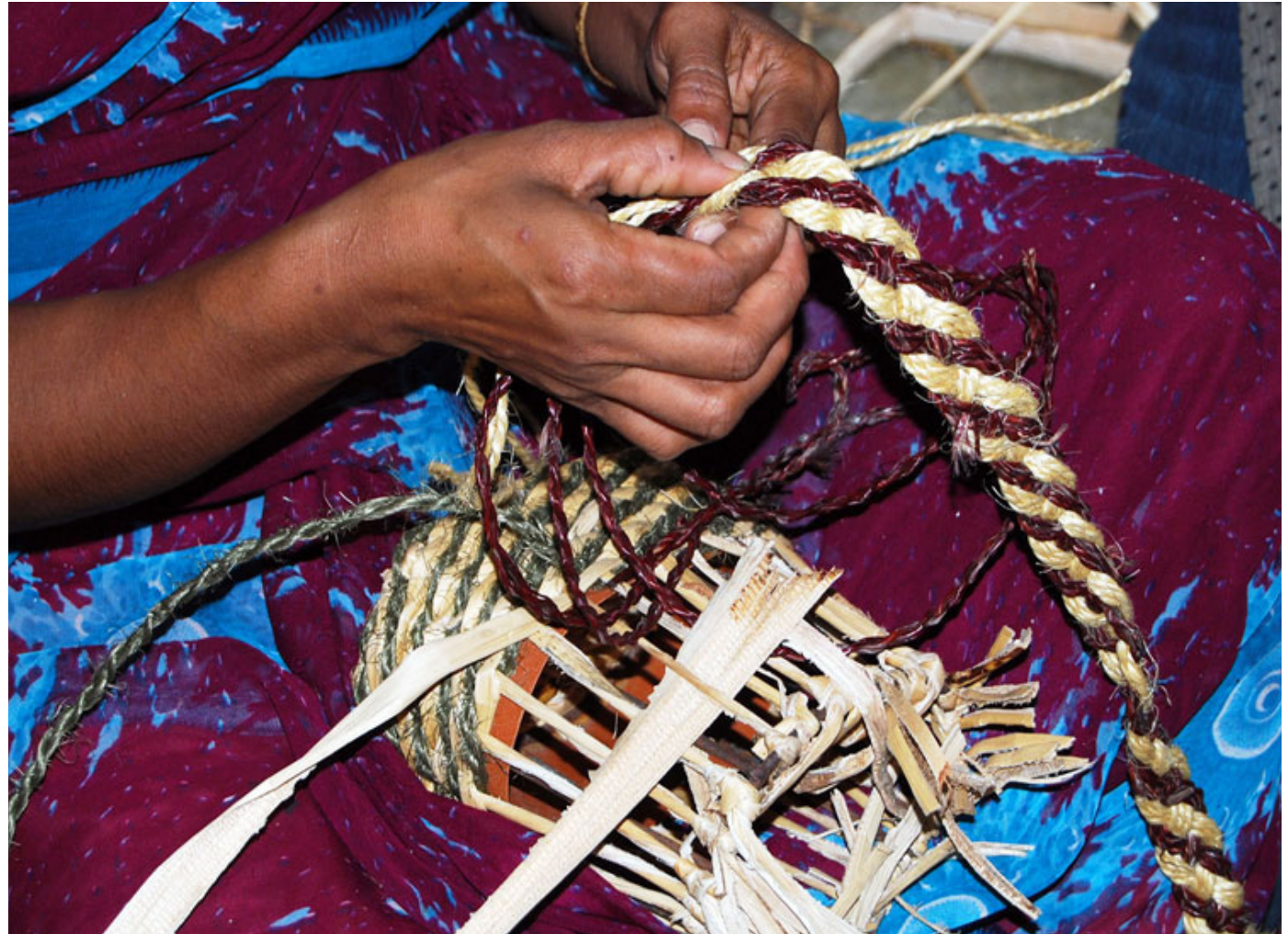
The twines are further twisted to make the handles of the basket/bag.
