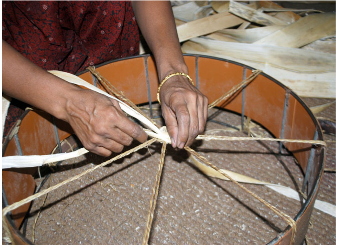
The weaving of the banana stem begins from the base-frame.
