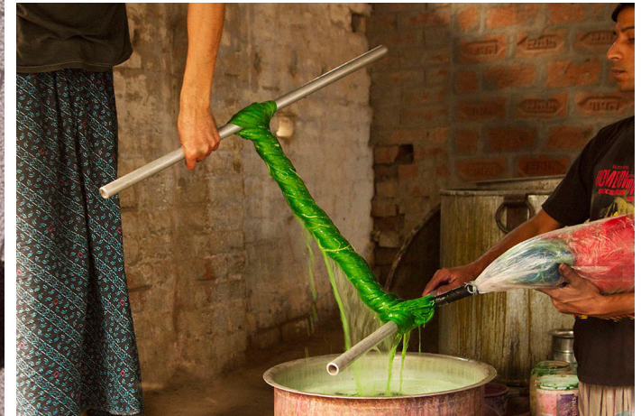
Twisting rods to remove the excess of solvent and rinse the yarn.
