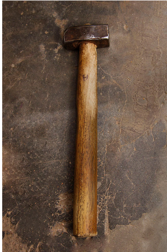
Hammer is used to punch on the bolt and make a hole on the cards (Jacquard).
