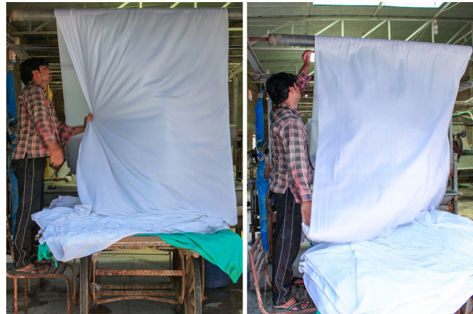
The fabric is pulled out from the bleaching machine to dry it.
