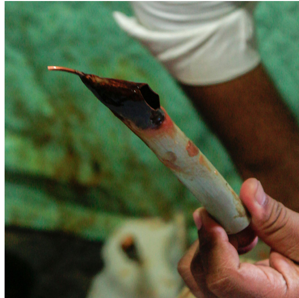
Canting tool used for applying wax on fabric in Indonesian style of batik printing.
