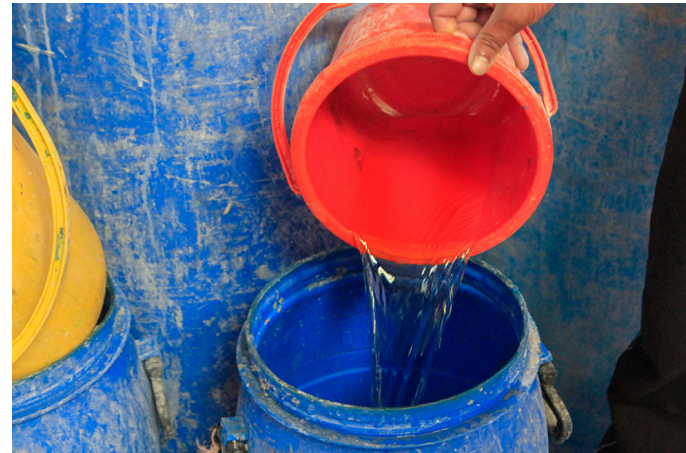
Mixture of bleaching powder and water is used to make fabric white.
