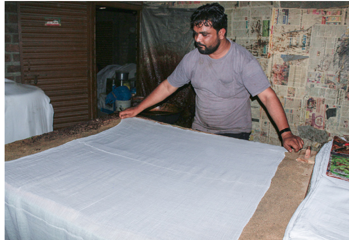
The fabric is placed on the layer of mud to reduce spreading of wax on cloth.
