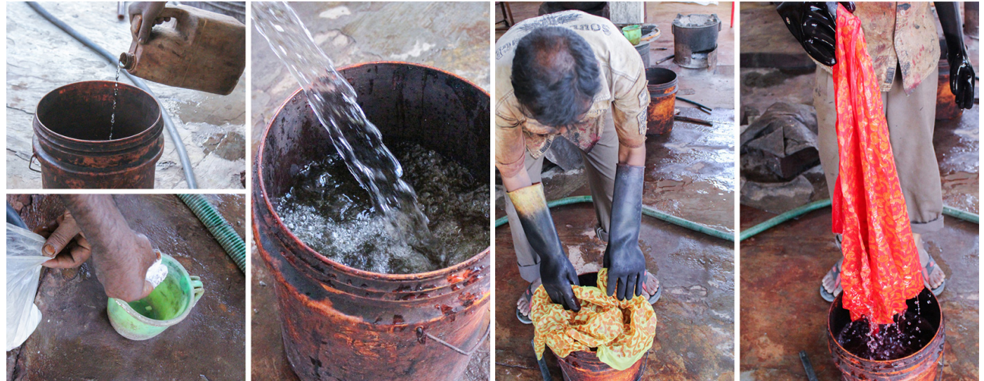
Required color liquid and nitric acid powder is mixed with water to give the fabric a permanent color.
