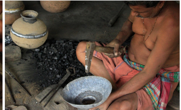
It is light hammered at the edges to bend sharp corners.
