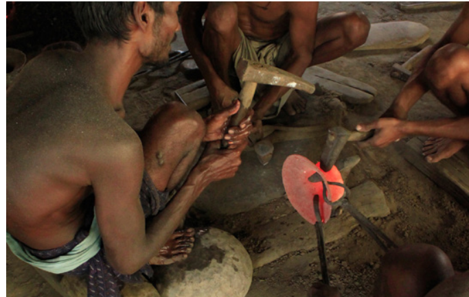
The metal is then heaved out of the mould.
