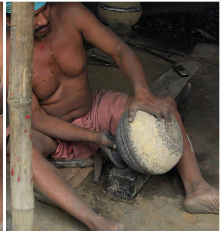
The artisan then checks for the accuracy of the aligned parts of the pot.
