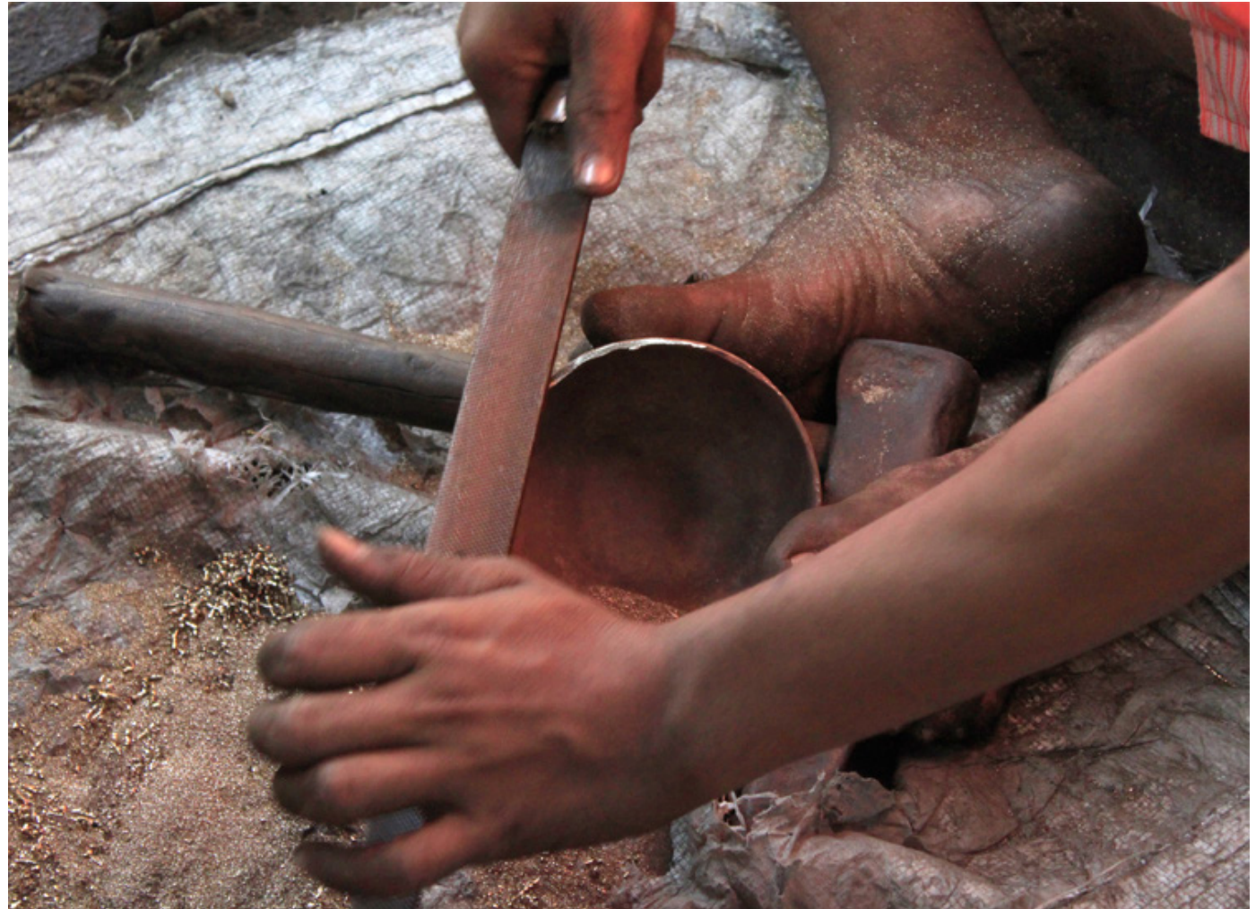
The file is used to scrap the extra material to smoothen the surface texture.
