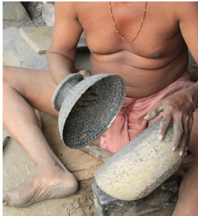
The artisan then aligns the two parts of the pot together.
