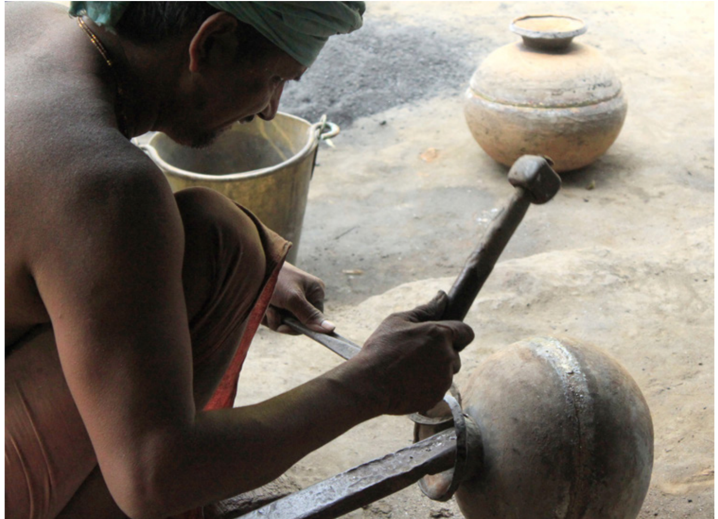
The pot is lightly hammered to make it more durable and long lasting.
