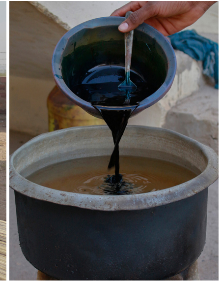
Mixed color is added to the boiling water for dyeing the yarn.
