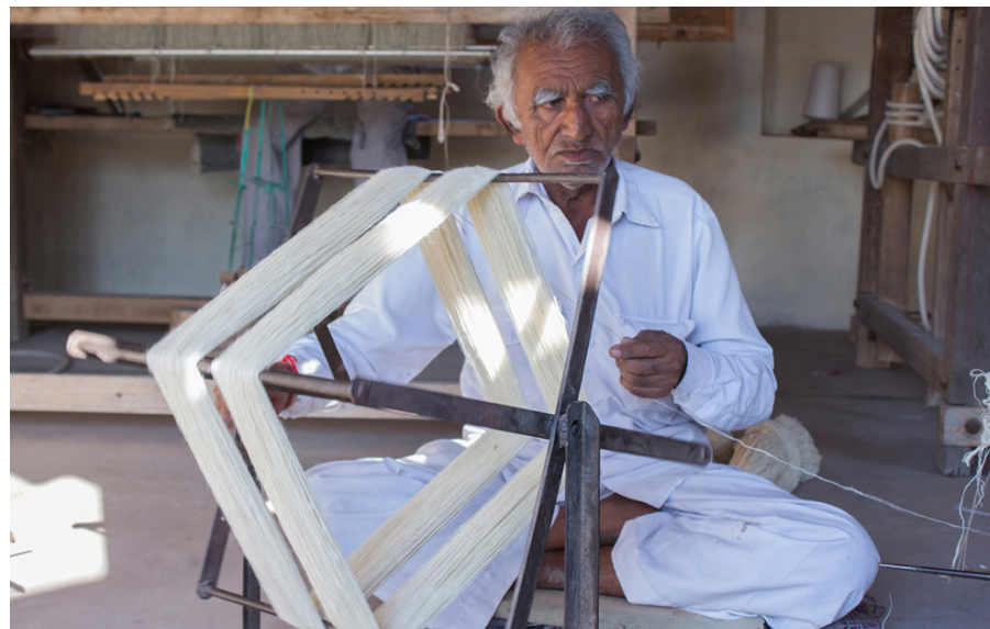
The yarn is winded appropriately on a yarn swift.
