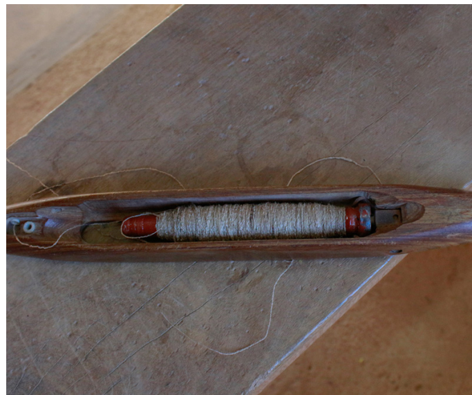
Flying shuttle is used in handloom for weaving.
