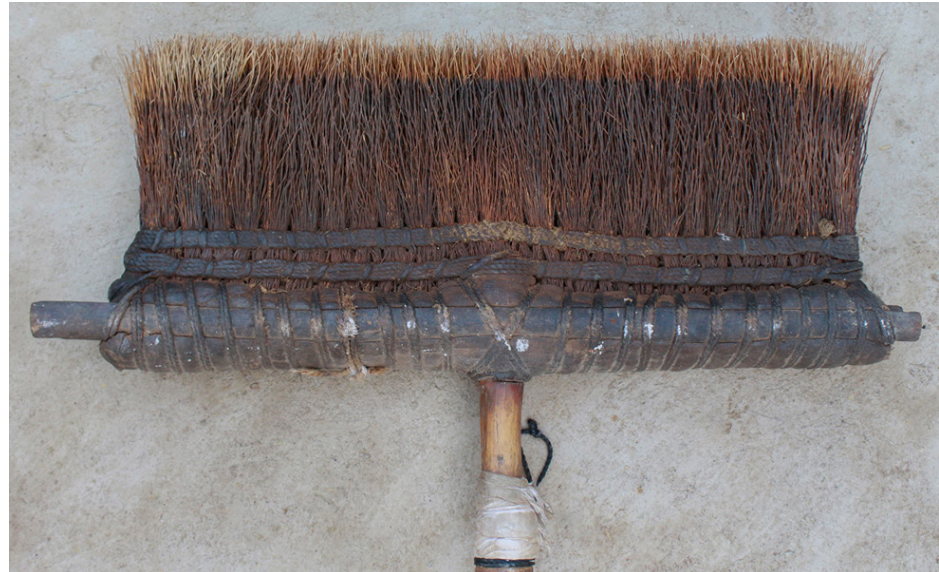
Coir brush is to separate the yarn from sticking.
