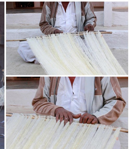
Yarn is tied between two sticks for starching.
