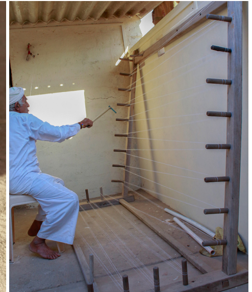
Yarn is warped in a frame for weaving process.
