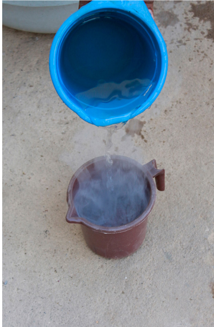
Acid is mixed with water for dyeing process.
