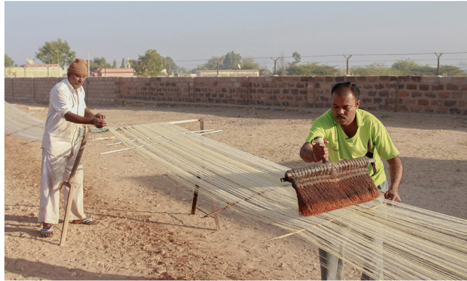
Coir brush is used to separate the yarn without sticking to each other.
