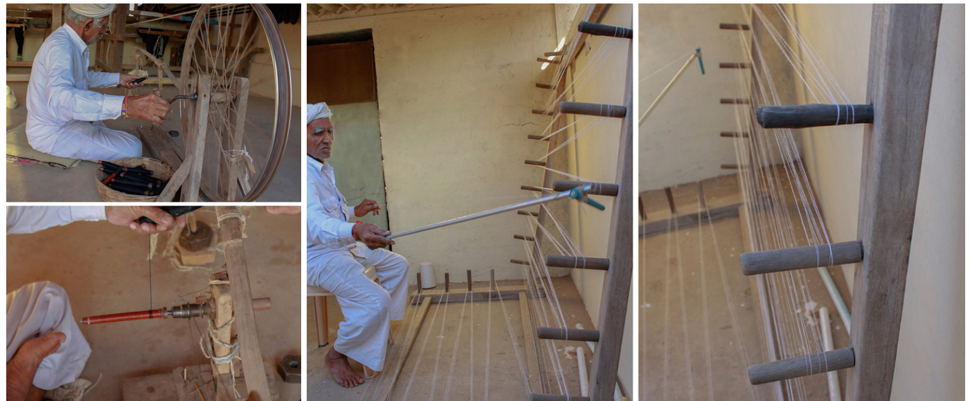
Yarn is winded in a pirns for weaving.
