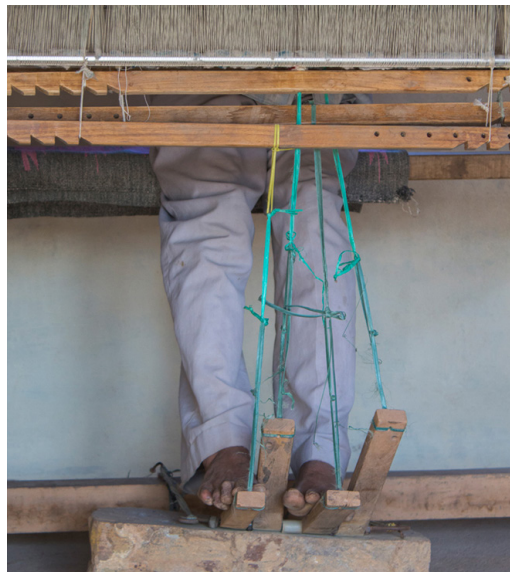
One of the important parts of handloom called foot paddles.
