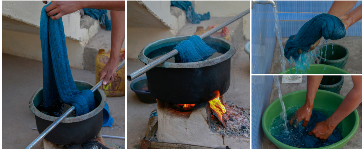
Yarn is again dipped into the dye.
