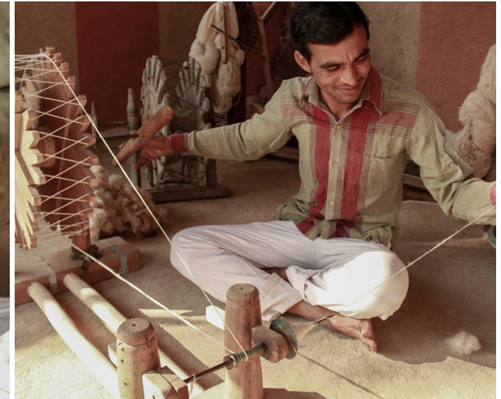
The yarn is extracted from wool using a spinning wheel.
