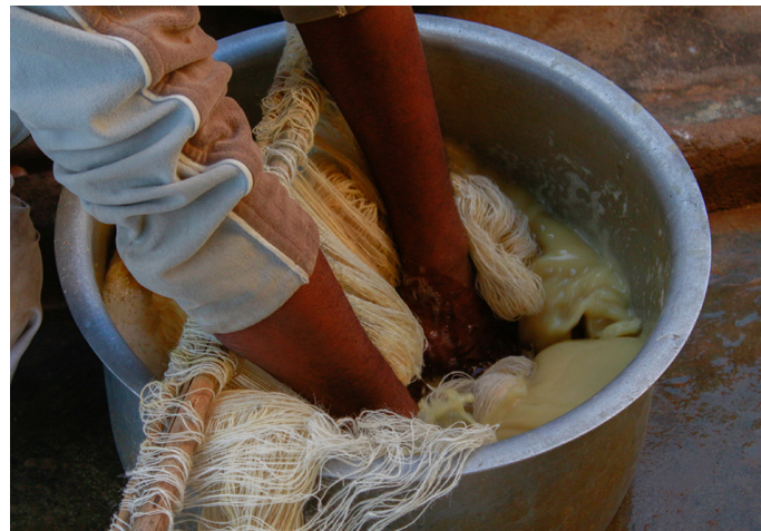
Yarn is soaked into the starch.
