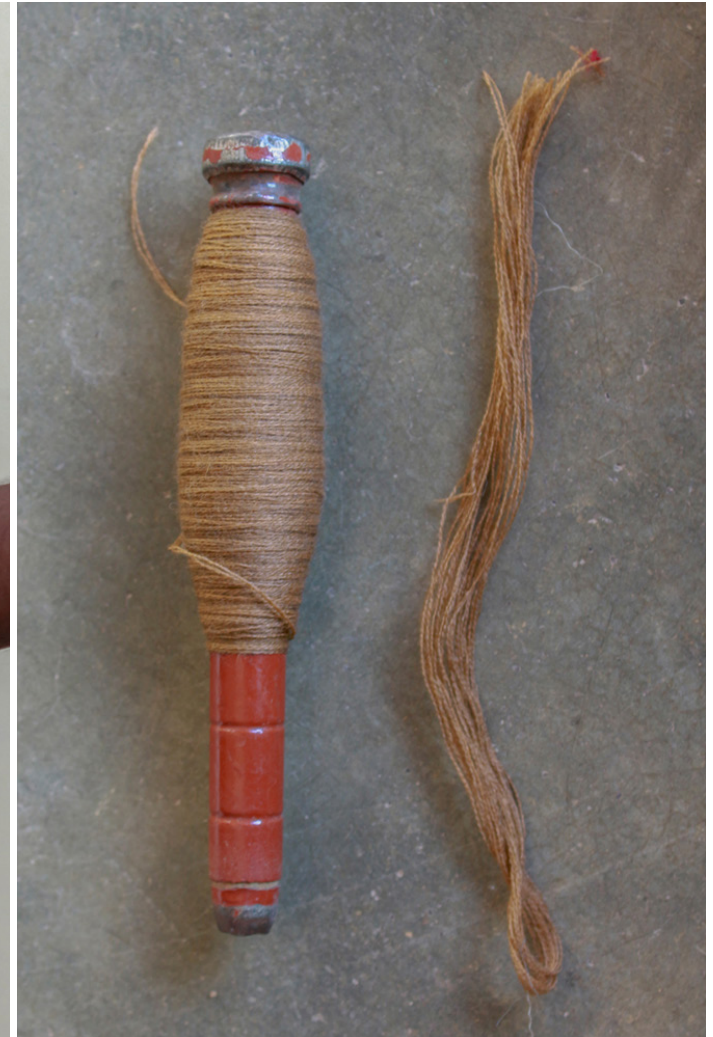
Acid is used in dyeing for long lasting color on the yarn. Yarn is winded on pirns and placed in flying shuttle.
