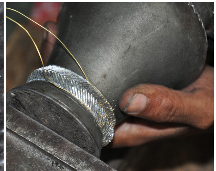
Brass metal wire is interposed into the grooves to enhance the outer look of design.
