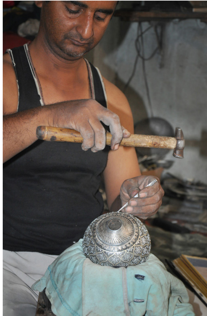
Artisan meticulously hammering the silver into the grooves.
