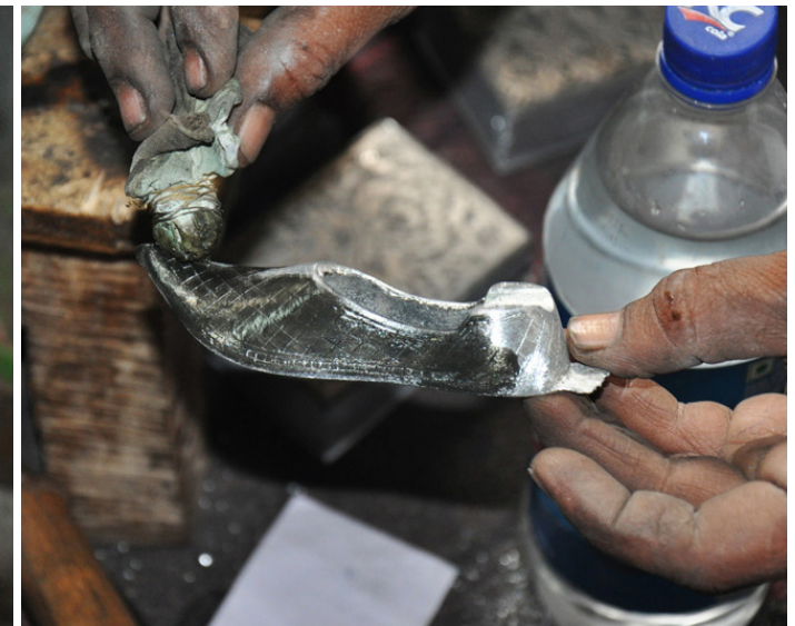
Copper sulphate is applied to temporary black colour.
