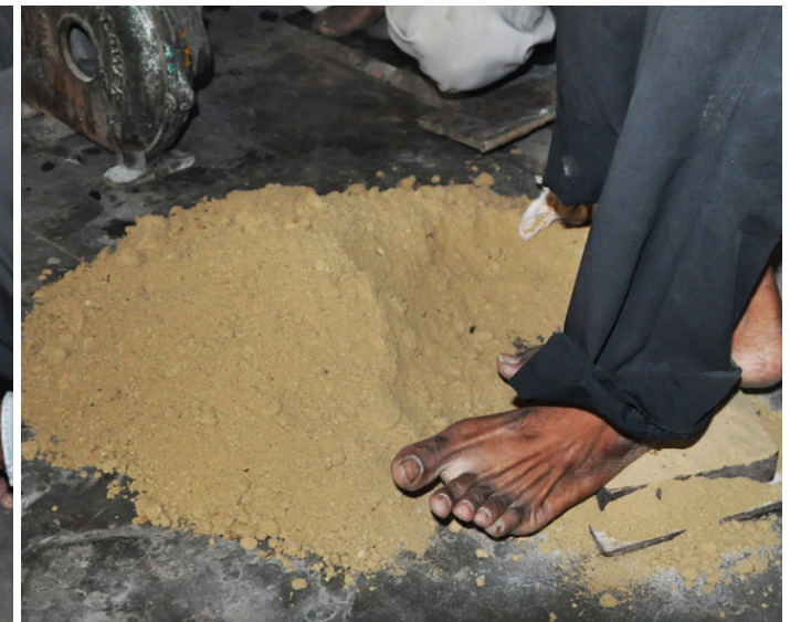
The frame is filled with clay and stamped on it.
