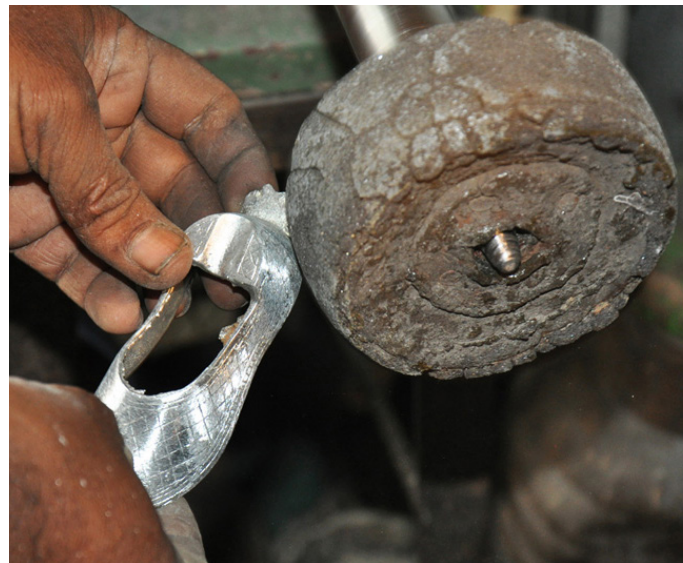
The casted metal product is removed and buffed.
