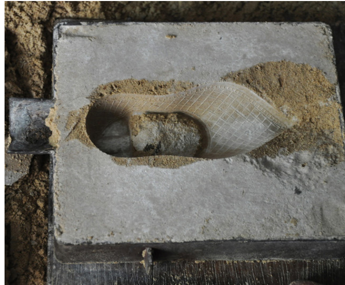
The mould is ready for the casting process.
