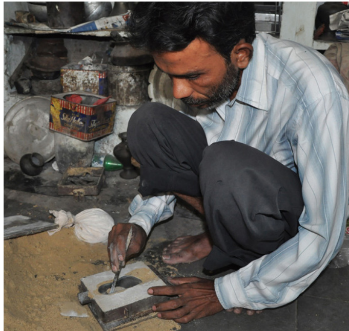
Bidri artisan engaged in mould making process.
