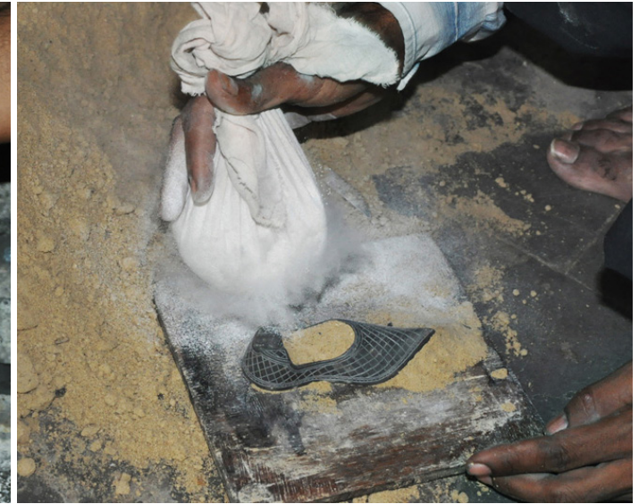
Boric powder is sprinkled on the clay filled mould.
