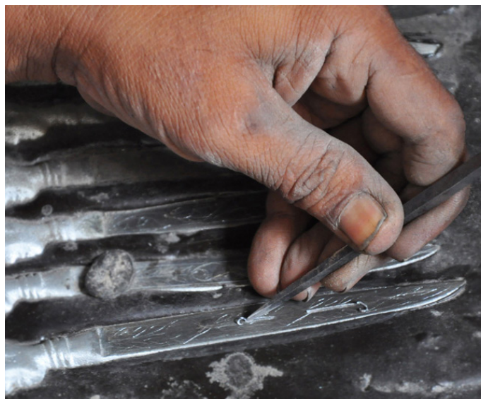
Surface of article is engraved with chisel.
