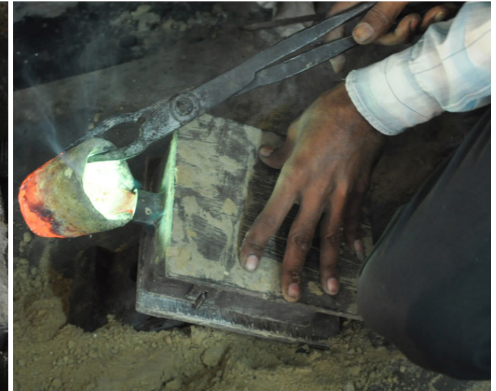
Melted metal is poured into the mould.
