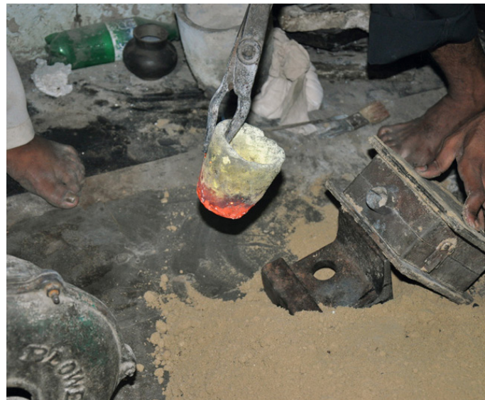
Zinc and copper are melted in crucible and poured into mould.
