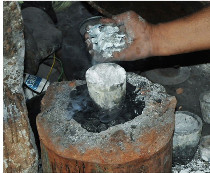
The alloy, raw material is melted.
