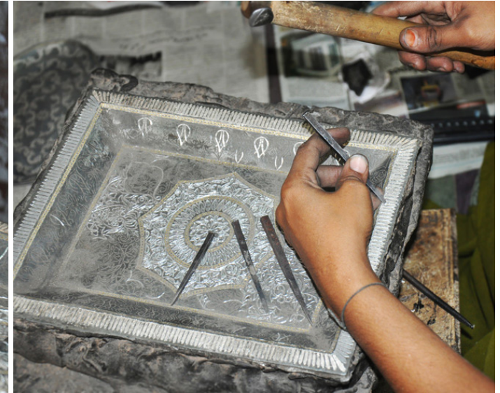
The inserted silver is properly aligned by hammering.
