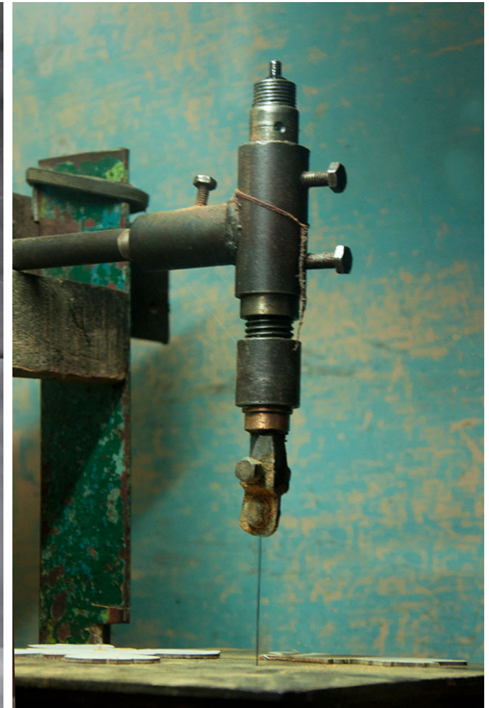
Customized cutting machine is used to cut plywood into required design patterns.
