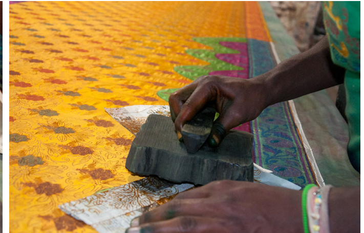
Block dipped in paint is used to create a design patterns on saree.
