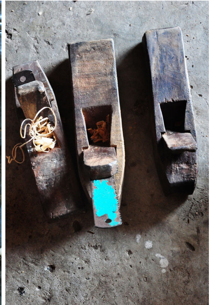
Wooden scrapper is used to smoothen he surface of wood.
