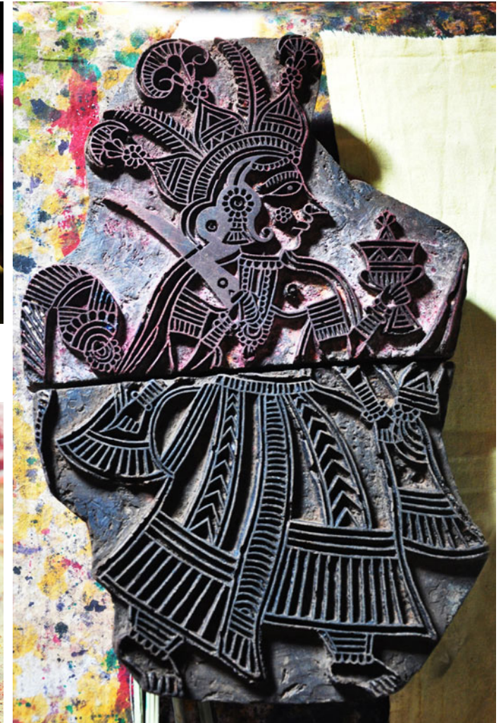
To print big design, the design is divided and carved on two block pieces.
