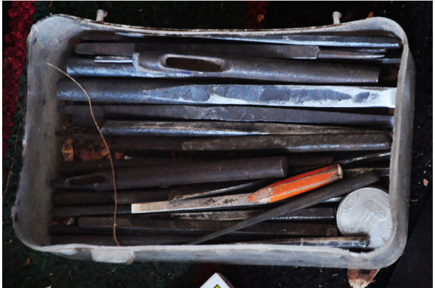
Different sizes of chisels are used to carve minute designs on the wood.
