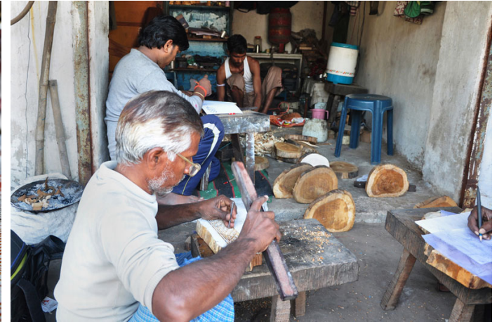
The designs are then traced on the wood to prepare the block for printing.
