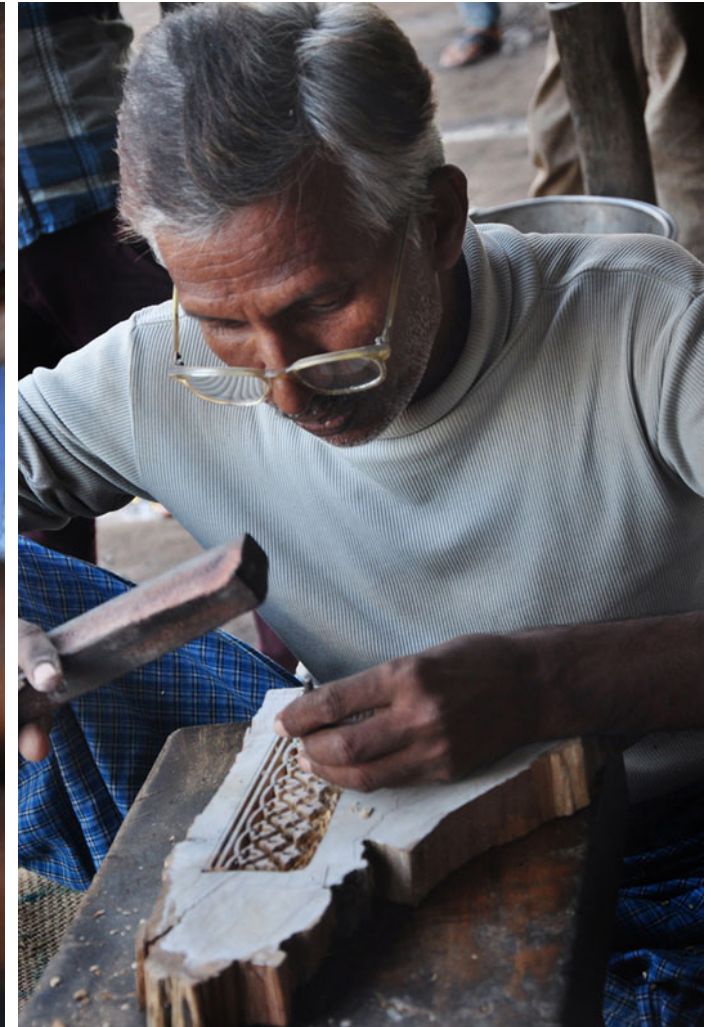
Minute designs are carved using hammers and chisels.
