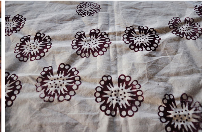
Selected portions of the cloth are only printed with hand blocks.
