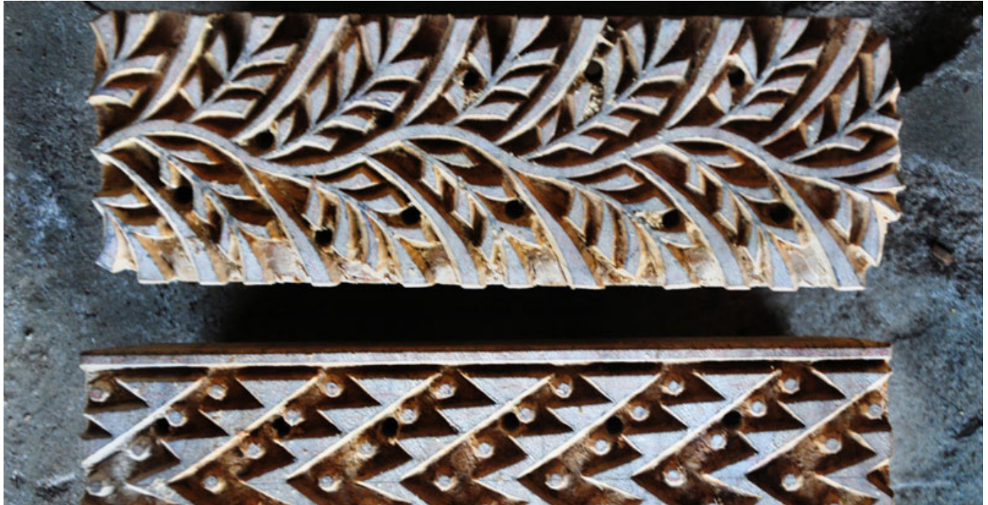
Patterns on the blocks are raised by scooping out the negative areas (designs are carved out).
