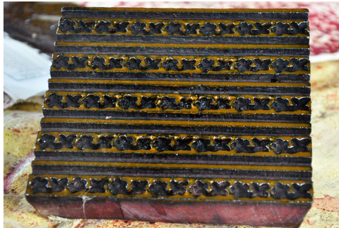
Block used to design borders on the fabric.
