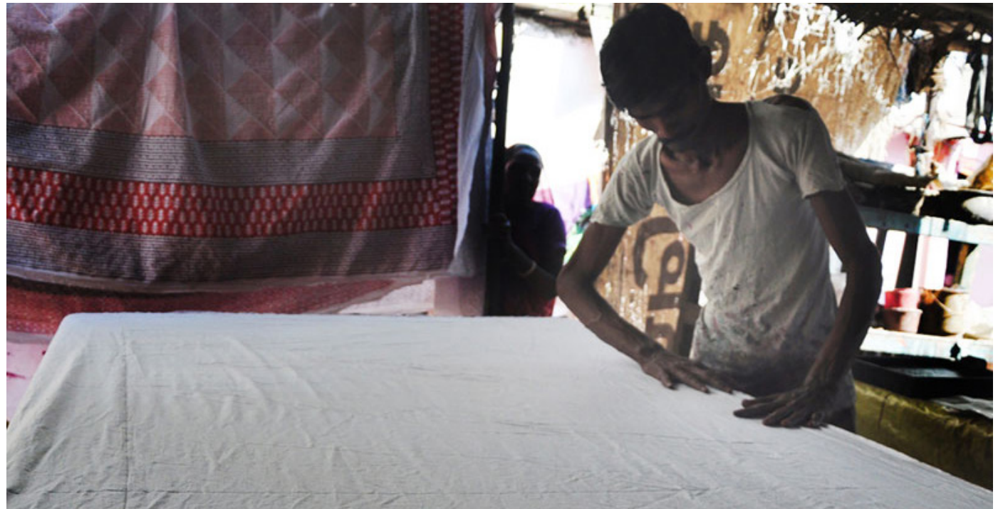
Cotton fabric is evenly spread on a table before printing.
