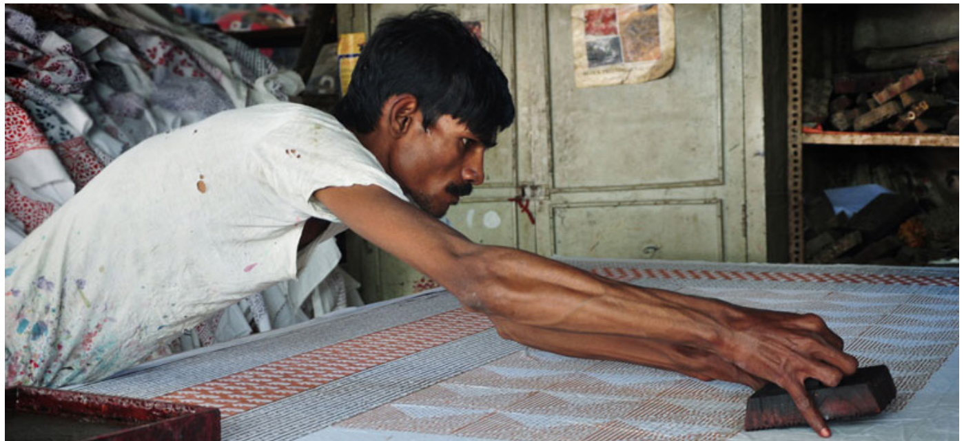
Artisan involved in block printing the designs on cloth.
