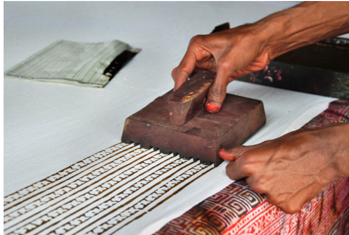
Each block is pressed on the cloth to print the design with the support of thumb finger.
