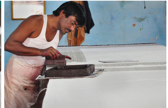
Printing block is immersed in the printing ink kept in a wooden tray.
