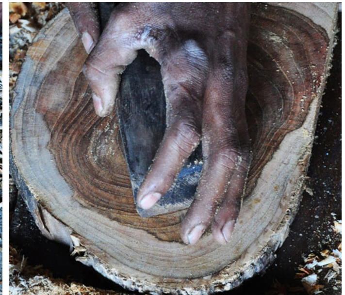
Surface of the wood is smoothened using wood scrapper.
