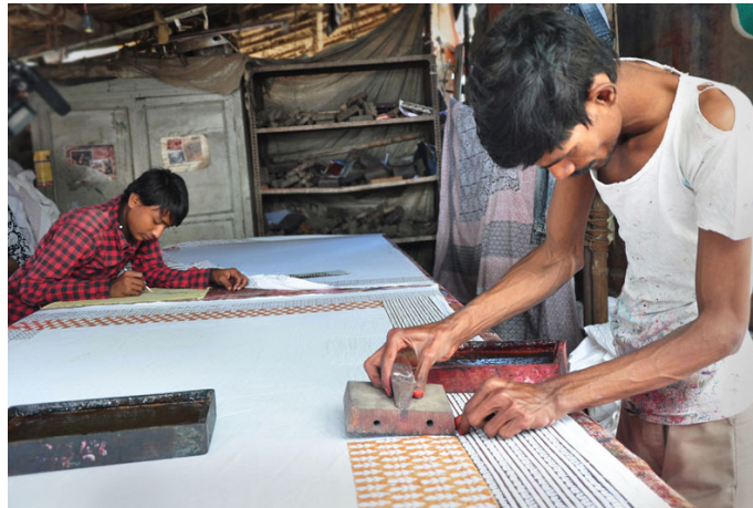
Separate blocks are used for different colour and pattern.
