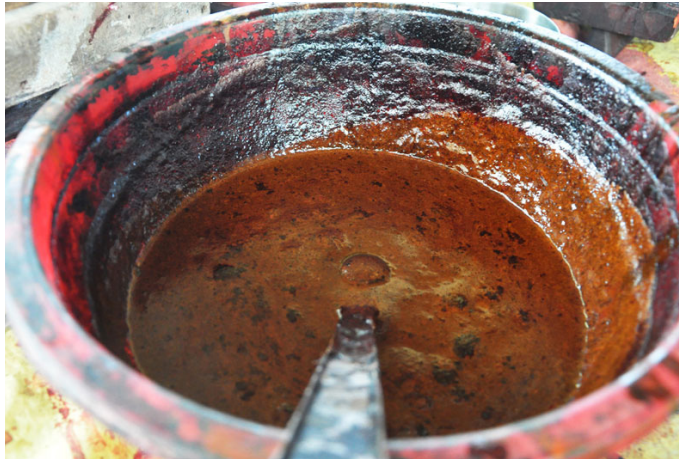
Printing paste is mixed in a tub before pouring into wooden tray.
