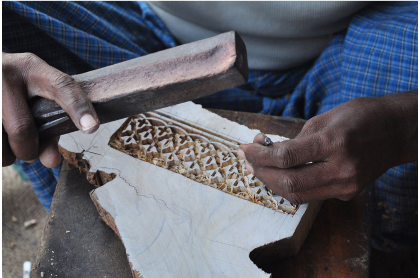
Minute designs are carved by chiselling and hammering.
