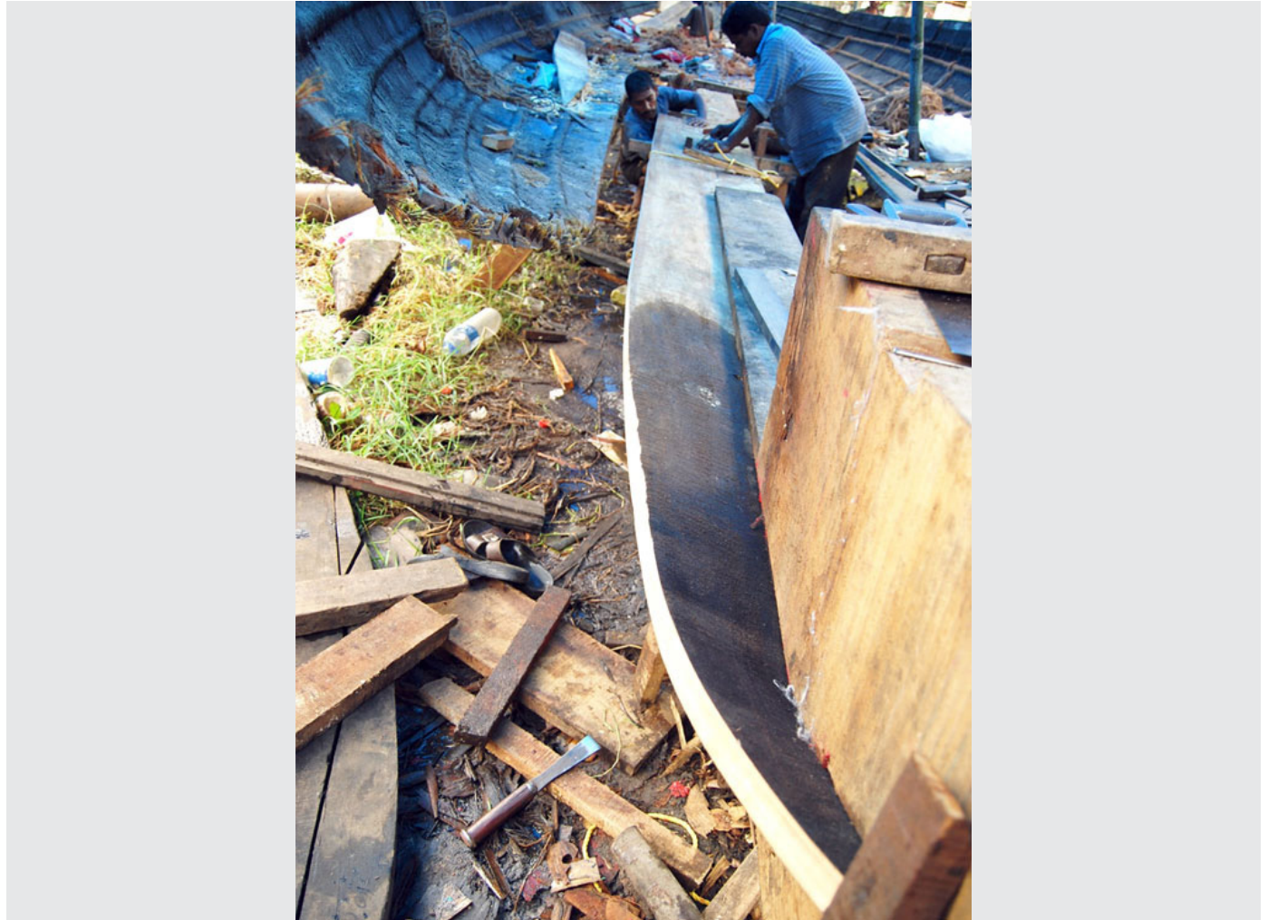
The additional planks are added for renovation and joined to the boat.
