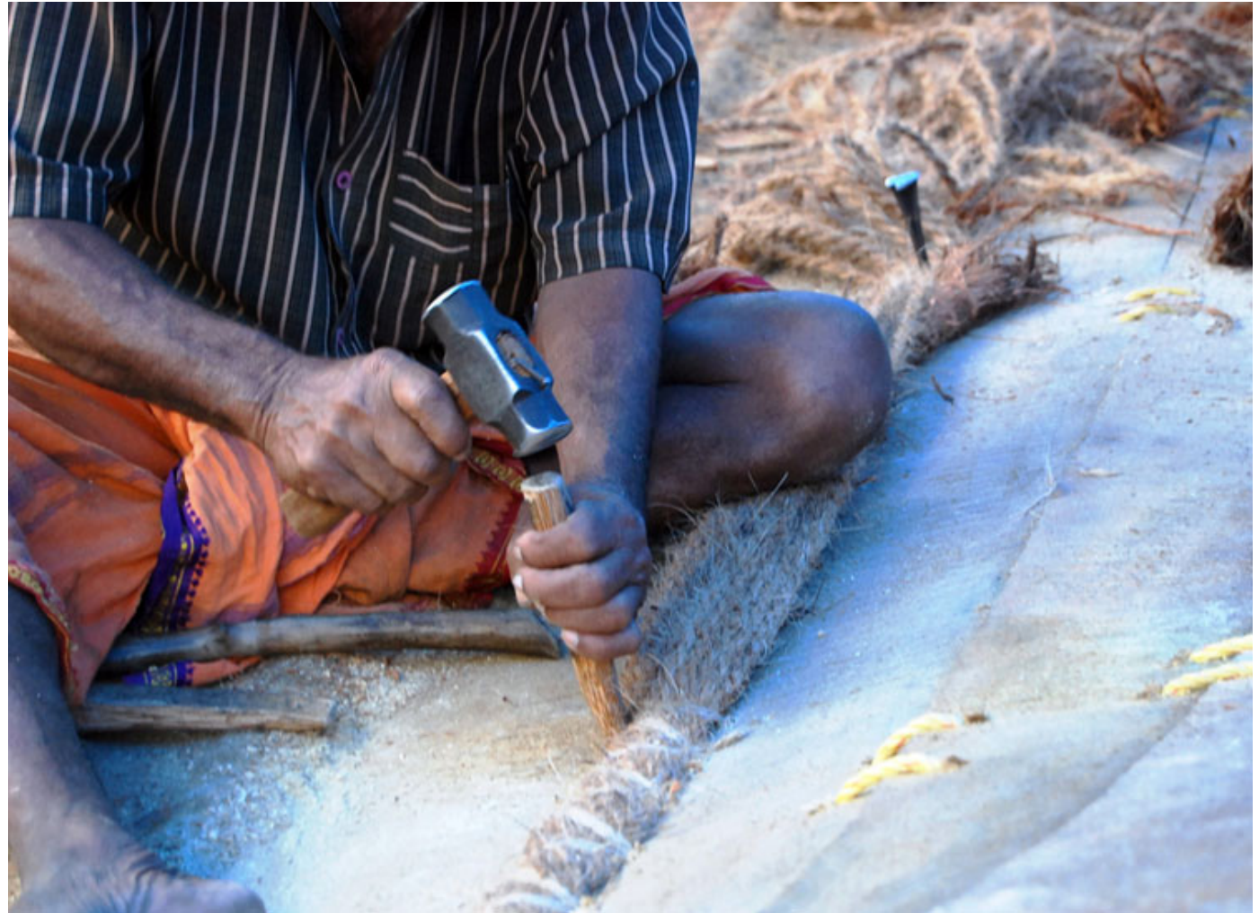
The strands of fibre are bundled and the twelve strips of twines are inserted into the coir.
