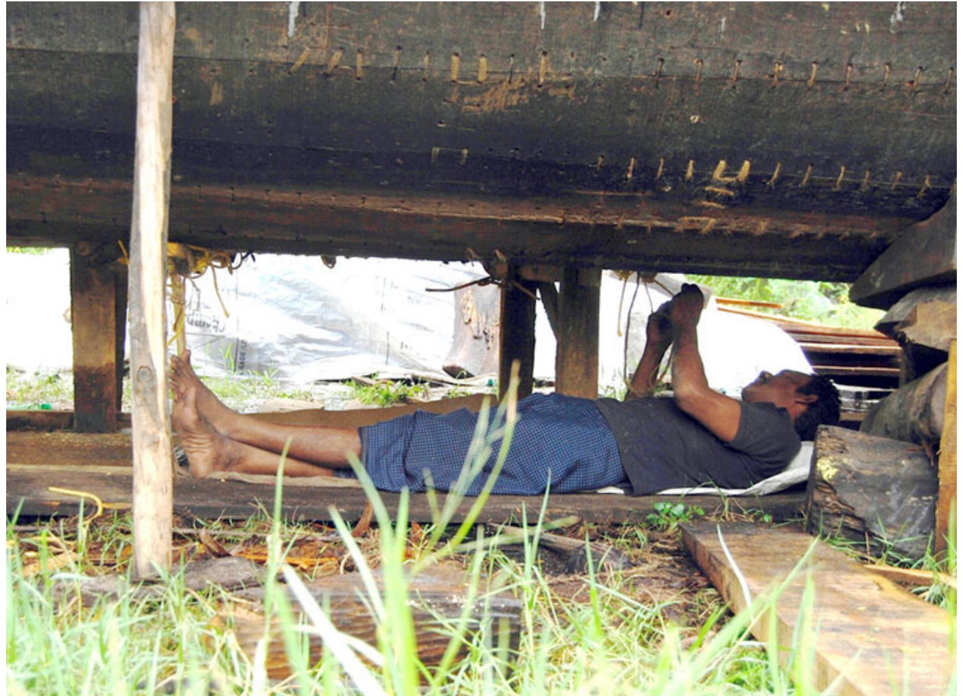
The craftsman hammers from beneath the boat and pulls and tightens the coir.
