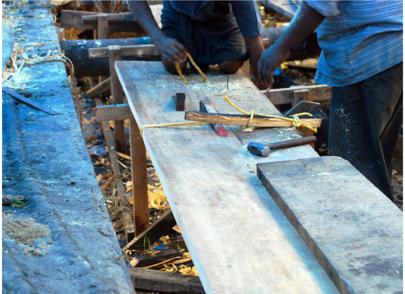
The planks are temporarily nailed and stitched together with the synthetic rope.
