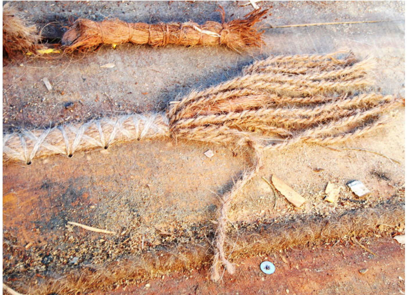
The closer perspective of sealing the joints of the boat.
