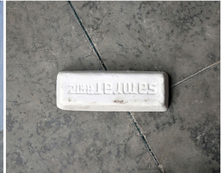
Buffing soap used to obtain glossy finish on the bone surface.
