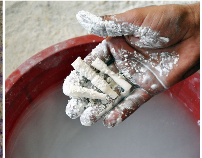
The products are coated with marble powder as it brightens surface of the final work
