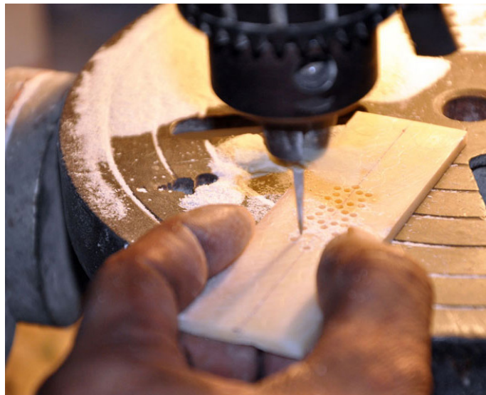
The holes are drilled as per the marked design.
