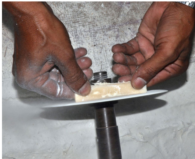
Artisan polishing the bone to smoothen the surface.
