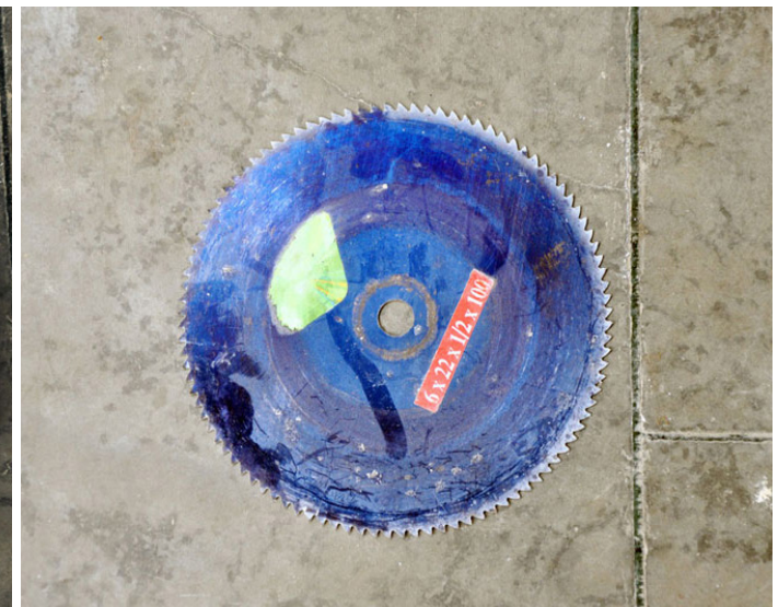
Cutter is attached to buffing machine to cut the bone into required pieces.
