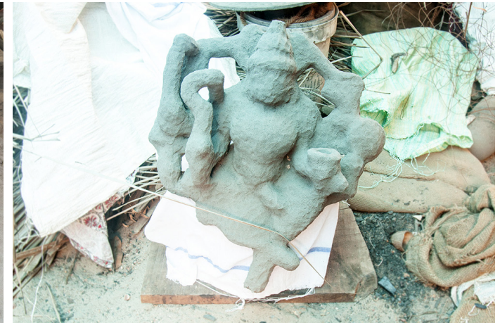
Image showing a wax model fully covered with mud, which is dried naturally.
