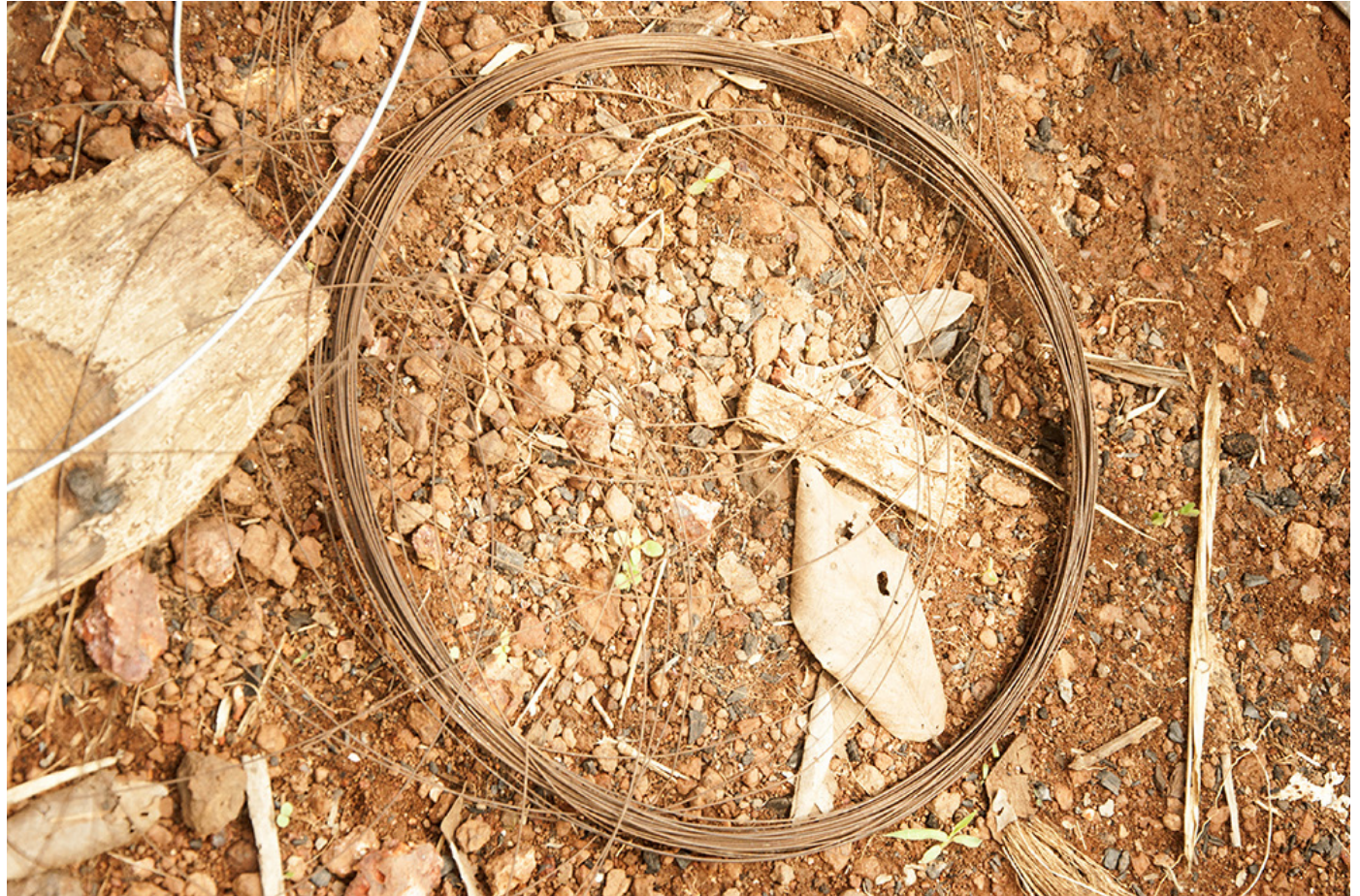
A bundle of GI wire, used in constructing large sized molds.
