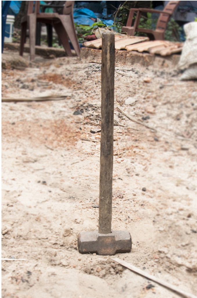
A Large sized hammer, used in reshaping iron, which are to be melted.
