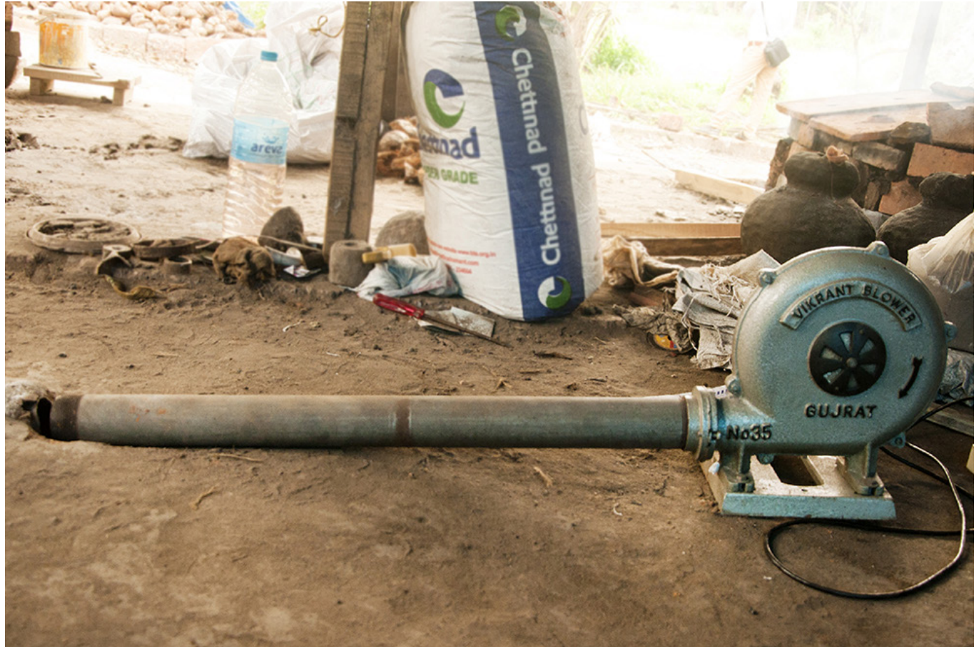
Air blower, used in firing up the furnace.
