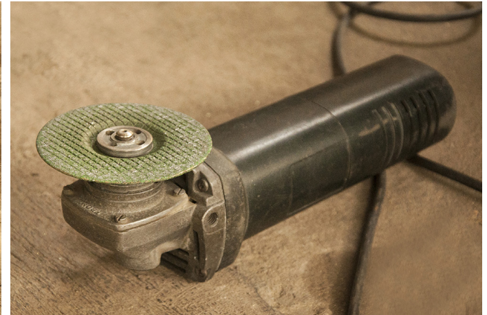
A handheld buffing machine, which is used in polishing the metal, after it is casted.
