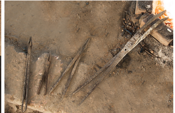
Pliers of different shapes and sizes, used in holding containers, in which metal is melted.
