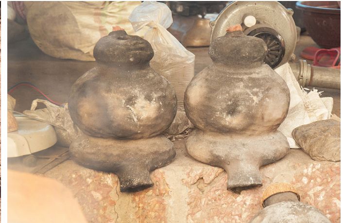
Set of negative molds made from a wax model.
