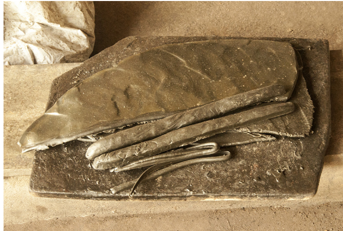
Sheets of wax, which are used in preparing an original wax model.
