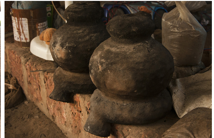
A clay negative mold, in which brass will be poured.
