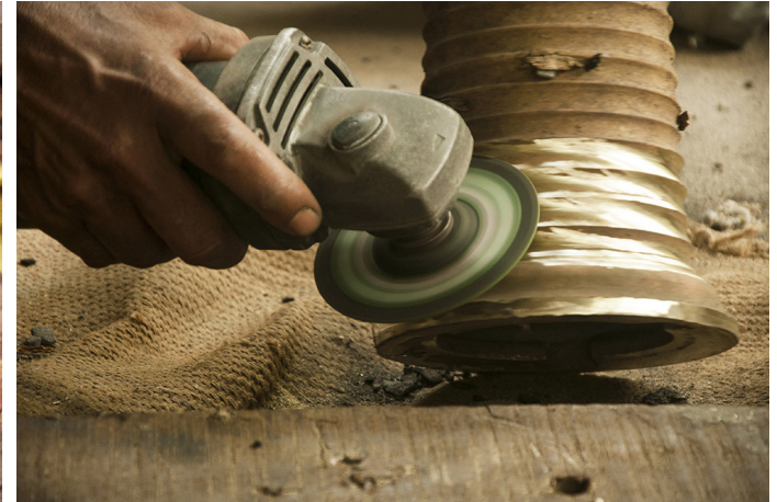
It is then buffed from a buffing machine, to clean it from sand and wax.
