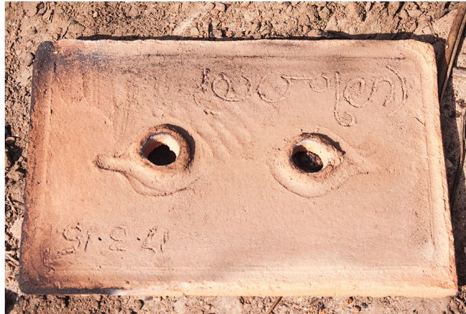
A lid, which is used in closing the wood fire operated furnace.
