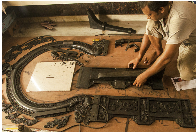
Artisan then places all the carved pieces on a diagram, to check the accuracy of the model.
