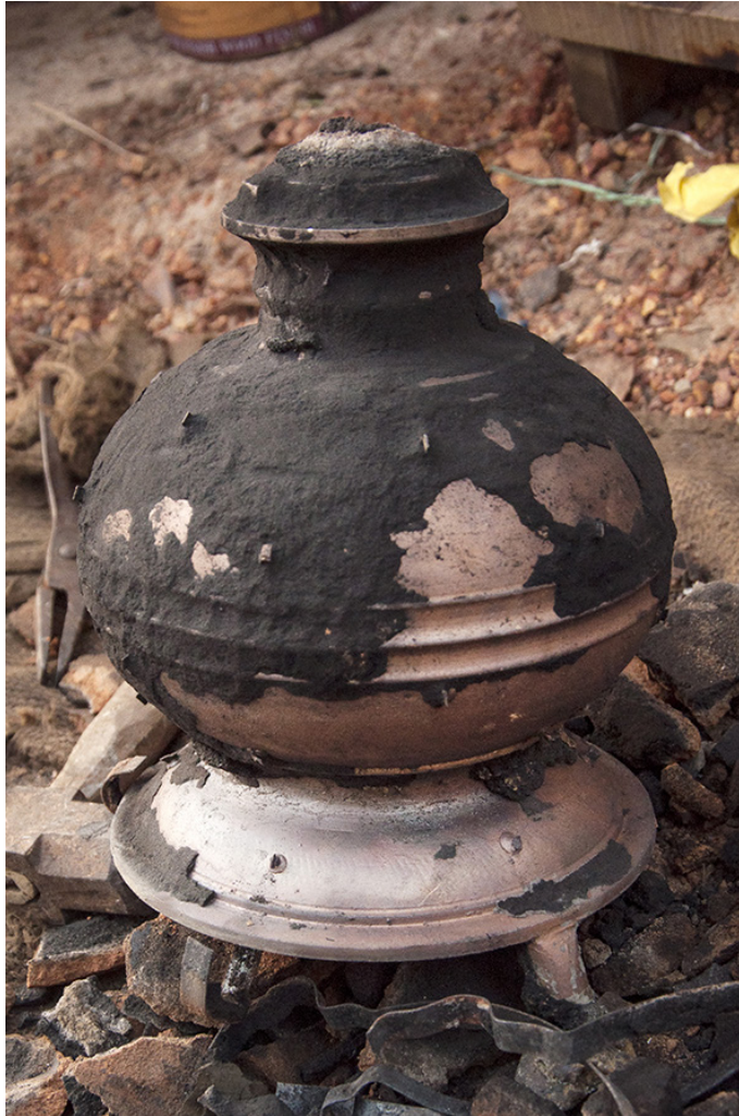
Image showing a freshly extracted brass ornament, from the mold.
