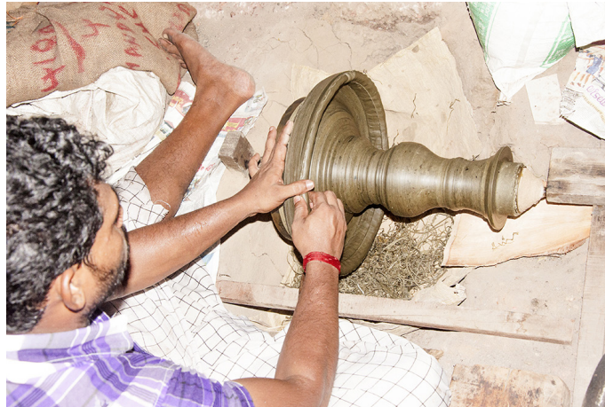
Artisan then corrects the wax model with reference to the diagram.
