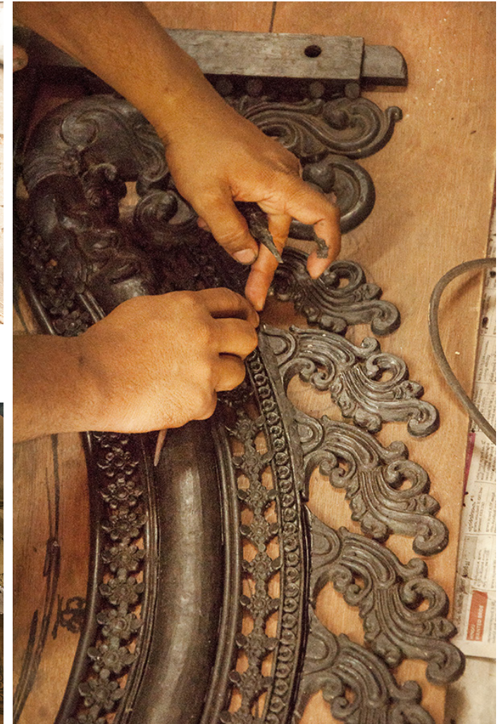
Artisan carving intricate details on the wax model, which has floral motifs.
