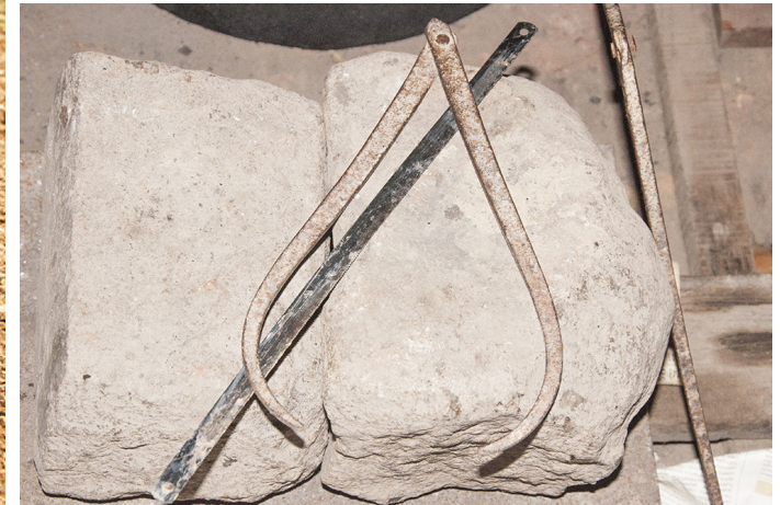
A large divider, used in measuring the accurate measurement of the wax models which are made.
