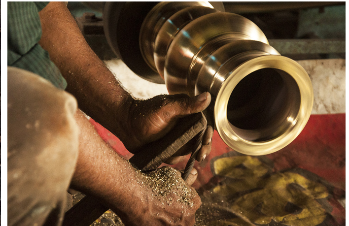
It is then finally buffed with a lathe machine, to give it a sheen look.
