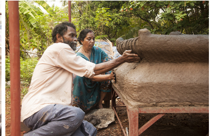
Image showing artisans applying wet mud over the wax model, to make a mold for pouring molten brass into it.
