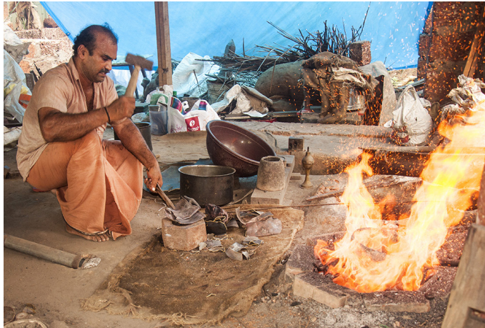
Artisan beating the sheet metal, to a smaller mass, so that it can be put into melting pot.
