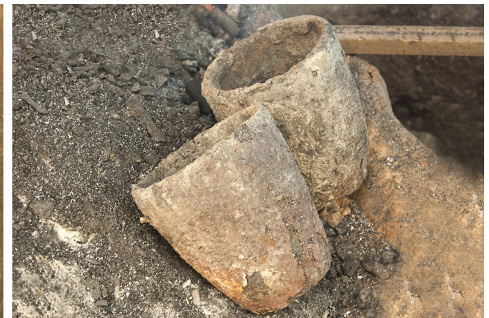
A heavy wrought iron container, in which other metals are melted, keeping it in a fire furnace.
