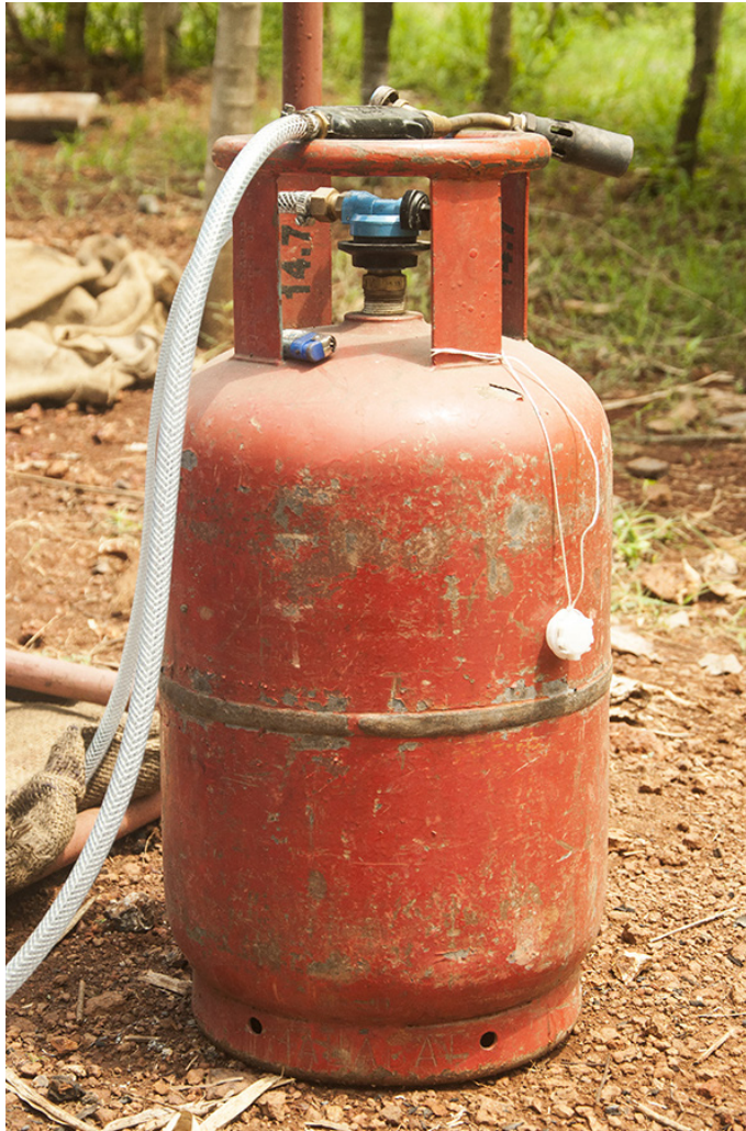
An LPG cylinder, used in burning up the wax and metal.
