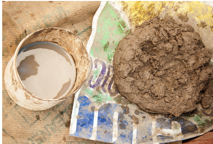
Clay and water, which are used in making of a mold.
