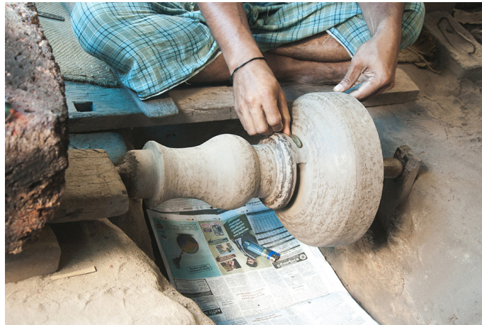
It is carefully packed in all the places, ensuring there are no leaks when the brass will be poured.
