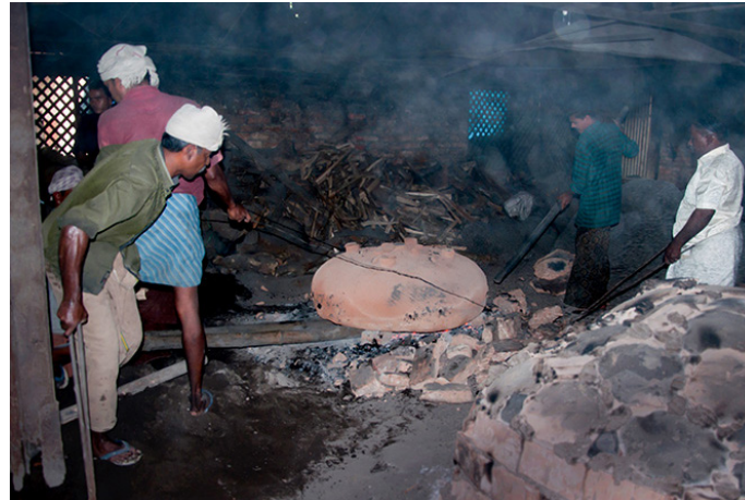
The mold is being moved to the pit made in the ground.
