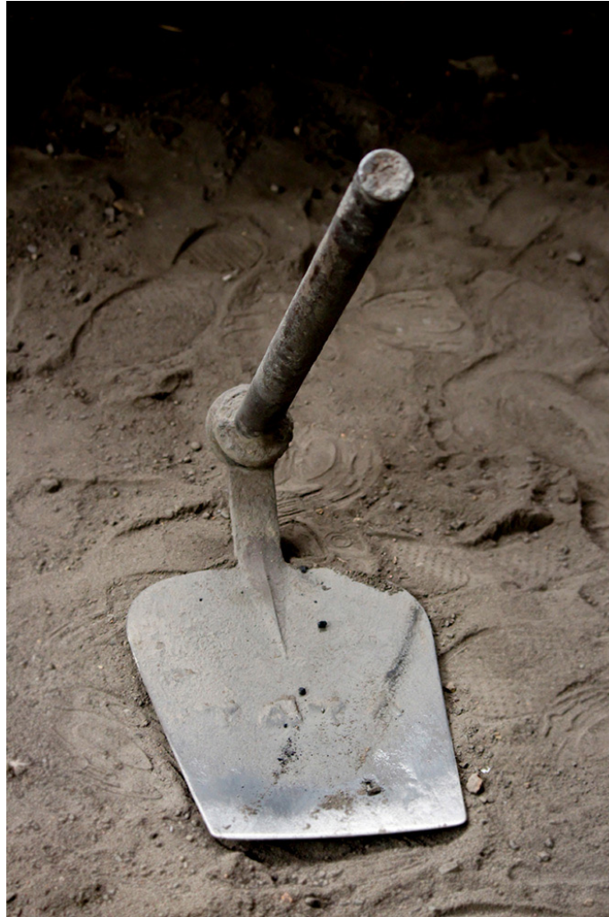
Spade: Used to remove mud or material from a place.
