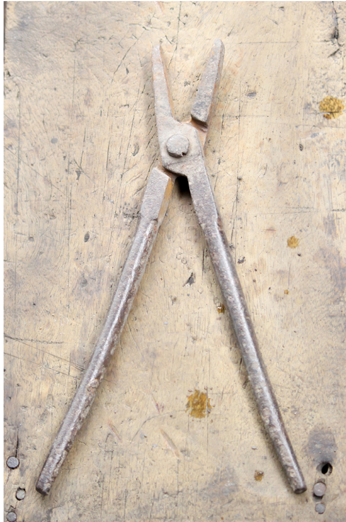
Tongs: To hold small size hot castings after removing from mold.
