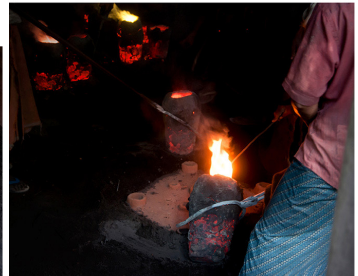
Molten metal is poured into the mold while the mold is still hot in order to avoid sudden cooling and breakage of the casting.
