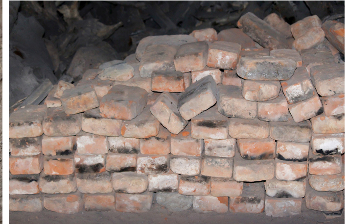
Bricks: They are used to construct a furnace around the mold to heat it.
