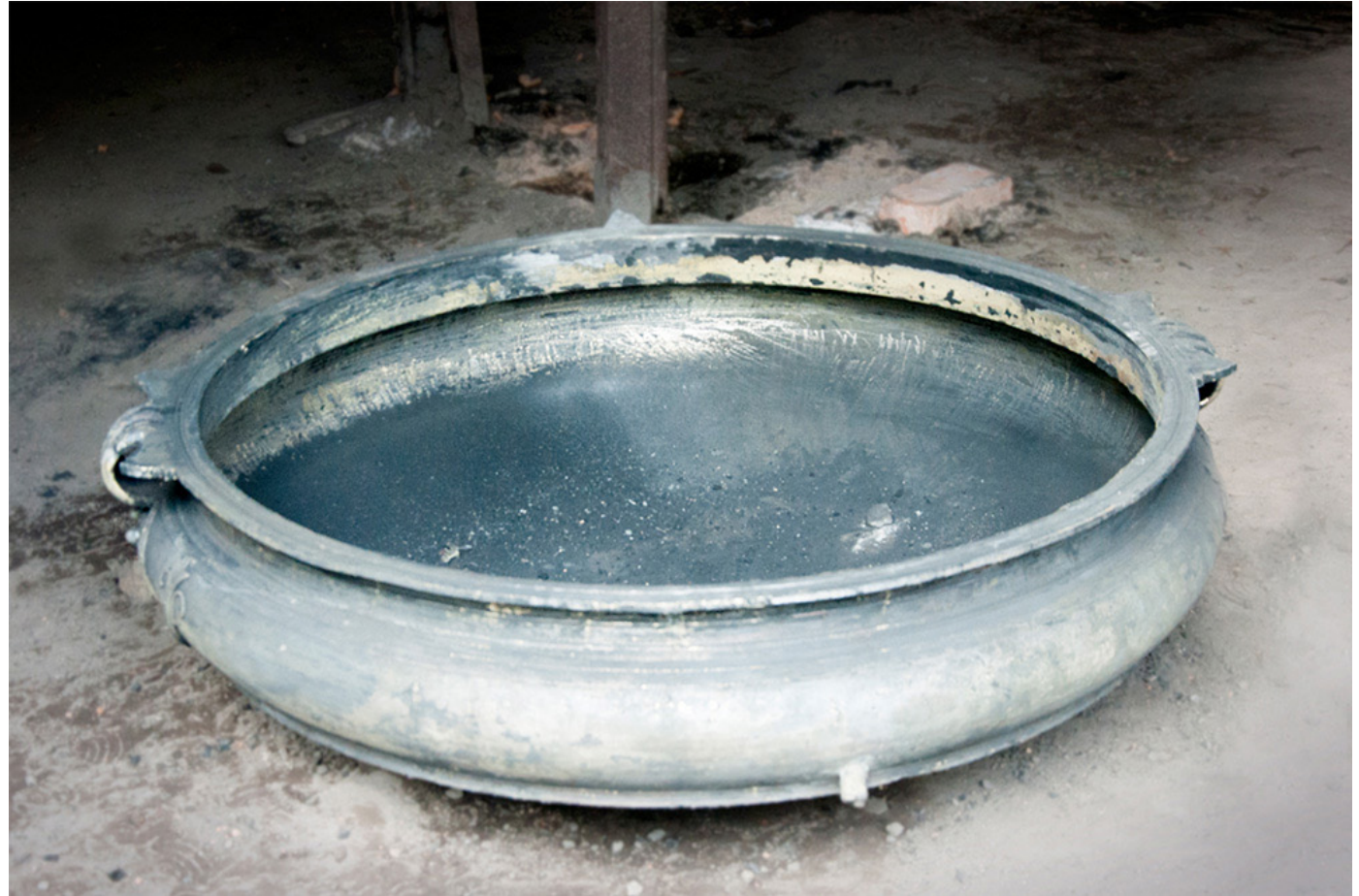
The casting is obtained but is unfinished and further processing is required.
