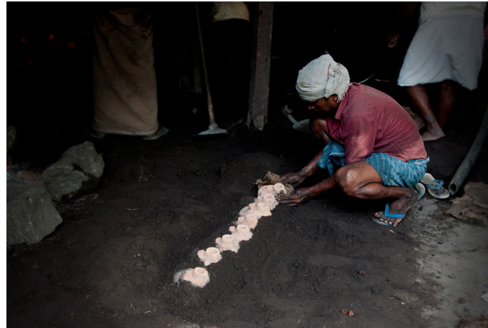
Small sized molds are being kept inside the clay, ready to put the casting.
