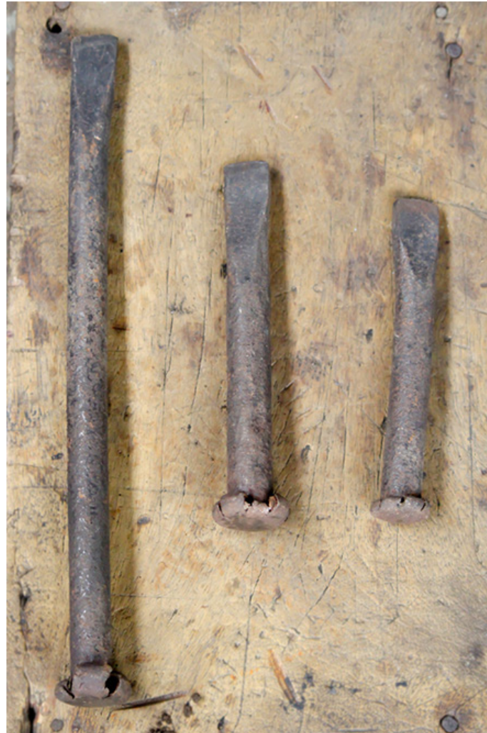
Chisels: Hand held flat blades, small ones are used for shaping the edges and bigger ones are used with hammer for engraving designs.
