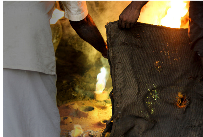
At the time of pouring molten metal, wet jute sack is used as a shield from flames and spilling of molten metal on to the feet of the craftsman.
