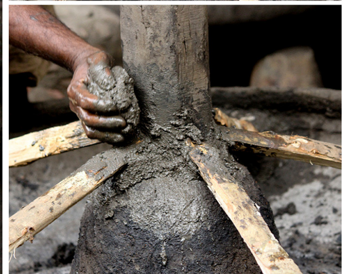
Clay is being applied to make the mold. Wood is used as support.
