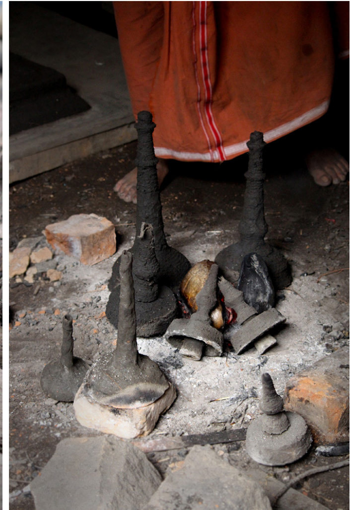
Clay molds of lamps are kept on hot charcoal to dry the clay.
