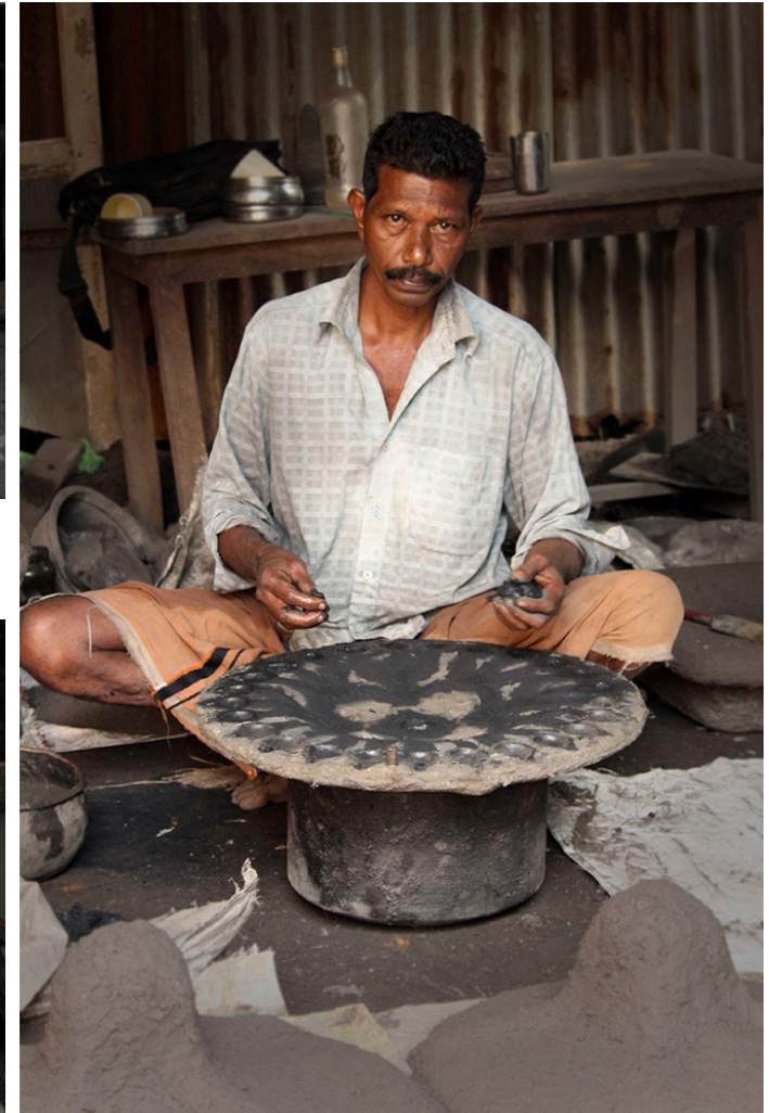
Wax is being applied by the artisan on the clay mold.
