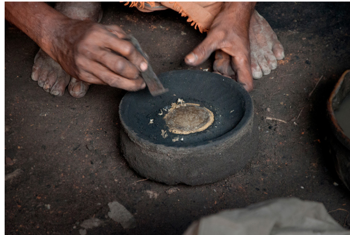
The mold is being given shape by the artisan by sculpting with a handmade tool.
