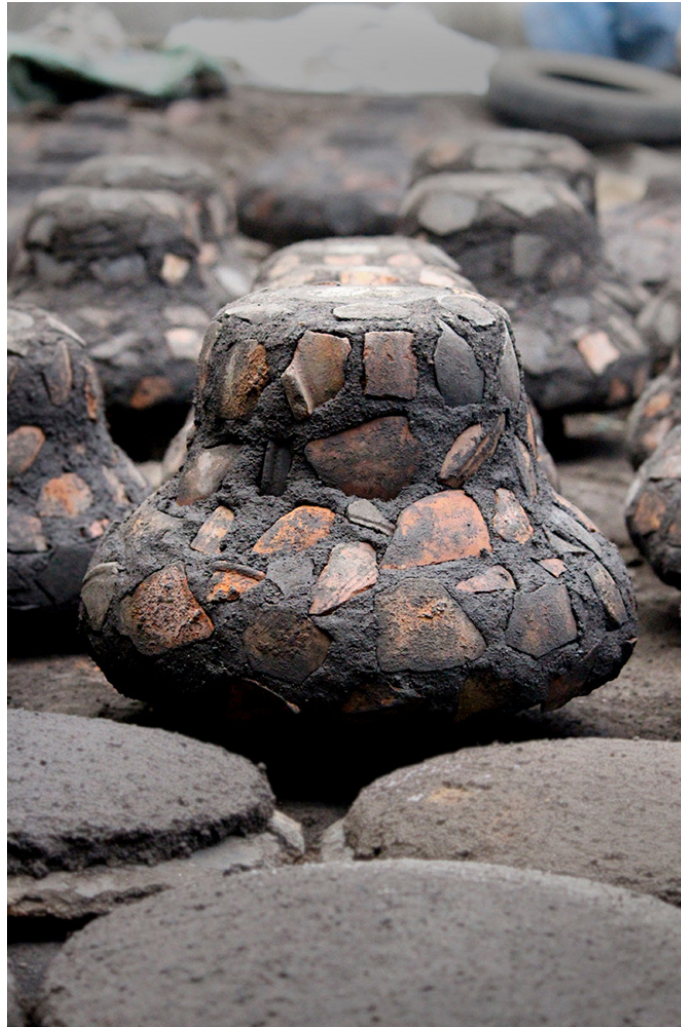
A clay mold having small pieces of tiles on its surface for strength.
