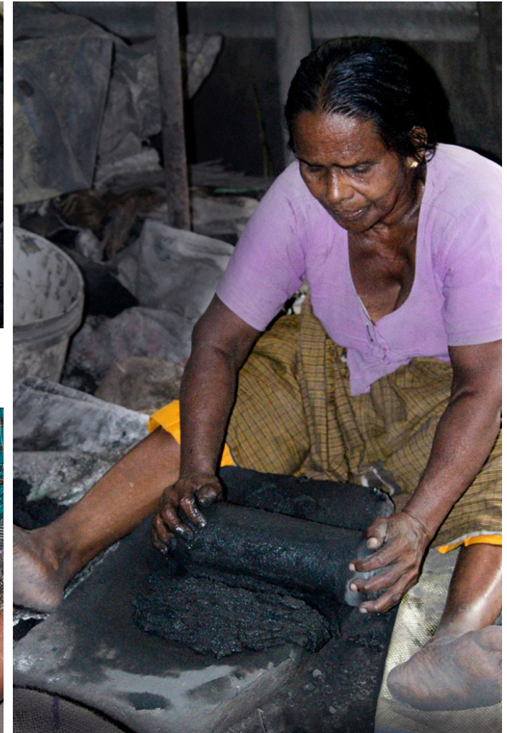
Artisan using roller to grind the clay pieces to powder.
