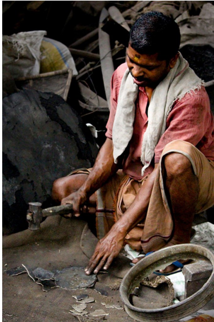
Scrap metal is beaten into tiny pieces to be melted into molten metal.
