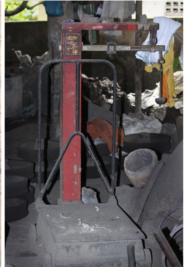
Weighing Machine: Used to measure the exact quantity of metal to be melted.
