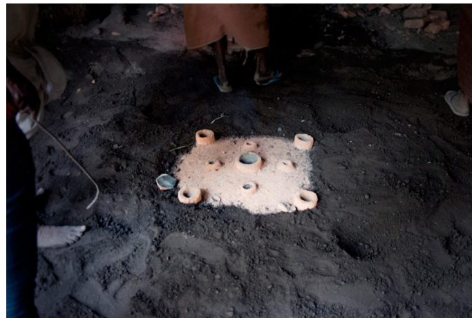
Mold is placed in the pit covering with sand all around firmly. Only the holes for pouring the molten metal and vent holes are spared and rest are covered completely with the sand.
