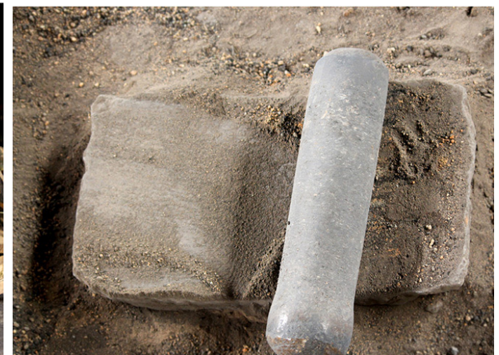
Roller Stone: It is hand operated grinder used for grinding the baked-broken mold clay pieces into powder.
