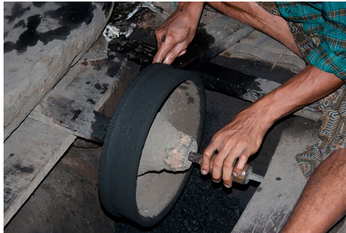
Artisan uses the powdered clay, adds water and makes it into a paste. This paste is made into the shape desired (in this case, urli). Artisan turns excess clay from the mold to remove excess and give it a definite shape.
