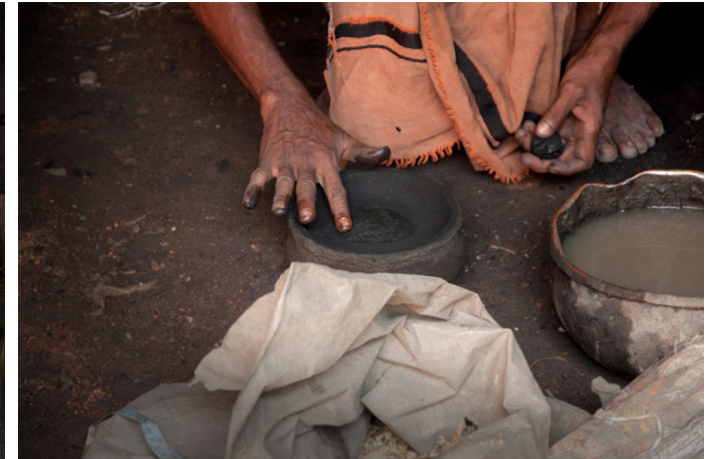
Artisan applying layer of wax on clay mold.
