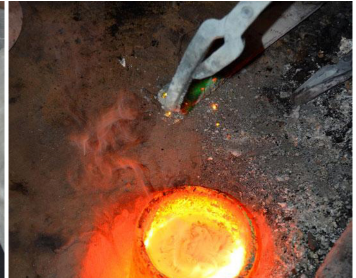
Molten brass is picked up from the furnace to be poured in the mould box
