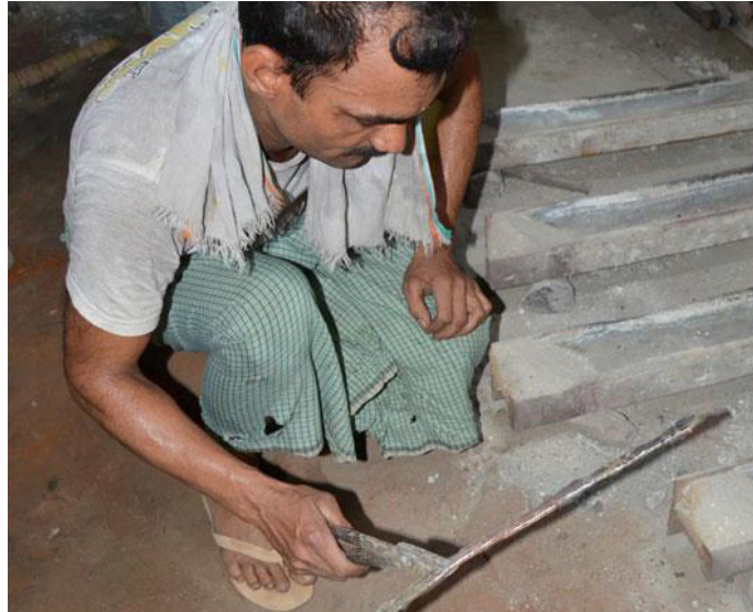
Testing the metal's ductility before pouring it out in strips
