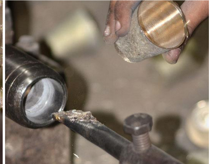
The filing tool attached to the lathe machine to scrap the tumbler
