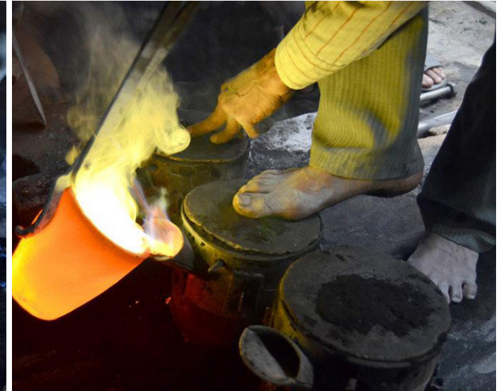
Molten brass being poured in the cavity
