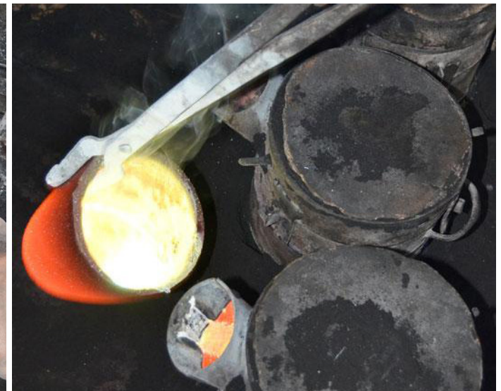
Molten brass being poured in the cavity
