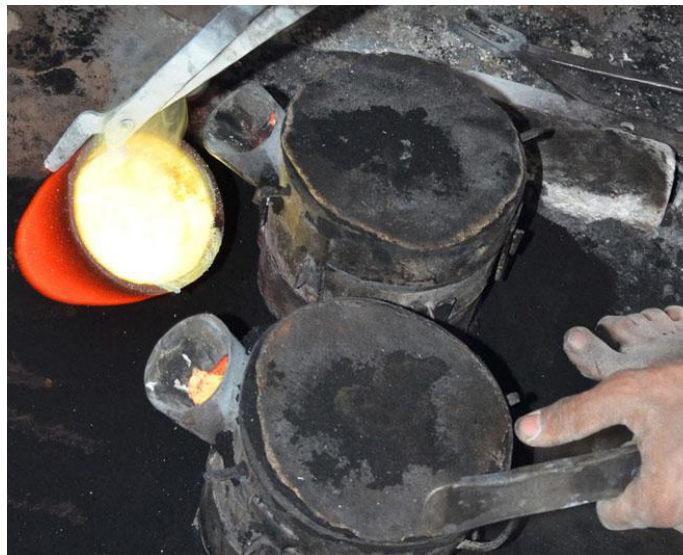
Molten brass being poured in the cavity
