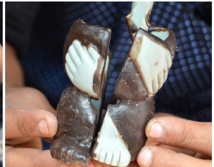
Mould for pen stand being made in wax
