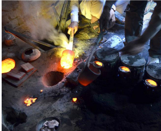
Molten brass being poured in the cavity
