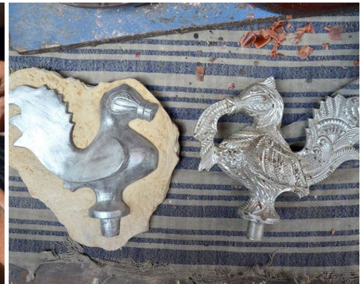
The 'master-copy' (mould) and its corresponding cast
