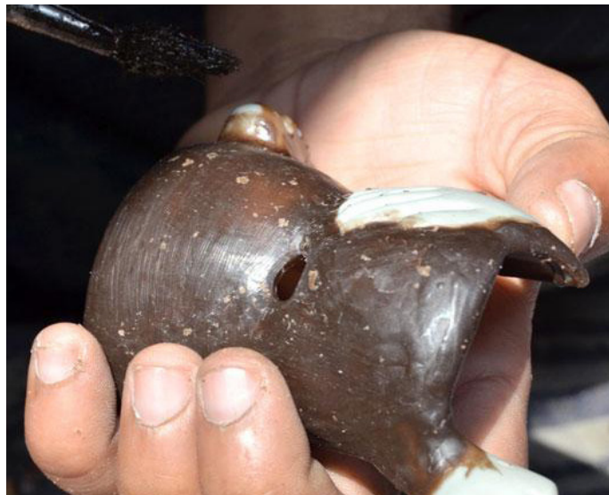
Mould for pen stand being made in wax
