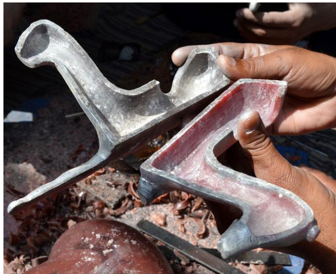
Two halves of the 'master-copy' for casting
