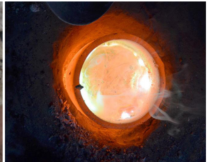
Pieces of brass being heated in the furnace for casting
