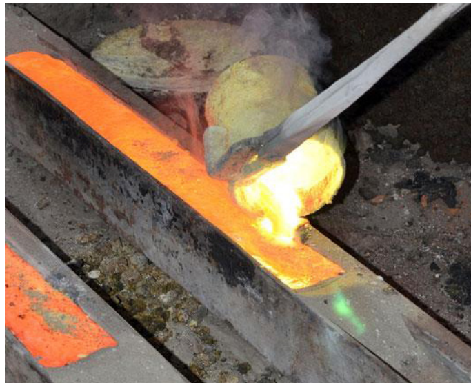
Molten metal being poured in the mould
