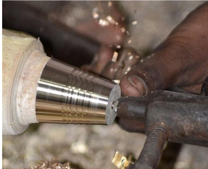
The wooden block attached to the headstock of the lathe machine to scrap the tumbler
