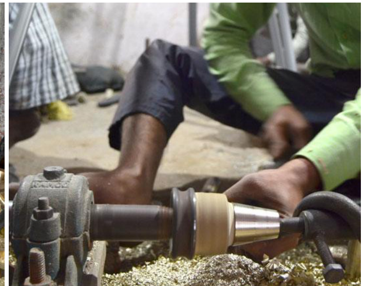
The wooden block attached to the headstock of the lathe machine to scrap the tumbler
