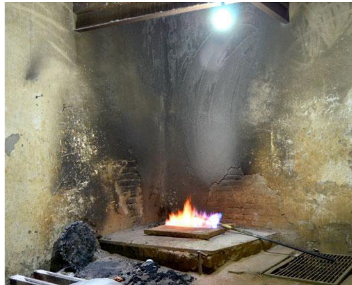
The furnace where brass is prepared by melting several metals
