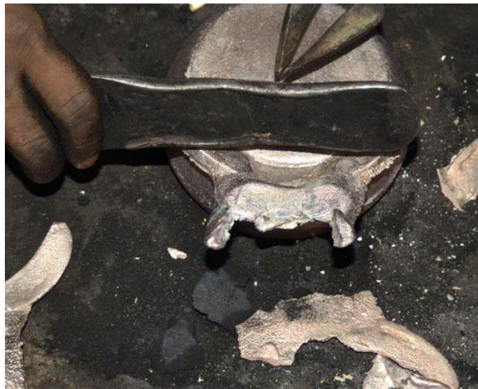
Gating' being hammered off from the cast
