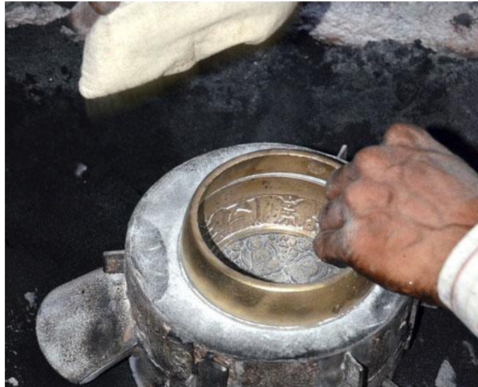
A karigar preparing the mould box with the 'master-copy' and sand
