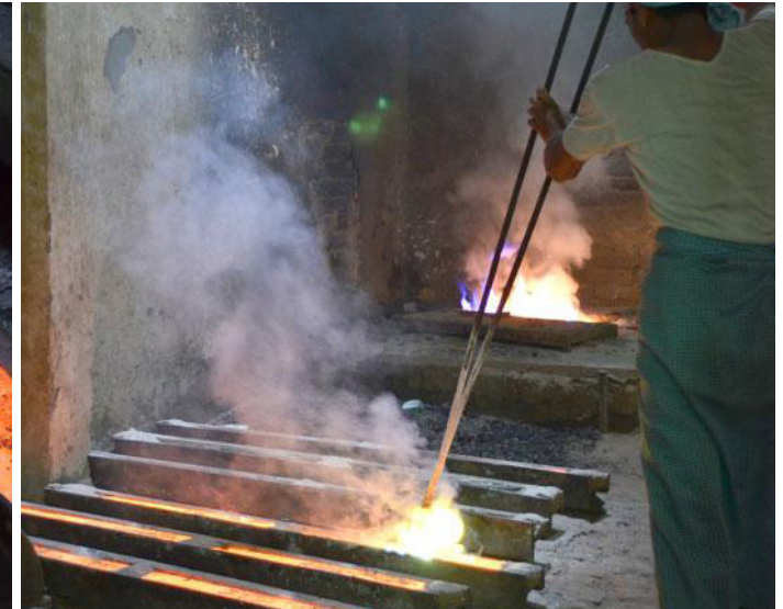
Molten metal being poured in the mould
