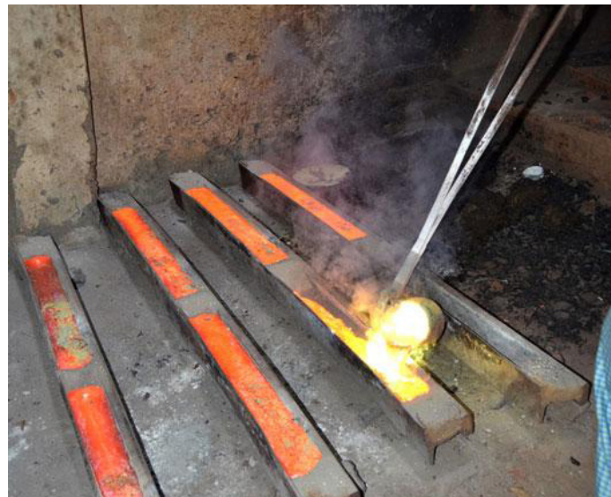
Molten metal being poured in the mould
