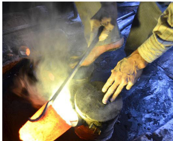
Molten brass being poured in the cavity
