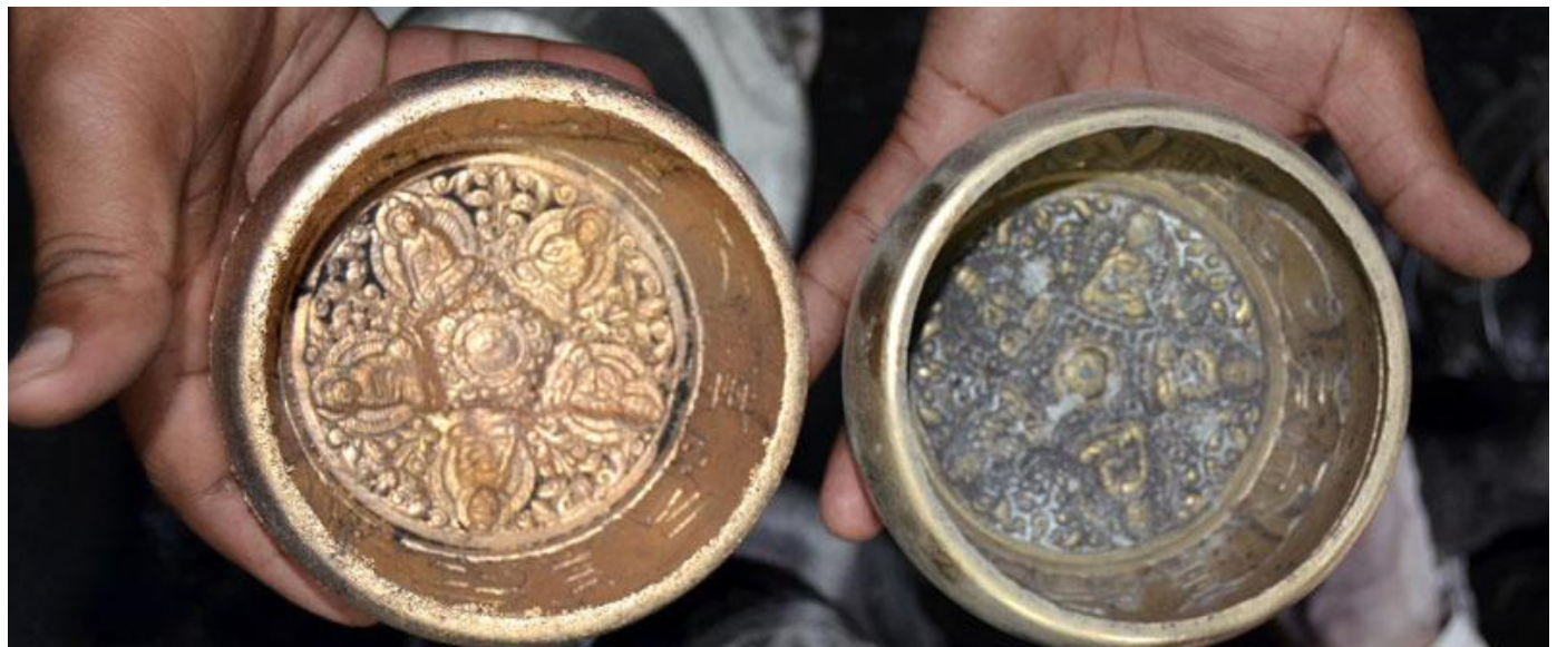
Brass mould ('master-copy') and cast
