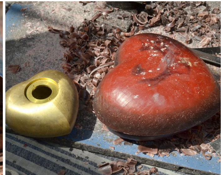
A brass cast heart and its corresponding wax mould (different size)
