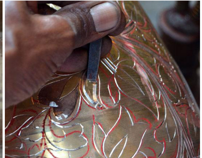
Pencil sketched design being engraved with varying depths for enamel
