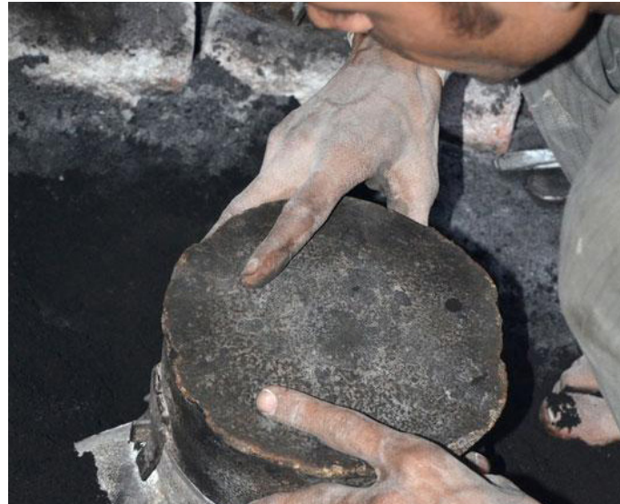
'Master-copy' is removed from the mould box and a cavity is created
