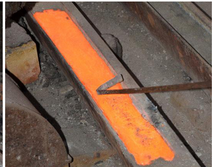
Molten metal being poured in the mould
