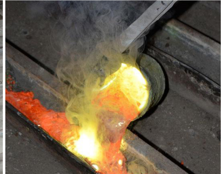
Molten metal being poured in the mould
