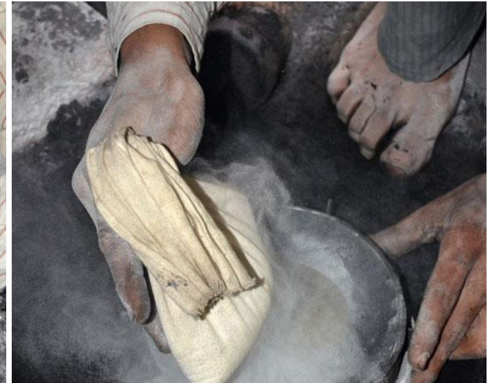
A karigar preparing the mould box with the 'master-copy' and sand
