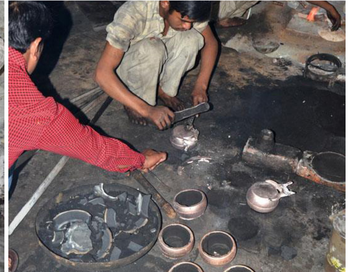
Gating' being hammered off from the cast
