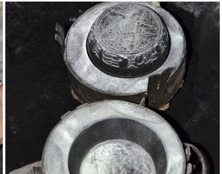
'Master-copy' is removed from the mould box and a cavity is created
