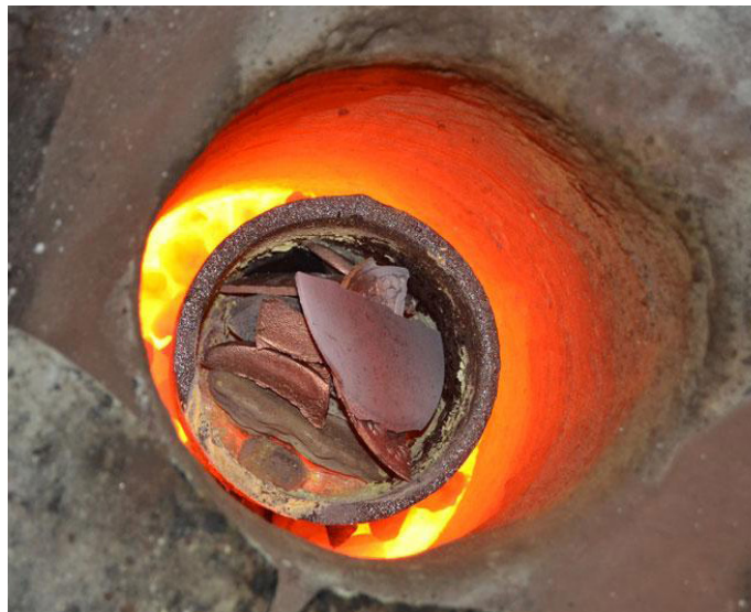
Pieces of brass being heated in the furnace for casting
