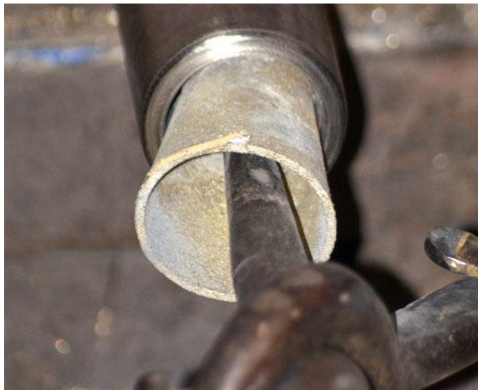
The filing tool attached to the lathe machine to scrap the tumbler
