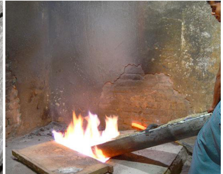
Brass shavings being poured in the furnace
