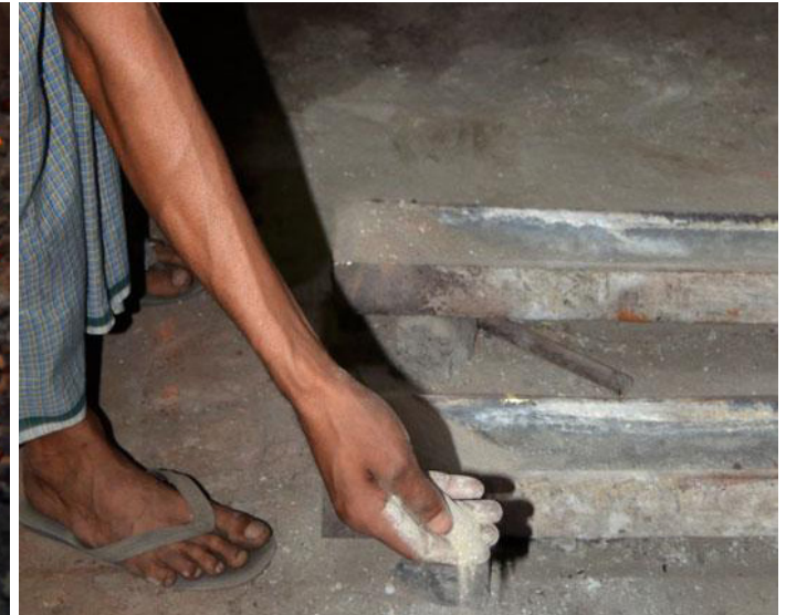
Putting sand in the mould to prevent molten metal overflow
