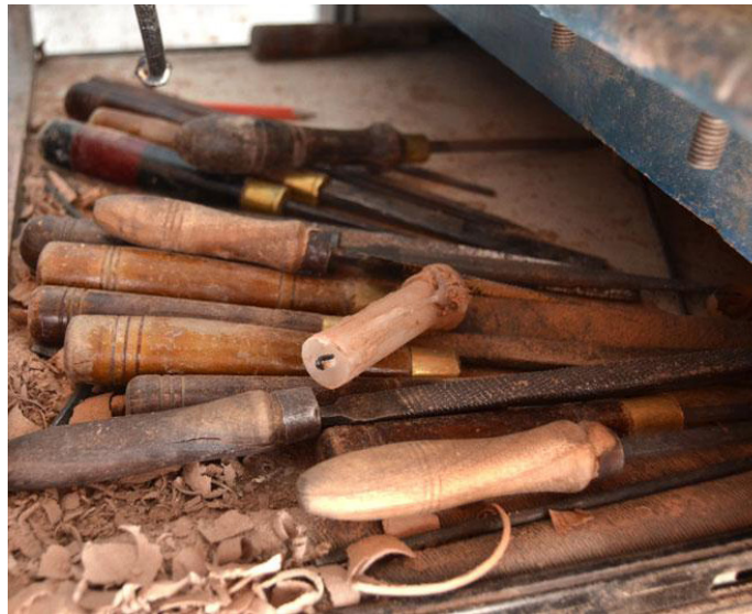
Tools for carving the wax and wooden moulds
