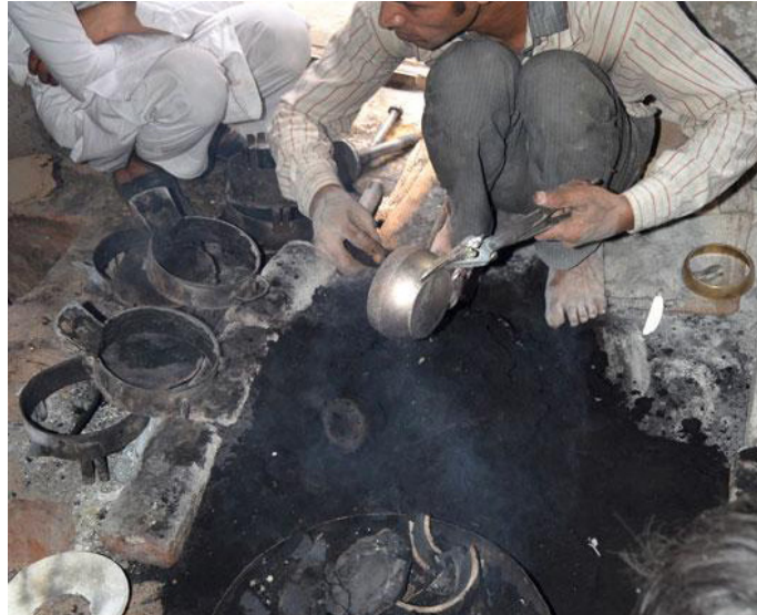
After cooling off, mould box is opened to remove the cast
