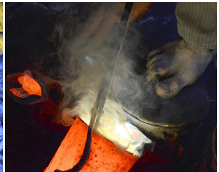
Molten brass being poured in the cavity
