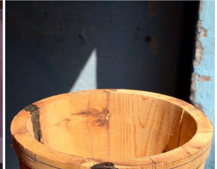
Mould being made in wood
