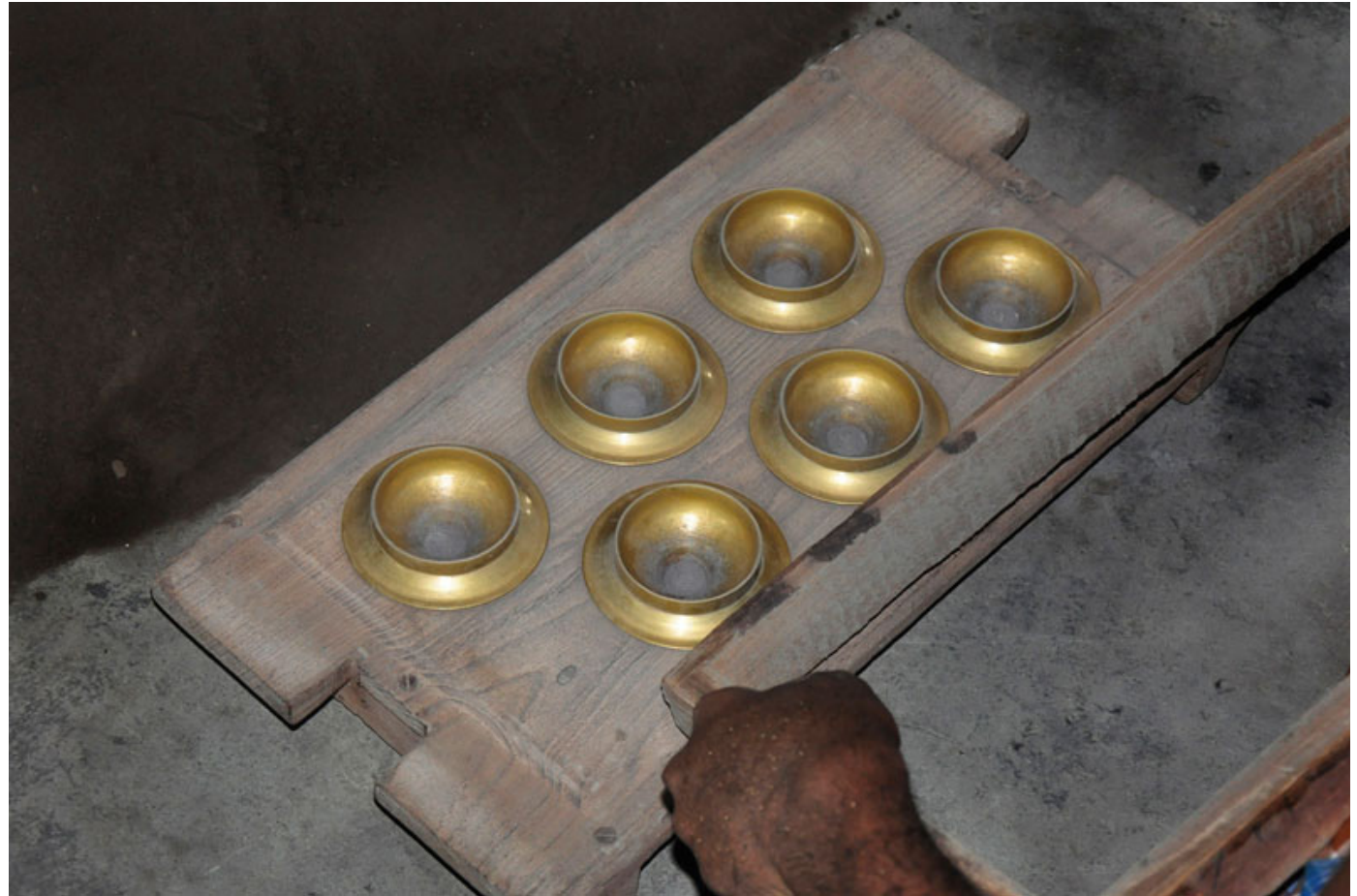
Articles are placed on the base to acquire the shape for the mould.
