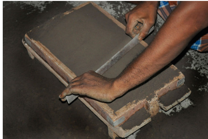
Excess mud is removed with a help of metal scale.
