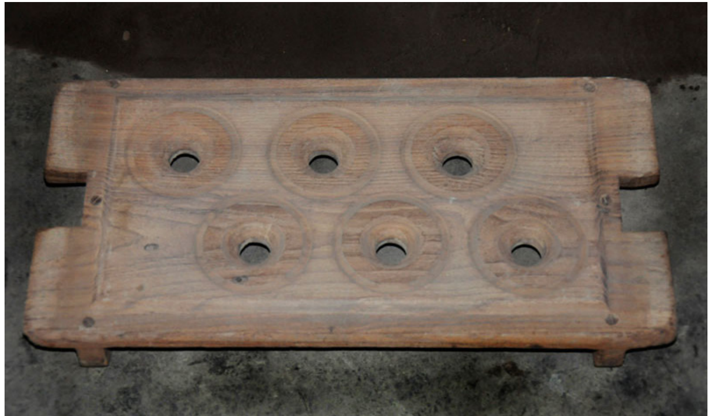
Wooden base is used to prepare the mould for casting the required brass article.
