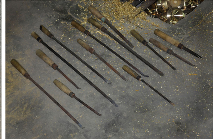
Different sizes of chisel to engrave designs.
