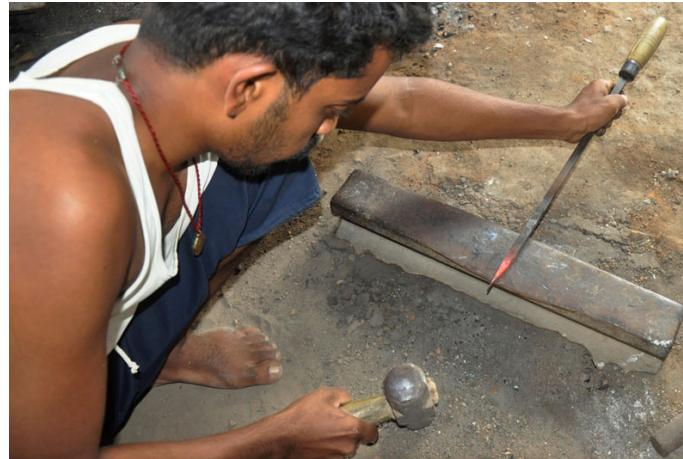
The chisel is heated and hammered to get the pointed edge.
