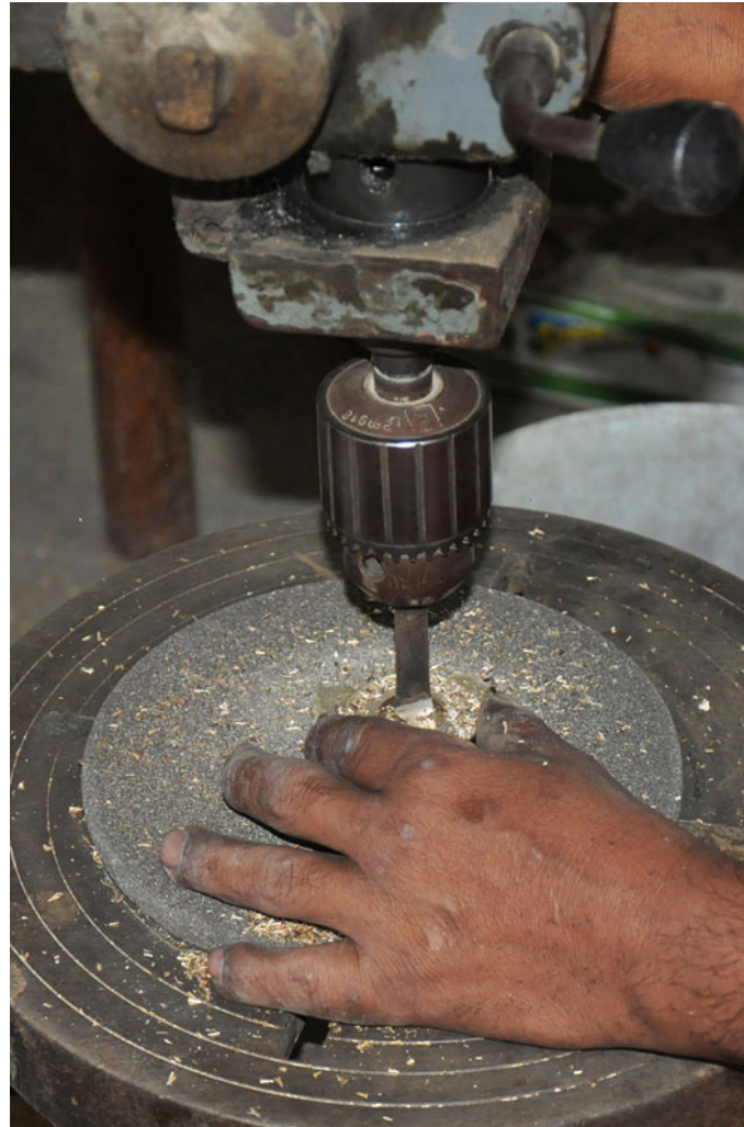
Internal tapping machine to carve the tread for joining the parts.
