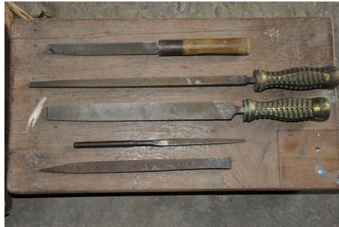
Varieties of filers/files are used to refine the product surface.
