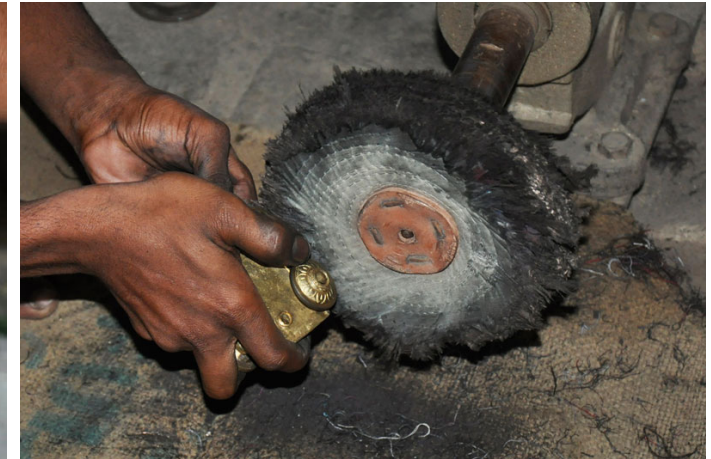
Buffing machine used for polishing the articles.
