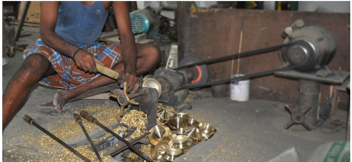
Artisan chisels the casted piece of metal to obtain the curved surface.
