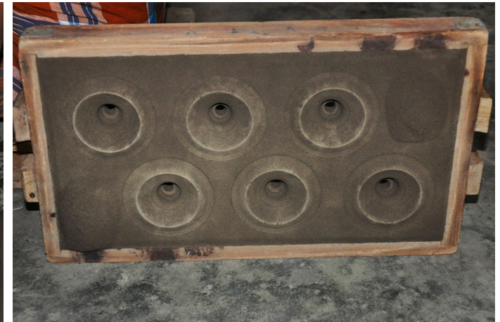
The mould is ready for the casting process.
