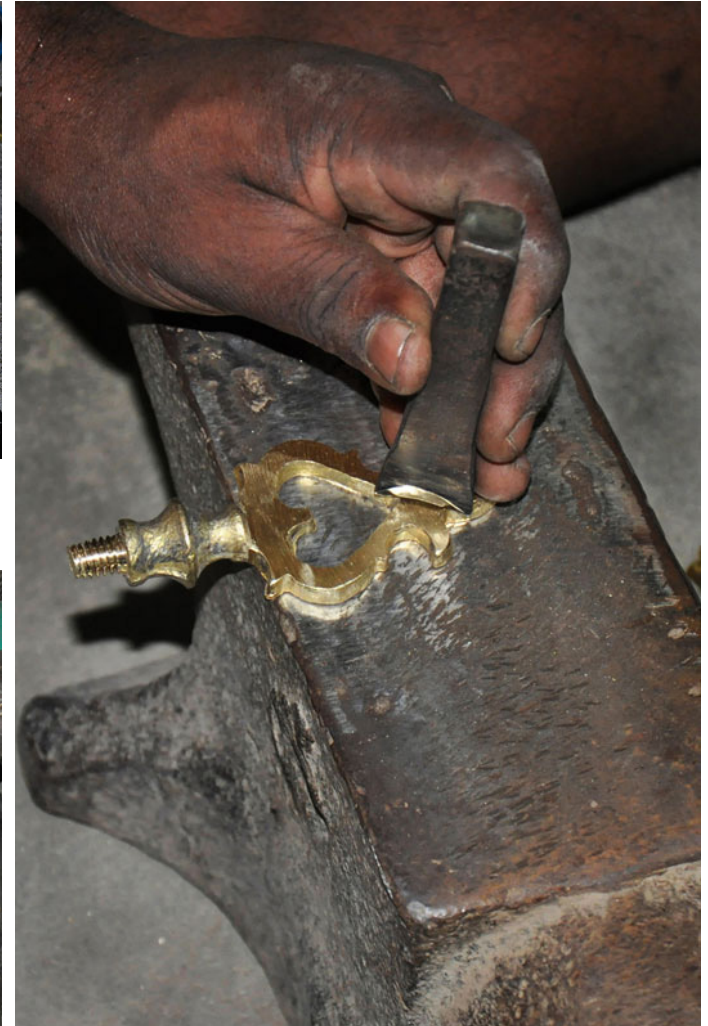
Article is chiseled to give required shape.
