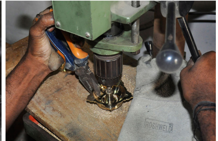
Internal tapping is done to join the parts.
