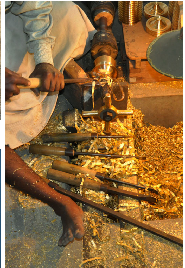
The lamp is carved to the required shape by chiseling.
