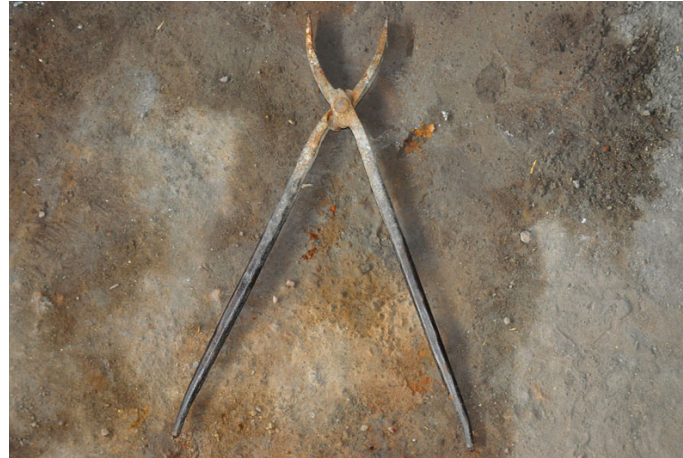
Tong used to hold the heated substance.
