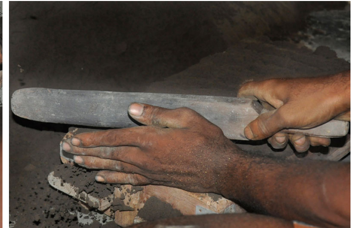
The mud is patted with wooden mallet to settle firmly in the wooden base.
