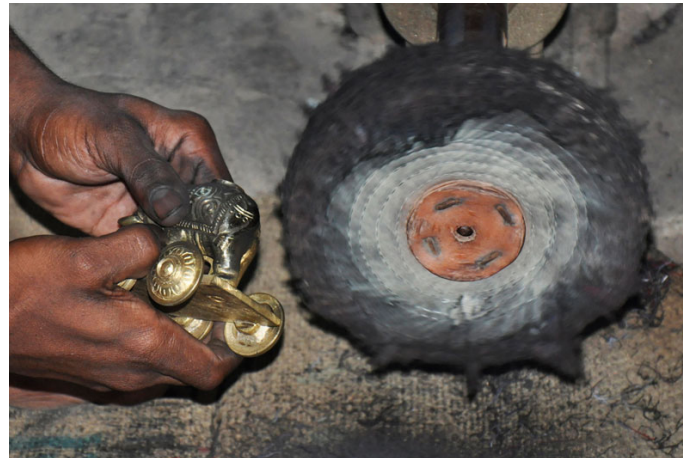
Buffing is done to smoothen the surface of the articles.
