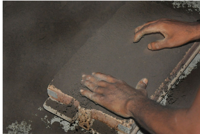
Mud is filled in the wooden base.
