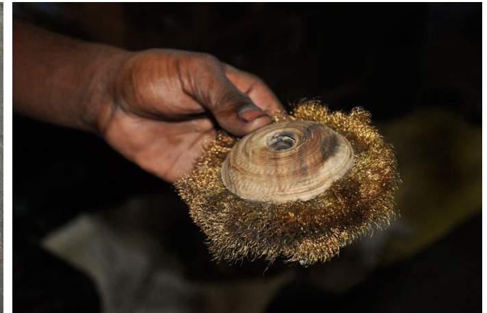
Brass fiber brush used in washing the product.
