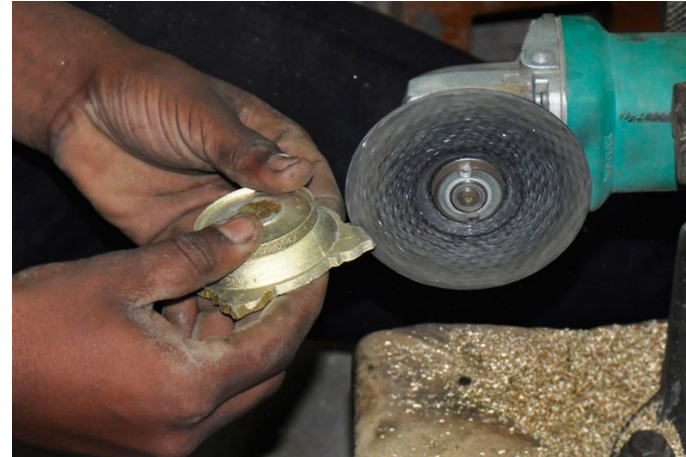
Edged are refined for smooth finishing.
