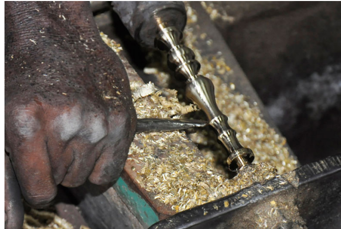
Brass Lamp stand is chiseled to the required shape in the turning machine.
