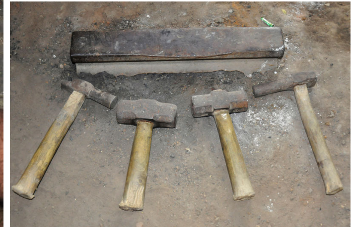
Verities of hammer used for hammering to shape the product.
