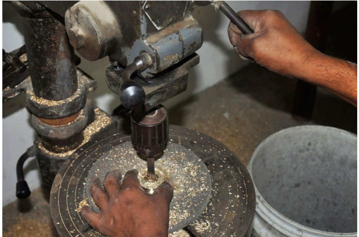
Internal tapping is made to join two piece.
