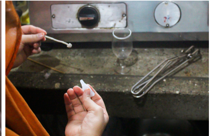
Artisan stick the wick using glue in the center of the container.
