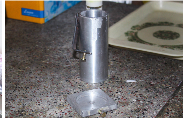
A mold to hold the melted wax.
