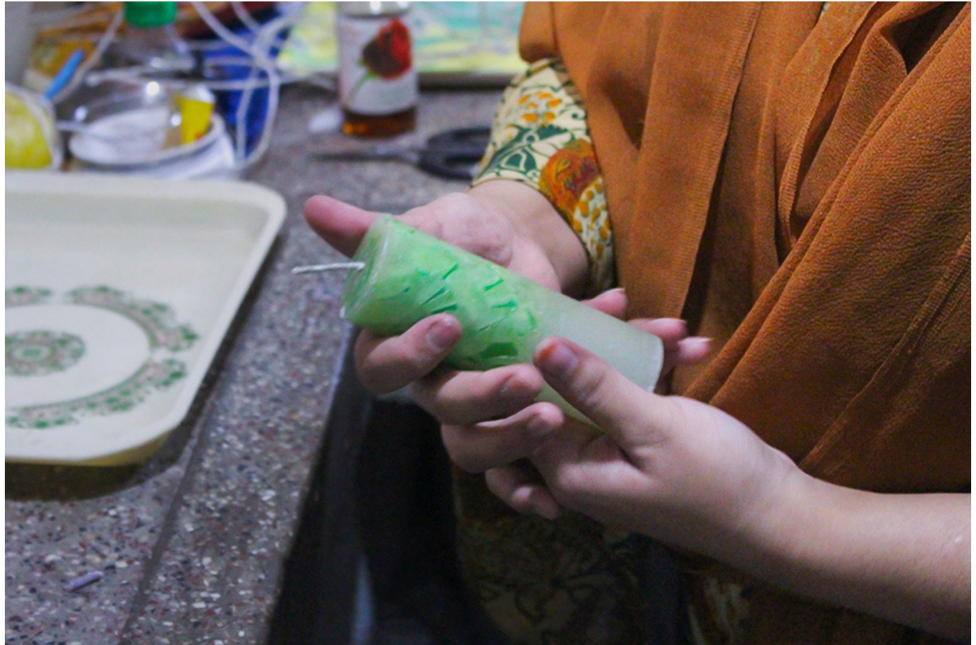
Artisan removes the completed candle from the mold.
