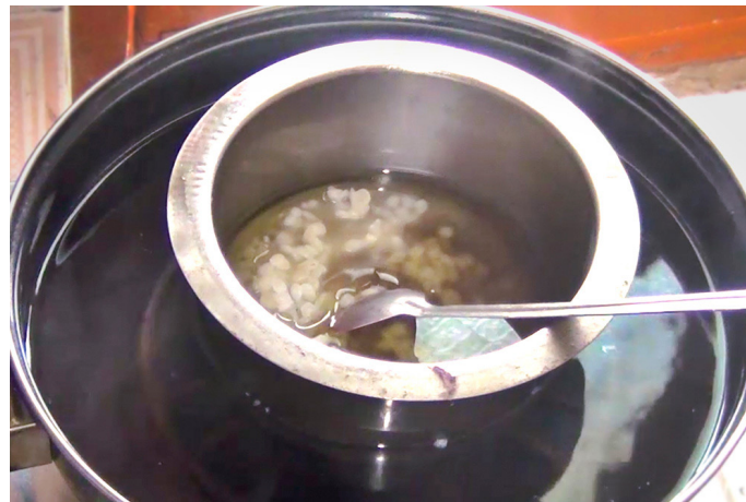
Paraffin wax chips were melted at 59 degree Celsius.
