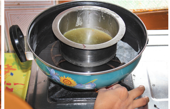
Artisan turn on the flame to high so that the water boils for melting the wax.
