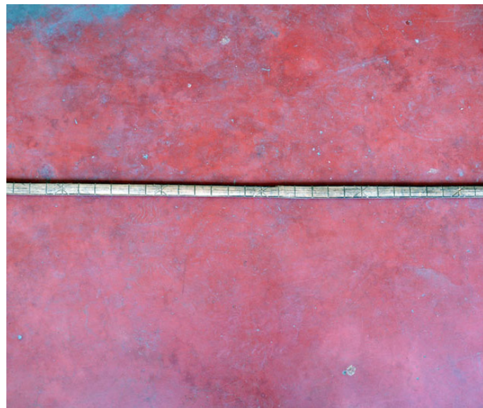
Local made scale made out of bamboo for measurement.
