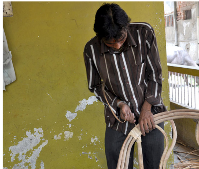
The parts are joined using thin cane strip.
