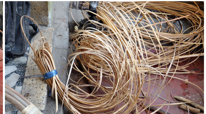
Processed cane skin used to combine/bind the different parts of chair.
