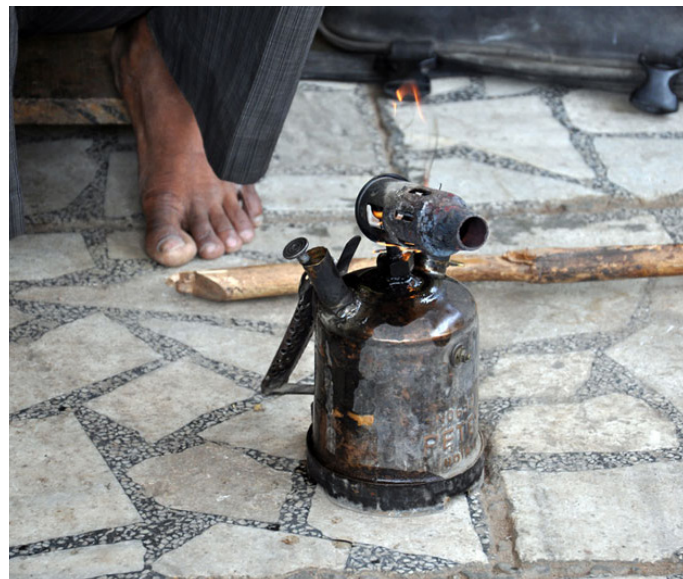
Kerosene burner used to produce the fire.
