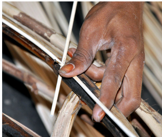
Initial joining of cane to the frame.
