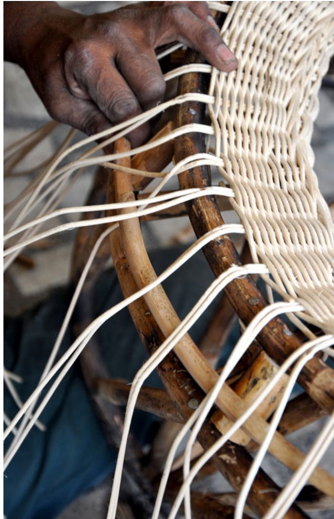
Thin processed cane is flexible to create patterns.
