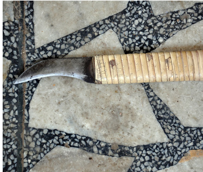
Chaaku used to smoothen the surface.
