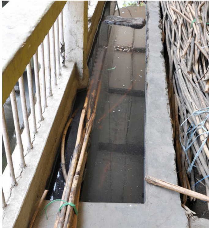
Bamboo sticks are soaked in water for 2 hours.
