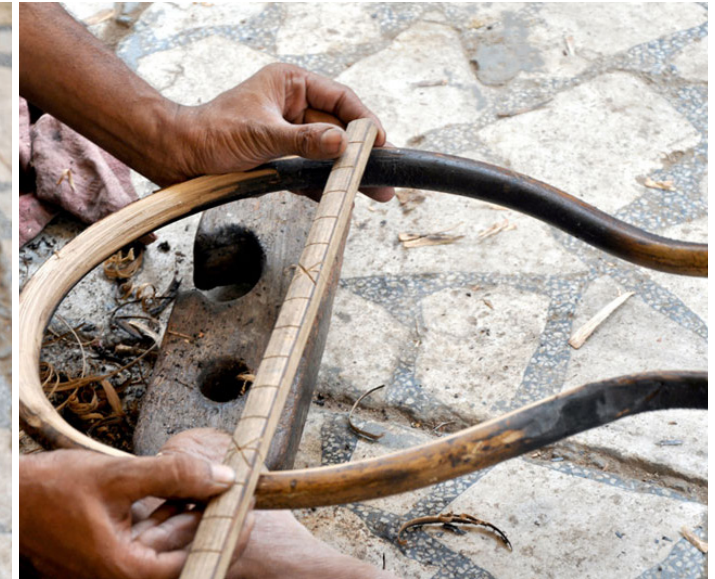
The burnt skin layer is removed and smoothed.
