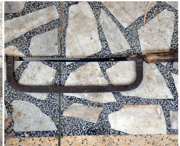
Hacksaw used to cut the dry bamboo.
