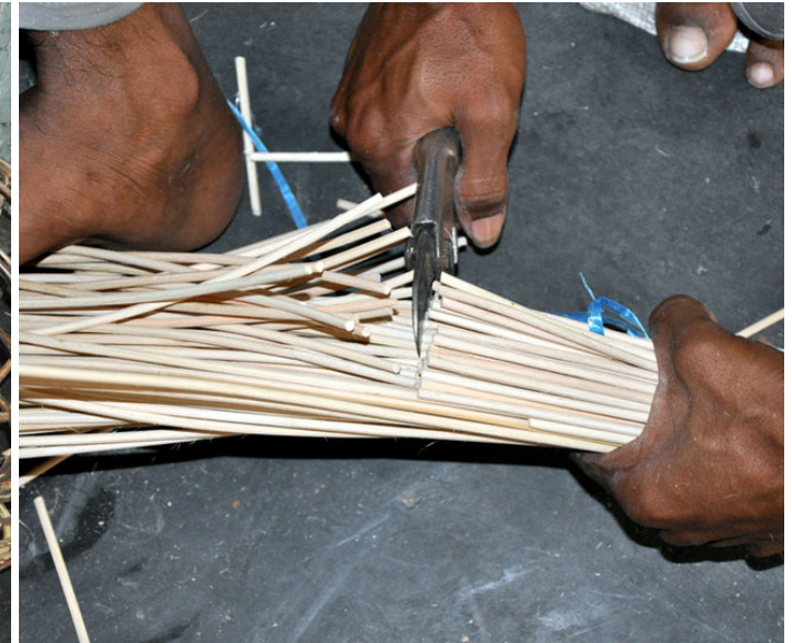
Cane is cut into different sizes.
