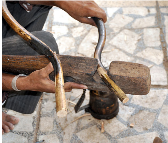
Measuring the Surai (motif name of shaped bamboo) to get accurate shape.
