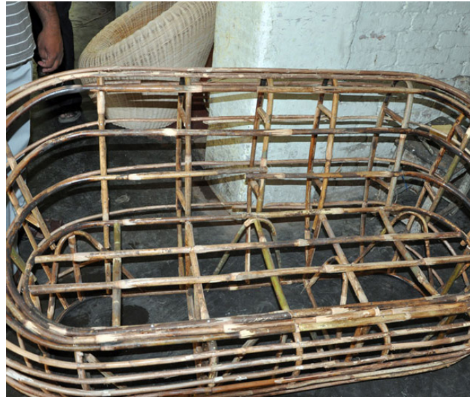
The bamboo frame is ready for cane rounding.
