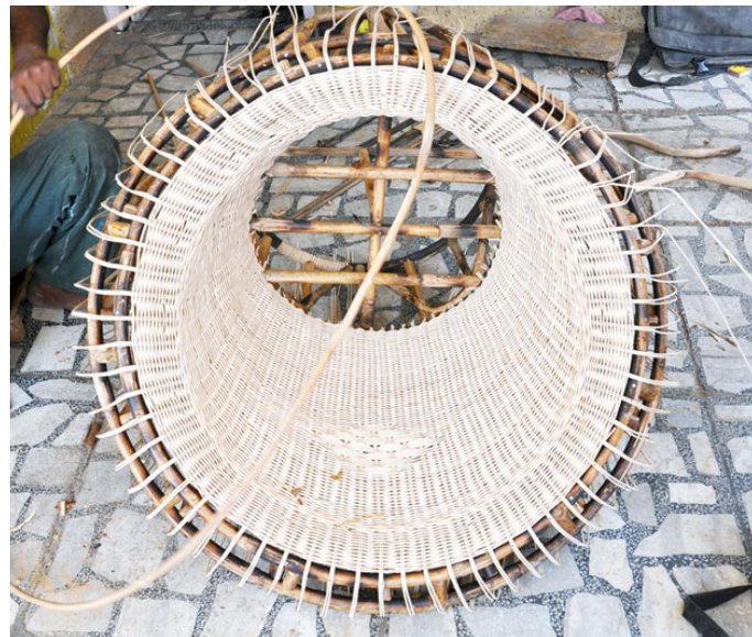
Adding mota cane (thick cane) to the furniture for better support.
