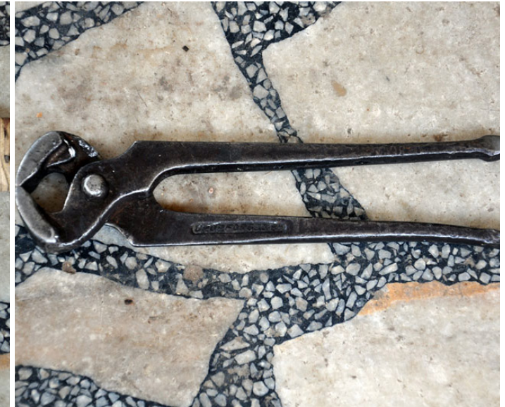
Jamura is the tool used to pull the cane while weaving.
