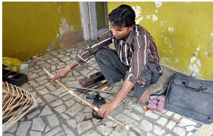
Heated bamboo is easy to bend.
