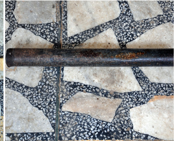
A metal rod used to bend the bamboo while heating/burning the bamboo stick.
