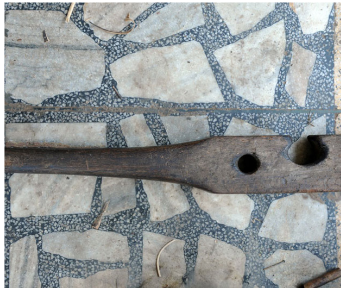
Mungri used in shaping process.
