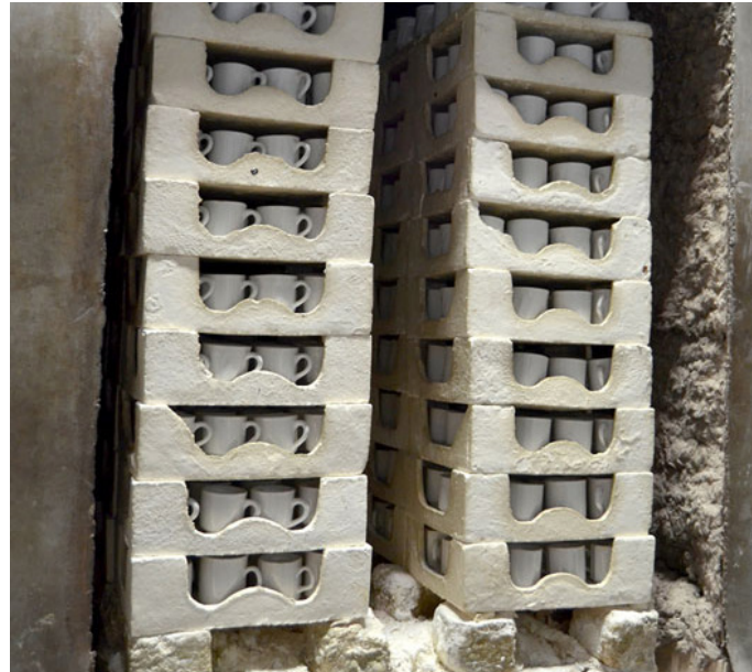
The fired cups to be removed from the cooling end of the furnace.
