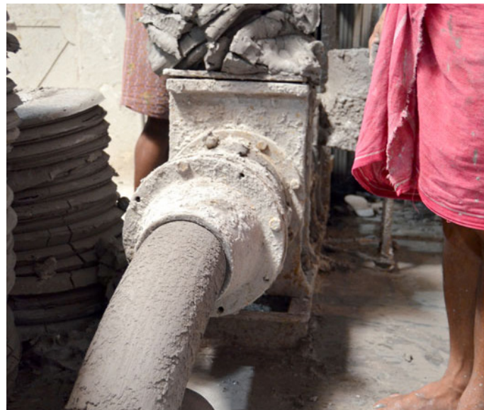
Clay being rolled out from a pug-mill.
