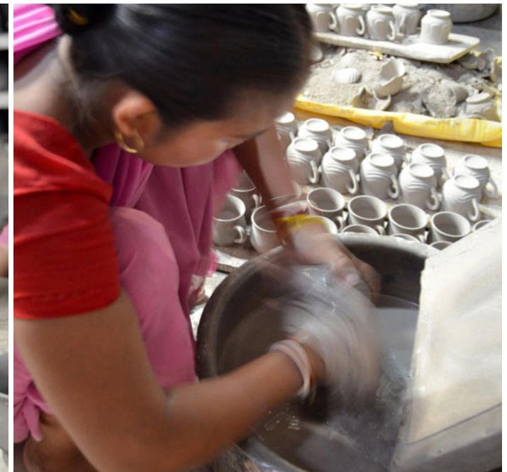
A woman finishing ('cleaning up') the rough edges of cups.
