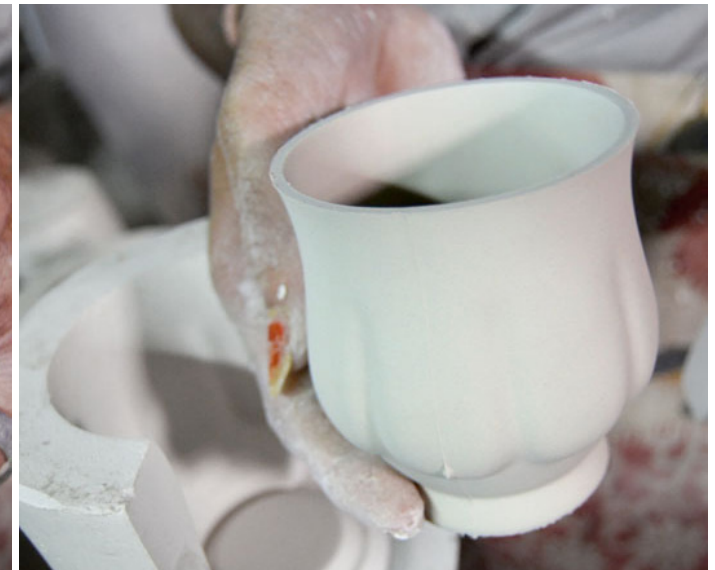
Clay cast being removed by opening up parts of the mould that were held together with rubber bands.
