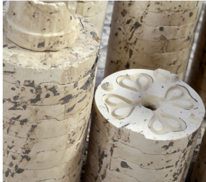
Moulds for casting handles for cups.
