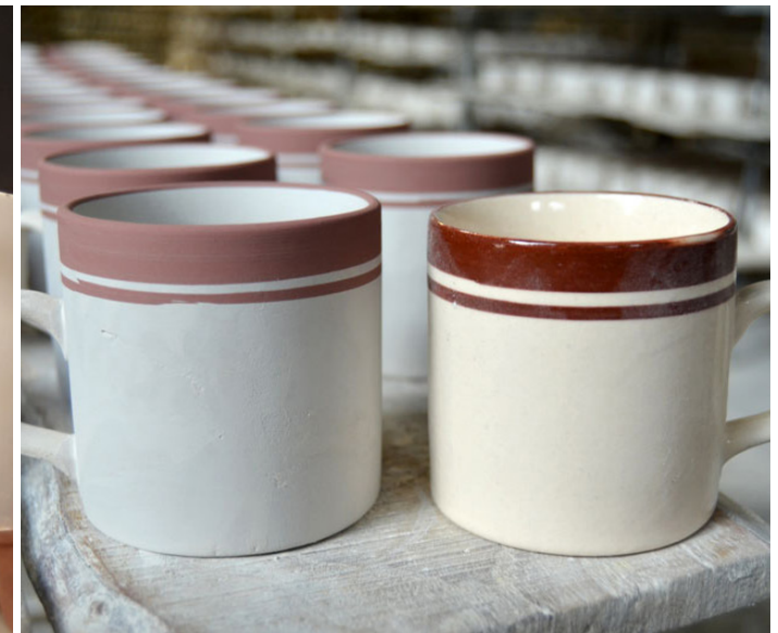
Difference between an unglazed and glazed cup.
