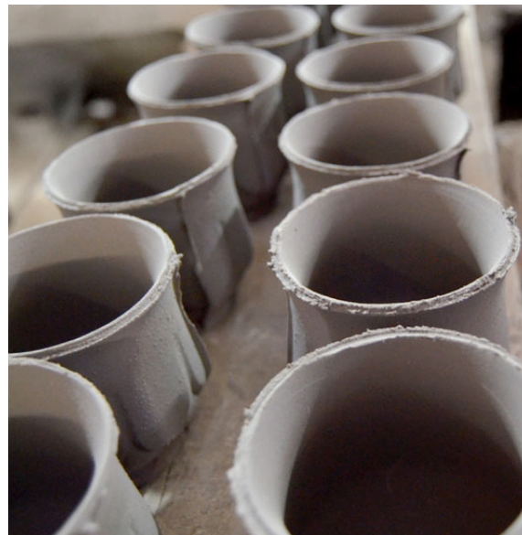
The clay cups, cast from the POP moulds.
