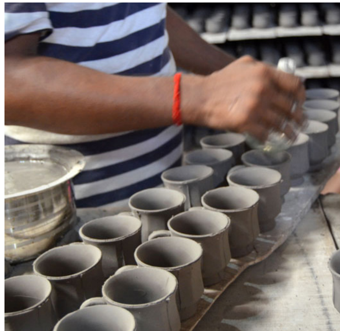
Clay handles just joined on cups.
