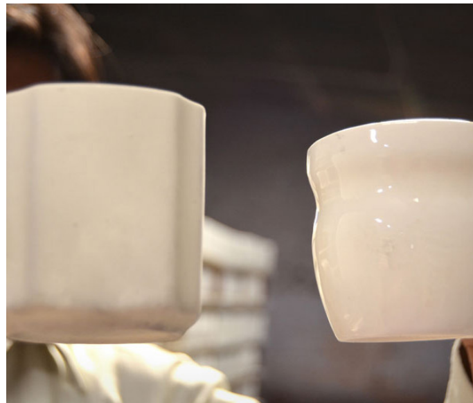
Difference between an unglazed and glazed cup.
