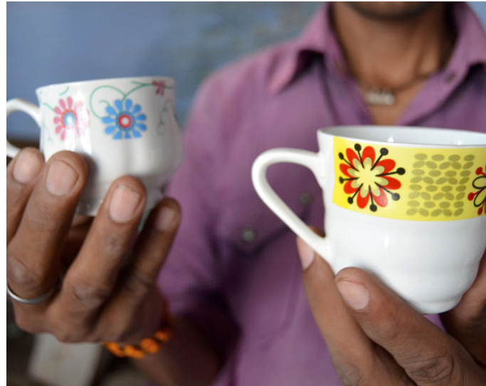
Difference between a cup with unfired sticker and fired sticker.
