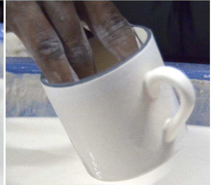
Hand-painted cups being dipped in clear glaze.
