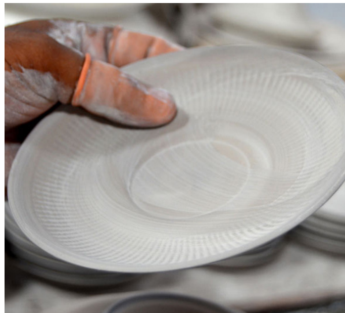
A saucer cast from a mould.
