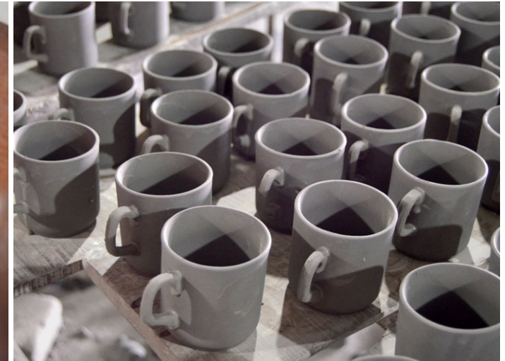
Clay handles just joined on cups.
