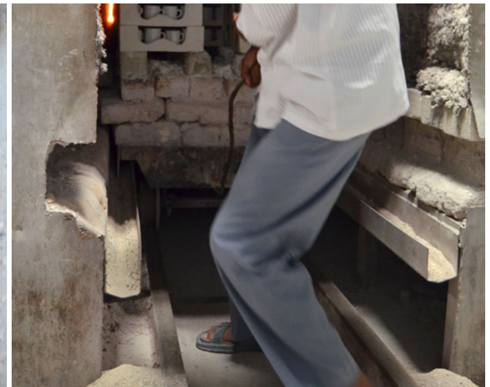
A karigar pulling out the car from the cooling end of the furnace.
