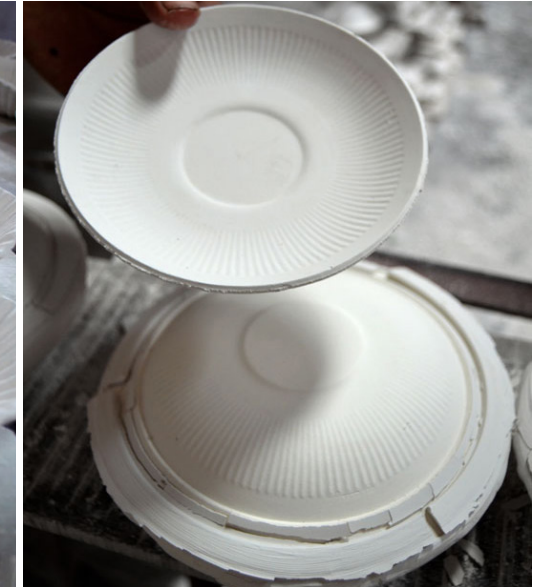
A saucer cast from a mould.
