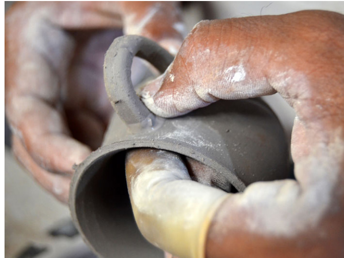
A clay handle being joined on a cup.
