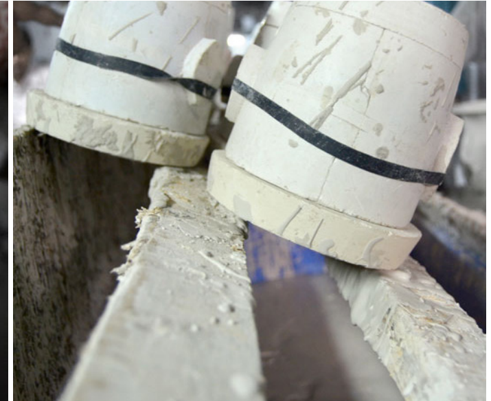
Excess slip being poured out from the mould.
