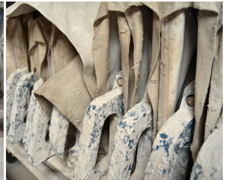
Clay discs in the filter press (pressed between metal plates and canvas).
