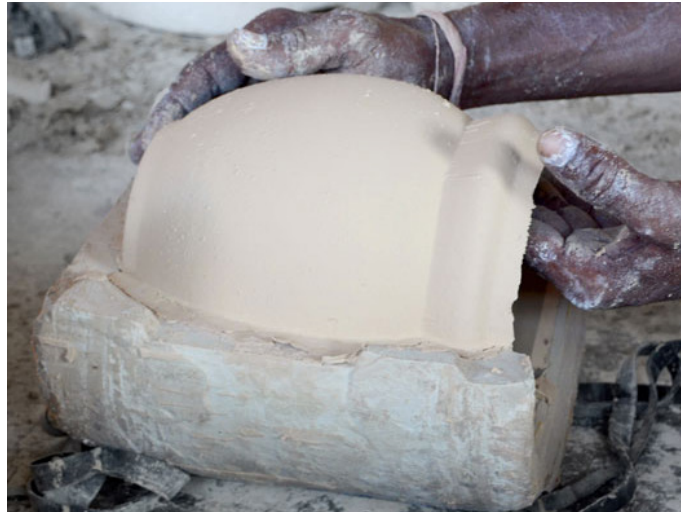
The karigar removing the clay pot from the mould.
