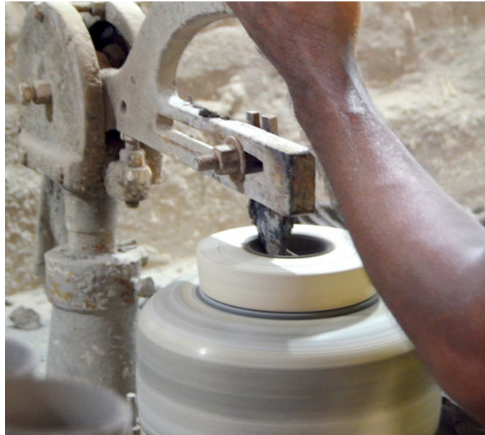
Clay being 'thrown' in along the walls of the mould using a hand tool on a rotating wheel-head.
