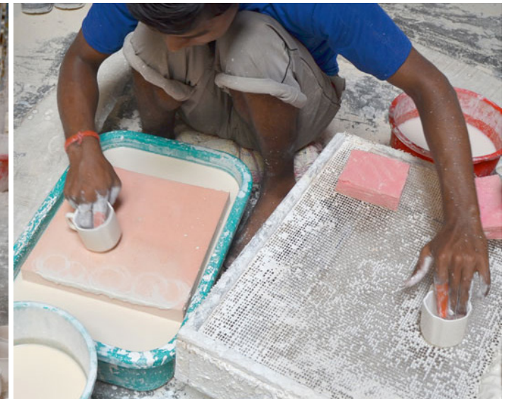
A karigar rubbing off the glaze from the bottom to prevent it from sticking on the furnace shelf.
