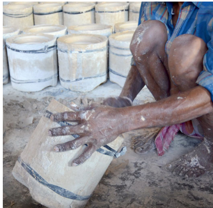
A karigar opening up parts of the mould that were held together with rubber bands.
