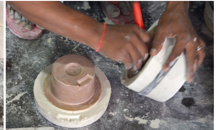
Soap and oil being brushed on the mould.
