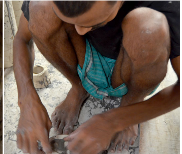
Clay handles being removed from the mould.
