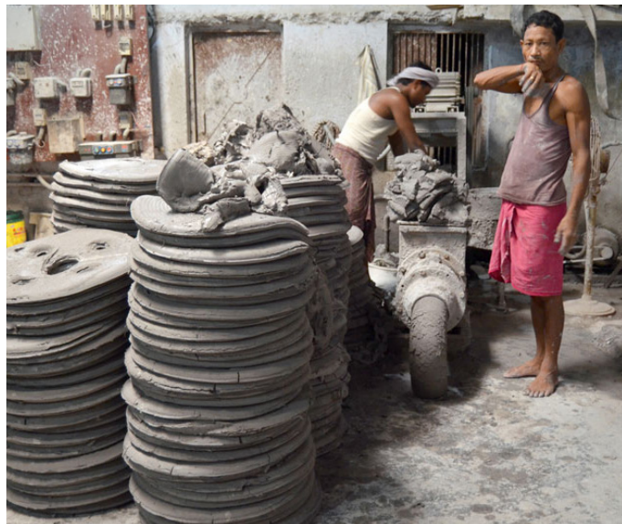
Clay cakes (discs) made by the filter press alongside a pug-mill.
