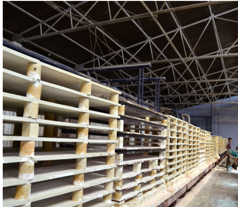
The shelves of the furnace.
