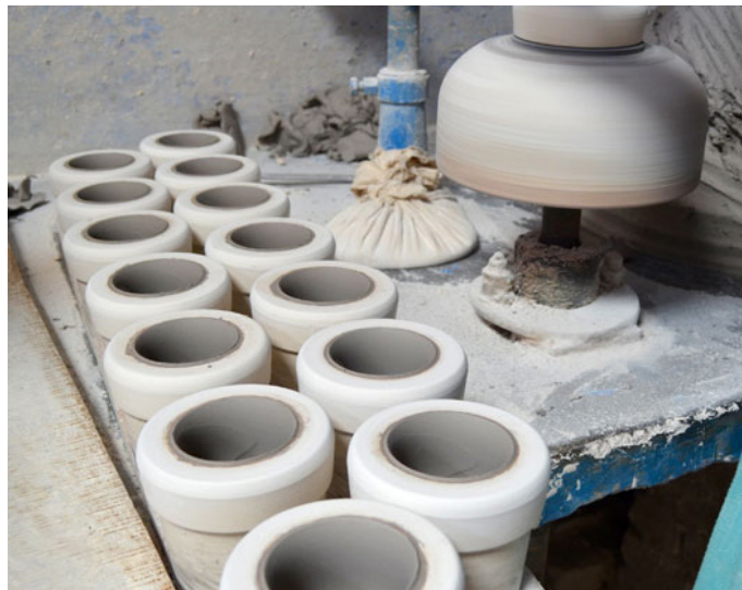
Clay being 'thrown' in along the walls of the mould using a hand tool on a rotating wheel-head.
