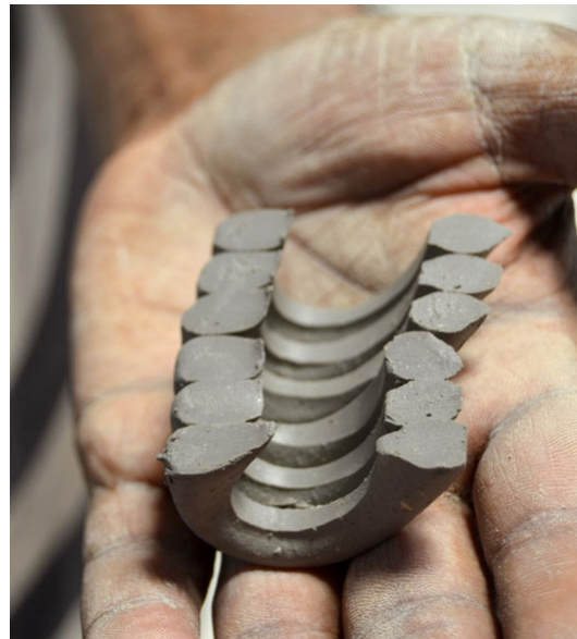
Clay handles ready to be joined on cups.
