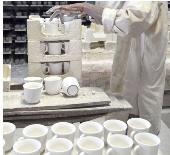
A karigar loading the car trays with cups.
