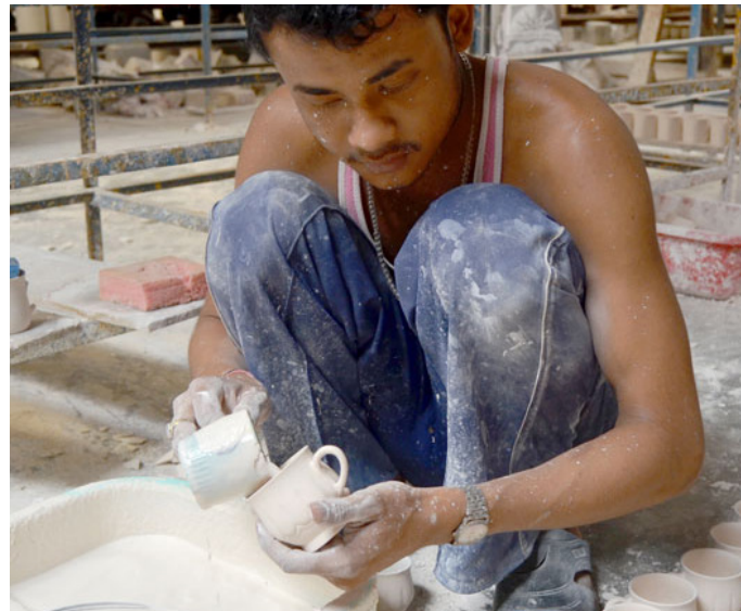
Clear glaze being poured inside as well.
