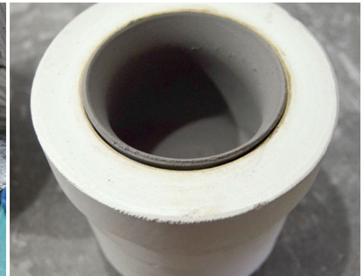
Clay, dry enough to be removed from the mould.
