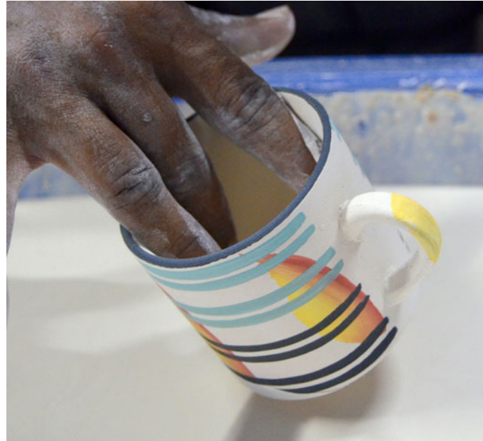
Hand-painted cups being dipped in clear glaze.
