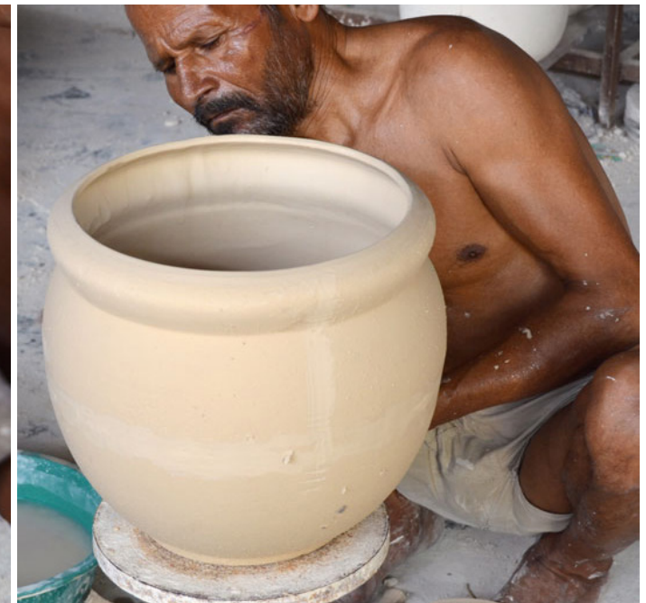
The karigar trimming the rim of the pot.
