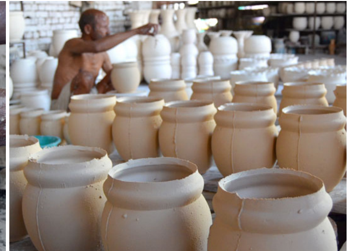
Just cast clay pots, ready to be finished.
