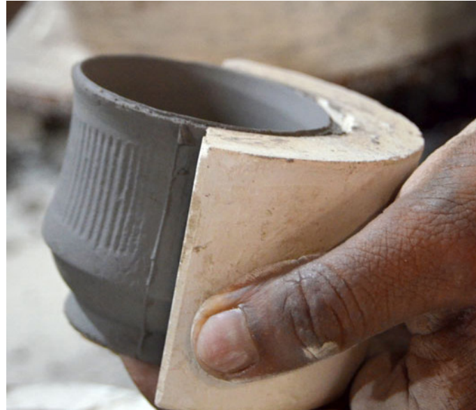
Clay cast being removed by opening up parts of the mould that were held together with rubber bands.
