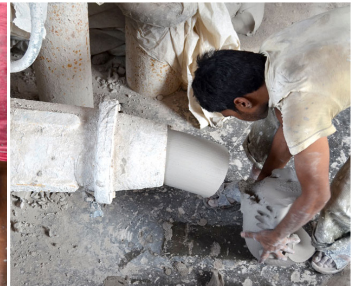
Clay being rolled out from a pug-mill.
