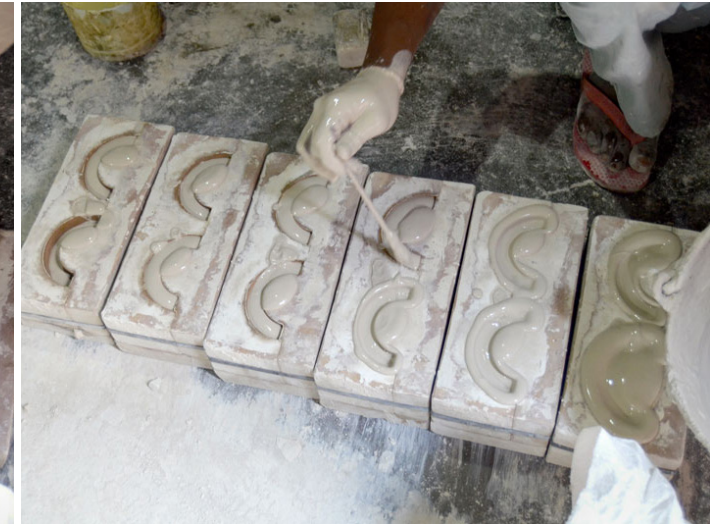
Air bubbles being removed from the POP liquid.
