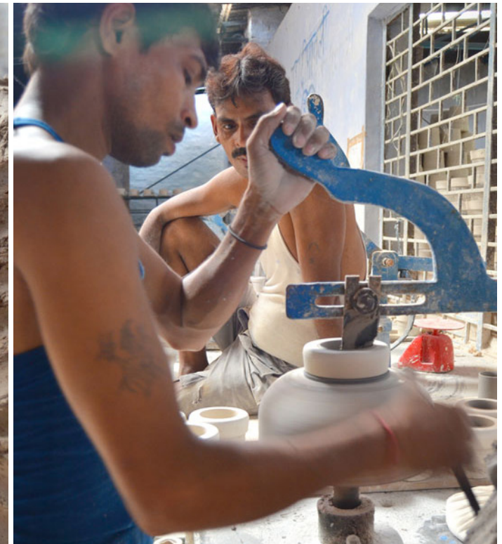
Clay being 'thrown' in along the walls of the mould using a hand tool on a rotating wheel-head.
