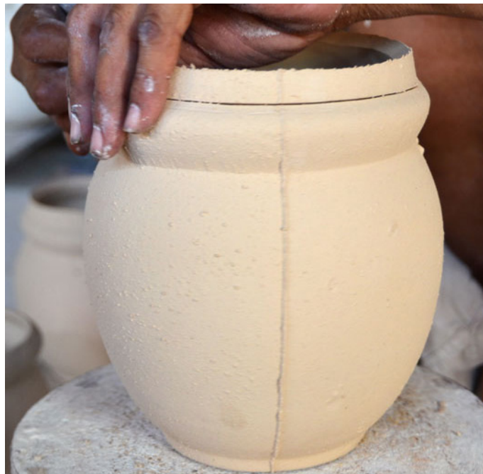
The karigar trimming the rim of the pot.
