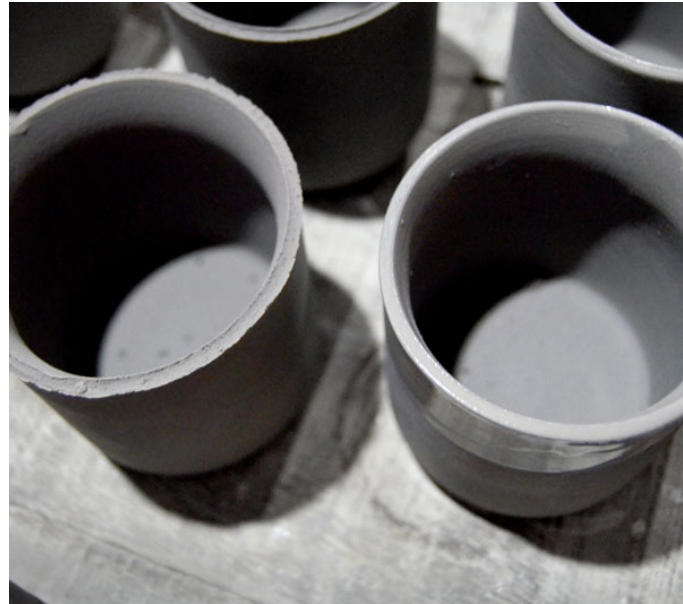
The difference between a 'cleaned up' and not 'cleaned up' cup. Rejects.
