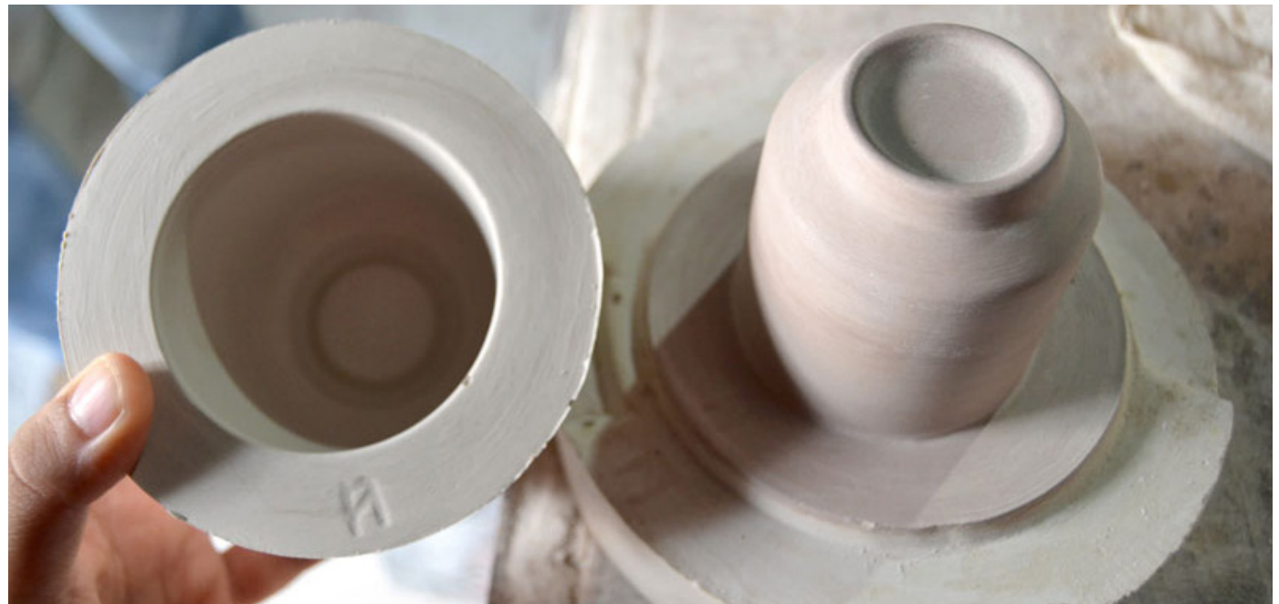
POP mould ready to be used to cast clay.
