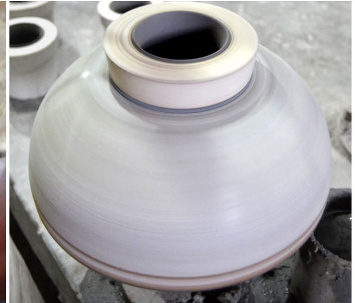
Clay being 'thrown' in along the walls of the mould using a hand tool on a rotating wheel-head.
