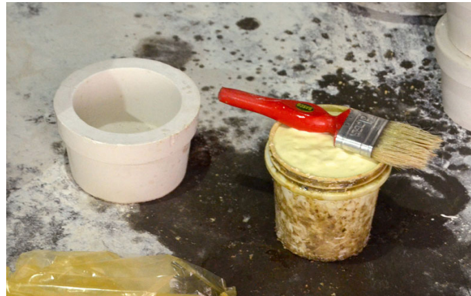
Soap and oil to be brushed on the mould.
