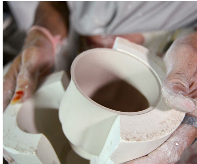
Clay cast being removed by opening up parts of the mould that were held together with rubber bands.
