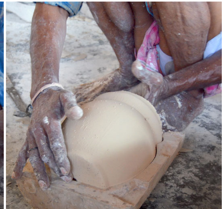
The karigar removing the clay pot from the mould.
