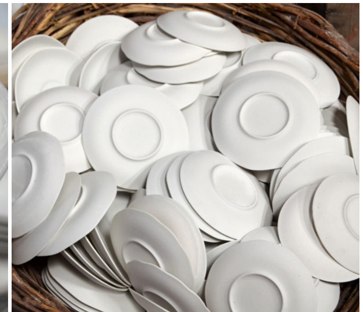
Saucers cast from a mould.
