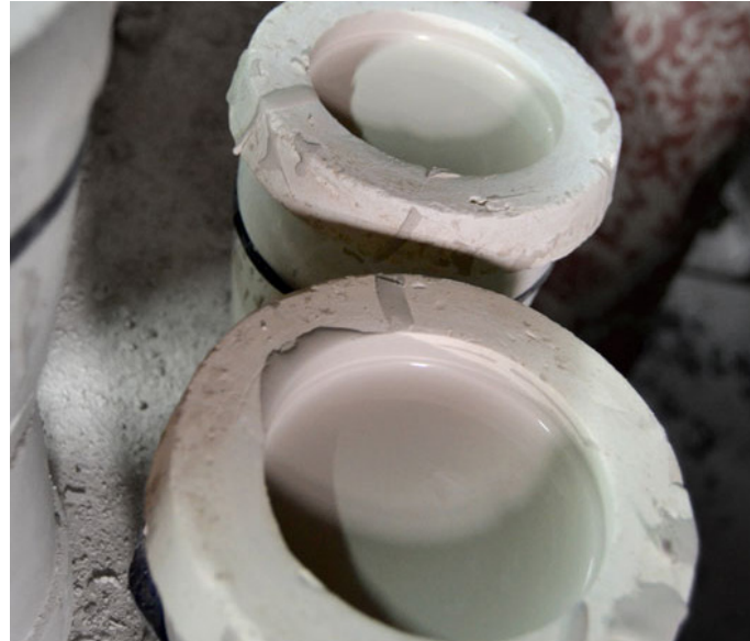
Slip (clay mixed in water) poured into the plaster moulds.
