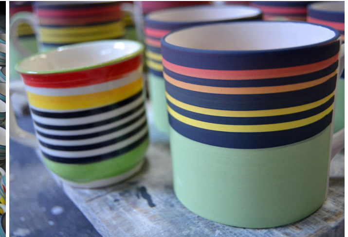
Difference between the two cups - one that has only stain painting done (right) and one that has been dipped in clear glaze and fired.
