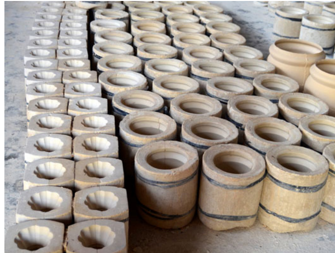
Series of moulds to cast vases and planters.
