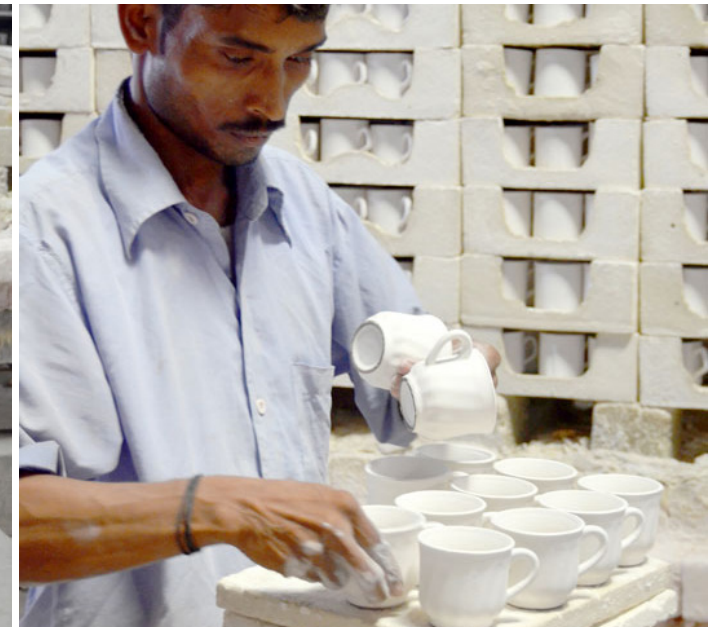
A karigar loading the car trays with cups.
