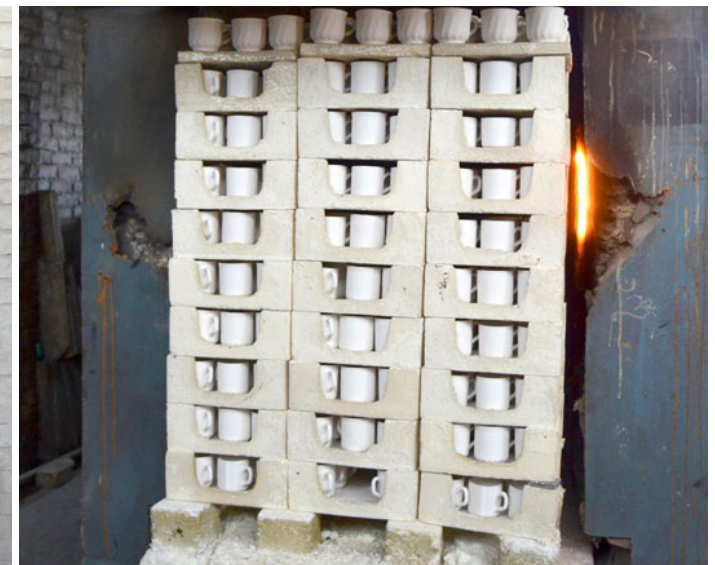
The fully loaded car entering the pre heating zone of the furnace.
