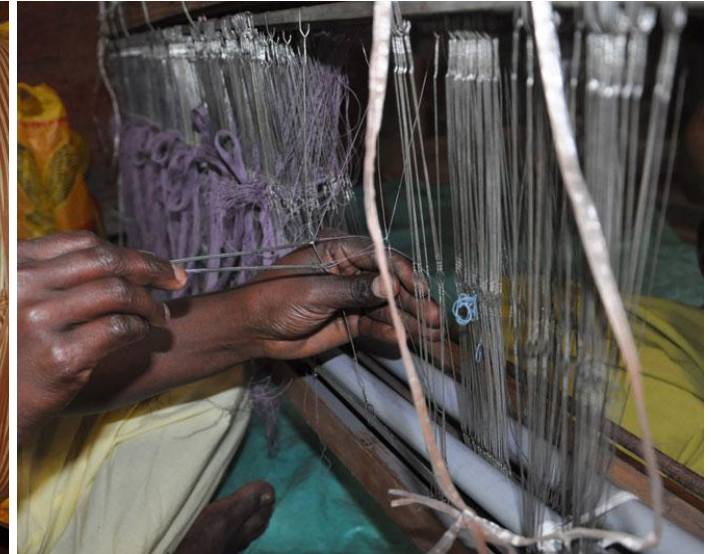
Each thread from the warp is taken and knotted to the weavers beam.
