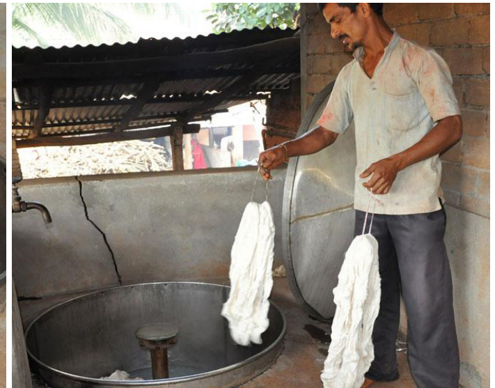
Cotton bundle is dipped in boiling solution.
