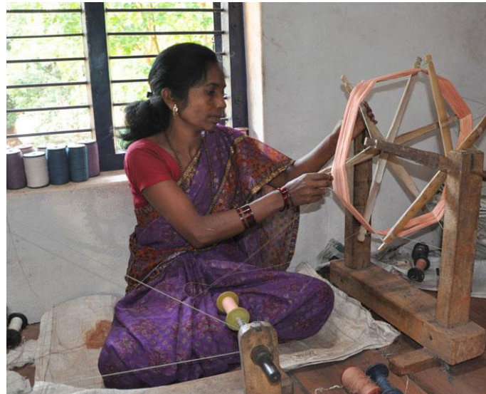
Cotton yarn is reeled onto spindle.
