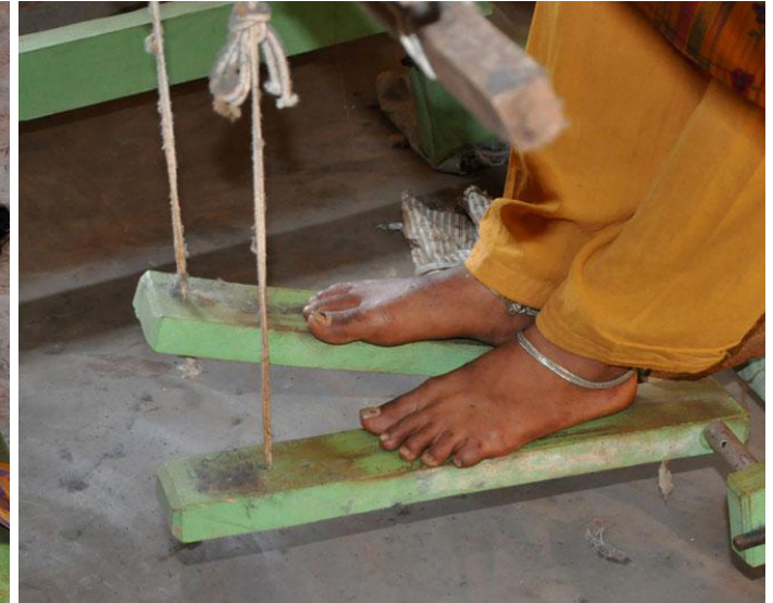
Continuous pedal movement required to operate loom.
