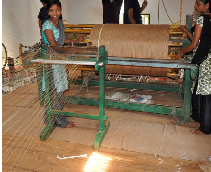
The threads from spool are reeled on warp beam.
