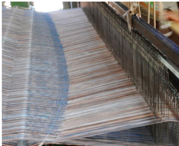
Warp threads are connected to the weavers beam to start weaving.
