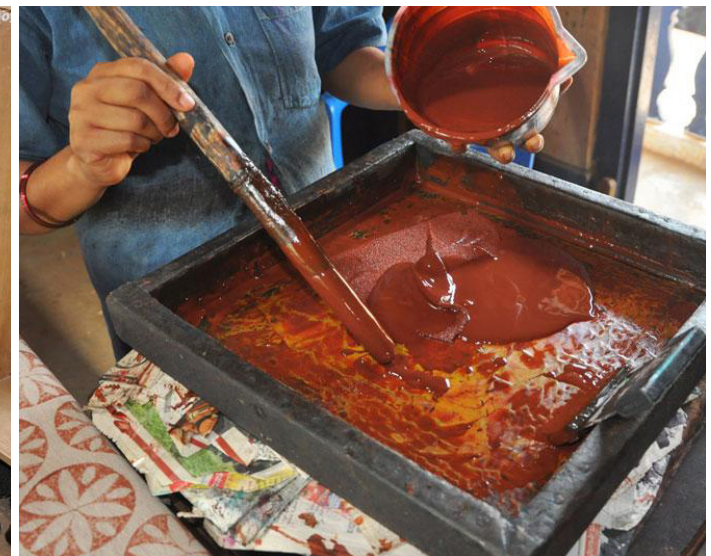
Chemical fabric colors used while block printing.
