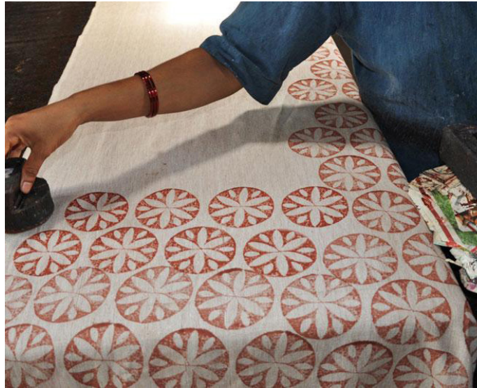
Wooden blocks are used to print the design on fabric.
