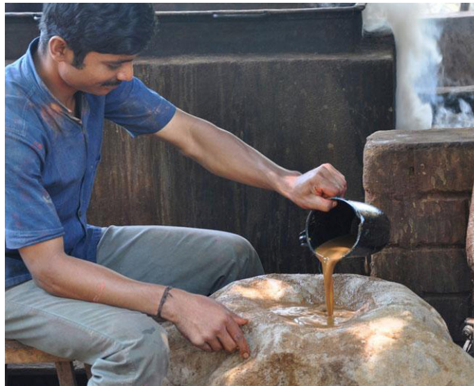
Powdered pomegranate is mixed in water and filtered to extract color.
