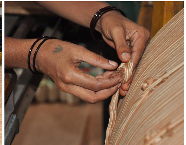
The warp is prepared and the ends are knotted.
