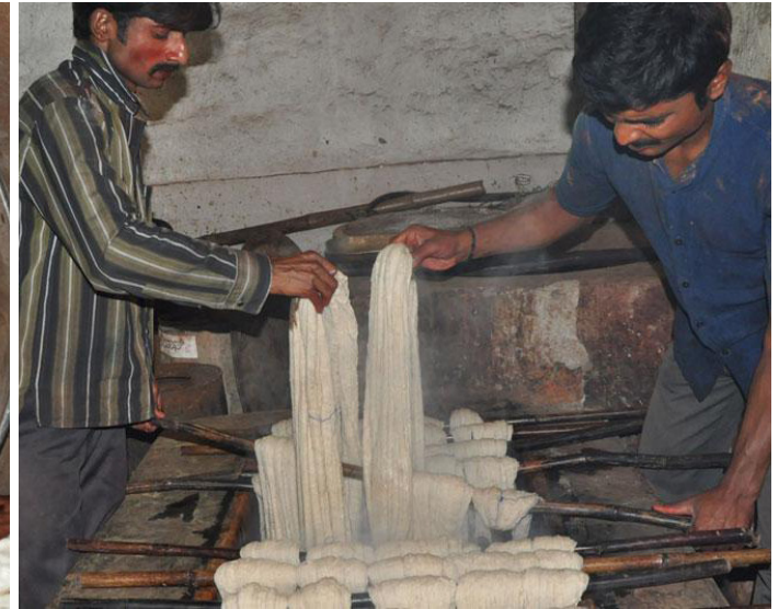
After chemical treatment, cotton is washed in hot water.
