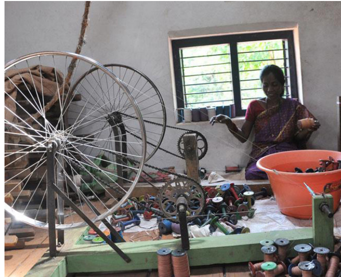
Spinning wheel used to wind yarn.
