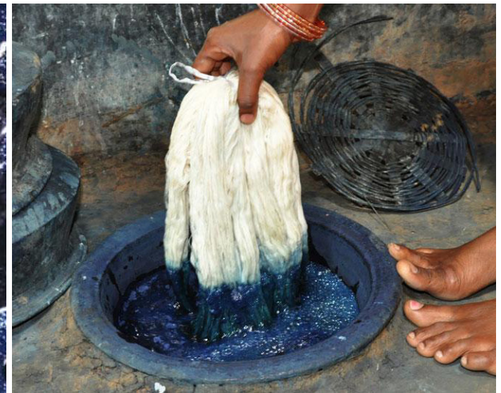
Yarn is carefully dipped to dye partially.
