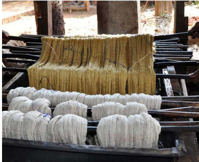
The yarn is dipped in boiling color solution.
