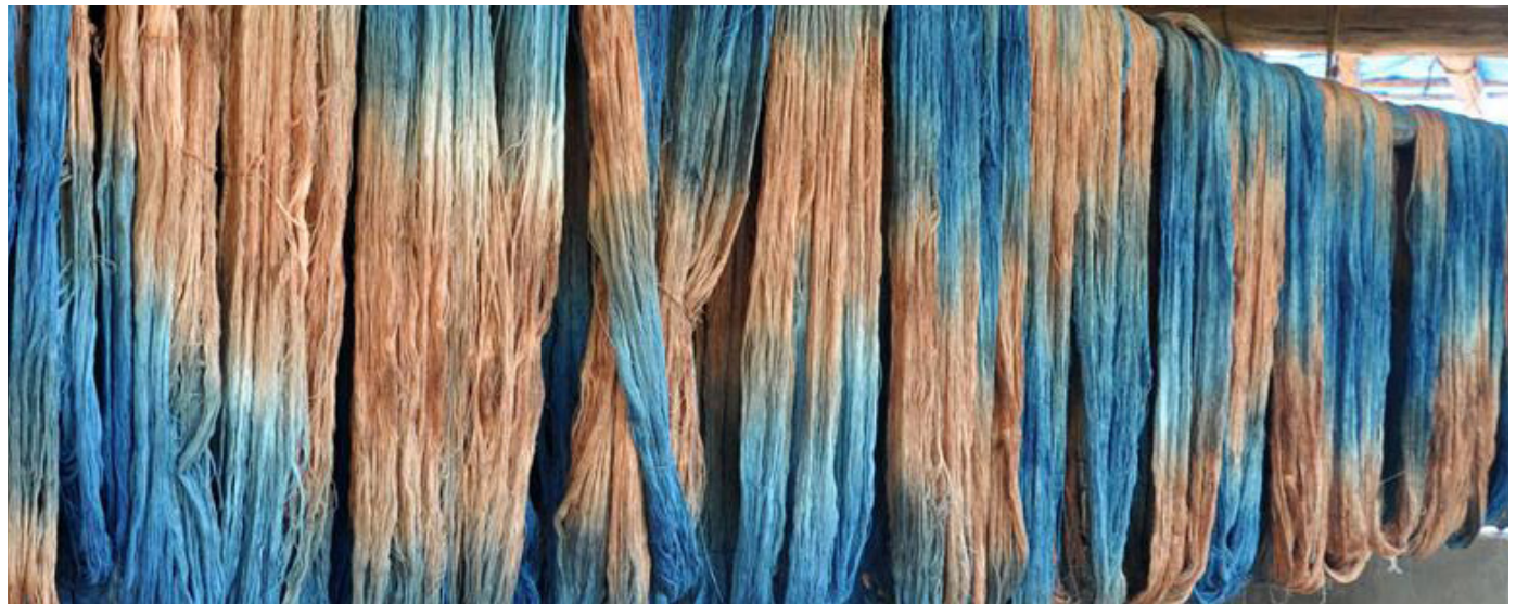
The dyed yarn is washed and dried.
