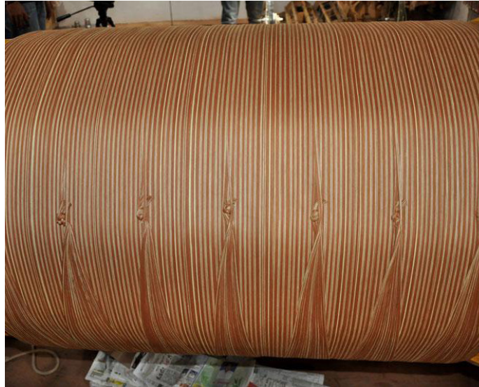
The warp beam is ready to load into loom.
