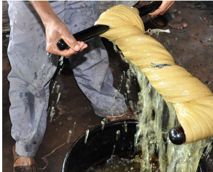
Excess water is removed by squeezing.
