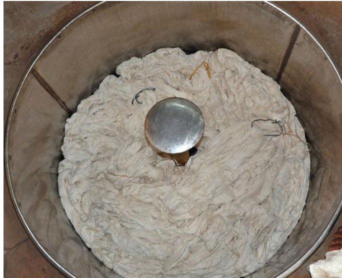
Cotton is boiled continuously for two hours.
