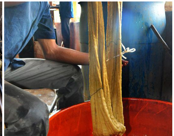
Colored yarn is washed in normal water to remove extra color.
