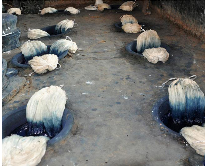
Yarn is dipped and allowed for several hours for coloring.
