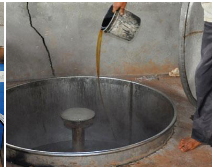
Soap oil is poured into boiler for cotton cleaning process.
