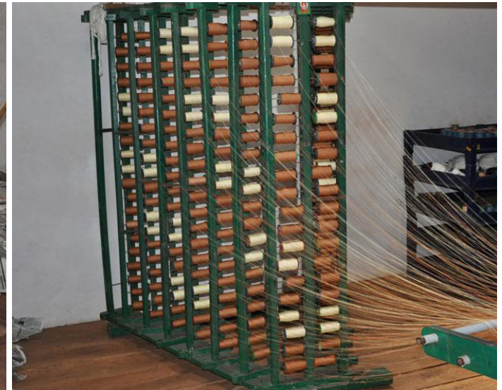
The spools are placed on warp machine to make warp.
