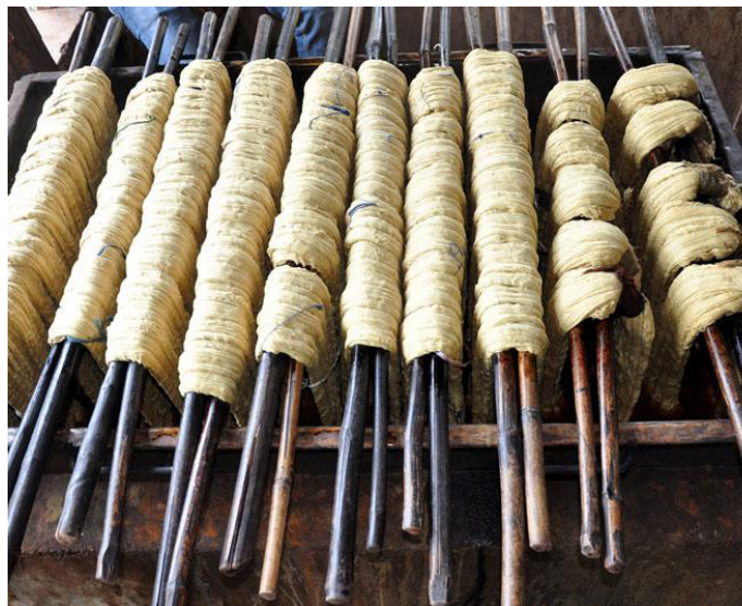
The yarn is kept in boiling solution for 30 to 40 min.
