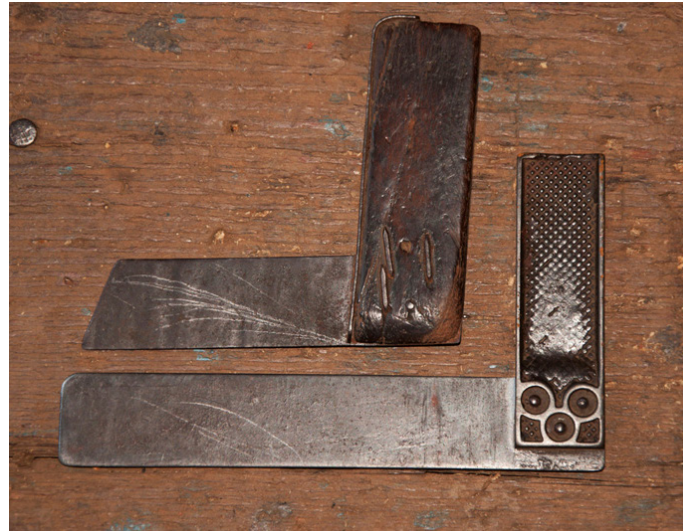
Measuring is done using right angle shaped tool.
