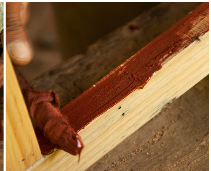
Varnish is mixed with color and coated on the products.
