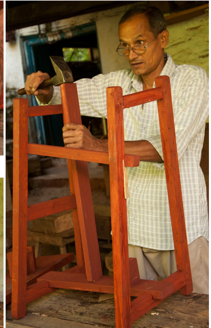
Stand of the charkha is being attached.
