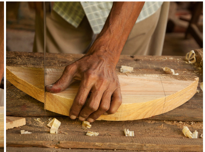
Wood is cut using a hacksaw blade.
