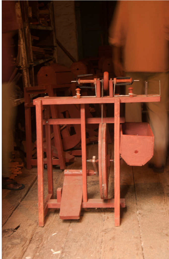
The finished product of charkha which helps in spinning wool threads.
