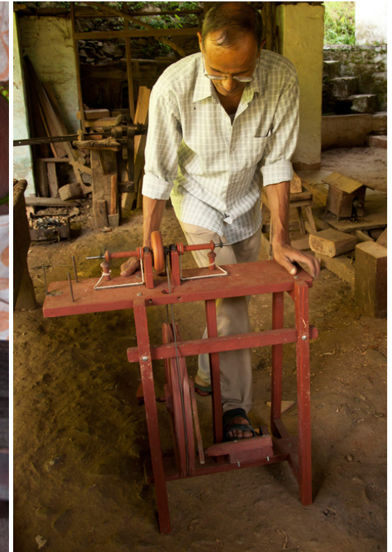
Charkha functions similar to spinning wheel by pedaling.
