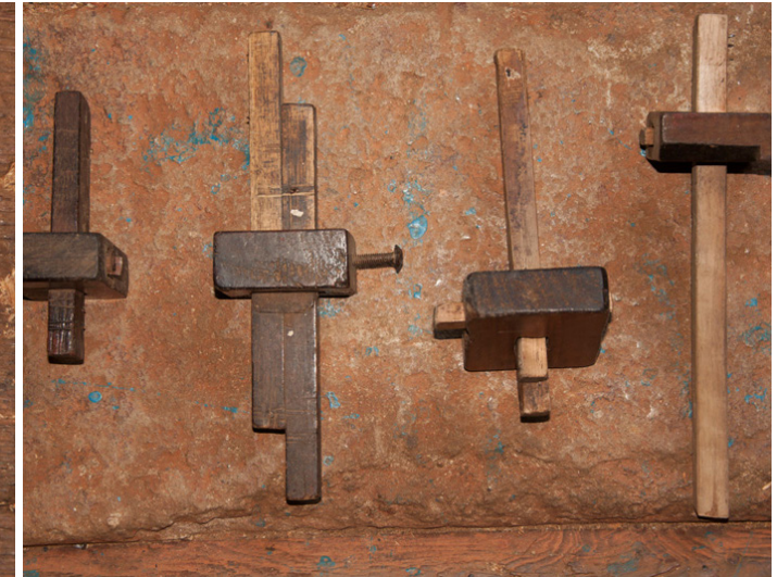
Edges of wood are marked using gauge.
