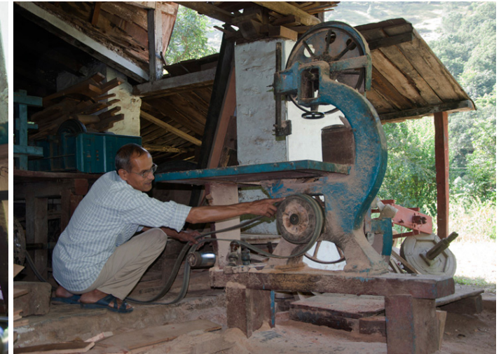
Belt from pulley is looped to wheel of Wood cutting machine.
