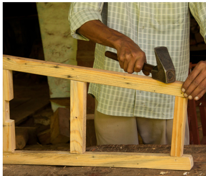
Hammering is done to fix the joined parts tightly.
