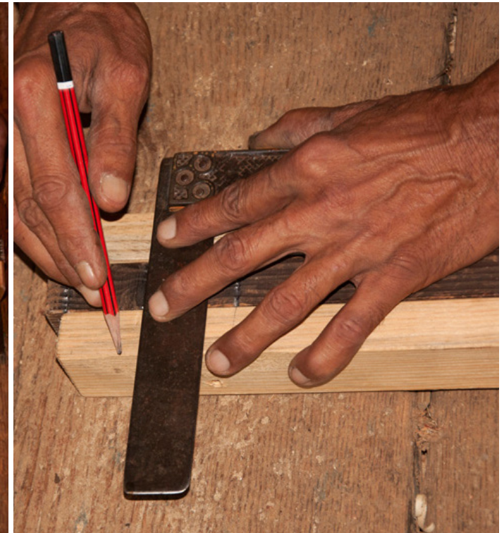
Wood slab is measured using right angle shaped scale. Marking is done to take exact measurements.
