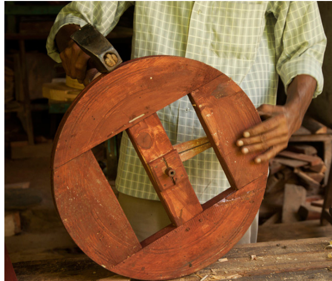
Artisan making wheel of charkha spinning machine.
