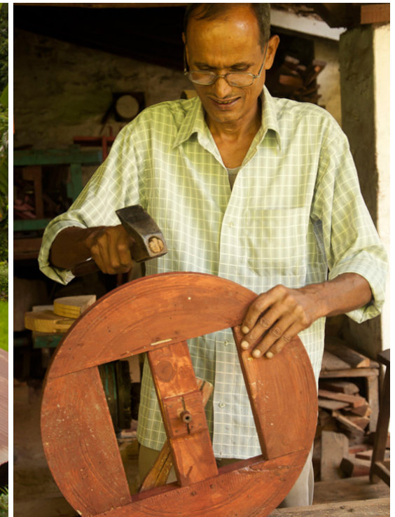
Different parts of the wheel are attached by hammering/fixing.
