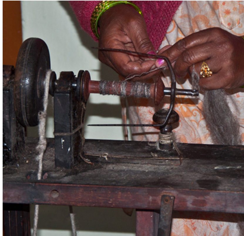
Closer view of process of spinning strands of wool into thread.
