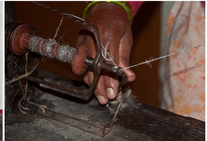
Charkha spinning process done by pedaling. Closer view of wool spinning.
