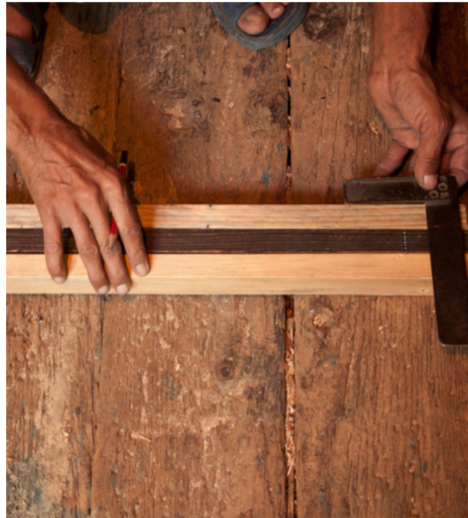
Wood slab is measured using right angle shaped scale. Marking is done to take exact measurements.
