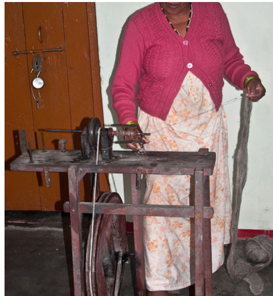
Charkha spinning process done by pedaling. Closer view of wool spinning.
