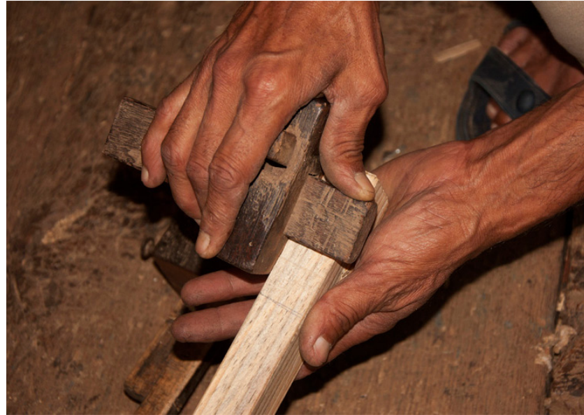
Edges of wood are made even by using a gauge.
