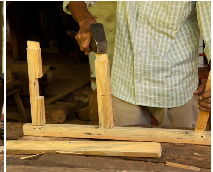
The wooden pieces are fixed to make stand- main structure.
