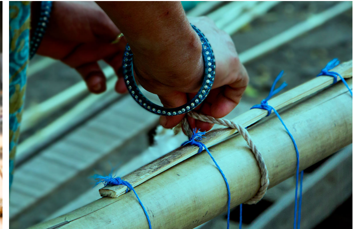
Bigger bamboo stick being tied with nylon threads as the base.
