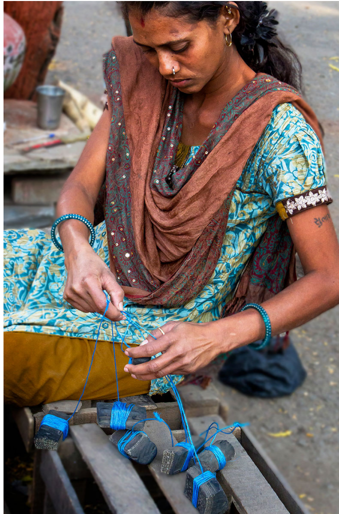
Nylon threads with a counter-weight tied at the end to as guides.
