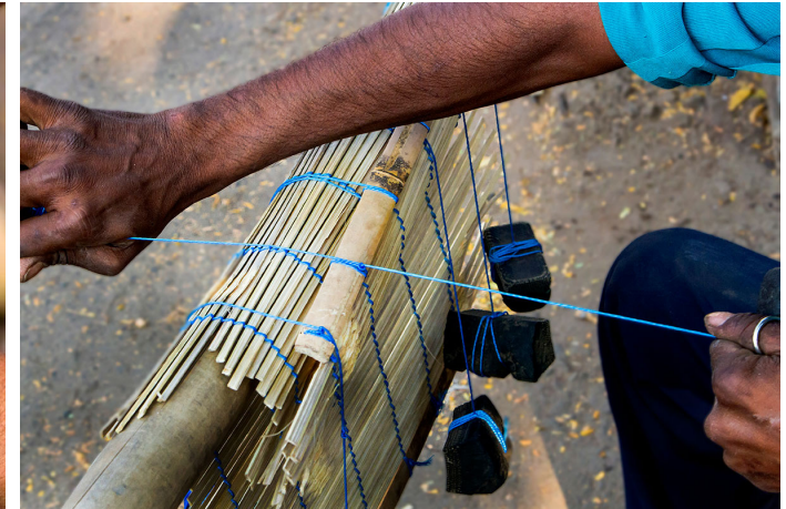
Bigger bamboo stick being tied at the mat as the border for the mat.
