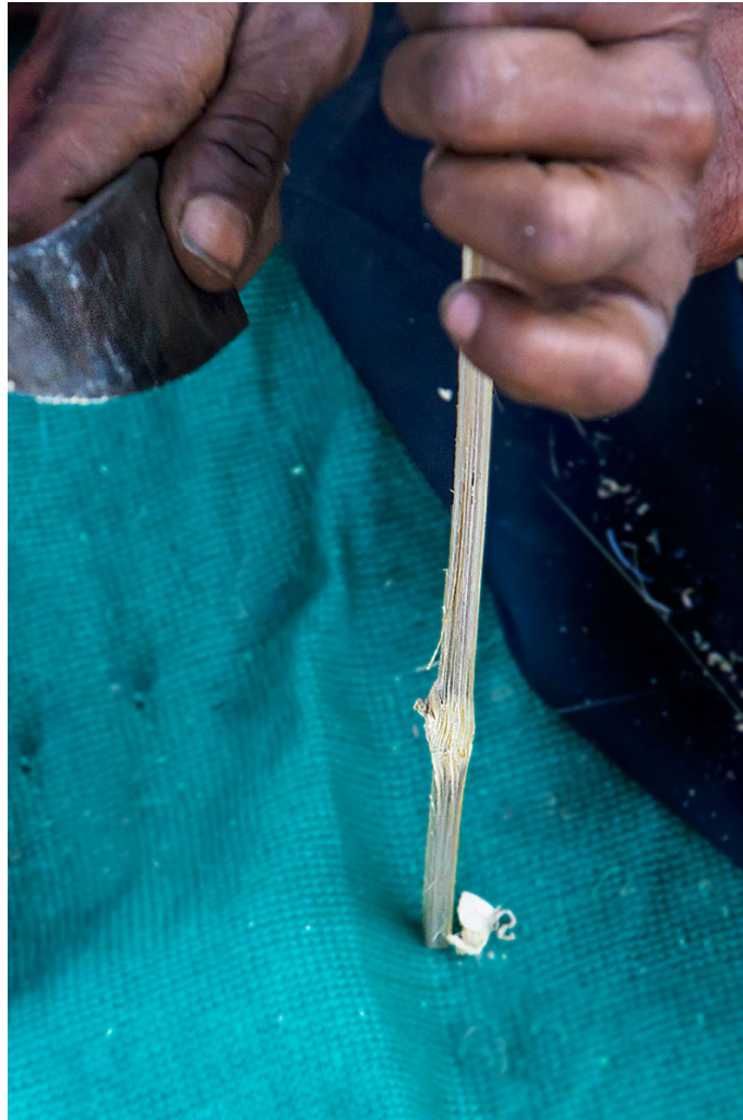
Hard fibers are removed from slices using a metal blade.
