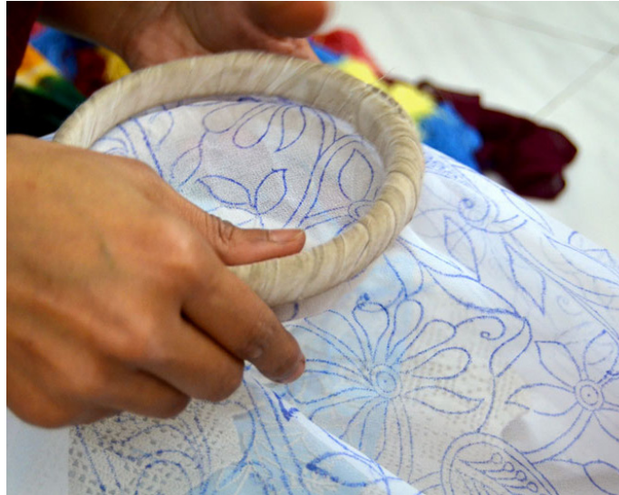
Printed fabric being fitted into the frame
