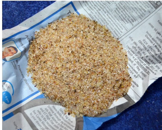
'Gond' - gum particles that hold the print on the fabric
