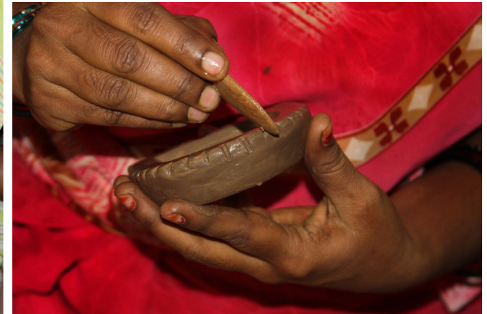
Design is made on the article using a sculpting tool made of bamboo.
