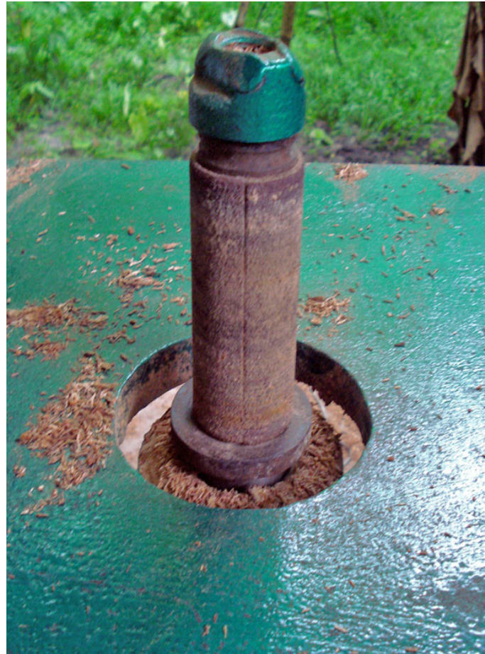
Another type of sanding machine used to smoothen the shell surface.
