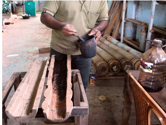
The mixture of Diesel, Chlorosulphate, Pesticide and Classic-20 applied to the inner surface using brush for chemical treatment.
