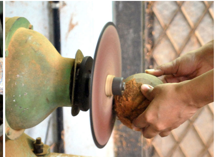
The husk on the coconut shell is removed by using sand-er disc.
