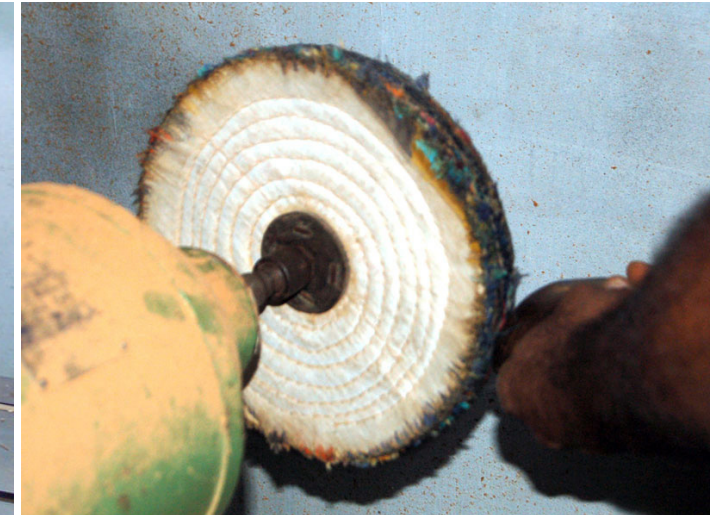
The Buffing machine is used to polish the shell.
