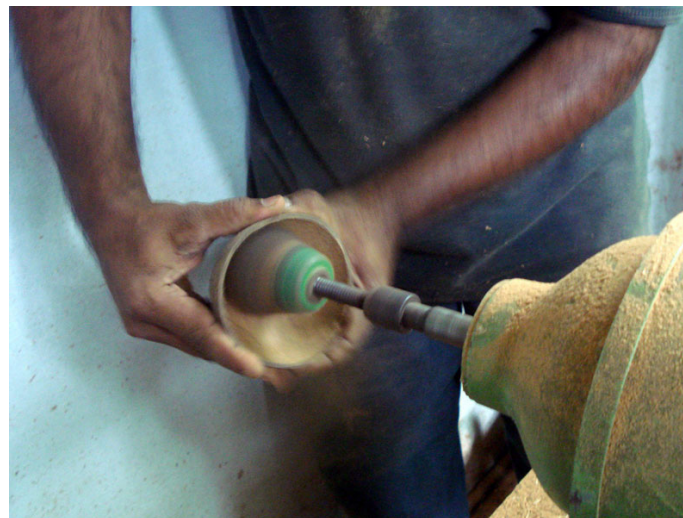
The inner surface of the shell is smoothened using another buffing attachment.
