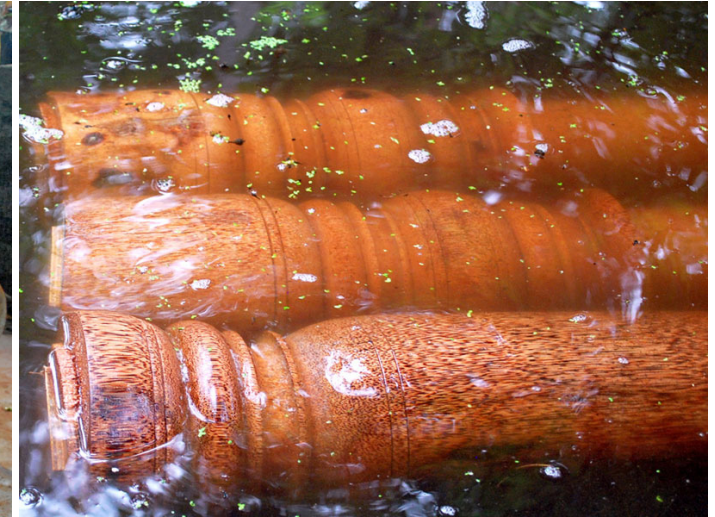
Coconut-wood logs soaked in tanks or ponds for 3 to 30 days – based on the nature of the product.
