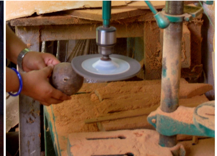
While smoothening, much care is taken to avoid damage to surface of the coconut shell.
