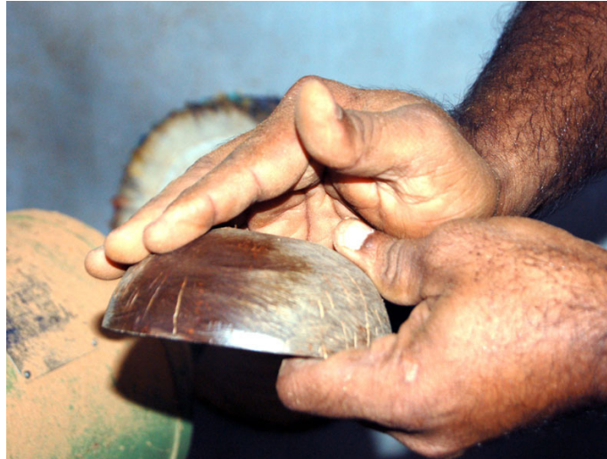
The shell is coated with wax and it is polished for shine.
