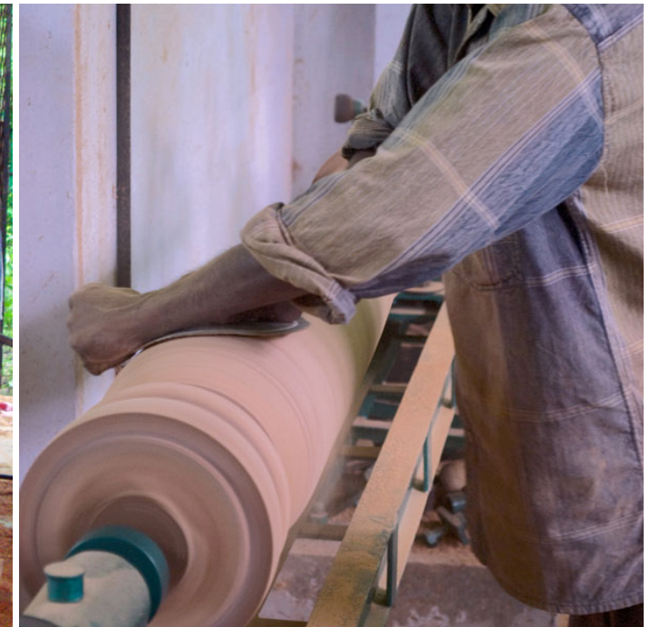
Turning machine rotates the log for smoothing of the outer surface.
