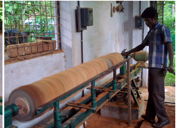
The log of coconut wood is laid on the lathe for carving.
