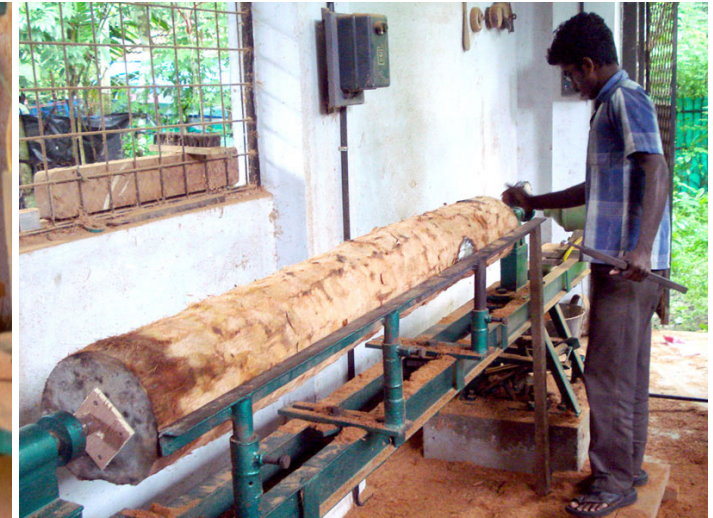
The wooden log is placed on the lathe machine for initial carving.
