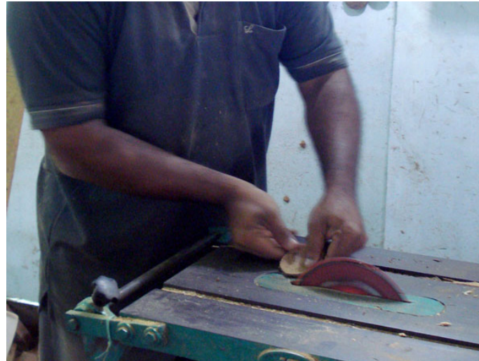
The shell is cut with a saw machine to give desired shape to it.
