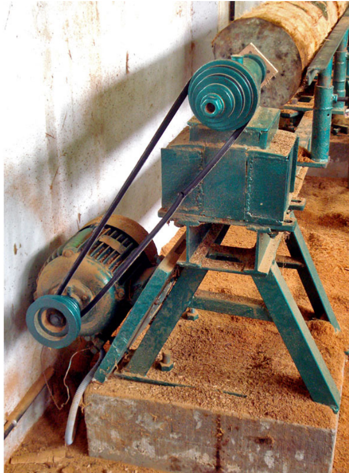
The motorised lathe.
