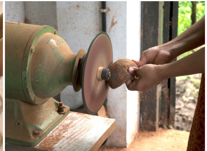
The husk on the coconut shell is removed using sander disc.
