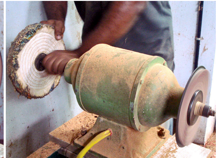
A multipurpose machine used for buffering and sanding. The artisan is fitting the buffering components to the machine.
