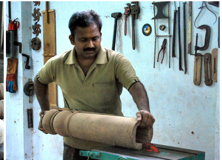
The log is marked at the center and cut in to two parts using a saw machine.
