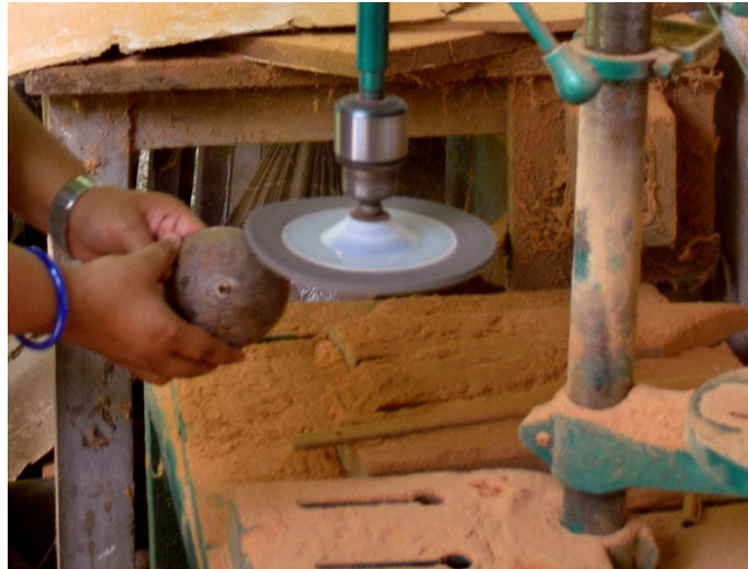
The outer surface of the coconut shell is being polished.
