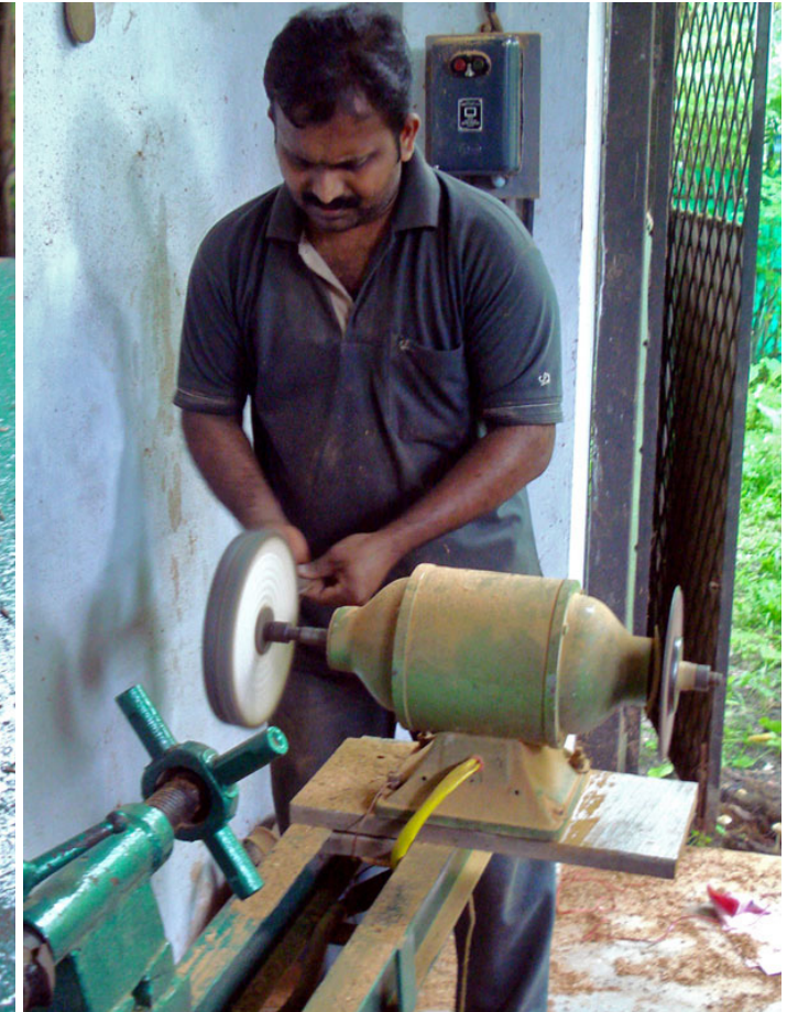
A buffing machine helps to smoothen the surface of the coconut shell.
