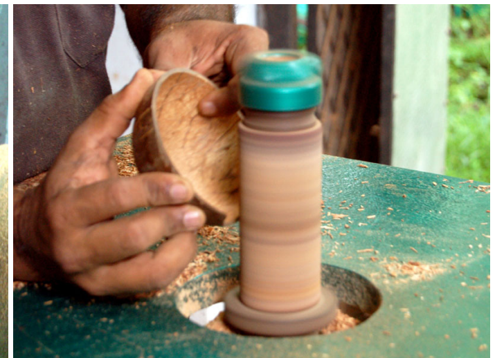
The circular sanding machine is used to create the curvatures.
