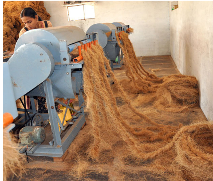
The roughly spinned coir is again fed into 2-ply-yarn spinning machine.
