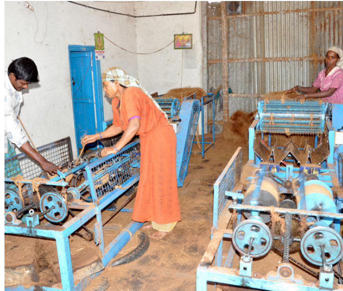
Attaching the discontinued coir rope.
