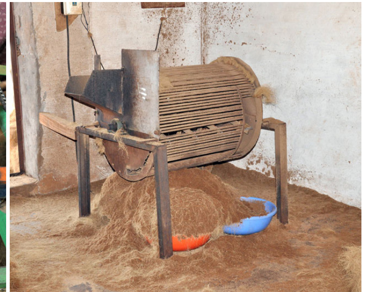
A machine to clear the impurities in coir.
