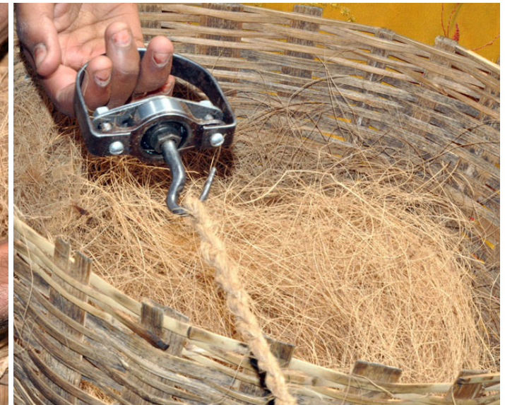
A hook used to hold the rope while twisting.
