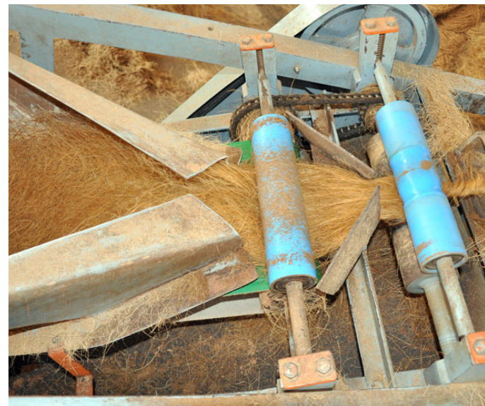
The finely processed coir is being twisted.
