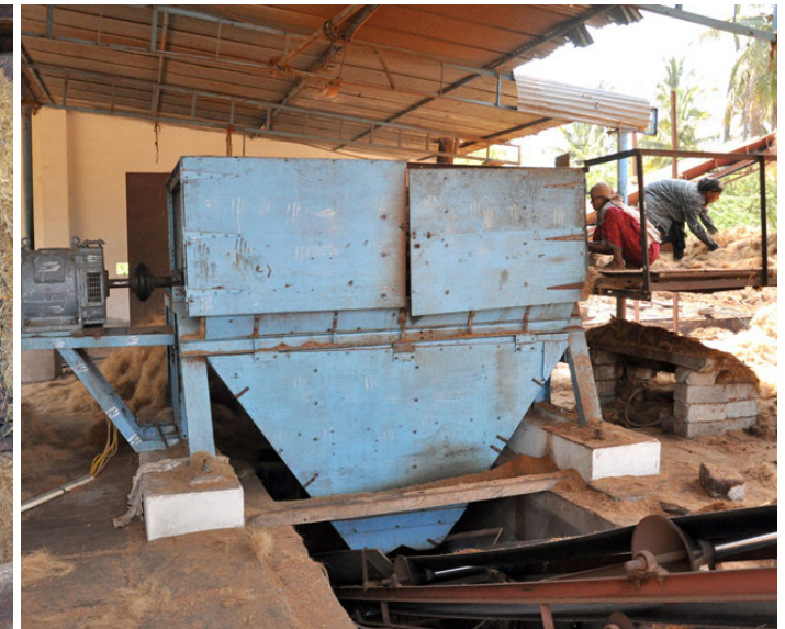
The husk is again cleaned using coir refining machine.
