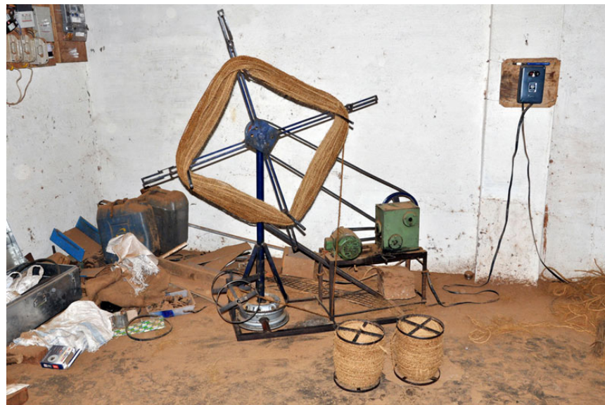
The bundle of coir is reeled using reeling machine.
