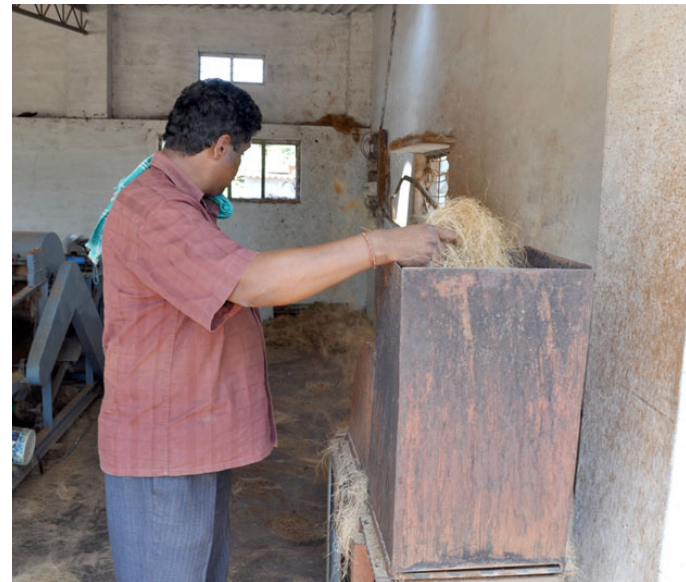
Coir is initially dried in drying machine.
