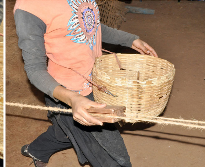
The twisting is done using triangular shaped wooden piece.
