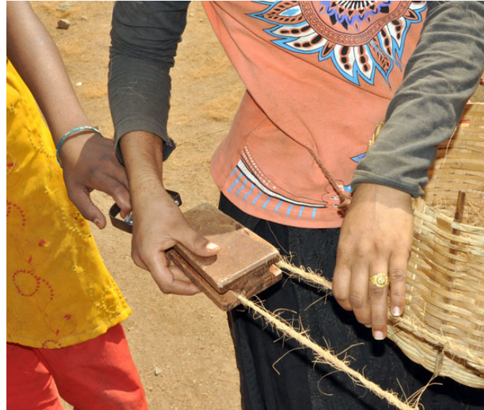
The two ply rope is twisted into single rope as to make it strength.
