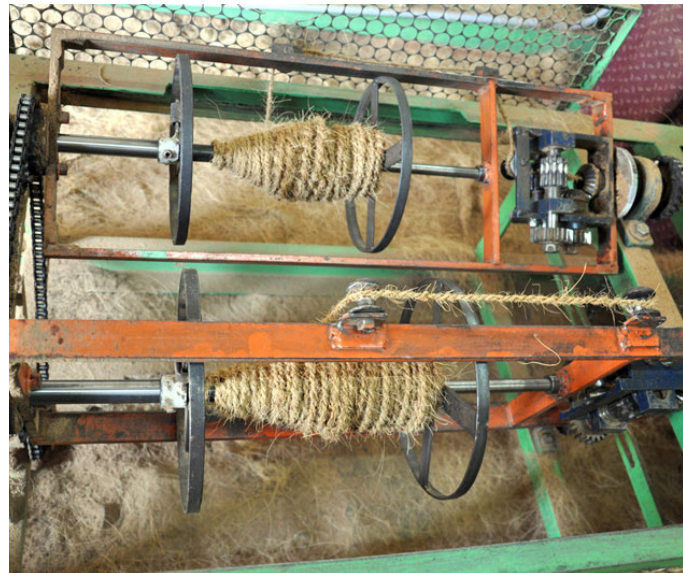
The two spools in machine reels the coir rope.
