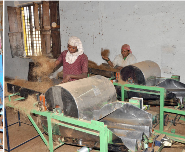
The coir is directly twisted into rope without processing.
