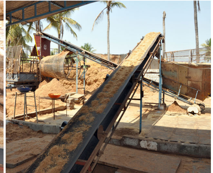
The husk powder is sent for filtering process.
