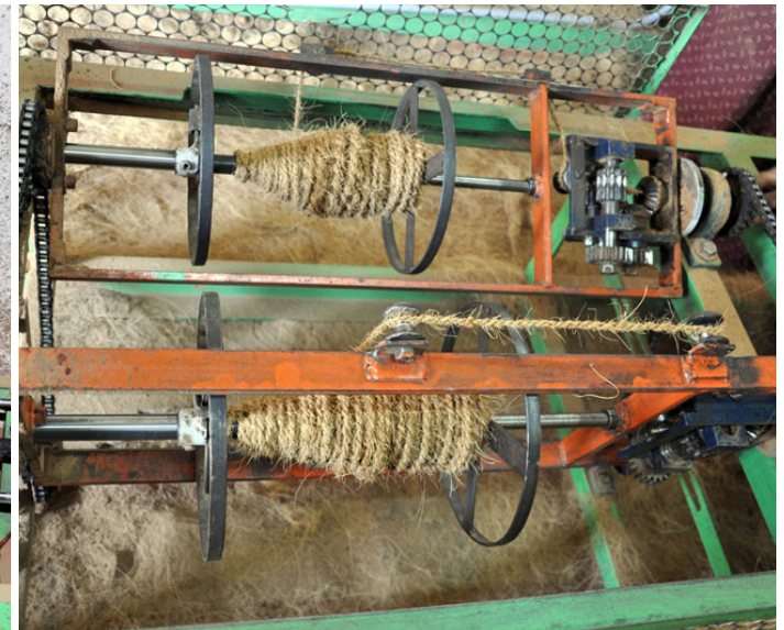
Yarn is being reeled automatically.
