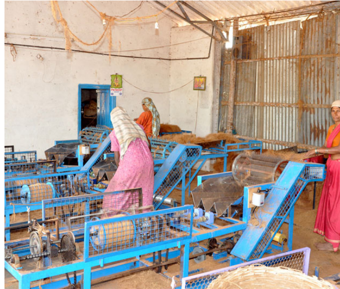
Rough coir is separately spinned in 2-ply-yarn spinning machine.
