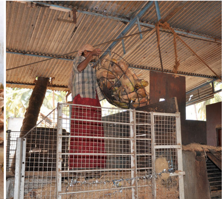
The husk is sent inside the defibering machine (beater).
