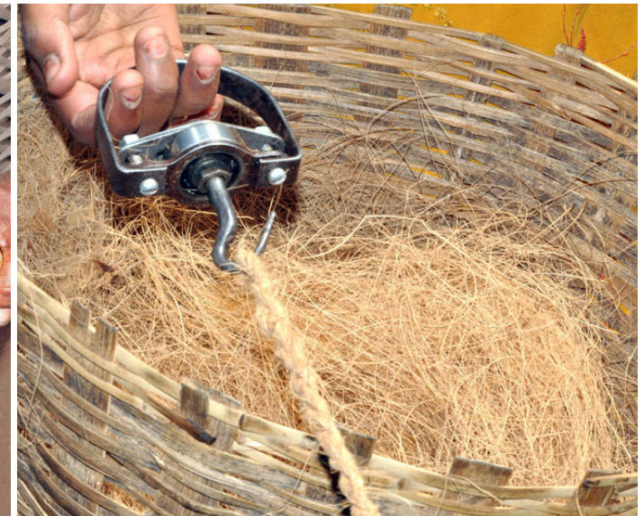
A mechanized hook that holds and rotates the coir twine.
