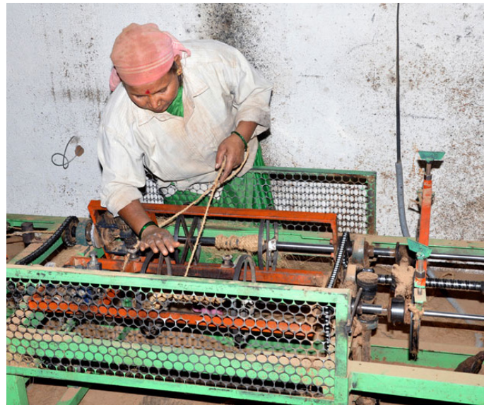
2 ply yarns are twisted into single rope.
