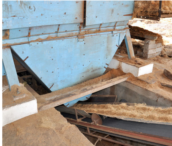
The waste husk powder is separated automatically inside the machine.
