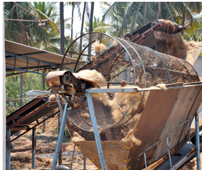
The circular grill that separates coir and pith.
