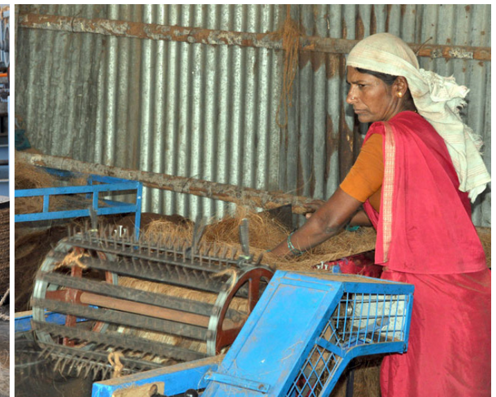
The lesser quality coir is twisted in different yarn spinning machine.
