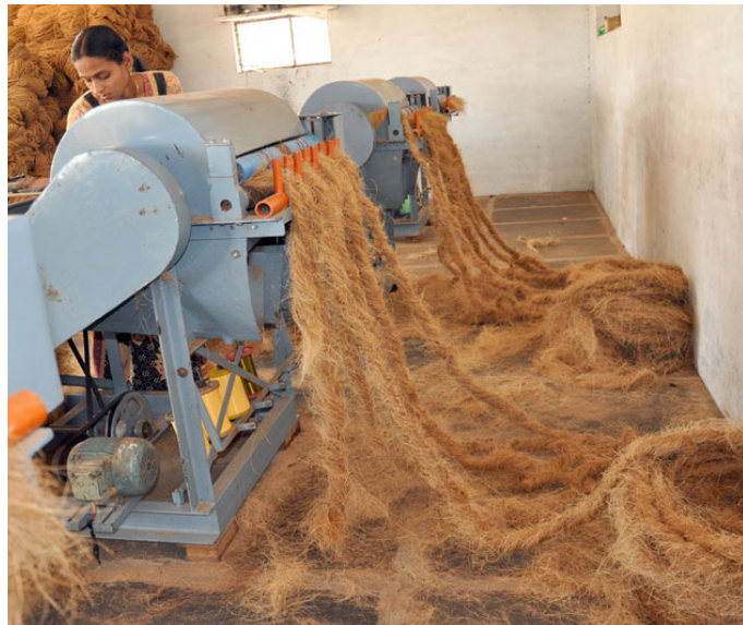
The rope is again finely twisted using another rope twisting machine.
