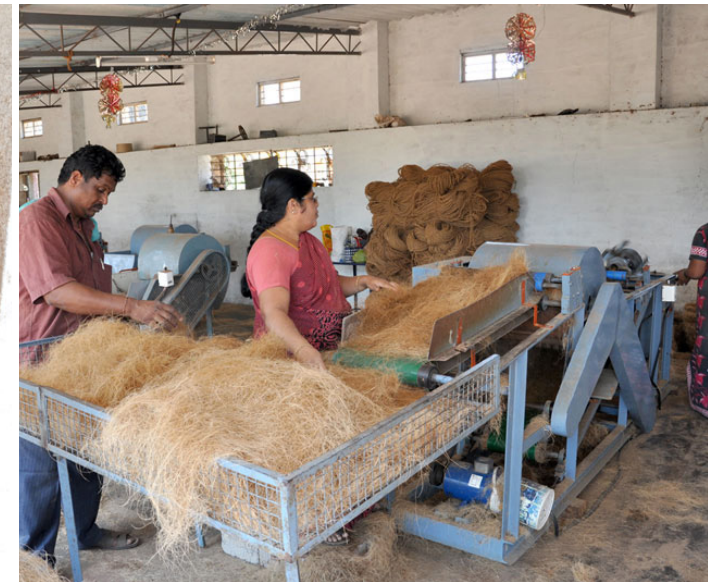
The dried coir is initially twisted roughly in an automated yarn spinning machine.
