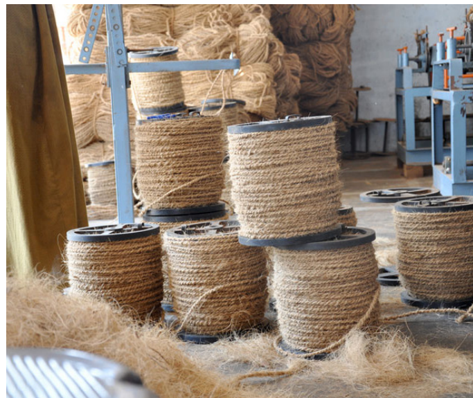
The twisted rope is finally reeled to big spools.
