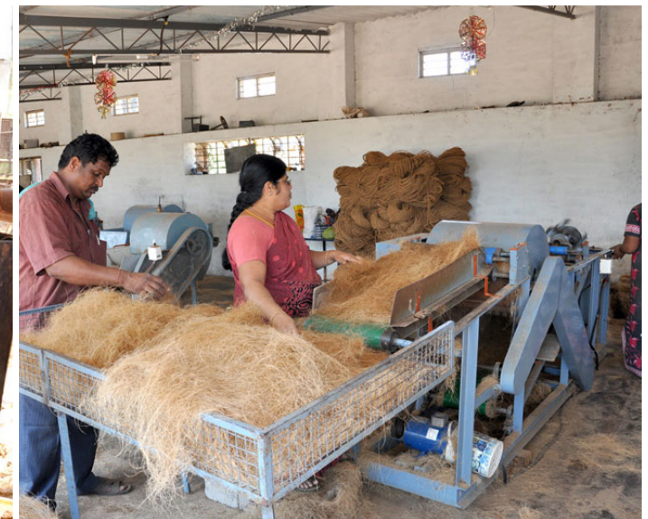
The yarn spinning machine that spins coir roughly.
