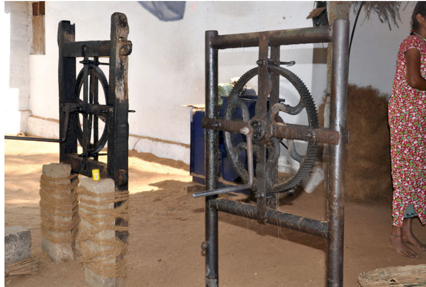
Manual process of twisting is done using coir spinning wheel.
