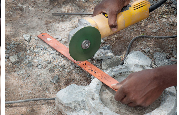
Used saw-blade is cut to make customized tools for carving.
