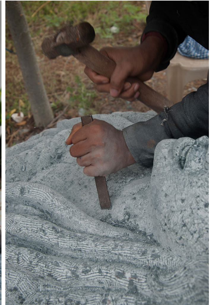
The four tooth chisel tool is used to carve.
