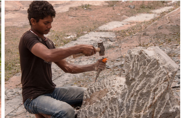
Rough carving is made out of bull point chisel.
