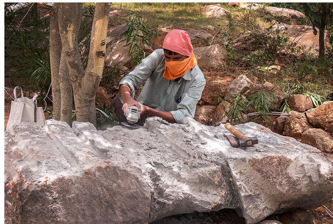
Smoothing the rock with the help of angle grinding machine.
