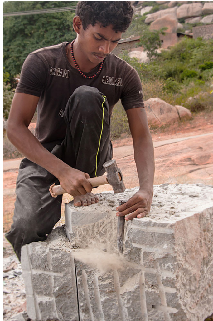
Artisan carving out the excess portion of the stone.
