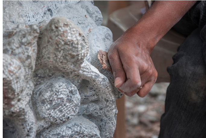
Emery paper is used in smoothening the surface of the stone.
