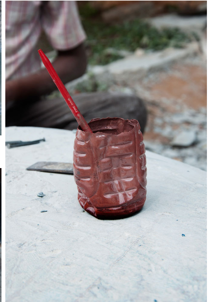
Red oxide used to mark on stones.
