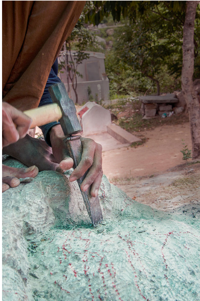
Flat chisel used in removed the excess of the stone.
