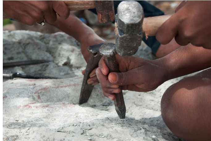
Bull point chisel and flat slant cutting chisel is used in removing the unwanted part of the stone.
