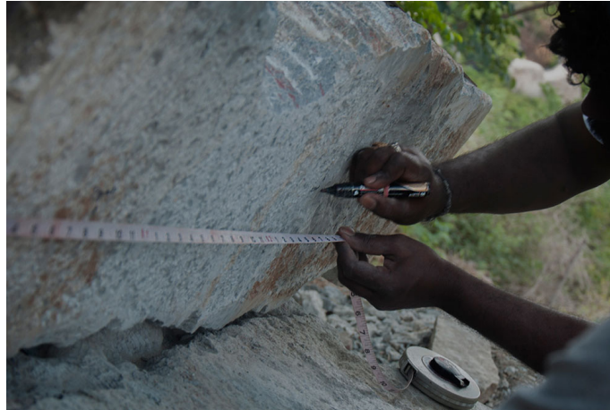
Marking with help of measuring tape and marker.
