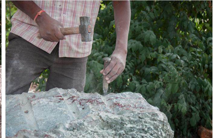
The stone is roughly carved with the help of bull point chisel and hammer.
