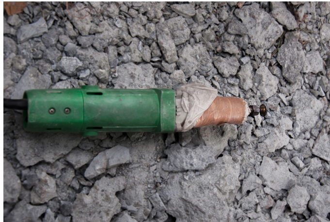
Drilling bit is used to get small markings on the stone.
