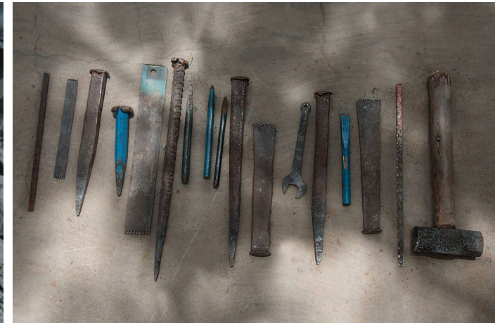
Set of chisels – pointed, flat and tooth chisels are used.
