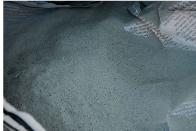
Stone powder, used as adhesive binder.
