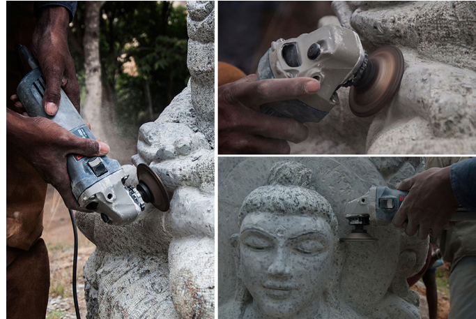
Power machineries like Angle grinder is used in buffing, cutting, grinding and polishing of the sculpture.
