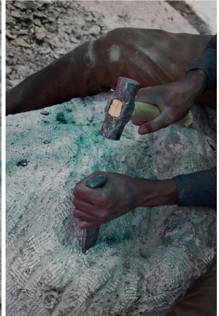
Artisan carving a narrow depth using flat chisel.
