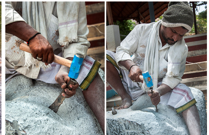
The flat tooth chisel is used to even the surface.
