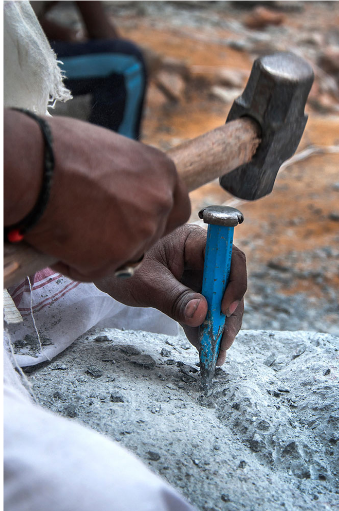
Bull point chisel is used to give the depth to the chin part.
