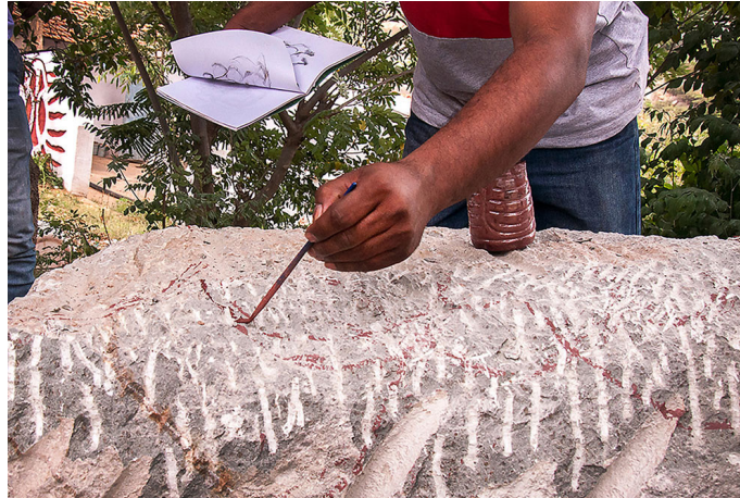
A block of stone is being marked by the red oxide paint.
