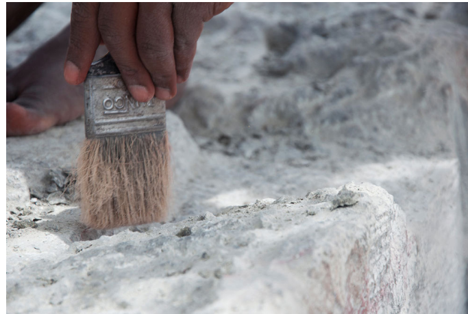
The dirt on the stone caused by carving is dusted with the help of two inch brush.
