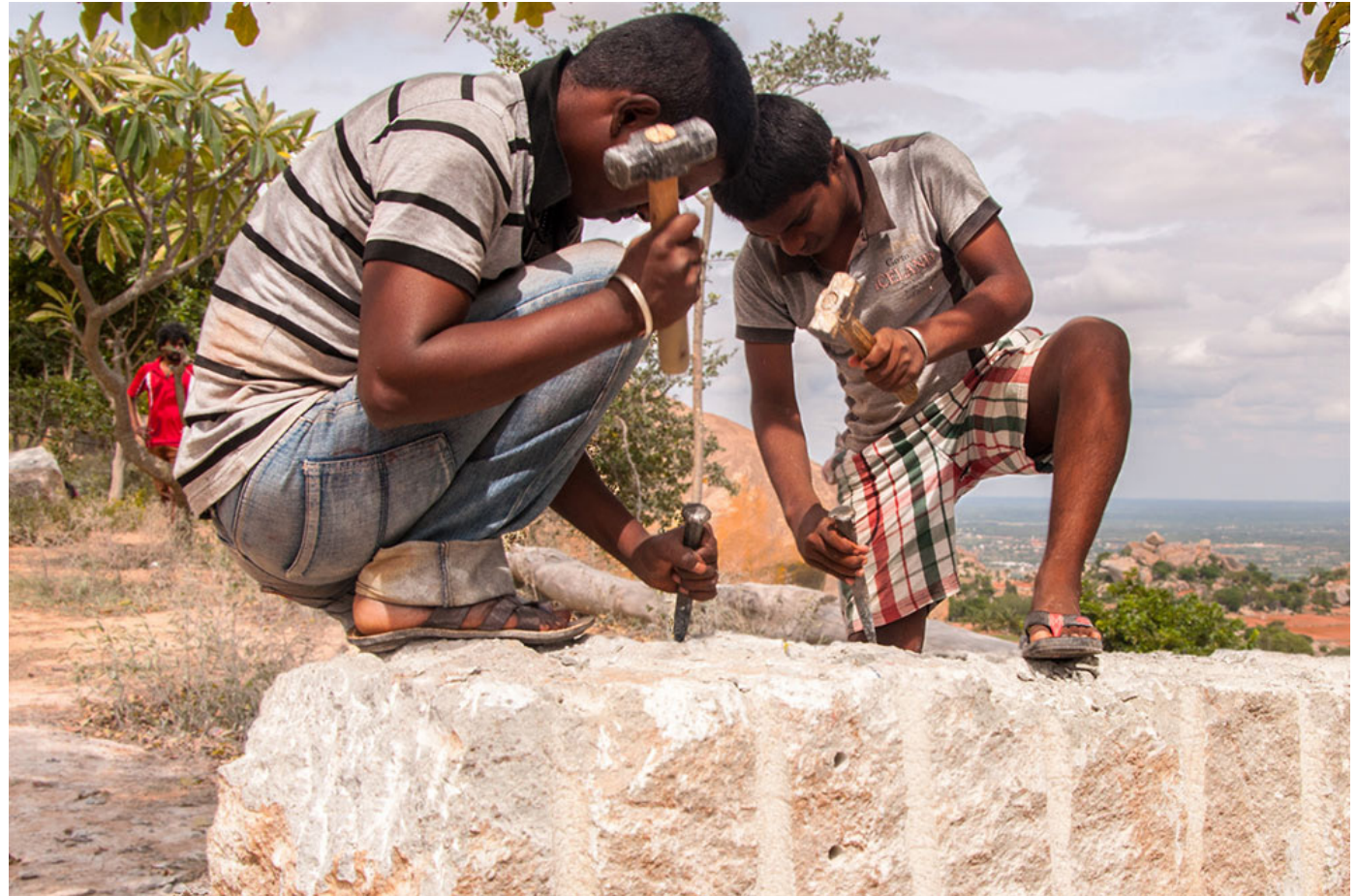
Artisans carving out the excess of stone with bull point chisel.
