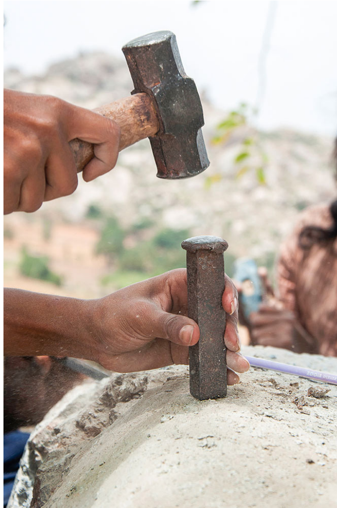
Bush head chisel used in flattening and leveling the surface of the stone.
