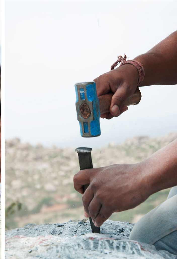
Artisan carves the outline of the design drawn with the small flat chisel.
