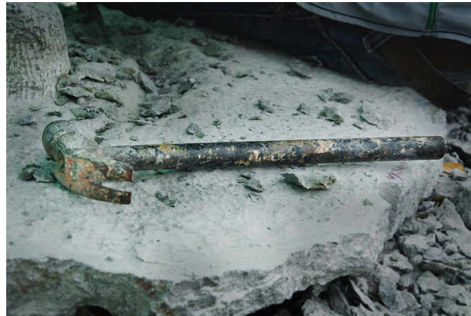
Claw hammer is used while carving stones.
