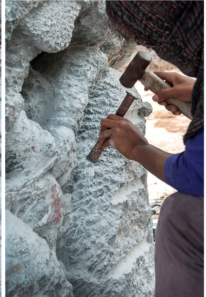
Artisan using flat chisel in leveling the surface of the rough carved stone.
