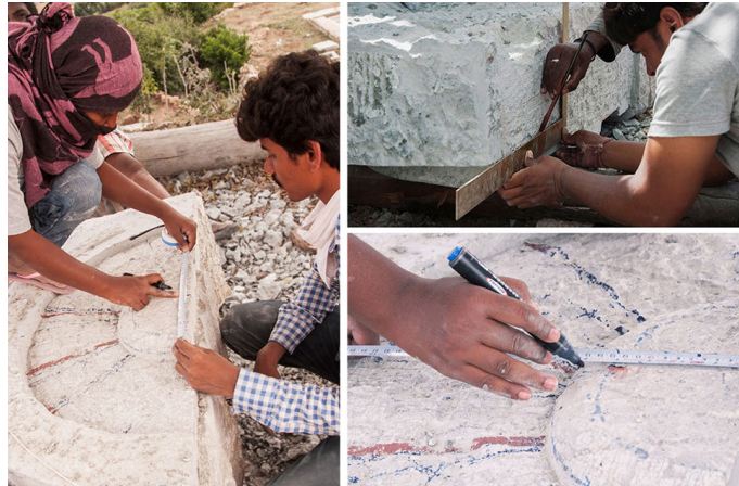
Artisans using various measuring tools like L shaped square tool and tape in marking accurate points of the design.
