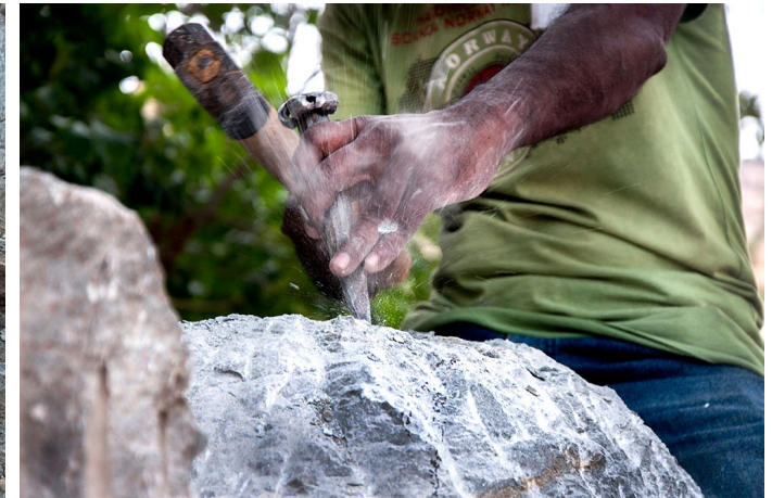
Carving the stone with the help of the chisel and hammer.
