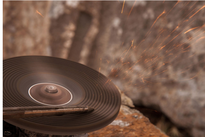
The tool is sharpened by placing it on silicon carbide blade.
