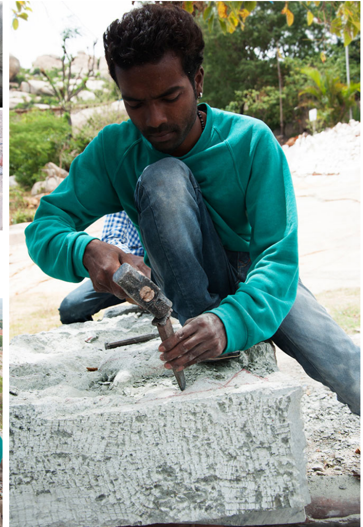
Artisan using Flat edge tool in carving the traditional door garland.
