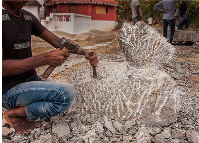
Artisan uses claw chisel in carving the stone when the sculpture is coming to the initial finishing.
