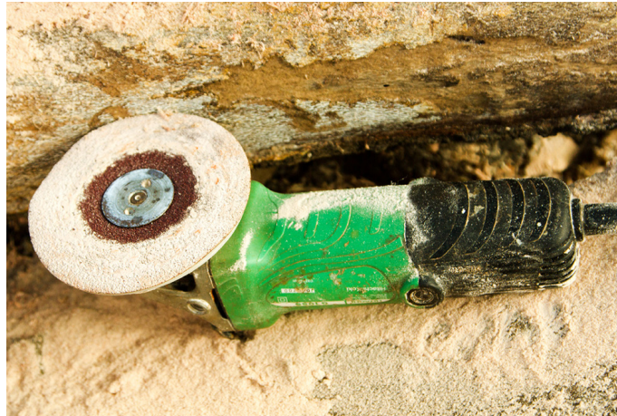
Grinding machine with sandpaper bid is used for giving the smooth finish for the sculpture.
