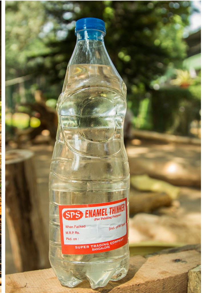
Enamel thinner is used for thinning the consistency of the wood finish.
