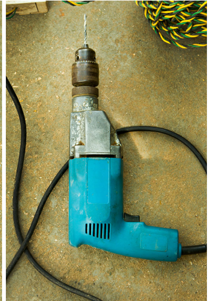
Drilling machine is used for drilling purpose to insert the nail.
