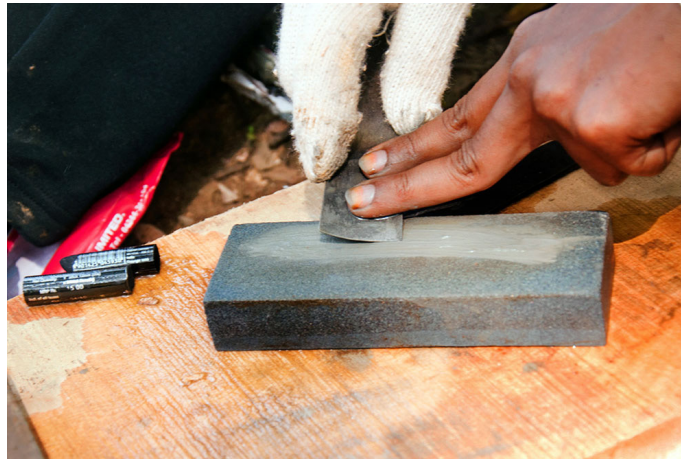
Chisels are rubbed to the carbide stone to sharpen it.
