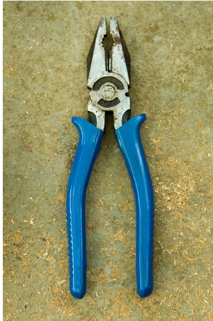
Cutting plier is used for cutting the metal wires.
