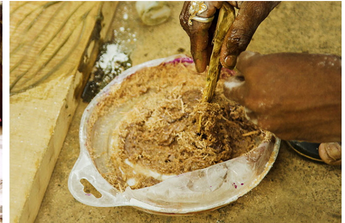
Then the wooden powder and adhesive agent (resin) are mixed.
