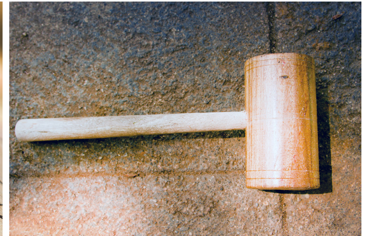
Wooden hammer is used to tap on the chisels with force to scrap out the unwanted outer layer of the wood.
