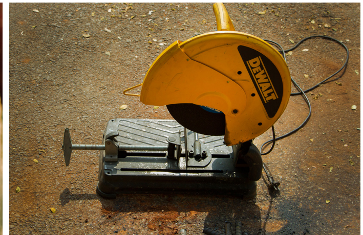
Rod cutting machine is used in cutting the metal rods.
