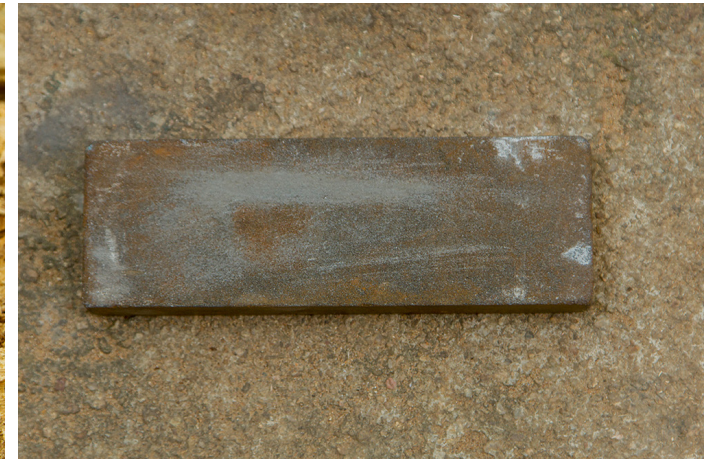
Carbide stone is used in sharpening the Chisels by rubbing it on stone.
