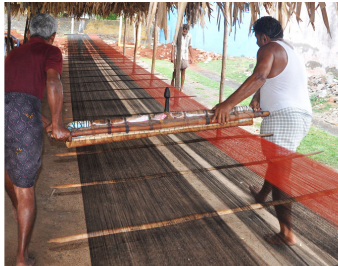
Natural brush is used to apply coconut oil on threads for softness.
