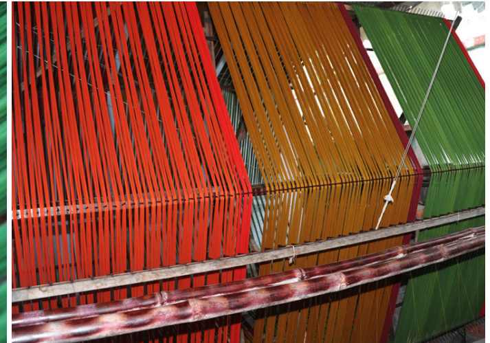
Three colors of sari yarn are reeled simultaneously to save the time.
