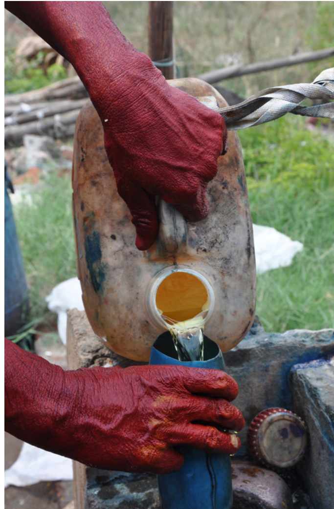
Diluted acid is used in washing process to give shine to the threads.
