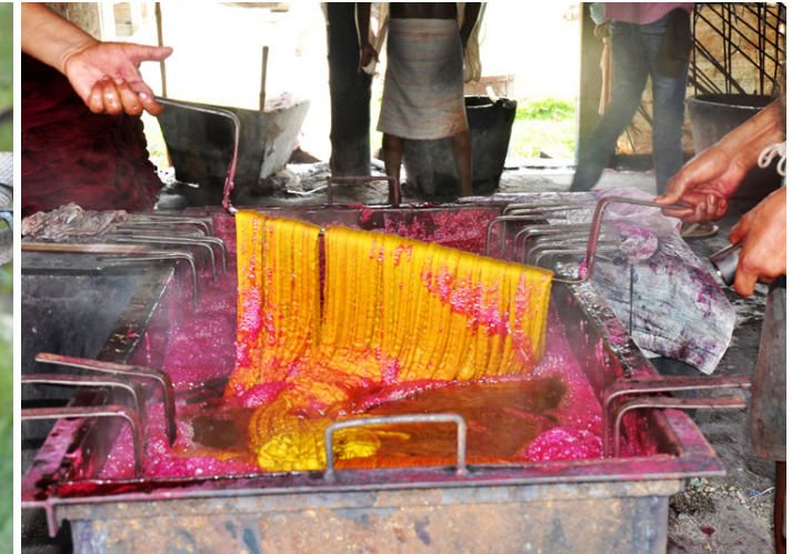
Metal handles used to steer the cotton thread while dyeing.
