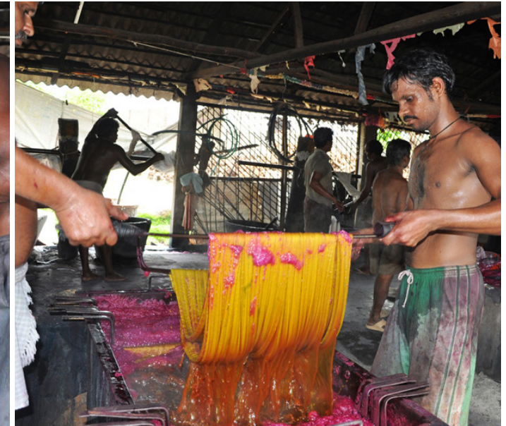
Thread bundles are rotated for proper color application.
