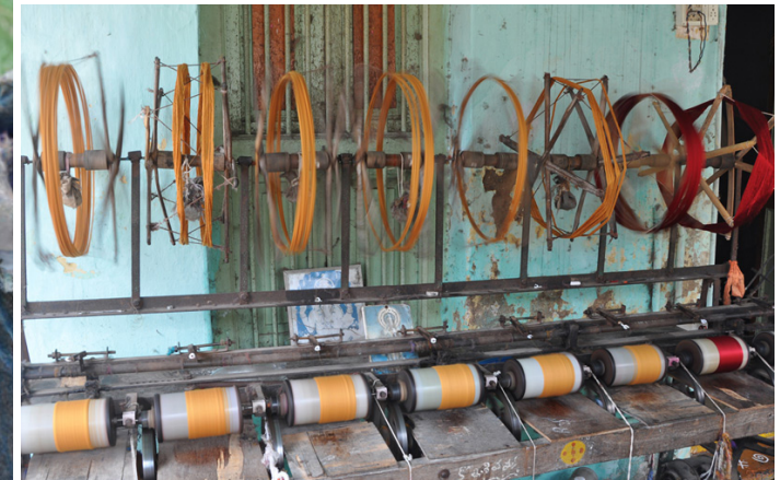
Reeling machine used to reel the cotton thread on spools.
