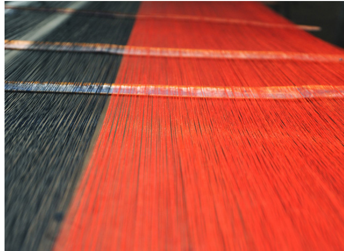
Application of starch strengthens the thread.
