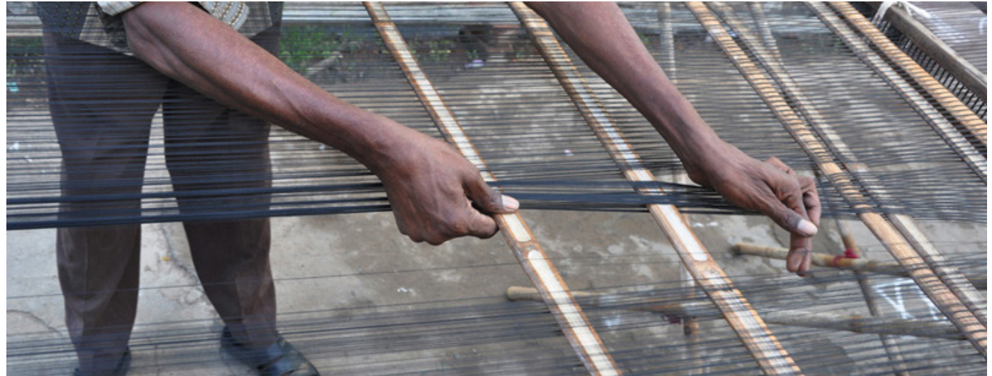
Bamboo sticks are inserted between the cotton threads.
