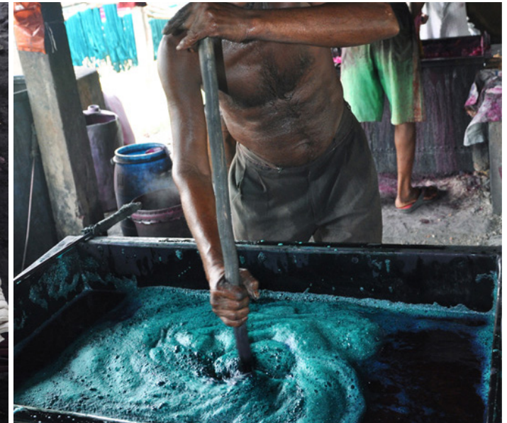
Dyeing color is mixed with hydrosulphite and costic acid is mixed in boiling water.
