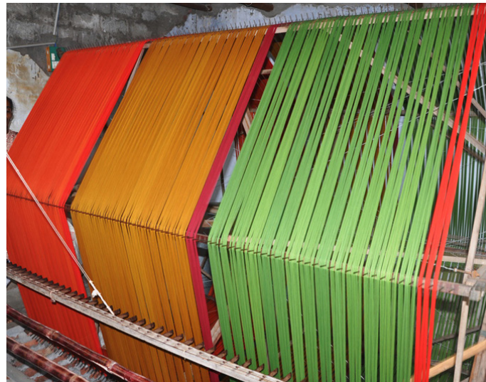
Bigger warping machine is locally called Aasu.
