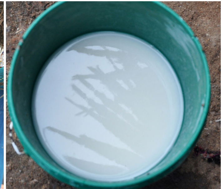
Rice starch used to strengthen the thread.
