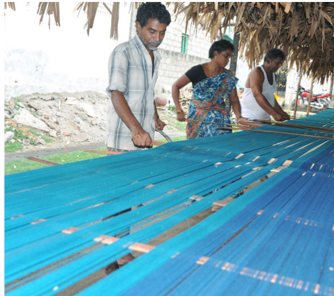
The view of using bamboo sticks while warping.
