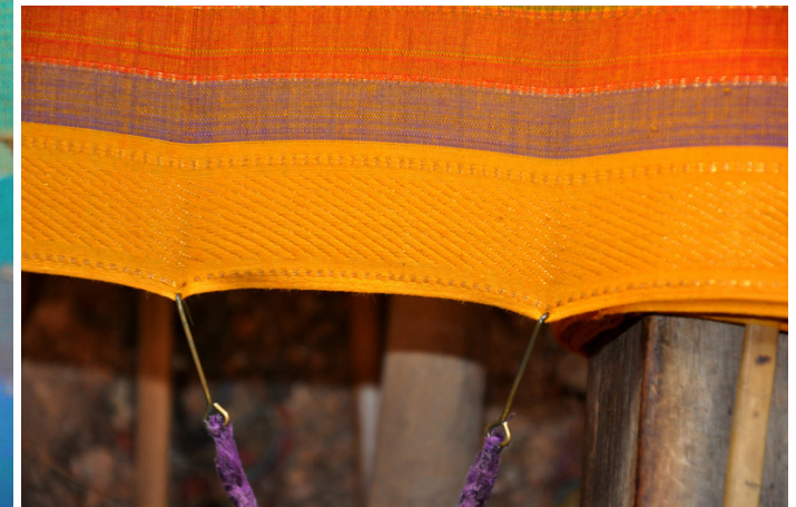
View of brass pins clamped to woven part of cloth.
