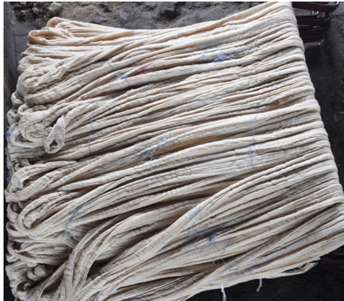
Plain cotton thread is boiled in water to clean and kept for drying.
