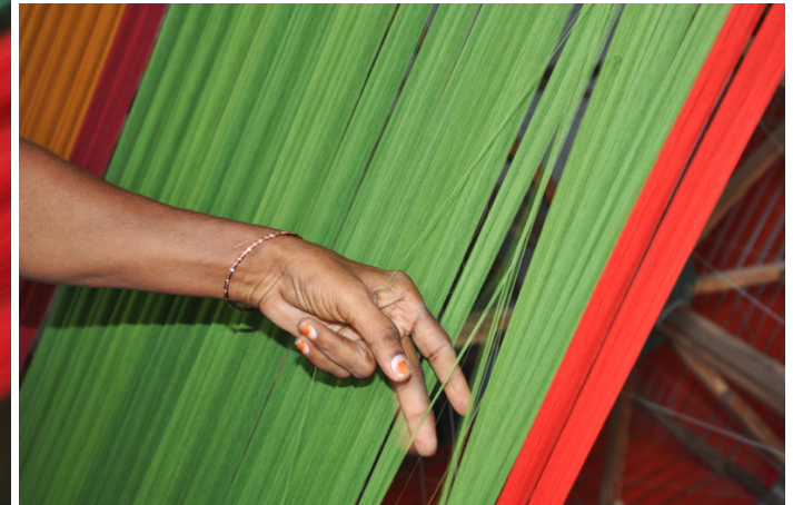
Knots and tangled threads are cleared to ensure smooth weaving.
