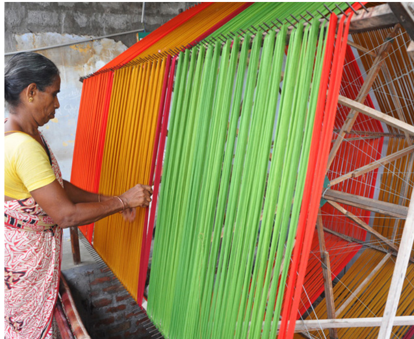
Cotton threads are rolled on the warping wheel.
