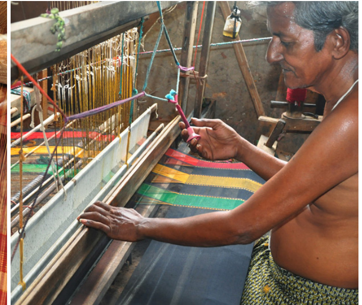
Once the shuttle is passed, the beater is pulled to join the threads.
