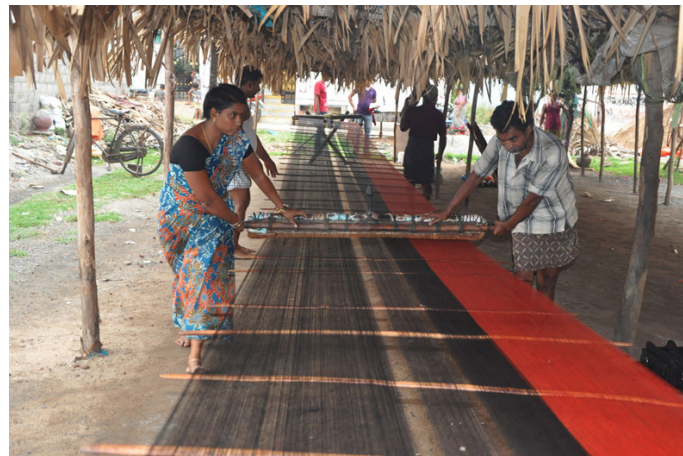
Coconut oil is spread using a brush for smoothing the threads.
