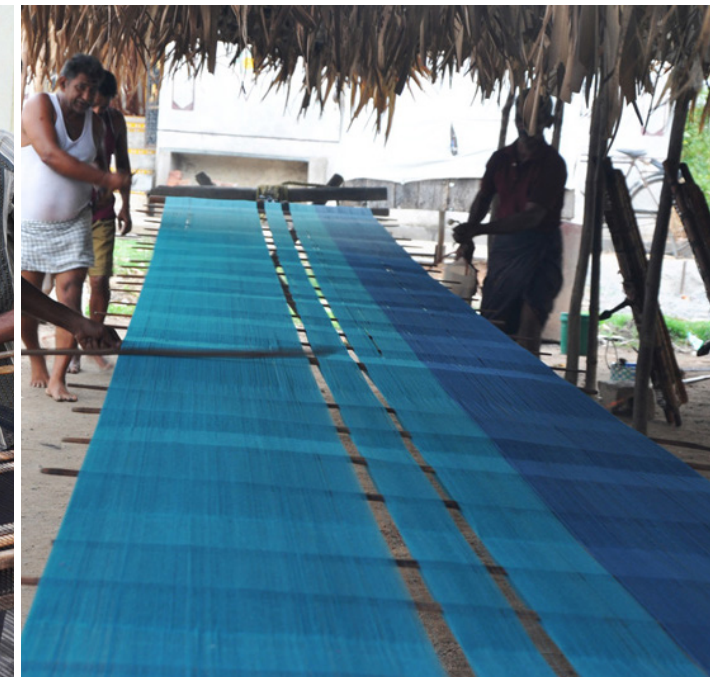
Starch is sprayed on the warp threads.
