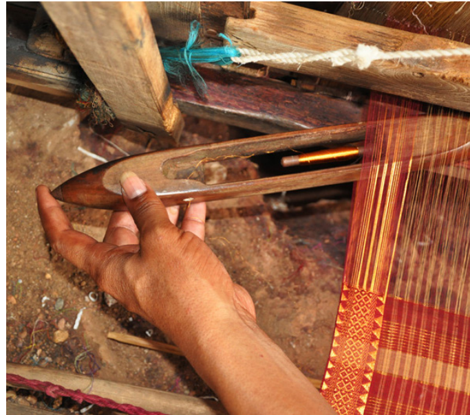
Fly-shuttle with spindle passes through the warp.
