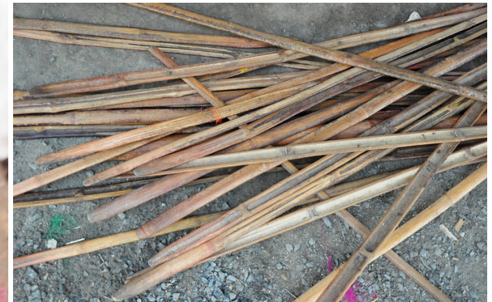
Bamboo sticks used to insert between the warp threads.
