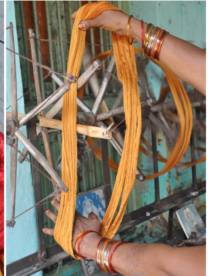
Yarn bundle is placed on wheel of automated spinning machine.
