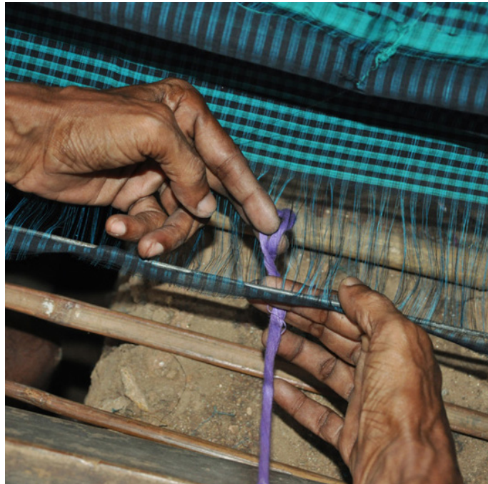
Initially, the warp threads are connected to the weavers beam.
