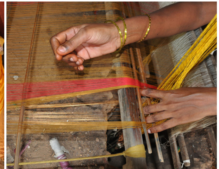
Few broken threads in warp threads are always joined and weaving continued.
