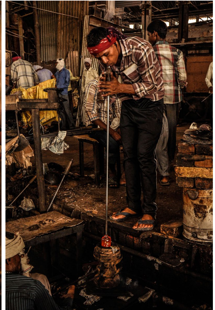
The glass material is put into a mold and blown to acquire the mold shape.
