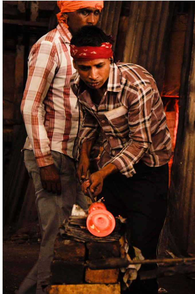
While shaping it is rubbed on a set of wet newspaper.
