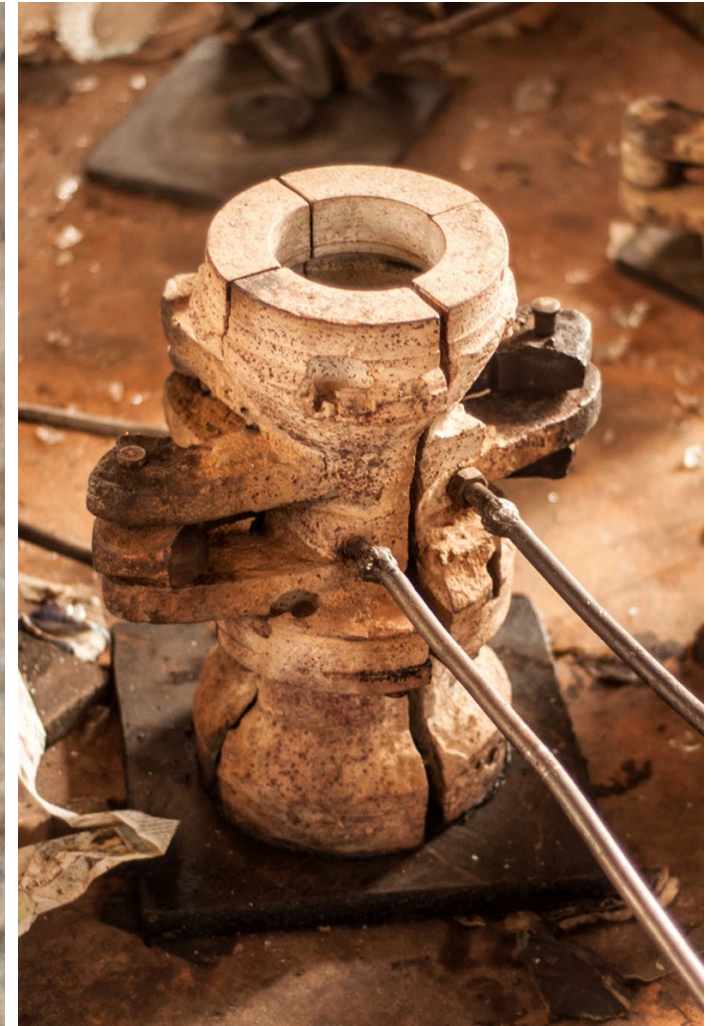
Mold used to make glass lamp stands.
