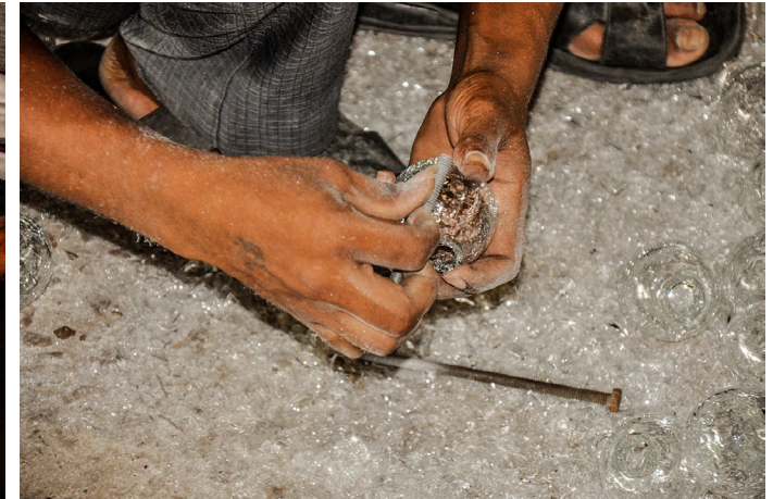
Surface of the articles are rubbed with screws to smoothen the surface.
