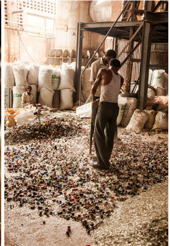
Waste glass articles are smashed and broken which is melted and used to make fresh products.
