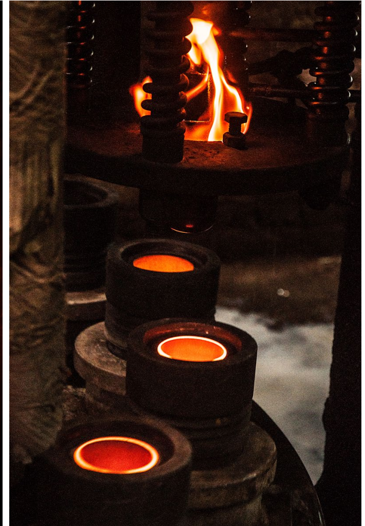
Molds are rotated on automatic machines to give shape to article.
