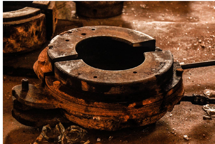
Mold used to make drinking or wine glasses.
