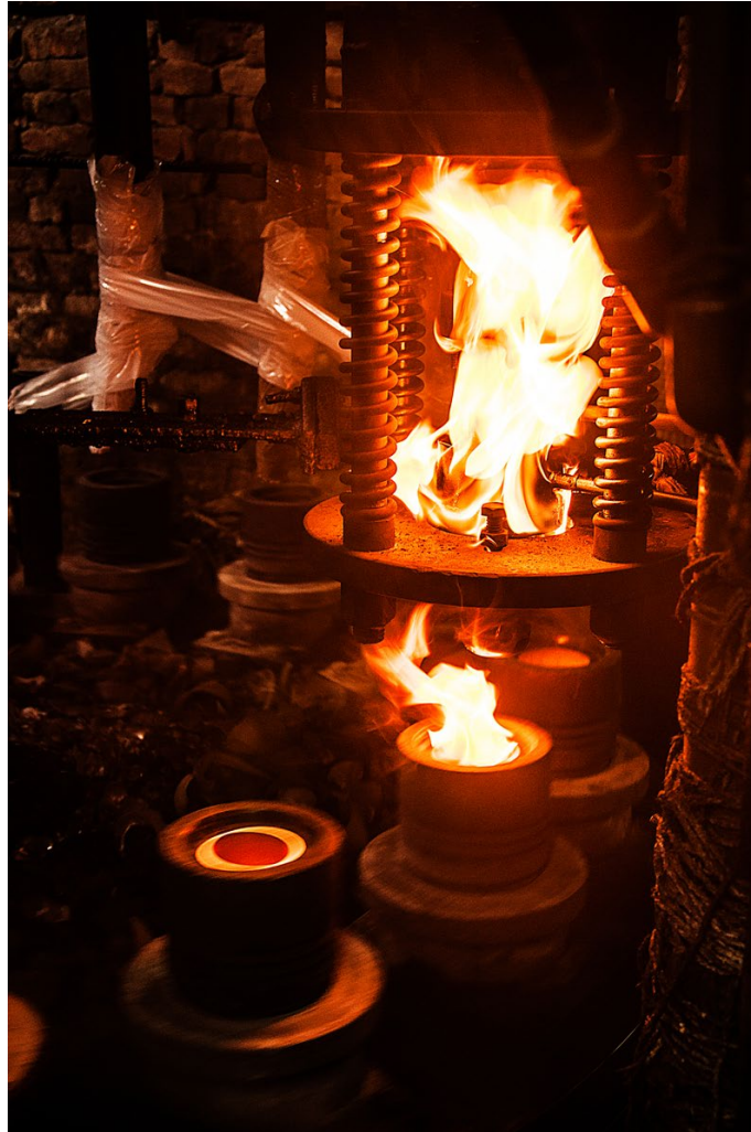
In another process molten glass is filled in molds.
