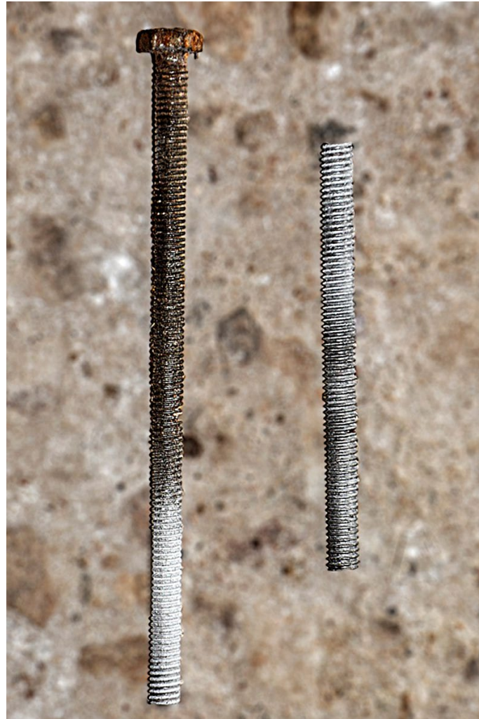
Screws used to rub on the glass articles to smoothen the surface.
