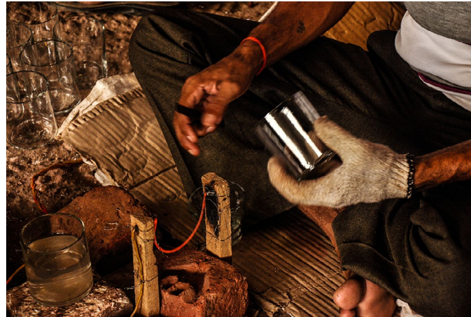
The heat slices the article separating the unwanted pieces.
