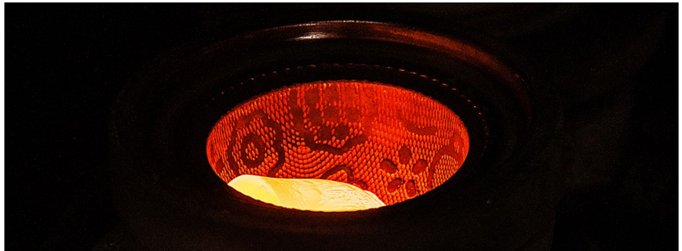
Molds with design used to emboss the design on the article.
