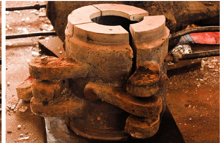
Mold to make design glass pieces for chandeliers.
