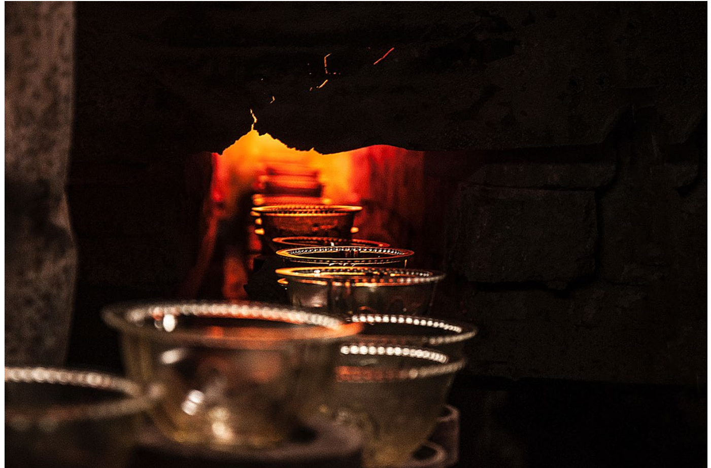
Prepared glass articles are passed through the kiln to heat the glass articles.
