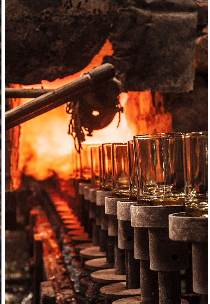
The prepared articles are again heated to fix the joints or cracks.
