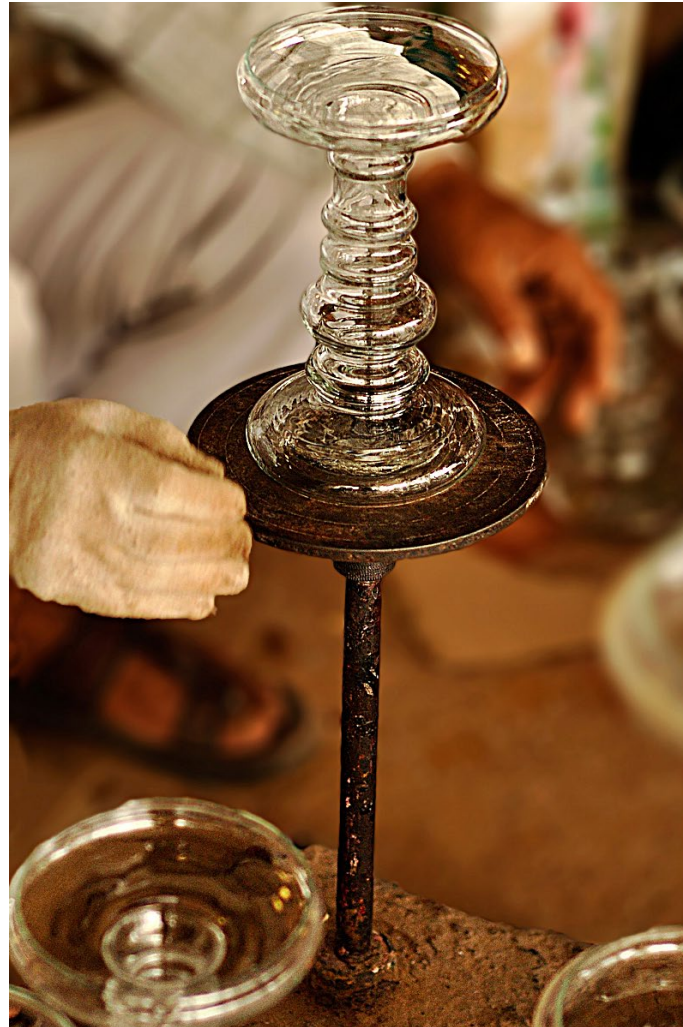
Rotating metal stand is used to check the products for damage.
