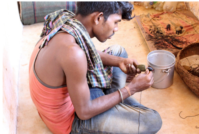
The wax is getting wrapped closely on top of the mold.
