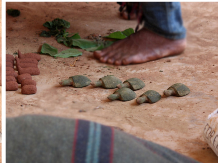
Bean leaf are crushed and apply over, which prevent the soil from sticking to the mold.
