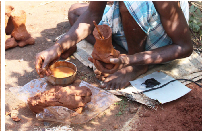
The wax runner is added to the top of the chamber.
