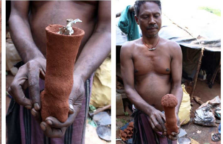
The metal is kept into the wax runner and cover with the clay.
