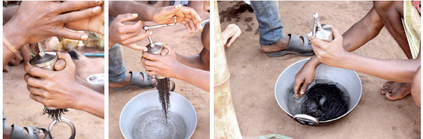
The wax is shaping into thread with the hand held press.
