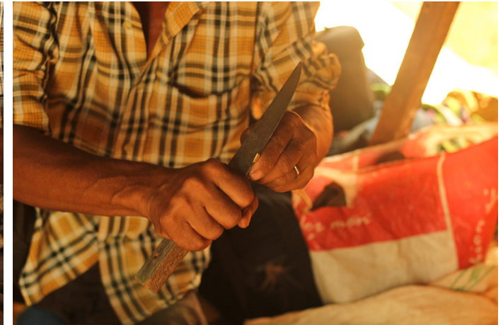
Rough edges are scraped out with knife.
