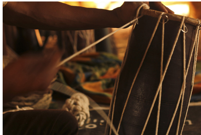
Metal rings helps in fine-tuning of the sound.
