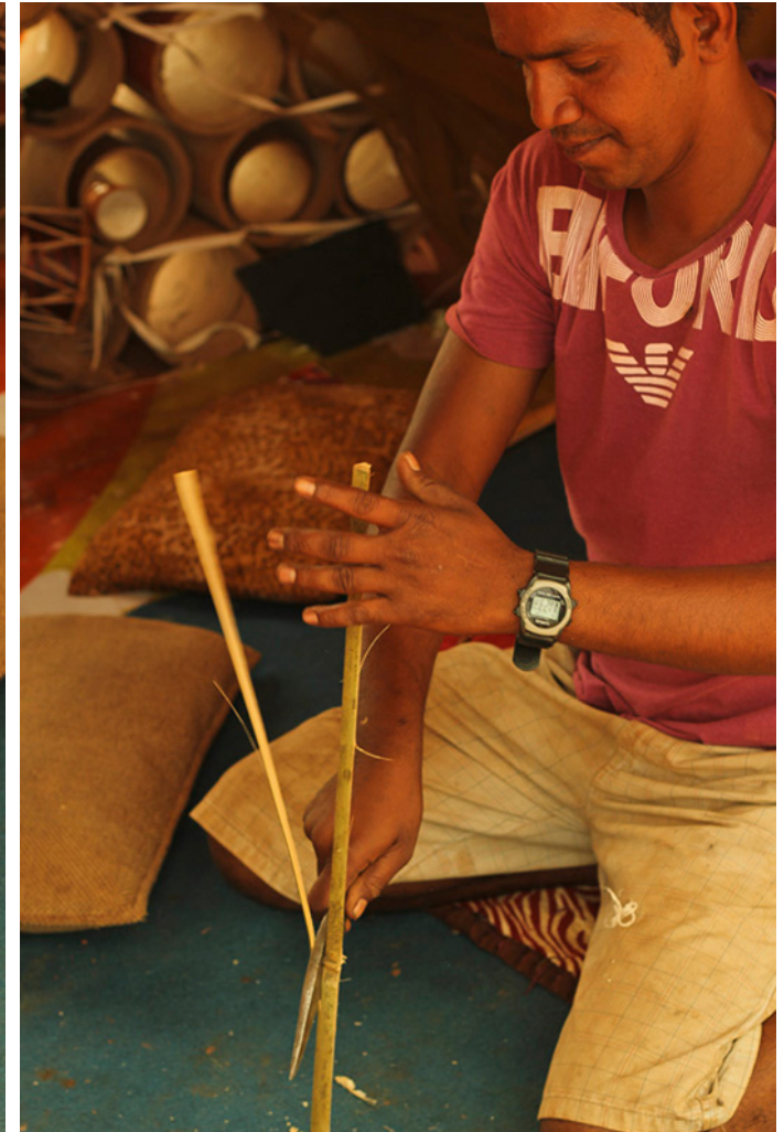
Bamboo is cut into thin sticks.
