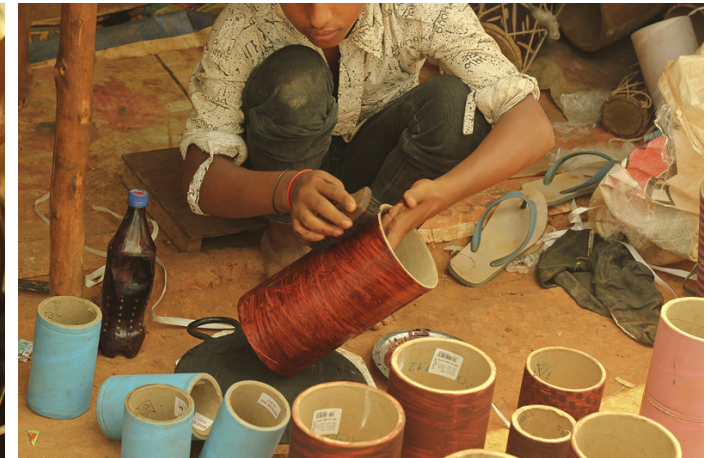
Using a shoe polishing brush, color is applied evenly.
