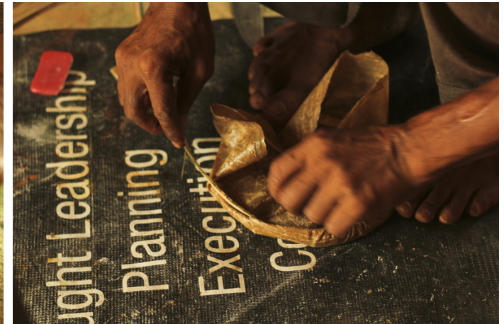
Another bamboo strip is inserted to prevent the leather from coming out.
