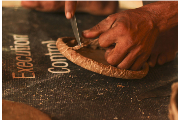
Excess membrane is cut using a knife.
