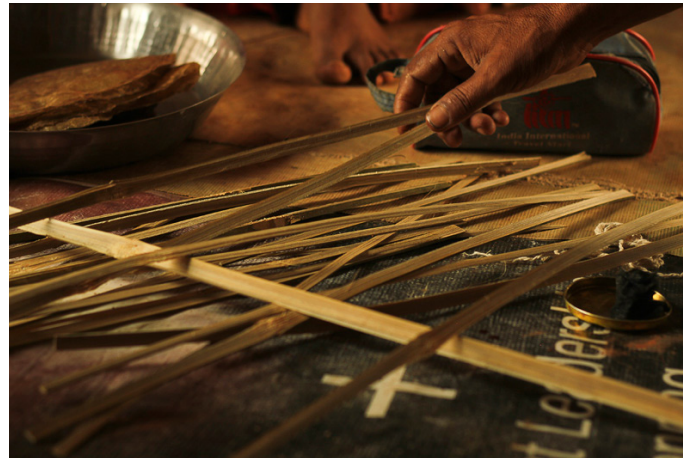
Bamboo strips are soaked in water to make them flexible.
