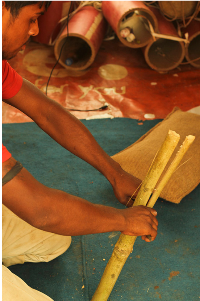
Bamboo logs are cut into half with a help of sharp knife.
