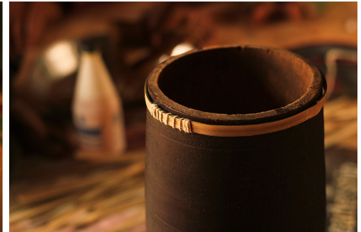
The rings are placed on the dholak body to ensure the measurements.
