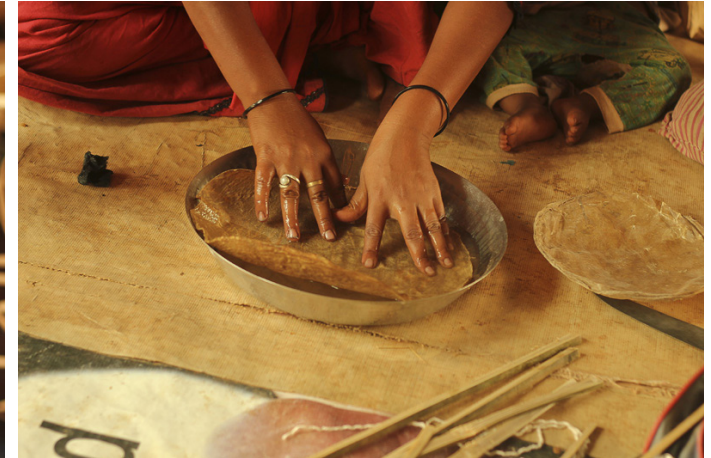
Leather (membrane) in circular shape is soaked in water.
