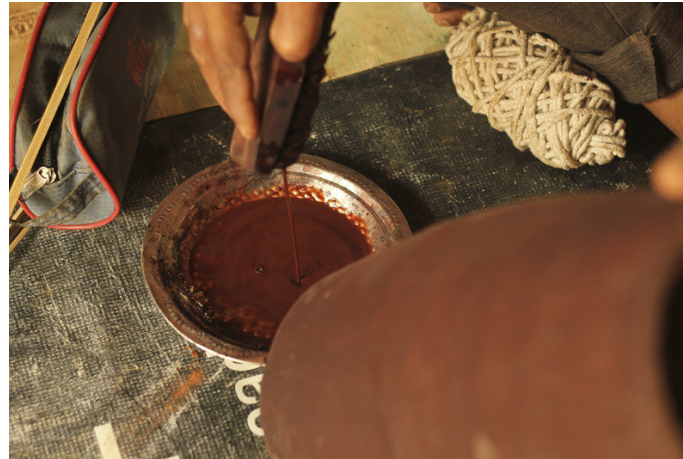
The mixture of Kataha, water and lime stone powder is applied on the barrel.
