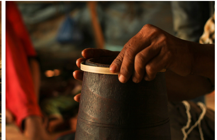
Bamboo strip is rolled around the end of dholak to get the measurement for the membrane.
