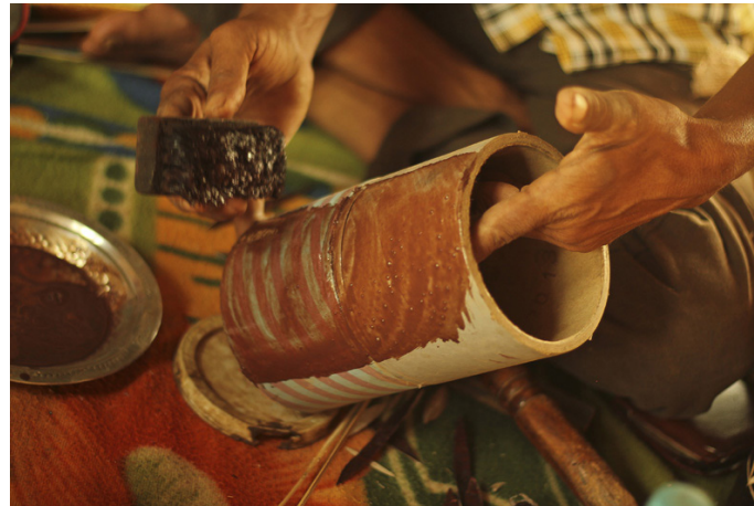
The prepared solution is applied on the roll.
