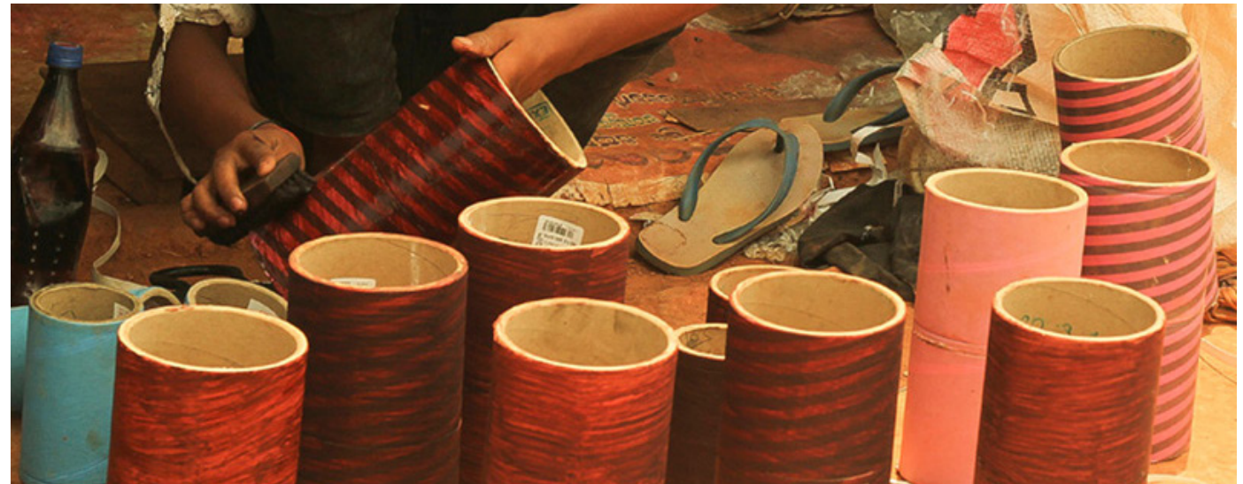
Body of the dholaks are polished and kept for drying.
