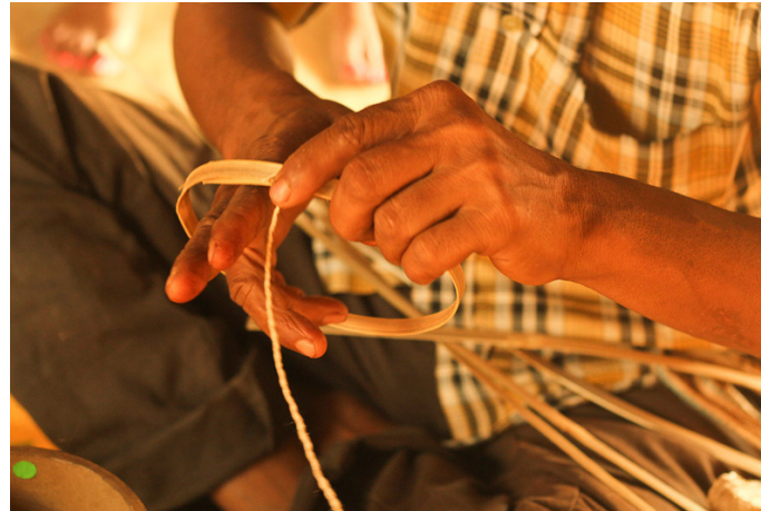
Bamboo strip is rolled to form a ring and tied with cotton thread.
