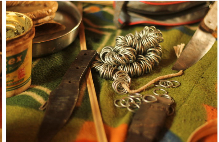
Metal rings are used to tighten the membrane for better tuning.
