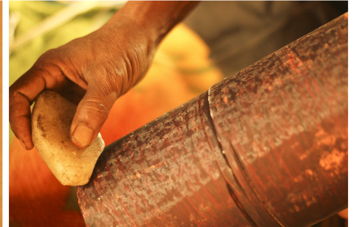
Bee wax is rubbed on the dried roll.
