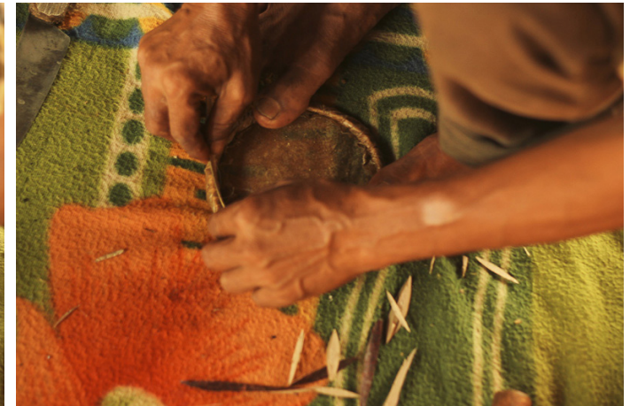
Supporting bamboo strip is inserted to lock the leather sheet and to prevent unlock.
