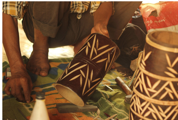
Wood turpentine is applied on the carved cardboard roll.
