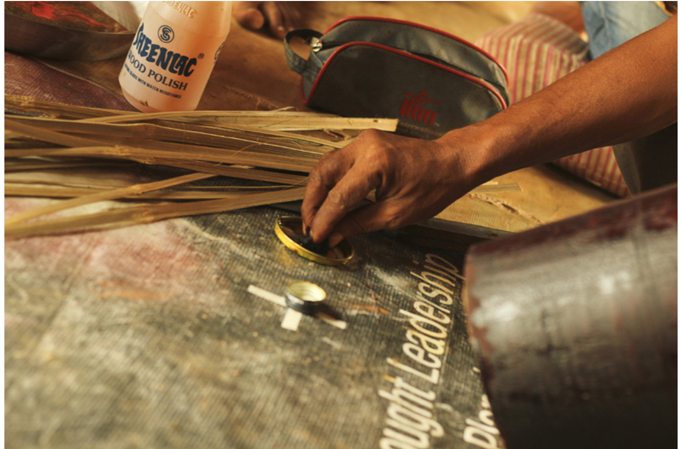
Wood turpentine is applied on the barrel.
