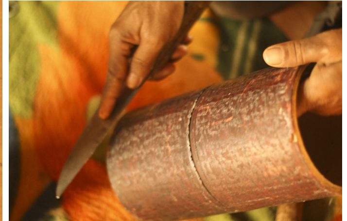
Surface of the roll is smoothen and the excess wax is scraped out using a knife.
