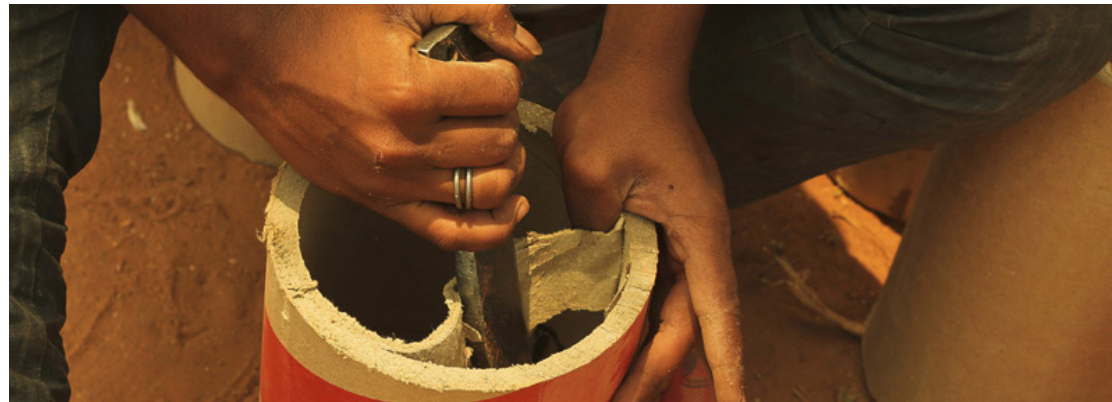
Excess material of the cardboard rolls are removed to reduce the weight.
