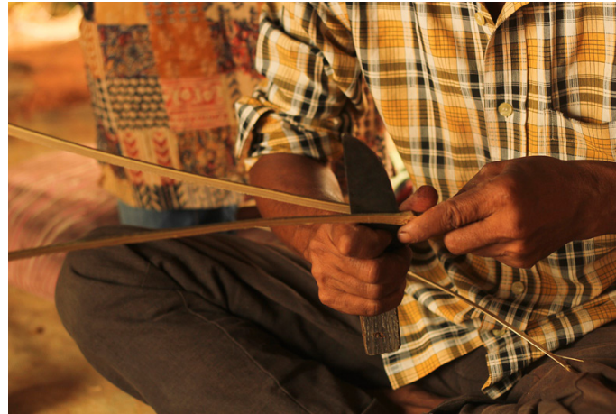
Thin strips are extracted from bamboo sticks.
