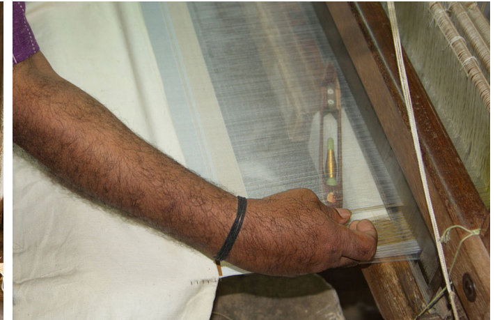
The weaver is inserting the fly shuttle inside the loom to get the golden zari as the border in the silk dhoti.
