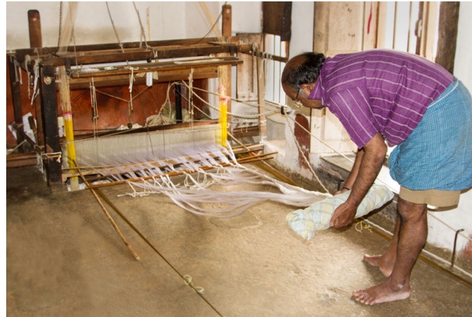
The silk yarn is equally spread out in the middle of the zari threads.
