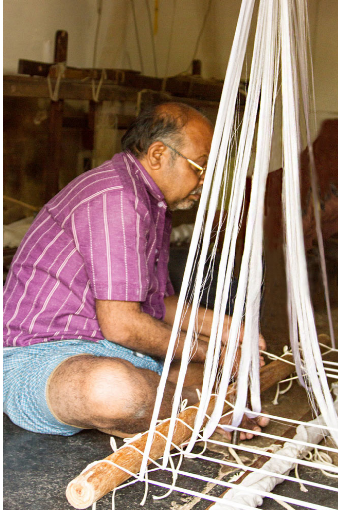
Weaver tying the silk yarns firmly to the wooden beam which are spread out from the heddle shaft.
