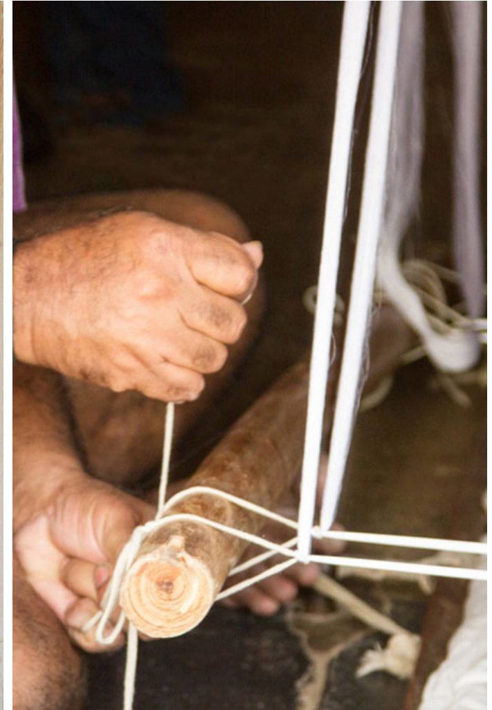
The process of tying the silk yarns to the wooden beam is begun.
