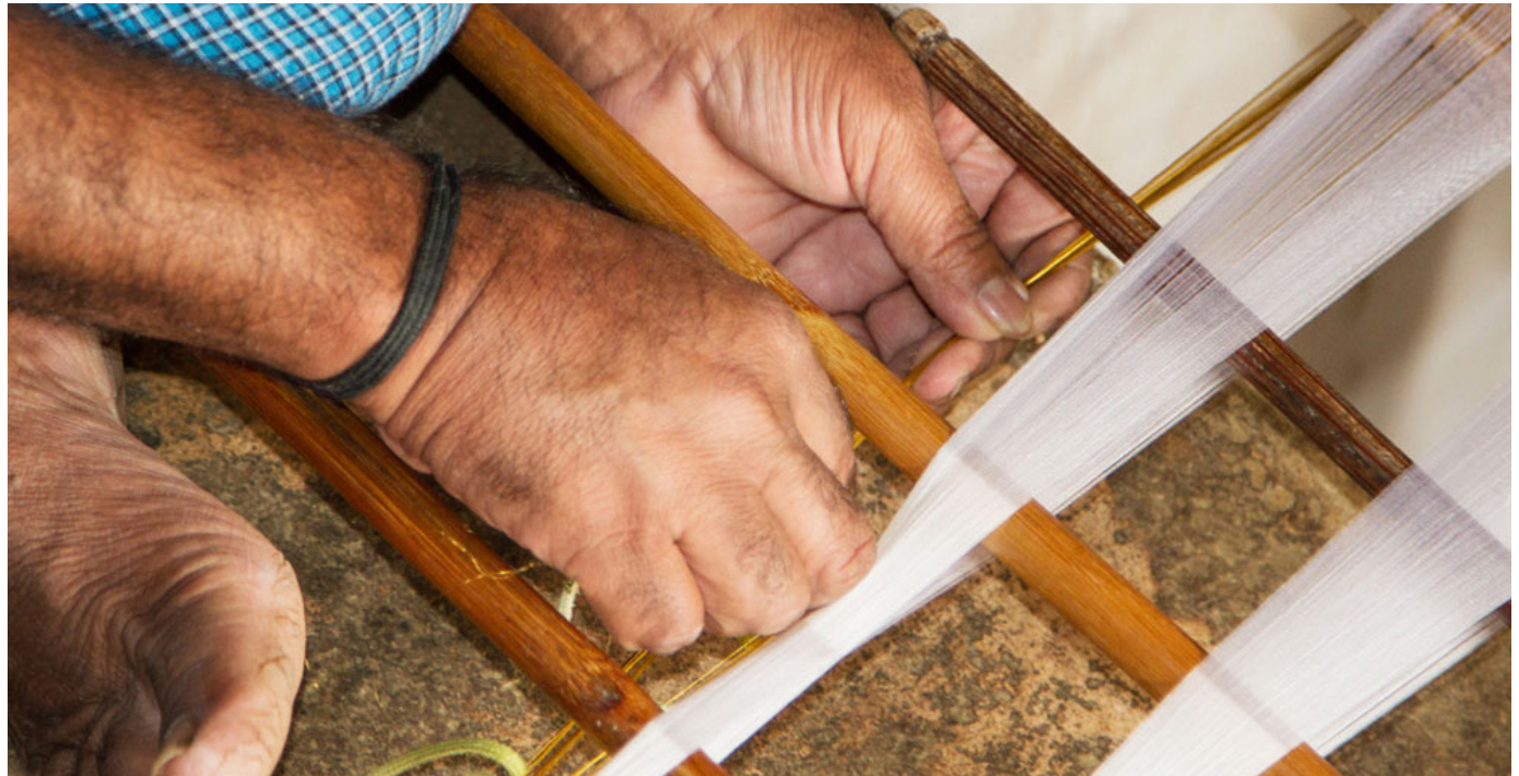
Warp yarns are divided and tied to the bamboo sticks so that they become warp beam.
