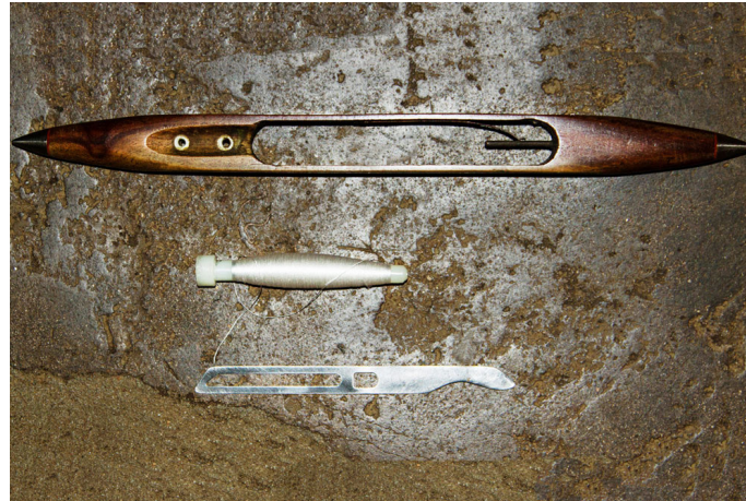
The fly-shuttle, fully loaded pirn and the sharp edged tool which is used to cut the thread.
