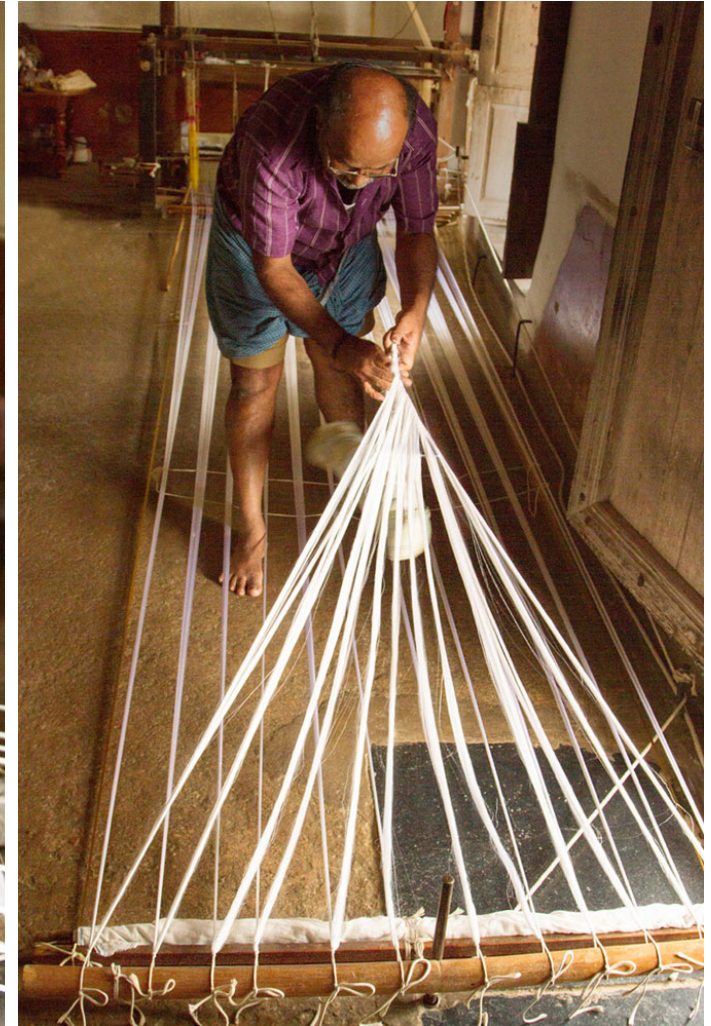
The excess of silk yarn is again twined and tied with the cloth and kept at the end.
