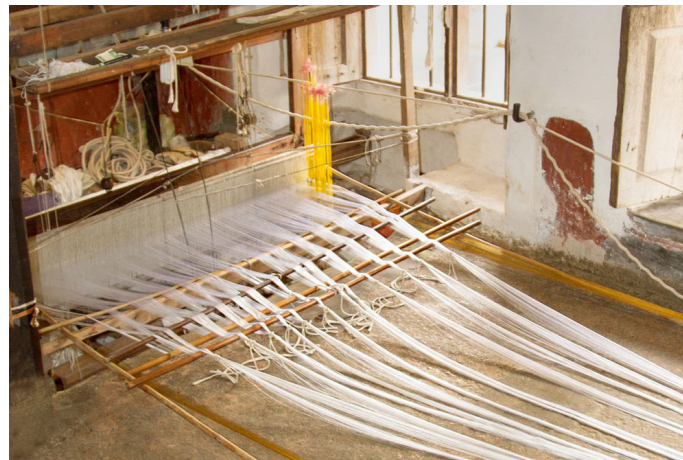
The close-up of the silk yarn and the golden zari threads spread out from the heddle shaft.
