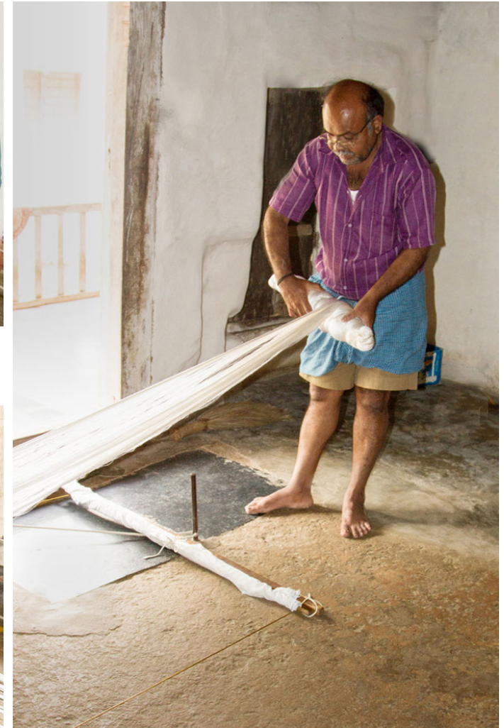
The excess of white silk yarn is rolled and tied with the cloth to avoid the yarn from getting dirty.
