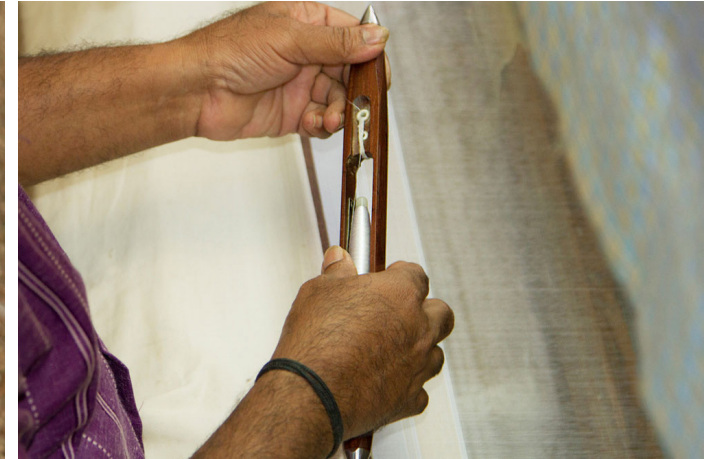
The loaded pirn is being inserted into the throw shuttle to insert the yarns while weaving.
