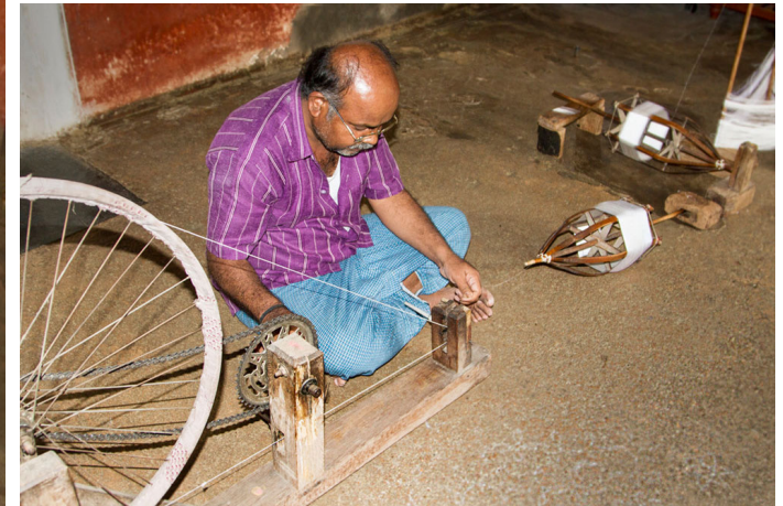
The pirn is being spun of silk yarn from the wooden Phirki.
