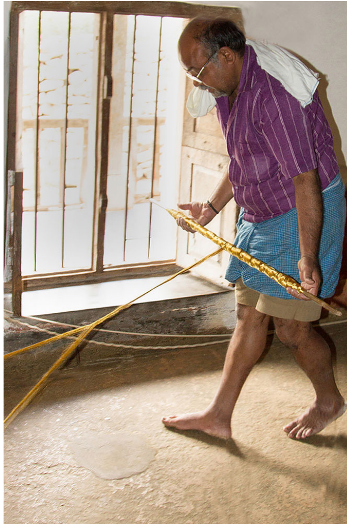
The golden zari is being spread at both the ends, till the required length.
