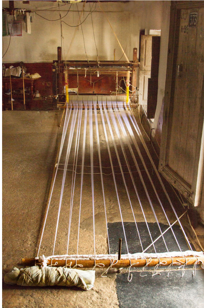
The loom is set completely with the silk yarns and zari threads for the further weaving.
