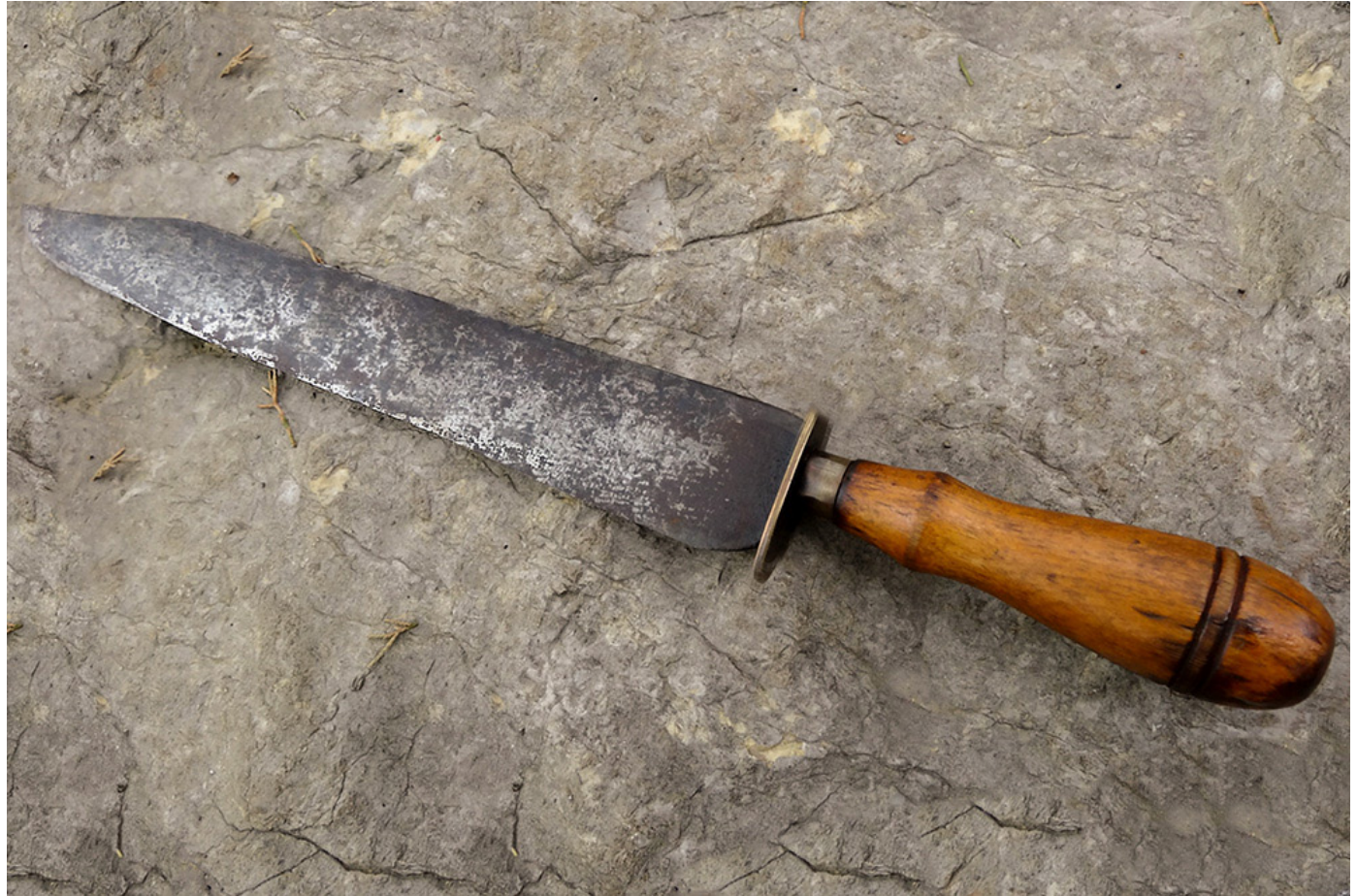
Knife to lacerate the outline of a Dhristi doll after it is being removed from the mold.
