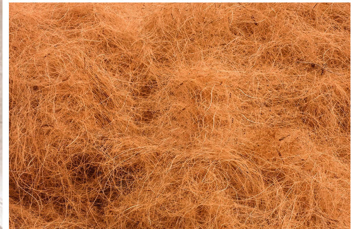
Coir is mixed with plaster of paris while molding to give strength.
