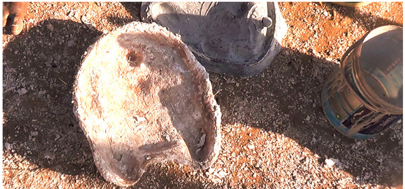
Depicted rubber mold with a base support of plaster of paris to get the shape.
