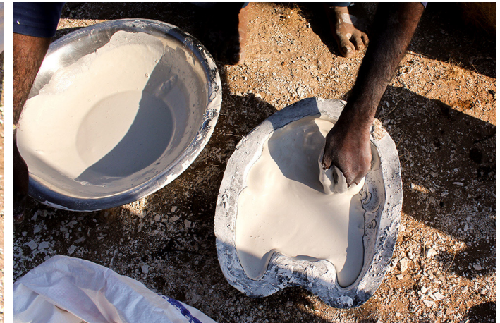
Replacing the POP liquid from bowl to the rubber mold.
