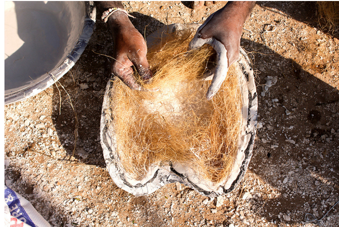
Covering up the POP liquid, complete with coir.
