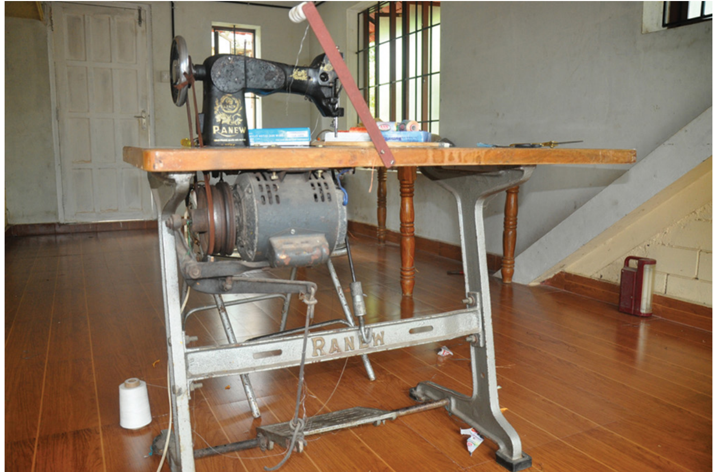
Embroidery sewing machine is used to make the embroidery work.
