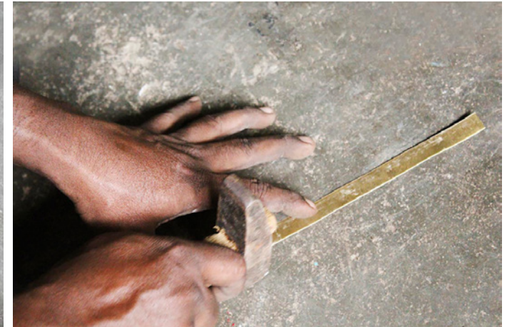
Metal strip is leveled by pressing it with hammer.
