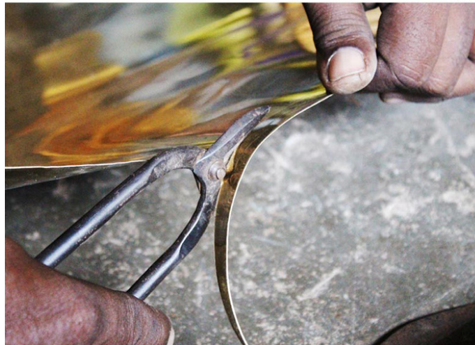
Brass sheet is marked according to the requirement and it is cut.
