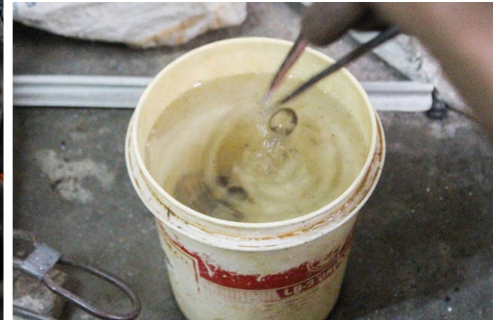
And dipped in water and allowed it to cool completely.
