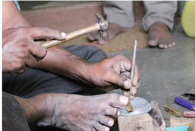
Small metal bits are designed at the border-using chisel.
