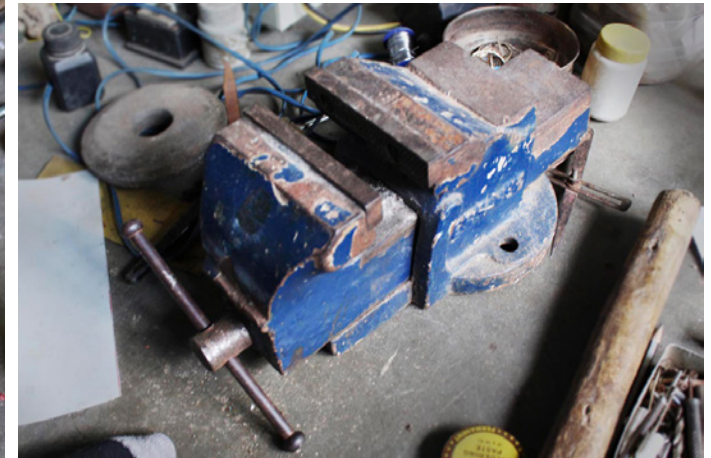
Holder in which the metal sheet is placed in it to file.
