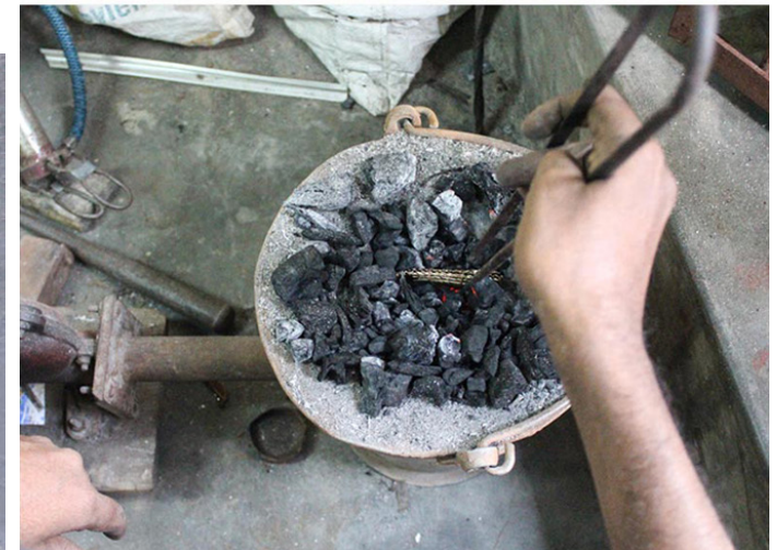
These brass bits are heated in the furnace.
