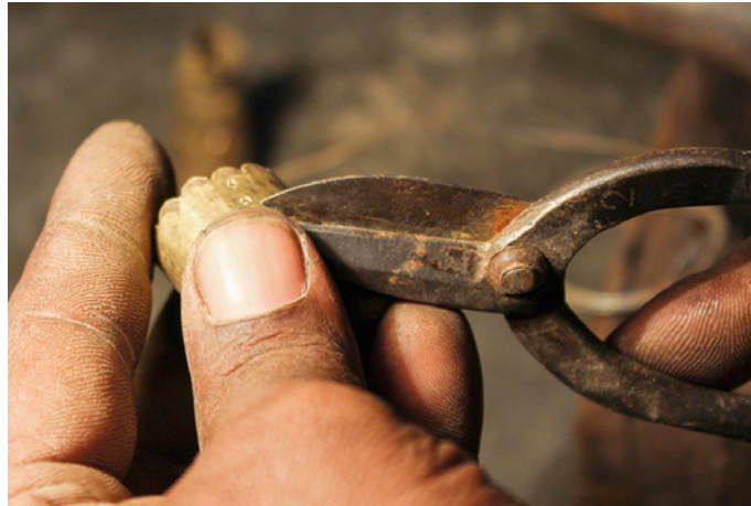
Metal scissor used for cutting the excess of metal.
