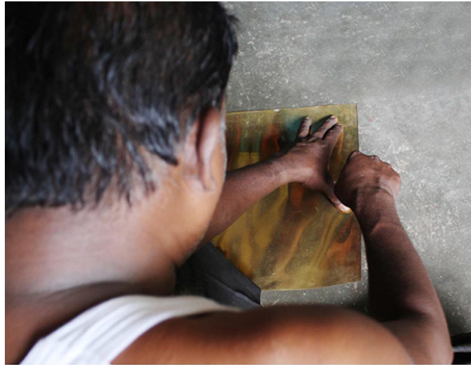
Metal strip is leveled by pressing it with hammer.
