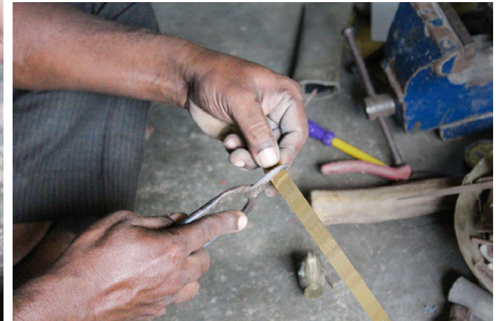
The metal strip is further cut into small bits as per the required breadth.
