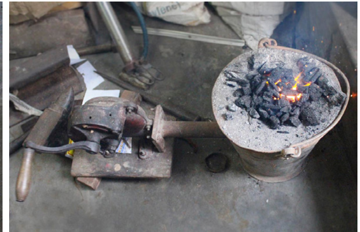
Charcoal is used in furnace to heat the metal sheet.
