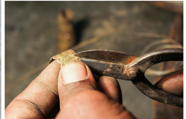
Excess of metal is precisely cut.
