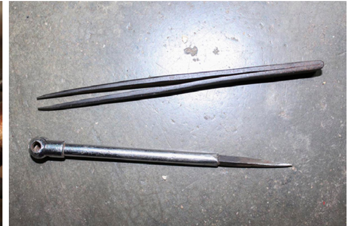
Metal holder and a pointed metal tool used while manufacturing the brass fish.
