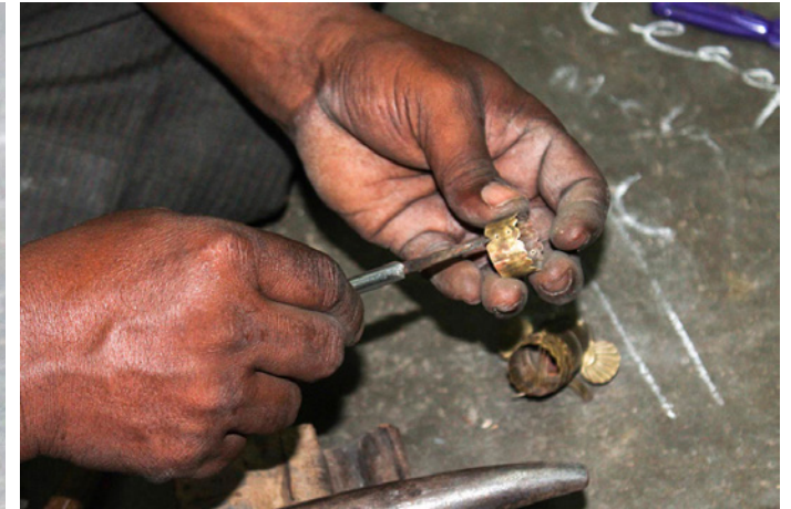
Circular forms are pierced through a sharp edged tool.
