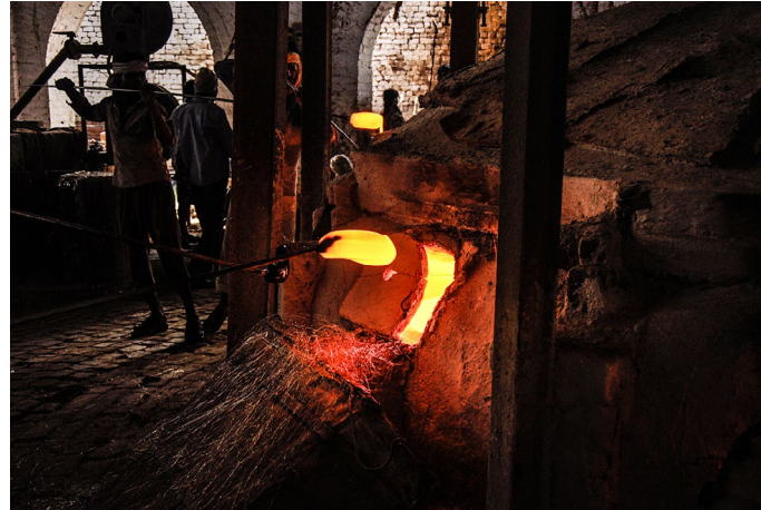
Molten glass is wound on a metal rod and taken out from furnace.
