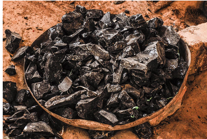
Black glass chunks is melted to make black color bangles.
