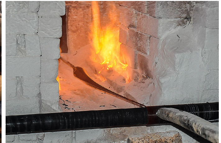
Prepared sphere is fixed in a kiln from which the material is pilled and placed on a metal rod.
