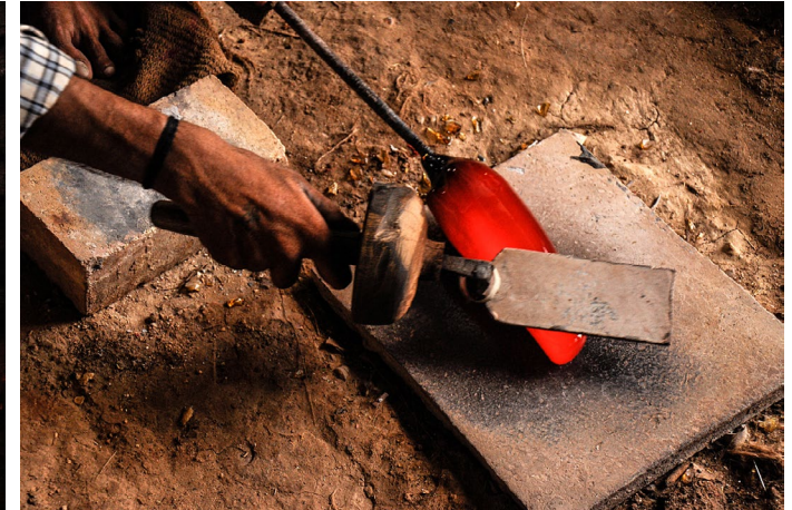
With a costumed tool the molten glass is shaped in a spherical shape.
