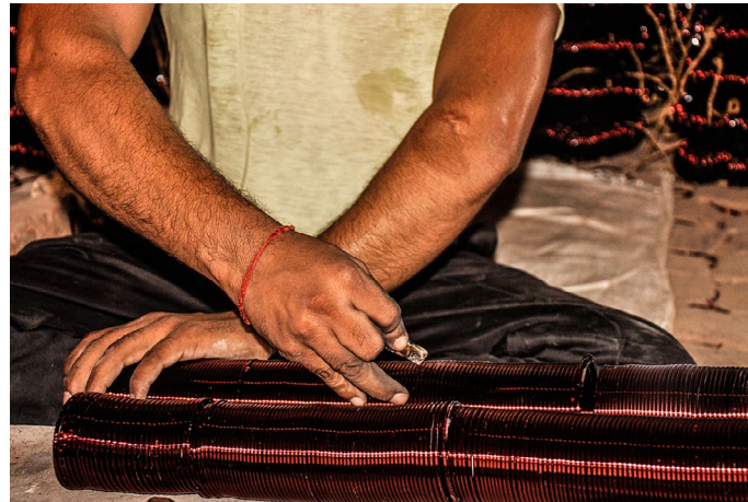
The bangles are the cut with diamond cutter to break the spiral.
