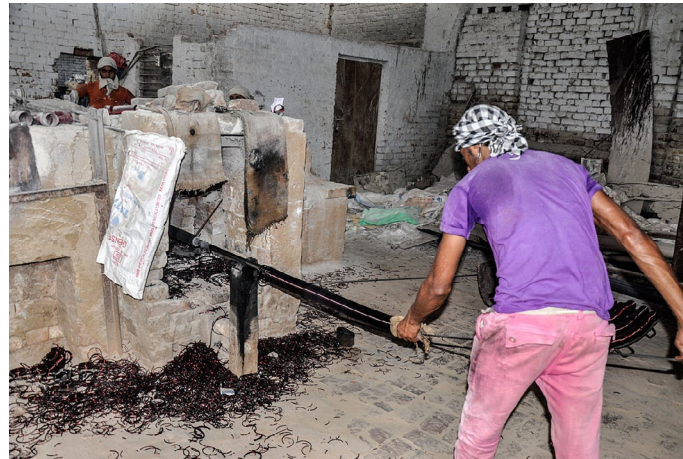
Craftsmen removes the bangles from the kiln.
