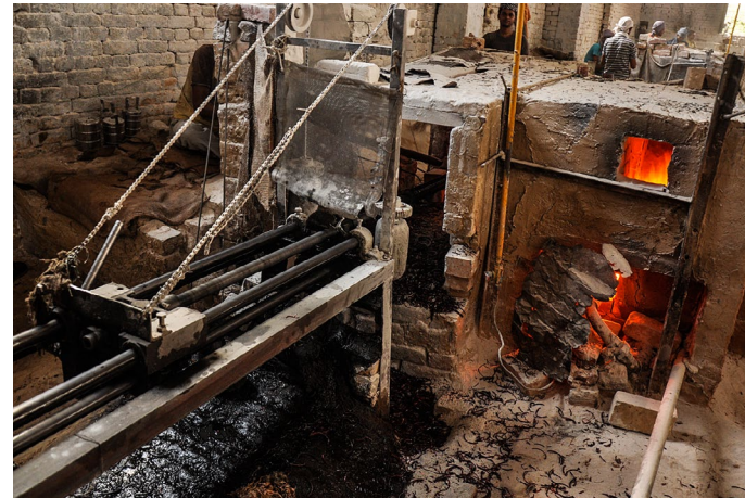
Kiln where the glass material is melted at high temperature.
