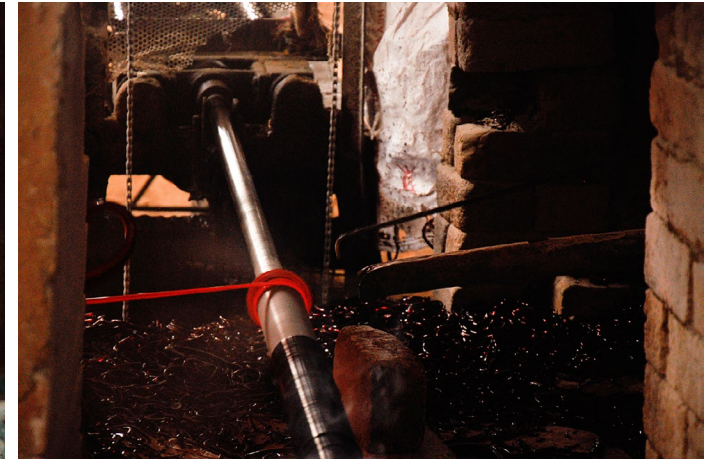
Liquid glass material is wound on a metal bar in spiral form to make a series of bangles.
