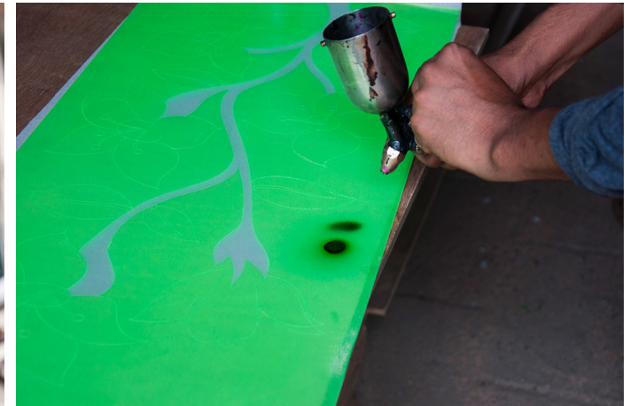
The color and its consistency are checked initially in a corner.
