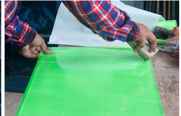
And the Vinyl sticker is stuck on the slab and by using scrub sponge pad air bubbles are removed.
