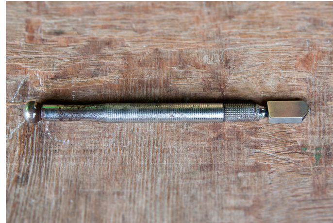
Diamond cutting tool used in cutting the glass according to the required measurement.
