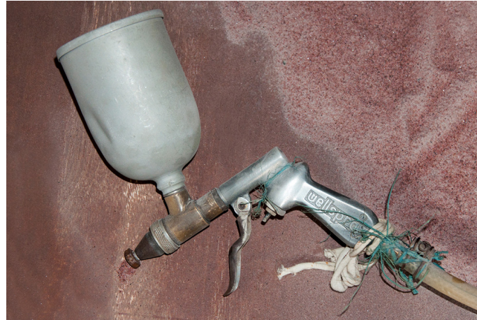
Gas gun is used for spraying the color on the glass.
