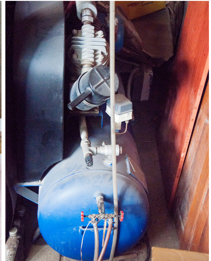
Air compressor machine that is attached to the gas gun, which is the main functioning motor.
