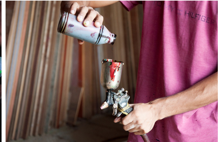
Required color for enamelling the frosted glass is poured in the gas gun.
