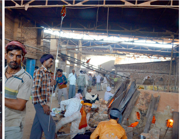
The craftsman getting glass the furnace on a metallic pipe.
