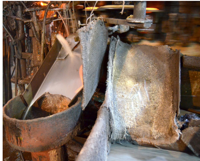
Conveyor belts to cool off the shell.
