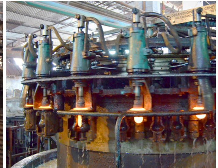
The automatic 'forming machine' making the glass shells.
