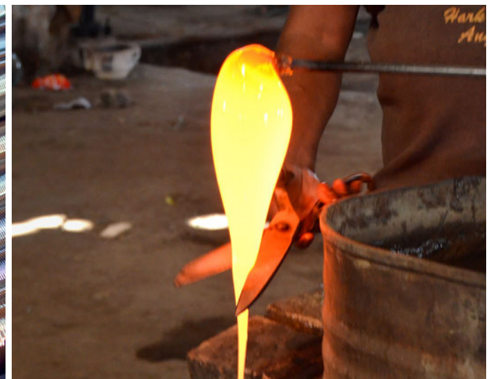
Another glass stream being cut to be coiled into bangles.
