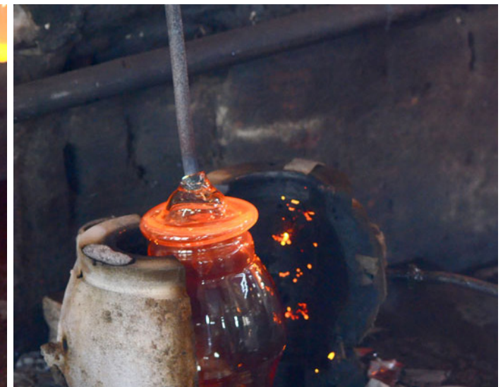
And the jar takes the shape of the mould.
