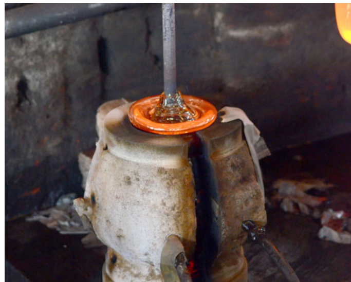
Mould being opened.
