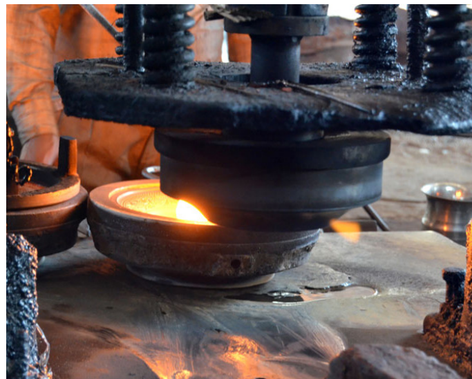
The moulds being pressed against each other to make the plate.
