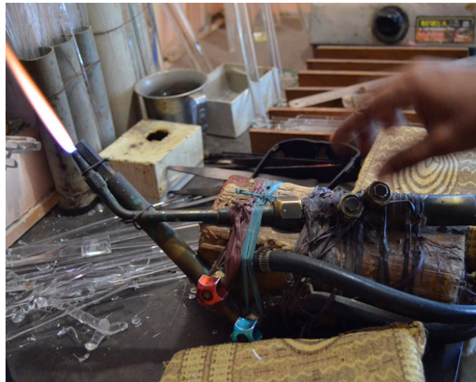
Gas burners for melting and fusing the glass.
