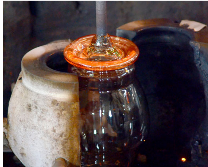
The jar ready to be removed while another gob is introduced in the mould.
