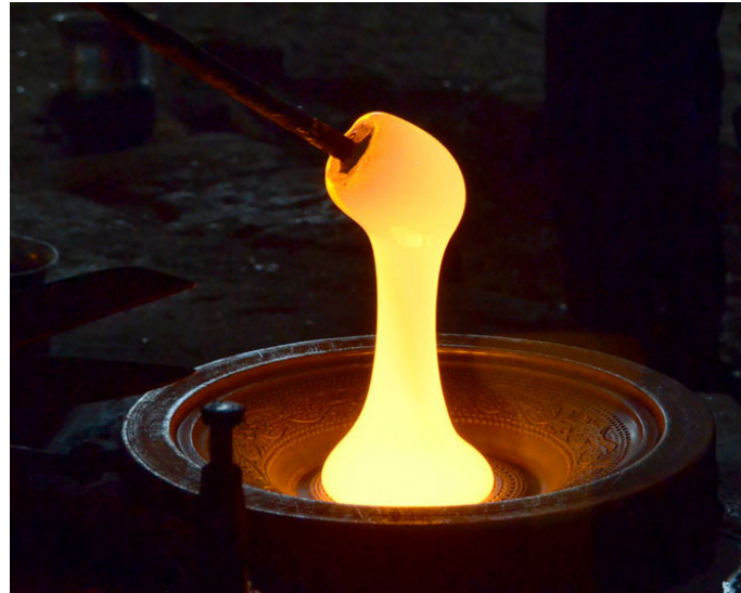
Stream of glass being put in the moulds.
