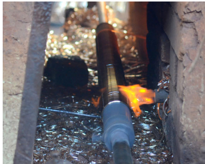
Heat is constantly supplied so that the bangles don't crack because of sudden cooling.
