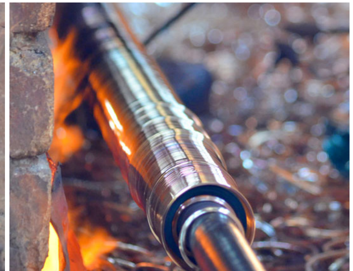
Heat is constantly supplied so that the bangles don't crack because of sudden cooling.
