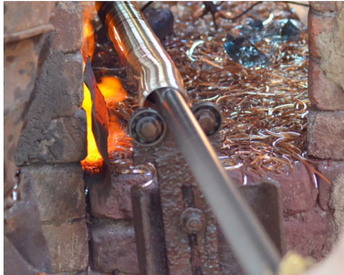
Since the rod is filled up, the bangles are being removed. Since the rod is filled up, the bangles are being removed.
