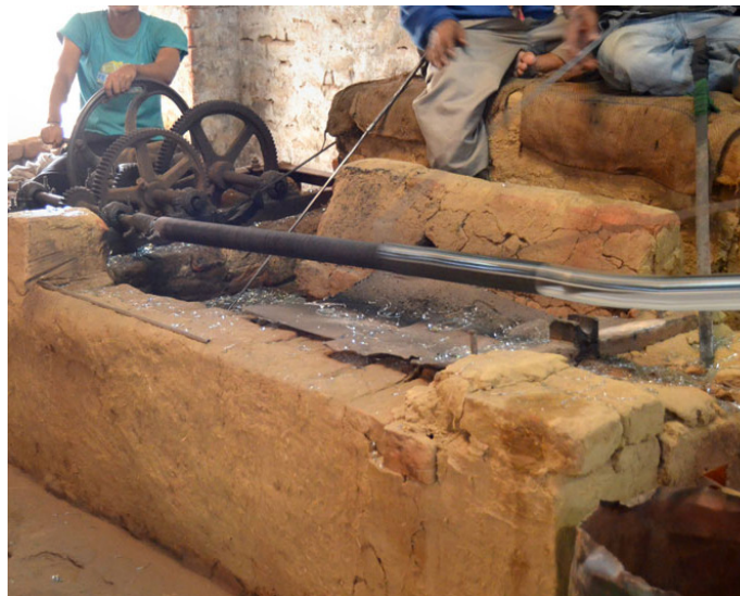
Bangles being removed from the rod.
