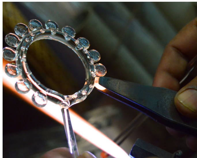
Flattening the circle with a tong.
