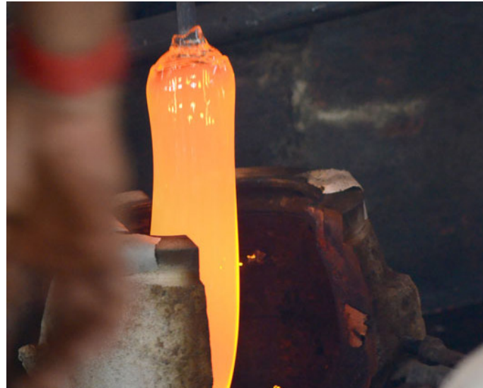
Gob falling by gravity.
