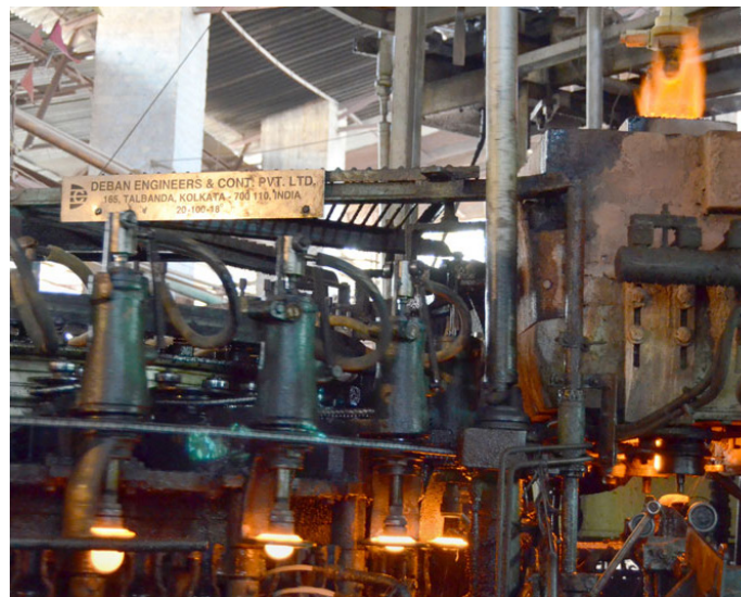
The automatic 'forming machine' making the glass shells.
