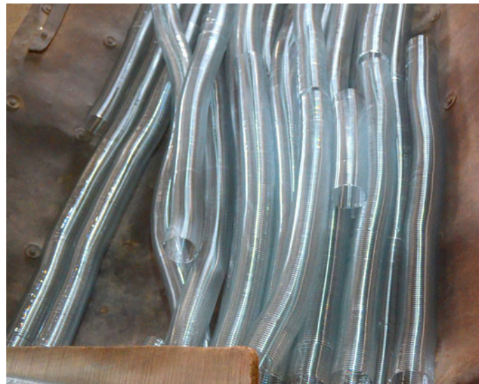
Glass spring generated by coiling the glass.
