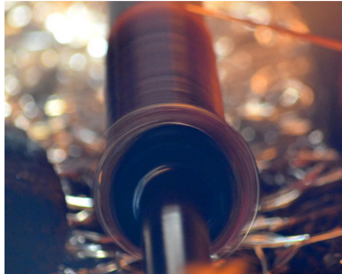
The thin glass coiling around the rod and taking the shape of the bangle.
