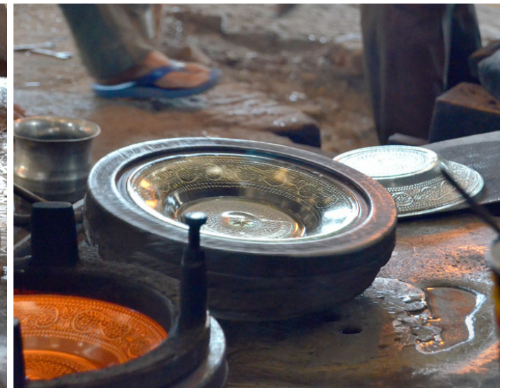
The plate takes the shape of the mould.
