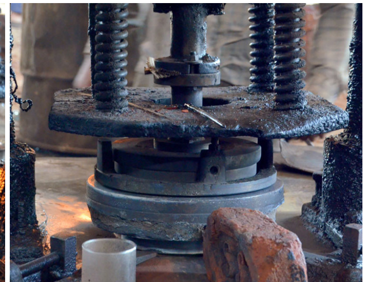
The moulds being pressed against each other to make the plate.
