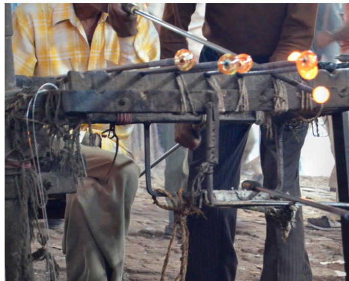
Air being blown from the other end of the hollow pipe.
