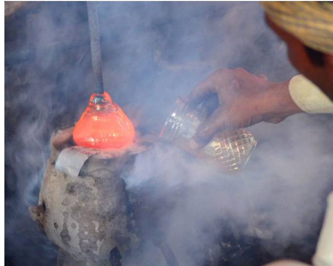
Water being sprinkled to cool off the mould.
