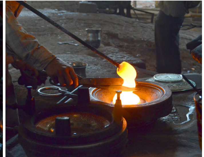
Stream of glass being put in the moulds.
