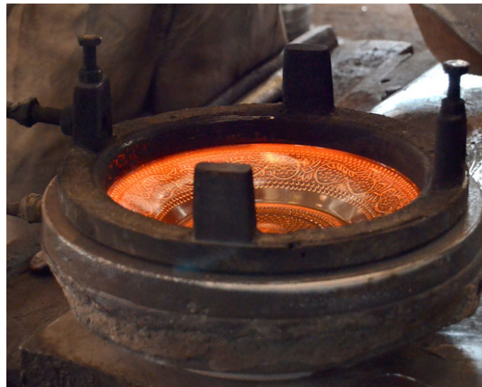
The plate takes the shape of the mould.
