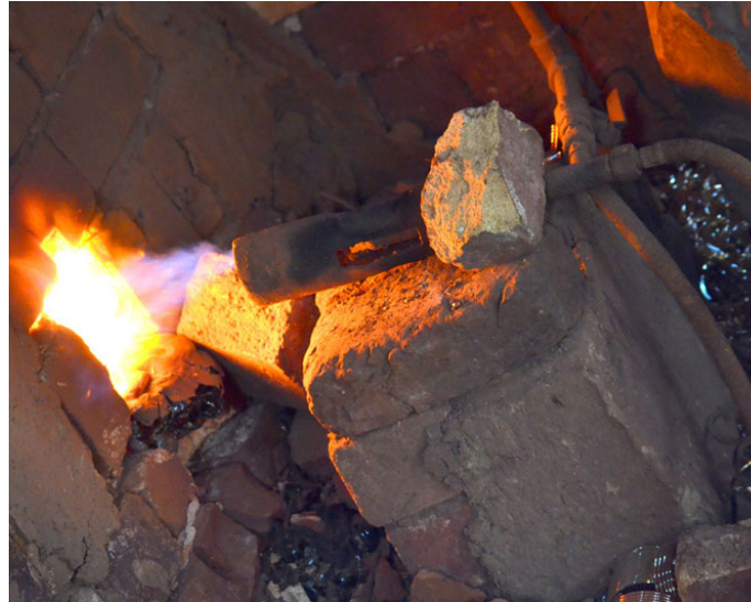
The gas burner of the furnace.
