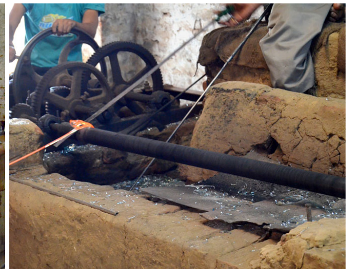
Glass being put on to the bangle rod.
