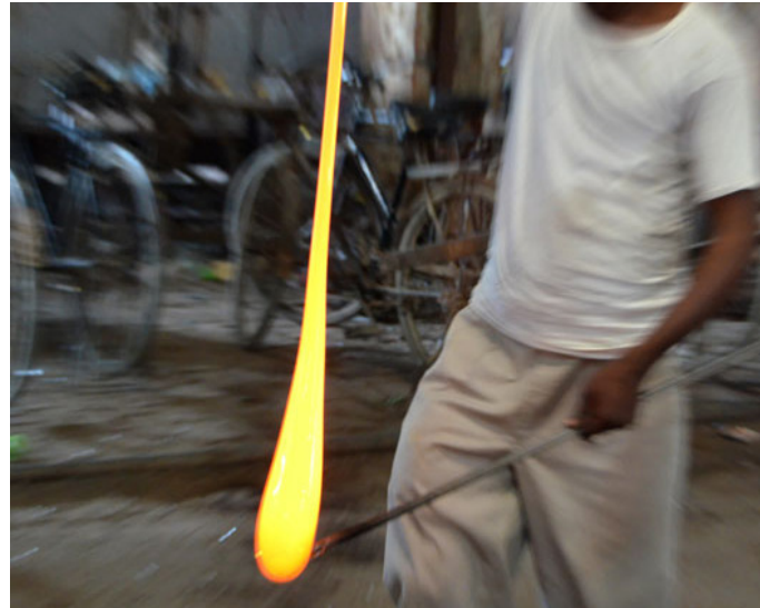
A craftsman preparing the glass stream to be put on to the bangle rod.
