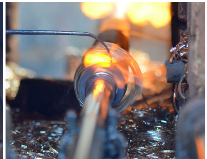
A pointed tool preventing the bangles from sticking with each other.
