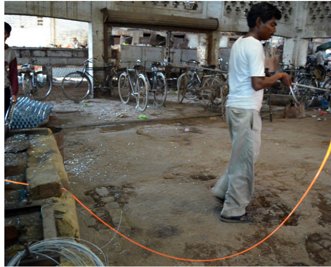
Glass being put on to the bangle rod.
