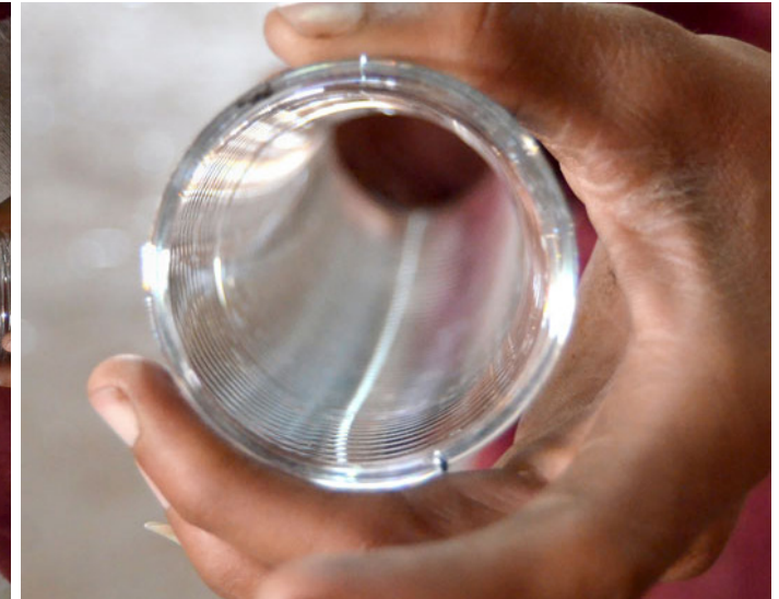
Glass spring generated by coiling the glass.
