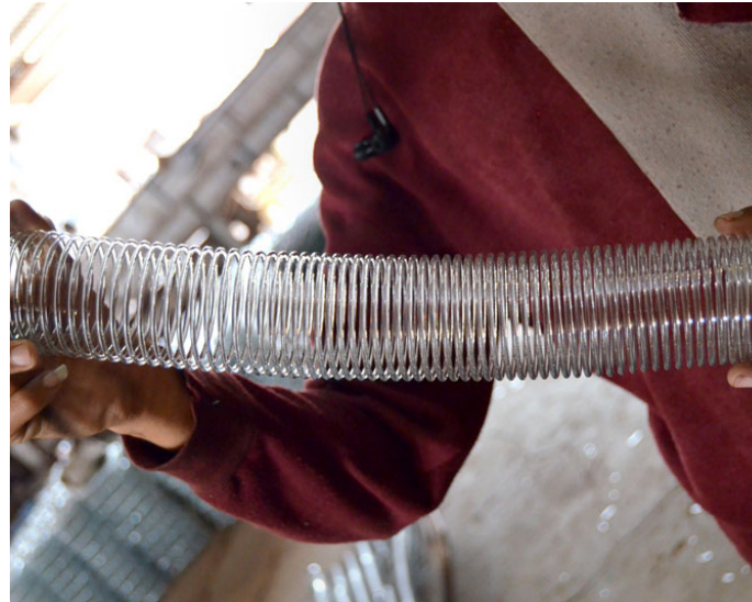
Glass spring generated by coiling the glass.
