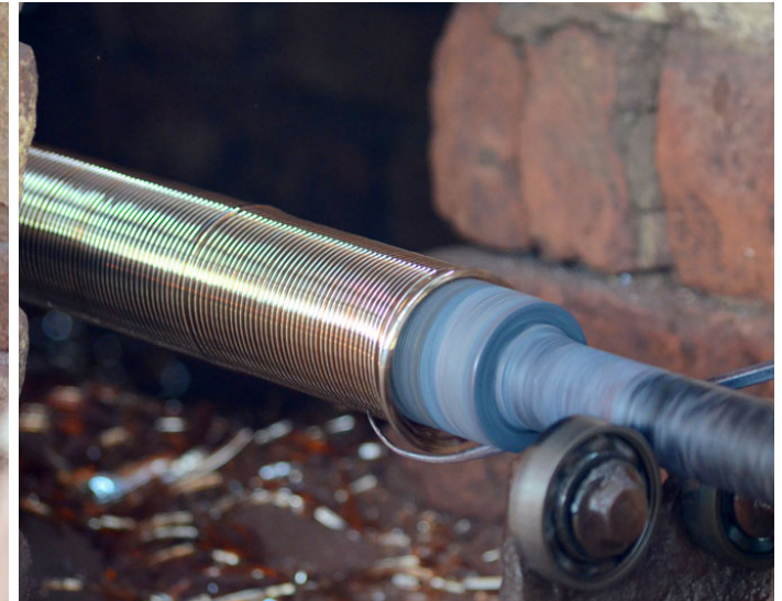
Since the rod is filled up, the bangles are being removed. Since the rod is filled up, the bangles are being removed.
