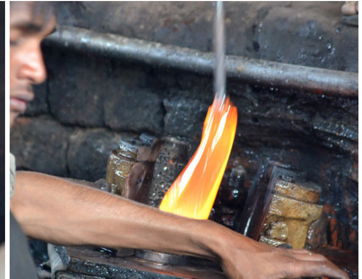
Gob falling by gravity in the mould.
