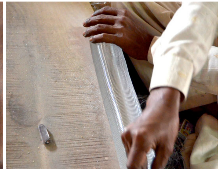
The coil being cut using a diamond cutter, separating the bangles from each other.
