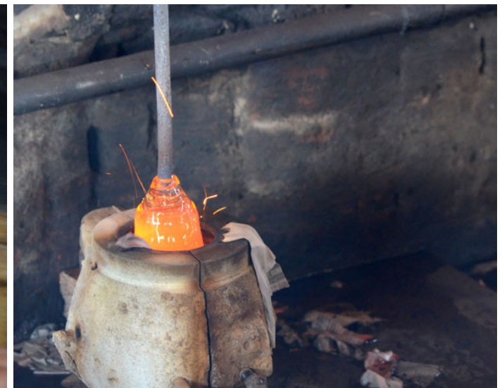
Glass takes the shape of the mould while air is being blown from the other end.
