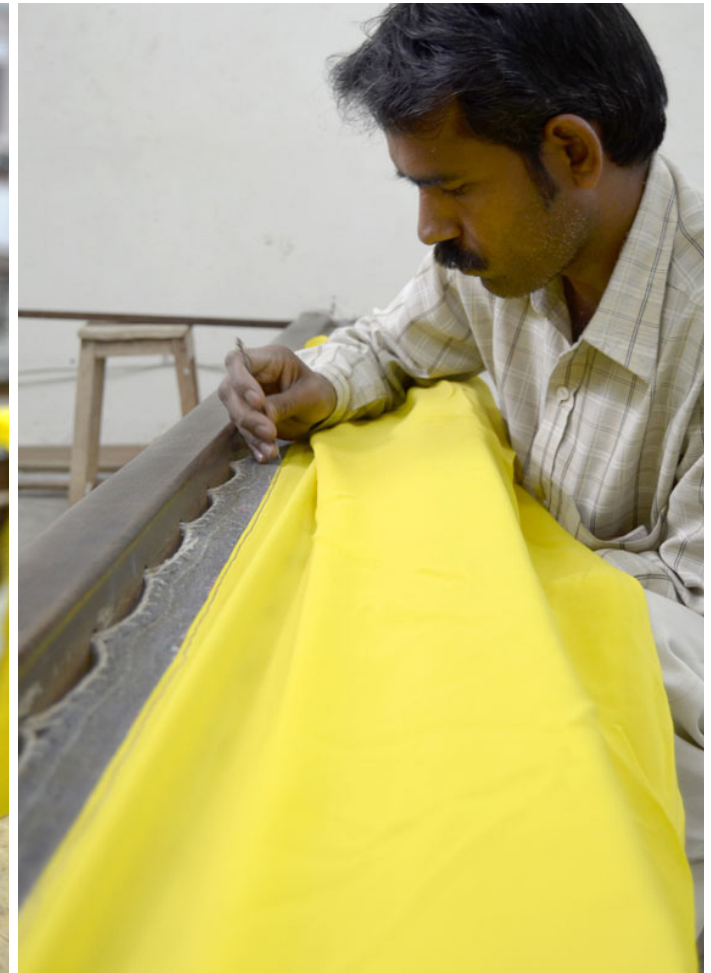
Fabric being tied to two sides of a wooden frame (known as 'khaat') using thick cords.
