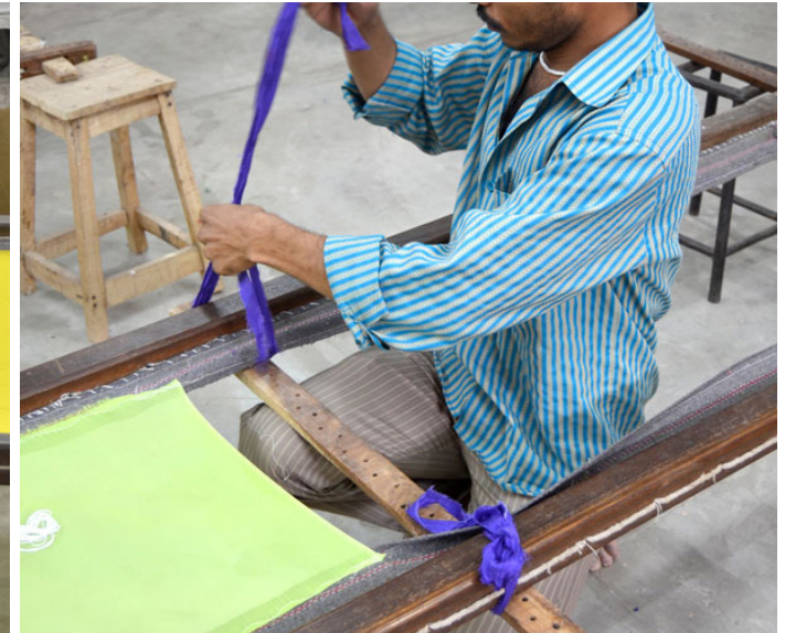
Fabric being tied to two sides of a wooden frame (known as 'khaat') using thick cords.
