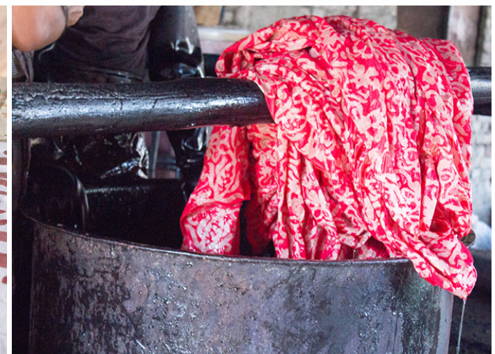
Fabric is getting dyed in a chemical color solution.
