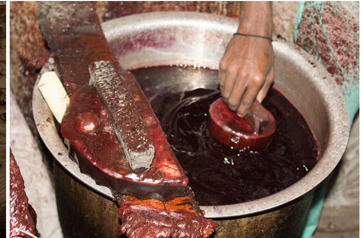
Wooden block is dipped in the molten wax color to be printed on the fabric.
