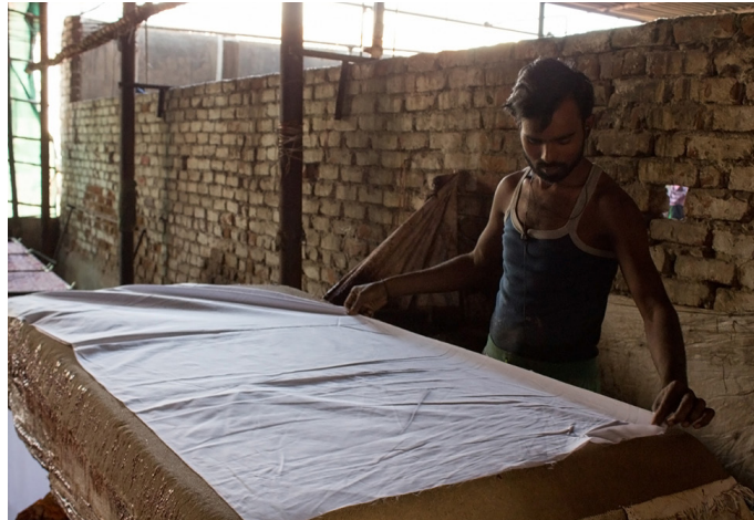
Fabric is evenly spread on a table before printing.
