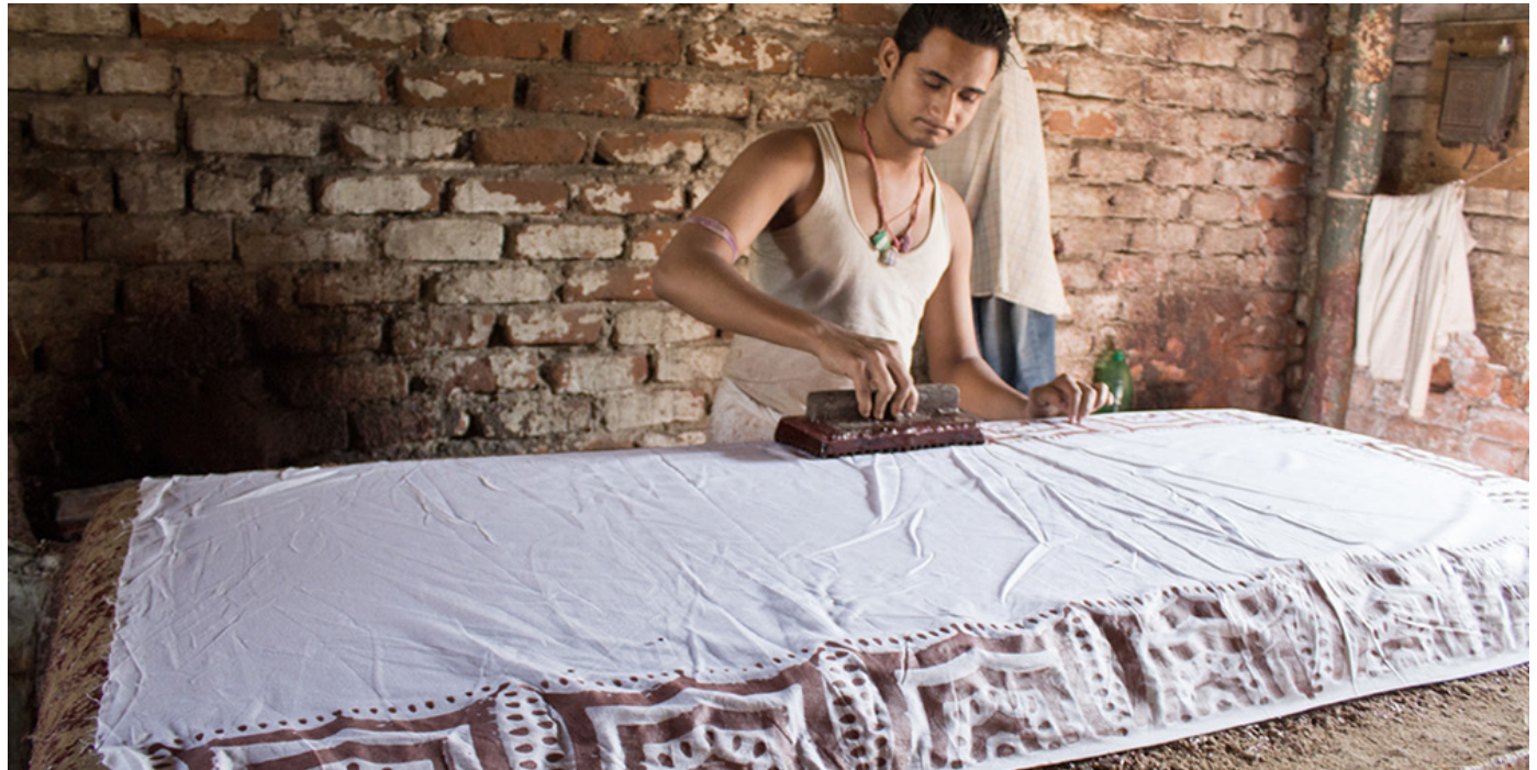
Artisan carefully placing the wooden block to print on the cloth.
