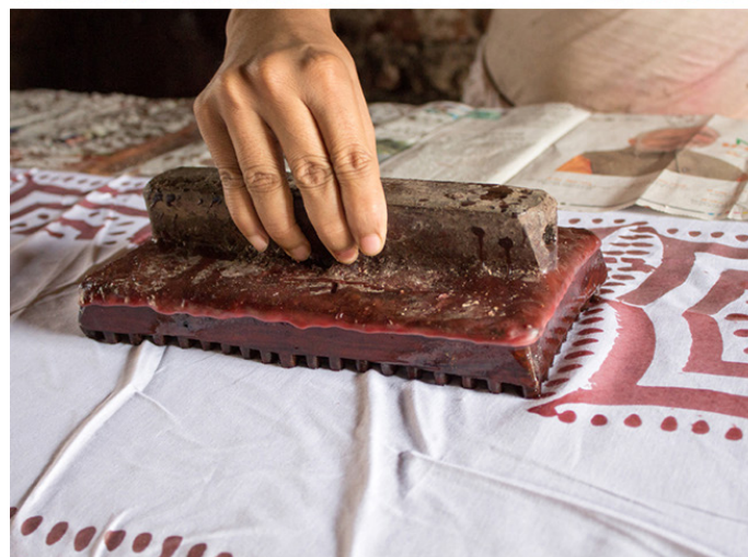
Artisan printing the design pattern on fabric.
