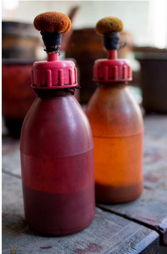
Bottle sponge applicator used to color on the fabric.
